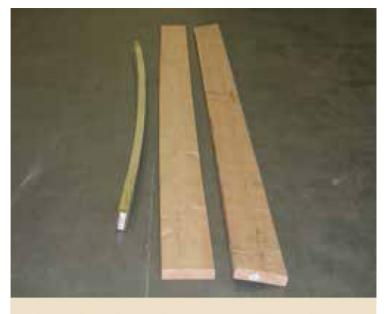
Examples of wood movement due to drying out
