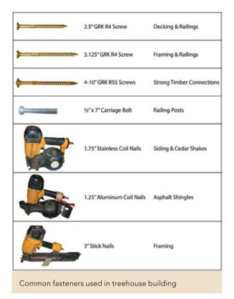
out as wood seasonally shrinks and expands. Nails are ideal fasteners for wall sheathing because the primary function of sheathing is to hold the wall studs perfectly plumb and keep the wall square. Some fasteners are hybrids, such as ring-shanked nails with increased pullout resistance and timber bolt screws with increased shear strength. The important *safe building skill* is to choose the type of fastener most appropriate for its application.
