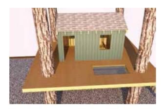
This siding is T 1-11 plywood, which is graded for exterior exposure. I strongly suggest staining it for looks and better weathering. It can be installed with minimum 2-inch screws or with ring shank nails. Irregular cedar shakes are shown here on the roof, which can be installed over plywood or lath.
