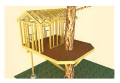
We suggest framing all the walls on the ground and lifting them into position with the help of a friend or hoist system. However, if you
