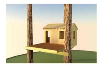
Install the wall and roof sheathing, as well as your roof felt. If your treehouse will not get a finished interior, then consider using two layers of roof sheathing so nails don't stick down and show from the underside. If the roof is high out of reach, then this may not matter to you.
