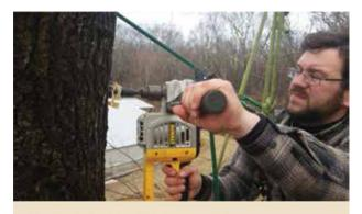
Start the hole with a 3-inch timber bit.
