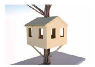
Install the wall and roof sheathing, as well as your roof felt. If your treehouse will not get a finished interior, then consider using two layers of roof sheathing so nails don't stick down and show from the underside. If the roof is high out of reach, then this may not matter to you.
