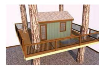
Install windows and doors and exterior trim on the building. Trim can be treated wood, cedar, or any material you have left over. Be creative and resourceful. The point of trim is just to cover the cut edges of siding material and the flanges from new construction windows.
