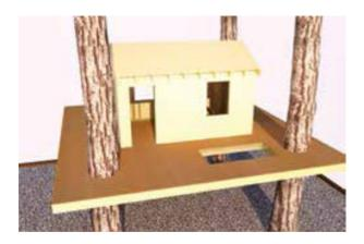
Install the wall and roof sheathing, as well as your roof felt. If your treehouse will not get a finished interior, then consider using two layers of roof sheathing so nails don't stick down and show from the underside. If the roof is high out of reach, then this may not matter to you. If you are not going to heat or air-condition the treehouse, then you might skip the wall sheathing and simply install the siding directly onto the wall frame.
