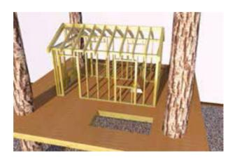
Normally I suggest framing all the walls on the ground and lifting them into position with the help of a friend or hoist system. However, with the size of this platform, the best place to frame the walls is right on the platform. Frame the window and door rough openings per the manufacturers' recommendations. Next, determine the pitch of the roof and the amount of overhang you want. Build your ridge and install it in place with temporary supports. Install the roof rafters.
