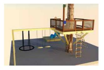
Install swing, rope ladder, cargo climb net, and slide. The swings can be tied around the beam with rope, but are more typically installed with pivoting swing hanger hardware. The spider swing is shown here in a double-rope configuration, which makes it swing back and forth only, but all four ropes can be joined at one spot to make it go in any direction, like a tire swing would.
