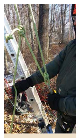
Double-rope system, with bowline attachment to harness and Blake's hitch
