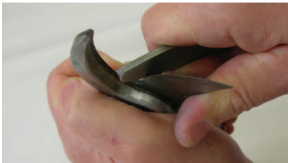
Figure 3.15 Burnish your blade to harden the cutting edge.
