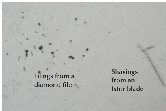
Figure 3.11 Files with embedded industrial diamonds are very effective, and produce fine filings (left). The Istor blade at the other end of this tool works like a carpenter's plane. It is used to rapidly reshape the edge of a worn and blunt blade (right).
