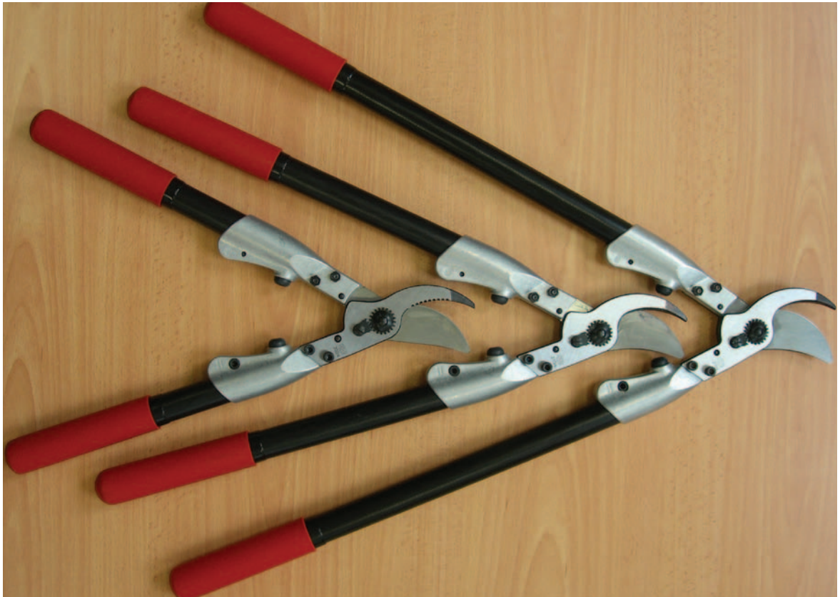
Figure 3.21 A range of loppers that can cut branches up to 35 mm in diameter. Generally the longer the handles the less strain on the pruner. The pair with the longest handles can cut branches up to 45 mm in diameter.
