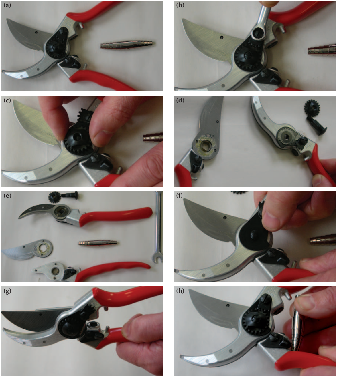
Figure 3.9 Maintaining your secateurs. First remove the spring (a). Loosen the screw that controls the central nut and bolt (b). Remove the nut from the central bolt (c). Take the secateurs apart (d). Clean and grease all the parts as required (e). Reassemble the secateurs (f). Before reinserting the spring, adjust the central nut so that the blade falls naturally to run against the by-pass blade for two-thirds of the blade's length (g). Re-insert the spring and check that the secateurs run smoothly. Adjust the central nut as required (h).
