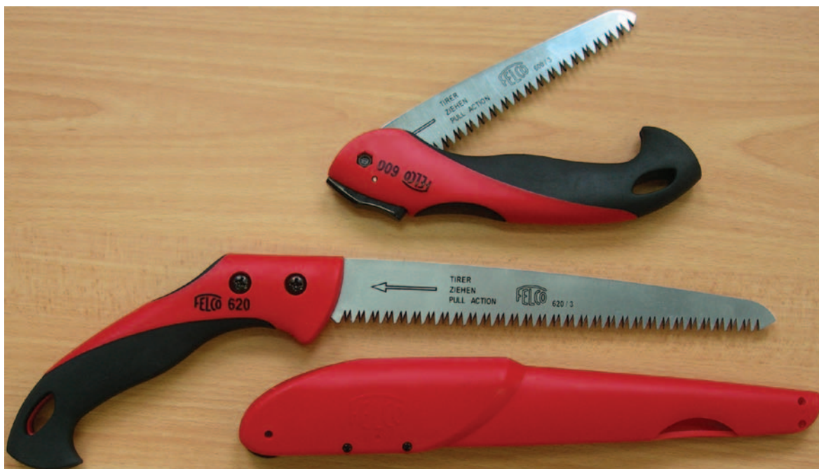
Figure 3.22 Smaller folding saws are easy to carry around safely and can cut branches up to 50 mm in diameter (1). Longer pruning saws that come with a scabbard and belt loop are ideal for branches up to 80 mm in diameter (2).
