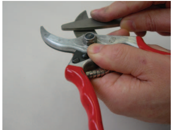
Figure 3.16 Make sure you remove the burr on the flat side of the blade.
