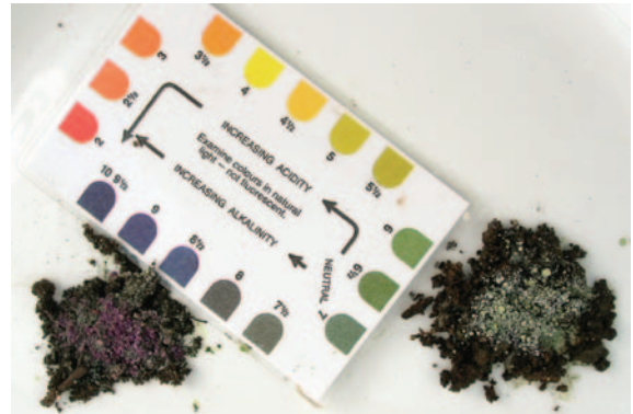
Figure 1.12 pH testing kits are freely available and easy to use. The soil on the left is alkaline (pH 9). The soil on the right is acid to neutral (pH 6).
