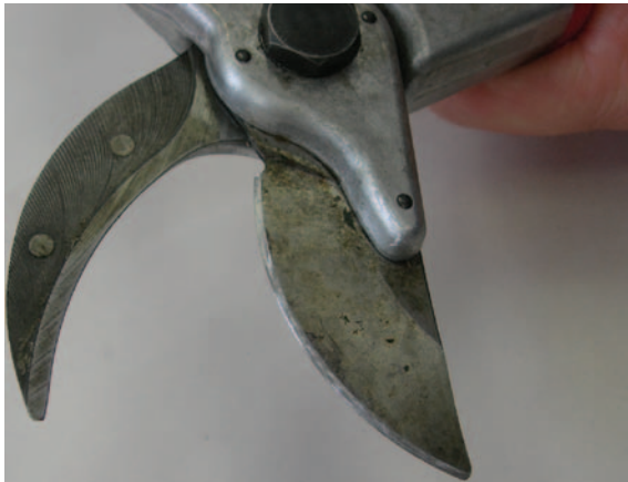
Figure 3.14 When the blade is shiny the whole length of the blade's bevel it should be evenly sharp.
