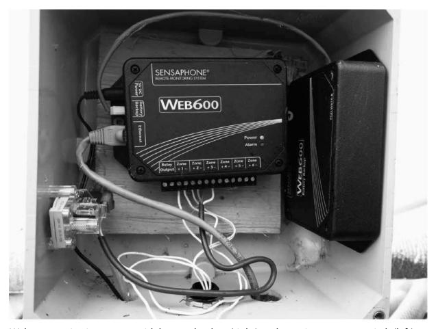
Web600 monitoring system with battery backup (right) and aeration pressure switch (left).
