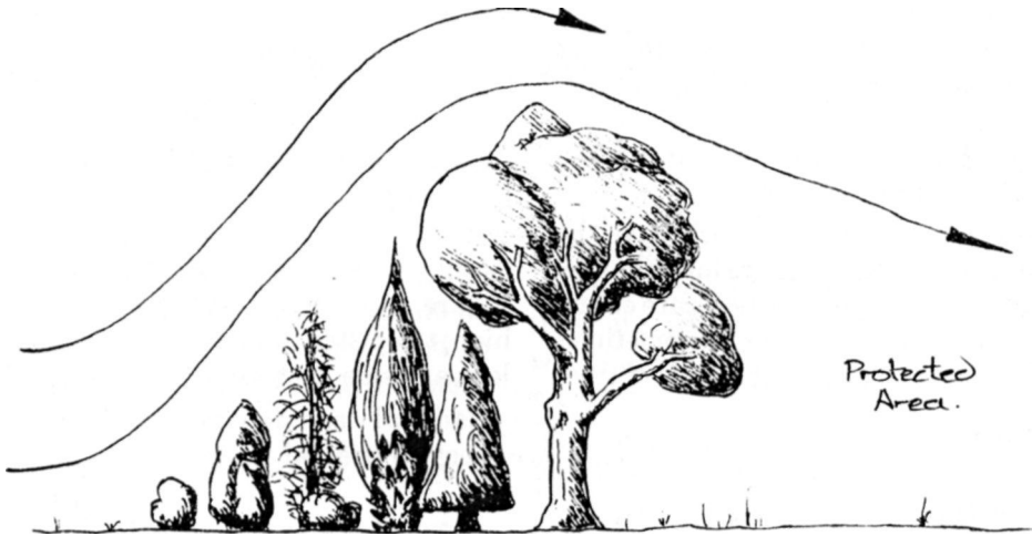
Figure 11.4 Windbreaks are used to deflect wind upwards.
