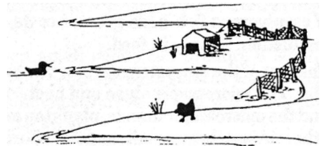
Figure 2.16 Fingers of land surrounded by water can be economically and easily fenced to reduce the impact of unwanted predators.
