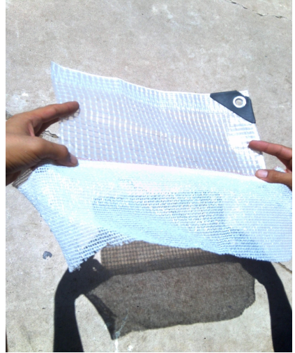
The top covering is a piece of the clear reinforced tarp and the bottom piece is the white shade-cloth we use.
