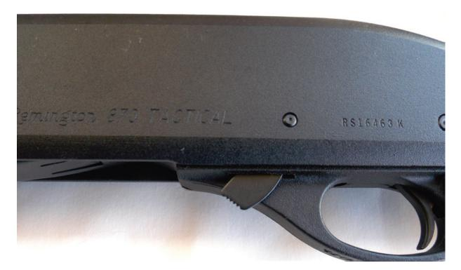
Remington uses a lever by the triggerguard to unlock the bolt.
