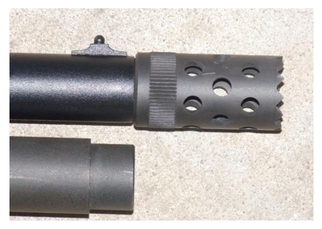
Remington's Express Tactical uses a muzzle brake that is also a choke tube, a nice touch in an inexpensive shotgun.
