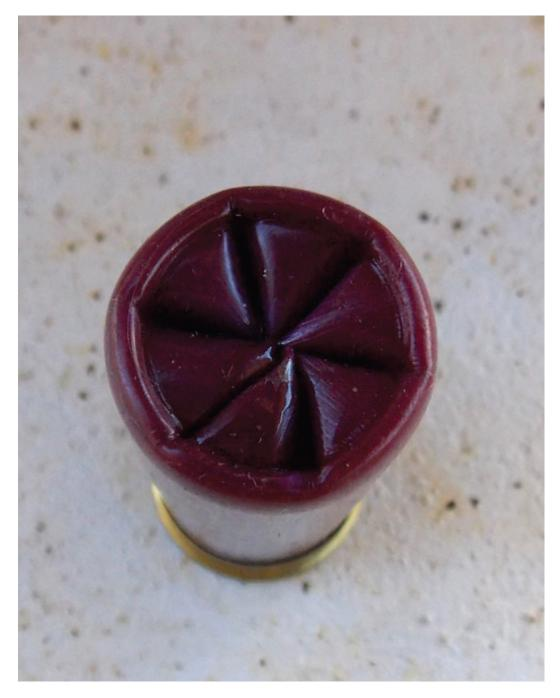
This is the now universal roll-and-fold crimp used with shotgun shells.
