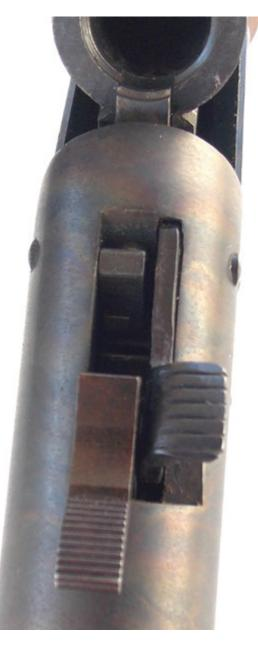
Note the transfer bar safety of the H&R shotgun.
