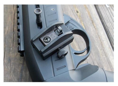
When using aperture sights, the type that are tightened onto a rail should be checked often. These fell off the Tec-12 during a training session.
