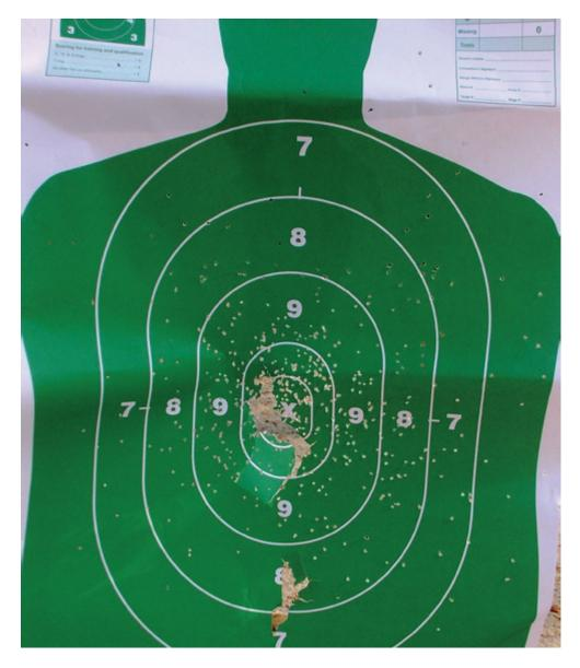
As range increases, so does the size of the pattern. The large holes are torn by the spent wad following the shot payload.
