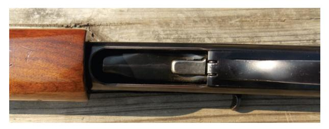
The Remington 1100 bolt release is located in the magazine well.
