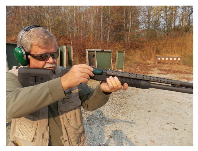
The pump-action may be chamber-loaded if desired, rather than racking the action to shift a round from the magazine up into the chamber.
