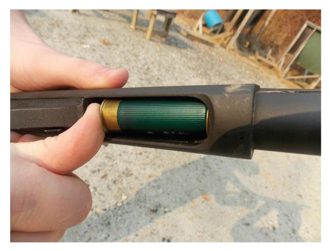
Shells are thumbed into the magazine one at a time.
