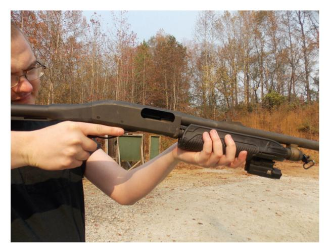
In this illustration, the pump-action is racked to the rear and the action is open, bolt to the rear.
