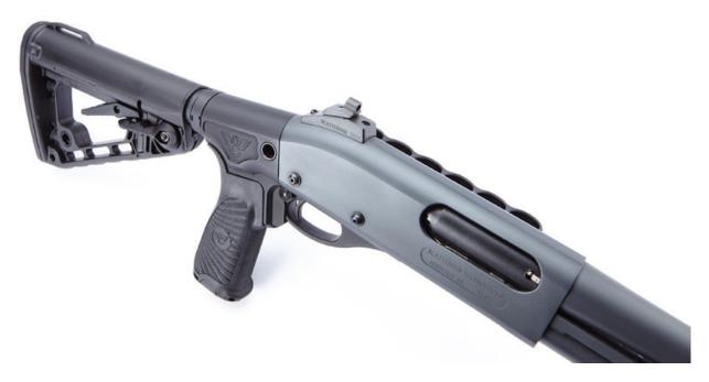
The Wilson Combat shell carrier, aperture sights, and adjustable stock are hallmarks of the modern tactical shotgun.
