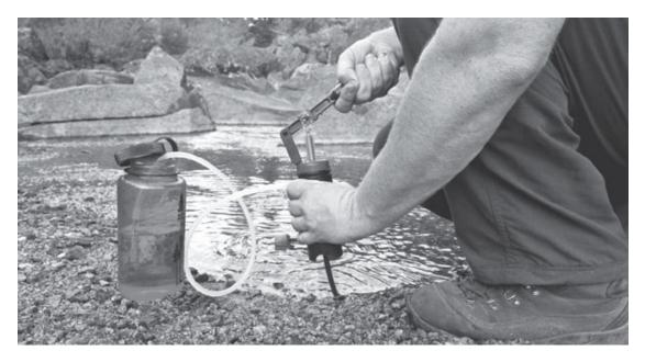
Water filtration pumps can clean up almost any water source, but it's best to use the cleanest water available.
