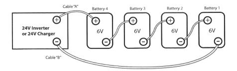
This diagram shows a single string connected for 24 volts. Adding a second identical string in parallel gives us our maximum storage.
