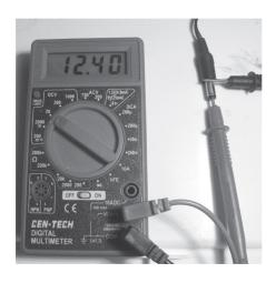
Checking the voltage of the plug
