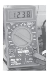
Voltmeter showing battery voltage reading
