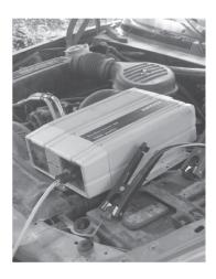
Inverter cables connected to car battery
