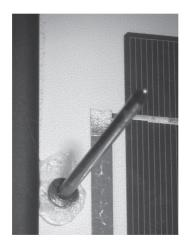
An example of using the nail test to correctly angle a panel
