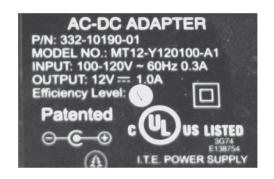
Look at the line that starts with "output." See the "12V"? That means that this power pack takes the 120 volts AC from the wall and converts it to 12 volts for the device it powers. Notice that little symbol next to the 12V with the solid line over the dashed line. That symbol means the 12 volts is *direct* current, not alternating. And finally, the "1.0A" means it can provide a maximum of 1.0 amps.
