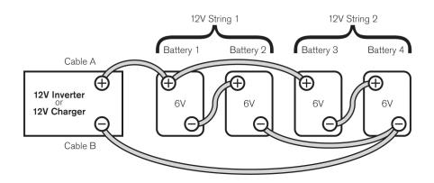
Battery bank wiring example
