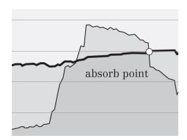
This graph shows battery voltage and charging current. The dark line on the graph represents the battery's voltage and the lighter line represents its charging current. The absorb point is when the voltage stops climbing and levels off and the current starts to drop. On a side note, this graph comes from our charge controller's ability to connect to the Internet to log its data.
