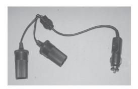
Cut the wire as close as possible to the male plug. You will end up with a bunch of female sockets on short wires. Strip back the insulation and connect the two wires inside to the same type of replacement AC plug that you used for the wall warts and power packs.
