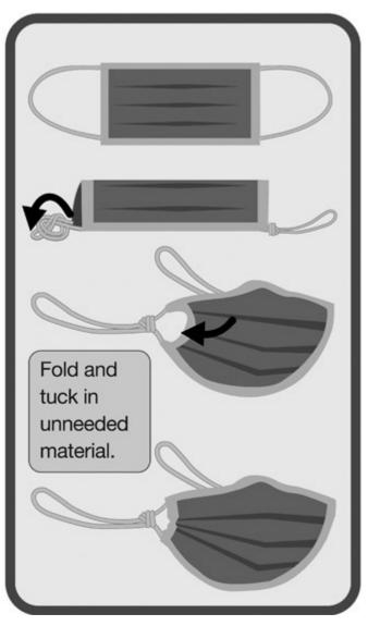
An illustration of the technique described in the YouTube video. The ear loops are knotted, then the crimped material is folded and tucked in.
