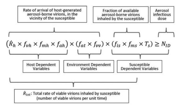
$T_s$  represents the duration of exposure of a susceptible person to the aerosols from the host, and  $N_{ID}$  represents the minimum number of inhaled virions required to initiate an infection in the susceptible.
