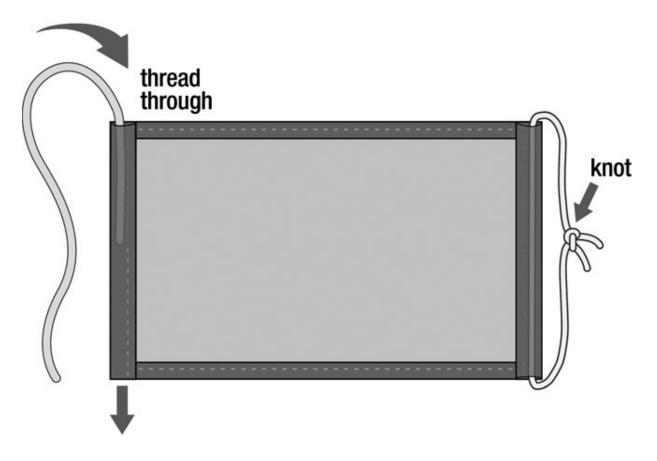
**Step 4:** Gently pull on the elastic so that the knots are tucked inside the hem. Gather the sides of the face covering on the elastic and adjust so it fits your face. Then securely stitch the elastic in place to keep it from slipping.
