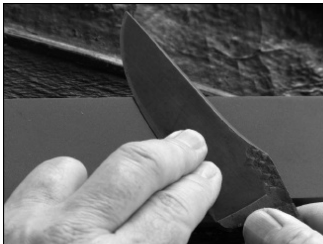
Sharpening a convex edge by drawing away from the edge.
