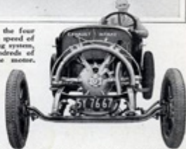
A front view, showing how the compressed air engine is mounted. An electric heater, operated by a battery and generator, heats the air until it attains a pressure of 200 lbs. As the warm air goes through the engine and is cooled, it is recovered and drawn into a compressing chamber, where it is heated again and returned to the tank.
