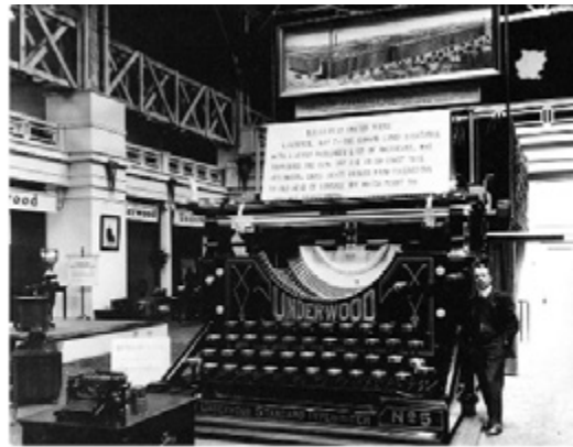
The gigantic Underwood on display in the Palace of Liberal Arts was operated using an ordinary-sized typewriter.
