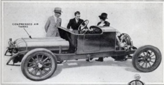
A side view of the compressed air car, showing the four fuel tanks which will drive the car 500 miles at a speed of 15 miles an hour. The engine requires no cooling system, no ignition system, no carburetor, nor the hundreds of moving parts included in a standard gasoline motor.
