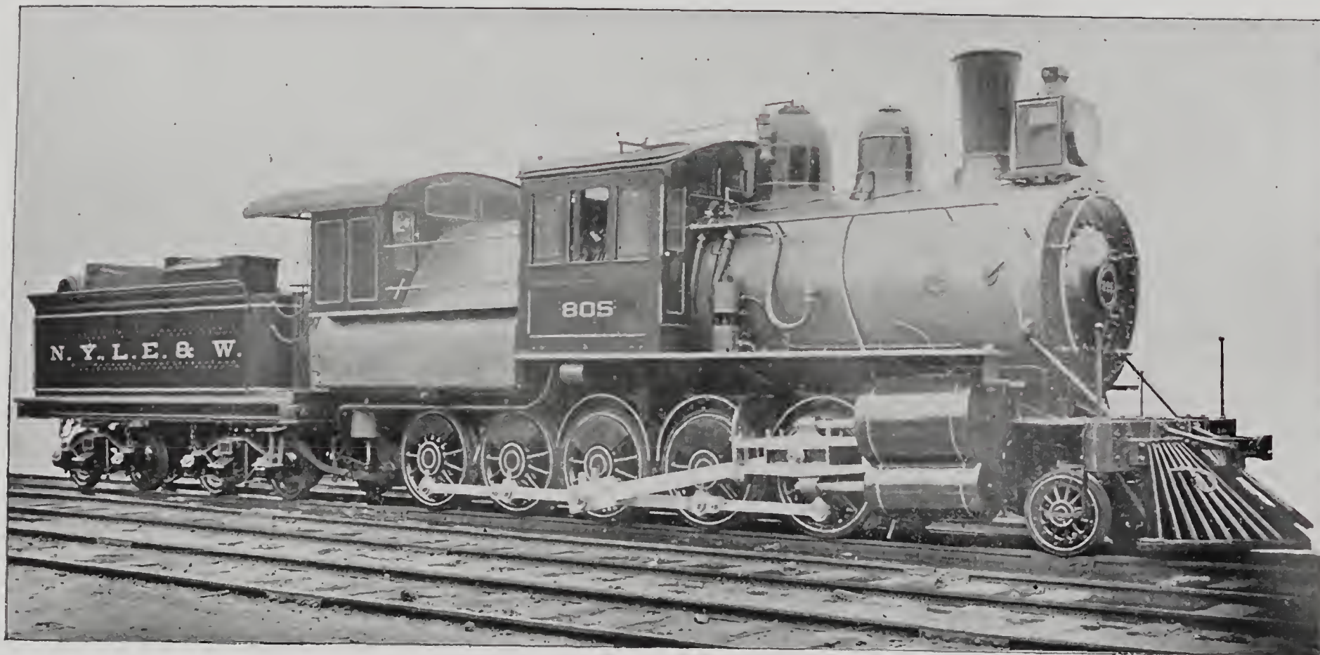
COMPOUND FREIGHT LOCOMOTIVE, "DECAPOD" TYPE. WEIGHT, 195,000 LBS. ( Exhibit of Baldwin Locomotive Works. )
