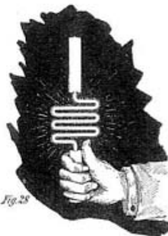
FIG. 28.—INCANDESCENCE OR PHOSPHORESCENCE OF RAREFIED GAS.—ILLUSTRATING FOUR KINDS OF LIGHT EFFECTS PRODUCED BY HIGH FREQUENCY CURRENTS OF HIGH POTENTIAL.
