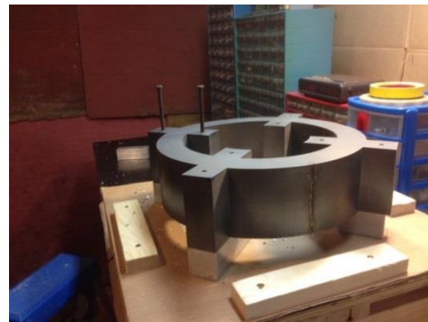
Welded lamination stack
