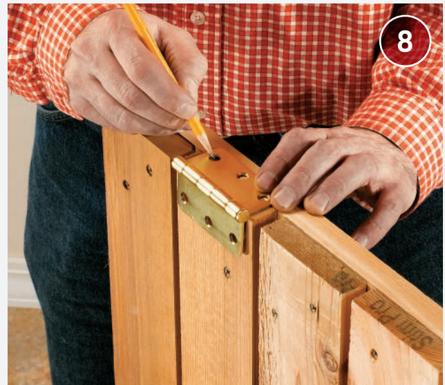
Hang the door and install hardware. Fasten the door hinges to the door (or doors if you choose to cover each opening) and then attach the door to the cart frame. Use a \frac{1}{4} " spacer under the door to position it.
