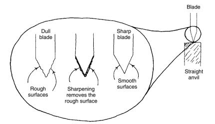
**FIGURE 6-2.** The two pruner types should be sharpened in different ways. The bypass (scissors) type must be sharpened only on the side of the blade facing away from the anvil. If it is sharpened on the anvil side, branches will bind and become stuck between the blade and anvil, causing the pruners to work incorrectly. On the other hand, the straight-anvil type blade should be sharpened evenly on both sides of the cutting blade. A fine sharpening stone works best to sharpen pruners.
