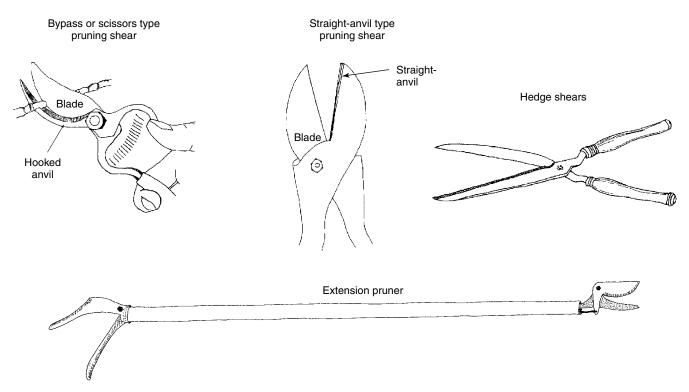
**FIGURE 6-1.** Pruning tools come in a variety of styles. The bypass type (left) is best for pruning live branches less than ½ inch in diameter. Hedge shears are suited for trees, and shrubs maintained as hedges; they are also used to shorten lower temporary branches in the tree nursery. Extension pruners are useful for reaching the upper canopy of nursery trees and for pruning shrubs in the landscape.
