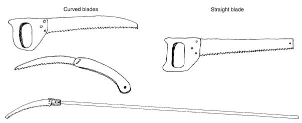
**FIGURE 6-3.** Saws with curved blades (left) cut on the pull stroke. The teeth are usually angled back toward the handle end of the saw. Many saws with a straight blade (right) cut on the push stroke. The handle on the straight-blade saw is designed to keep your hand in place as the saw is pushed through the wood. The newer, triple-sharp, Japanese-type blades cut entirely on the pull stroke, even when the blades are straight.
