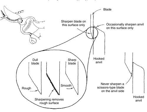
Sharpening a scissors type bypass pruner
