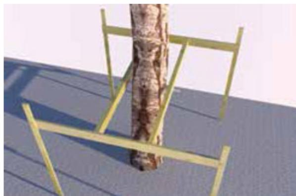
Attach your rim joists. Temporary 2x4 posts on the corners will help hold everything level while you work. If needed, you can detach one of the doubled joists from stage 2, slide it left or right a bit, and reattach. It's worth the time to make sure you build the structure square (not a parallelogram) and that it is centered on the tree trunk.
