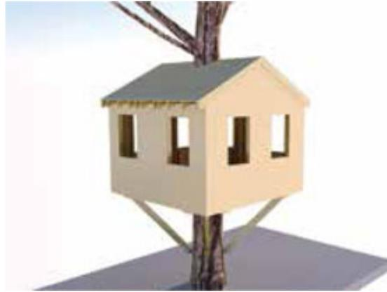
Install the wall and roof sheathing, as well as your roof felt. If your treehouse will not get a finished interior, then consider using two layers of roof sheathing so nails don't stick down and show from the underside. If the roof is high out of reach, then this may not matter to you.
