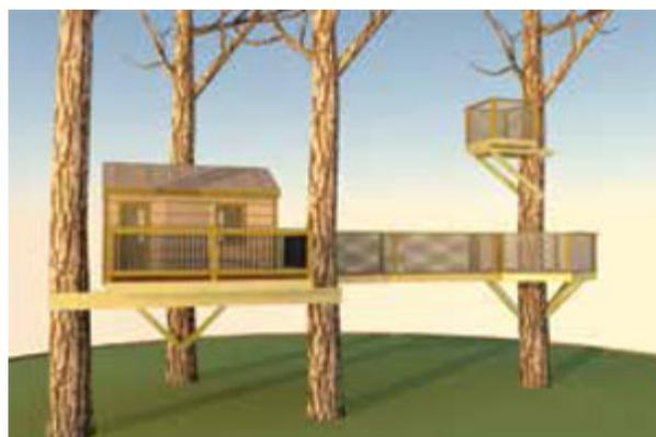
This project uses some black aluminum spindles on the main treehouse and netting railings everywhere else. Netting is flexible and so is the best choice for flexible bridge styles. We connect
