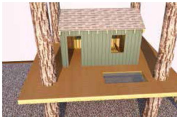
This siding is T 1-11 plywood, which is graded for exterior exposure. I strongly suggest staining it for looks and better weathering. It can
