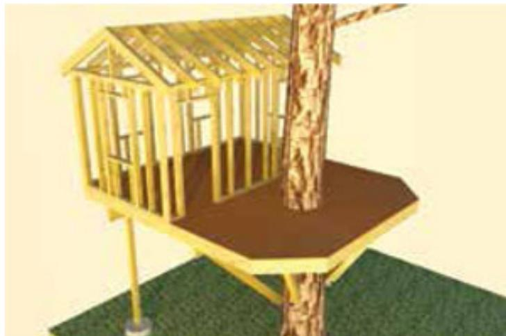
We suggest framing all the walls on the ground and lifting them into position with the help of a friend or hoist system. However, if you
