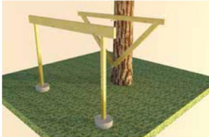
Lay out and build your concrete footings to support the 6x6 posts and beam. Carefully use a laser, water level, or regular spirit level to notch the posts for the beam to ensure that the top of the tribeam is level with the top of the beam on the two posts. Important: Check your local codes to determine footing size/depth. For a 10x10 single-story treehouse, a double 2x12 beam should be sufficient, or a double 2x8 beam with properly connected angle braces to shorten the span.
