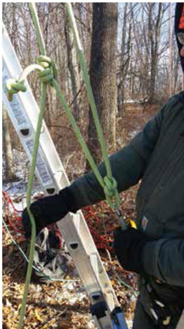
Double-rope system, with bowline attachment to harness and Blake's hitch
