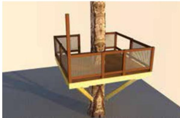
Cut 4x4 posts at a work station on the ground, and then install them as desired. Normal post spacing is 3 to 6 inches apart, with 2x4 rails running horizontally. I always start by identifying which accessories and access points I want to have, because each of these requires a post on either side. In this case, we have a rope ladder, a cargo net, and a slide. The opening size for the rope ladder and slide should be
