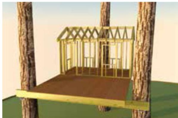
We suggest framing all the walls on the ground and lifting them into position with the help of a friend or hoist system. However, if you don't have a flat spot on the ground, and the platform is large enough, then it may prove easier to frame the wall lying flat up on your completed platform. Frame the window and door rough
