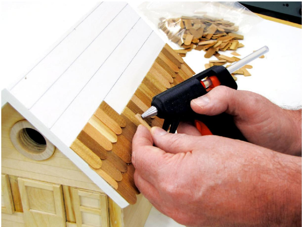
**Figure 9** *I opted for hot-melt glue, which not only makes the job of hanging shingles much faster, it's far easier to remove a damaged shingle and replace it.*
