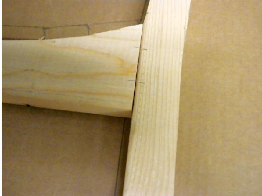
**Step Seven** *I secured the clamping blocks to the work surface with screws that I drove in from the underside. I suggest working one curve at a time. As the blocks go into place, they can be used to hold the strip in position and then you can move onto the next spot that needs to be supported.*
