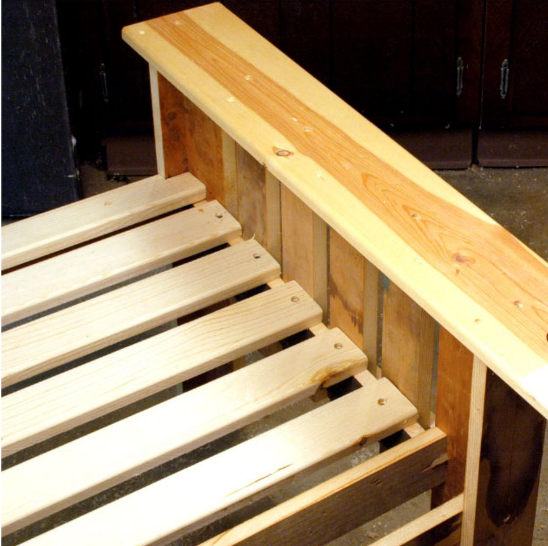
**Step 21** *The rest of the seat slats are screwed into the seat supports on either side. The two arms are also rounded with the router, then screwed in place.*
