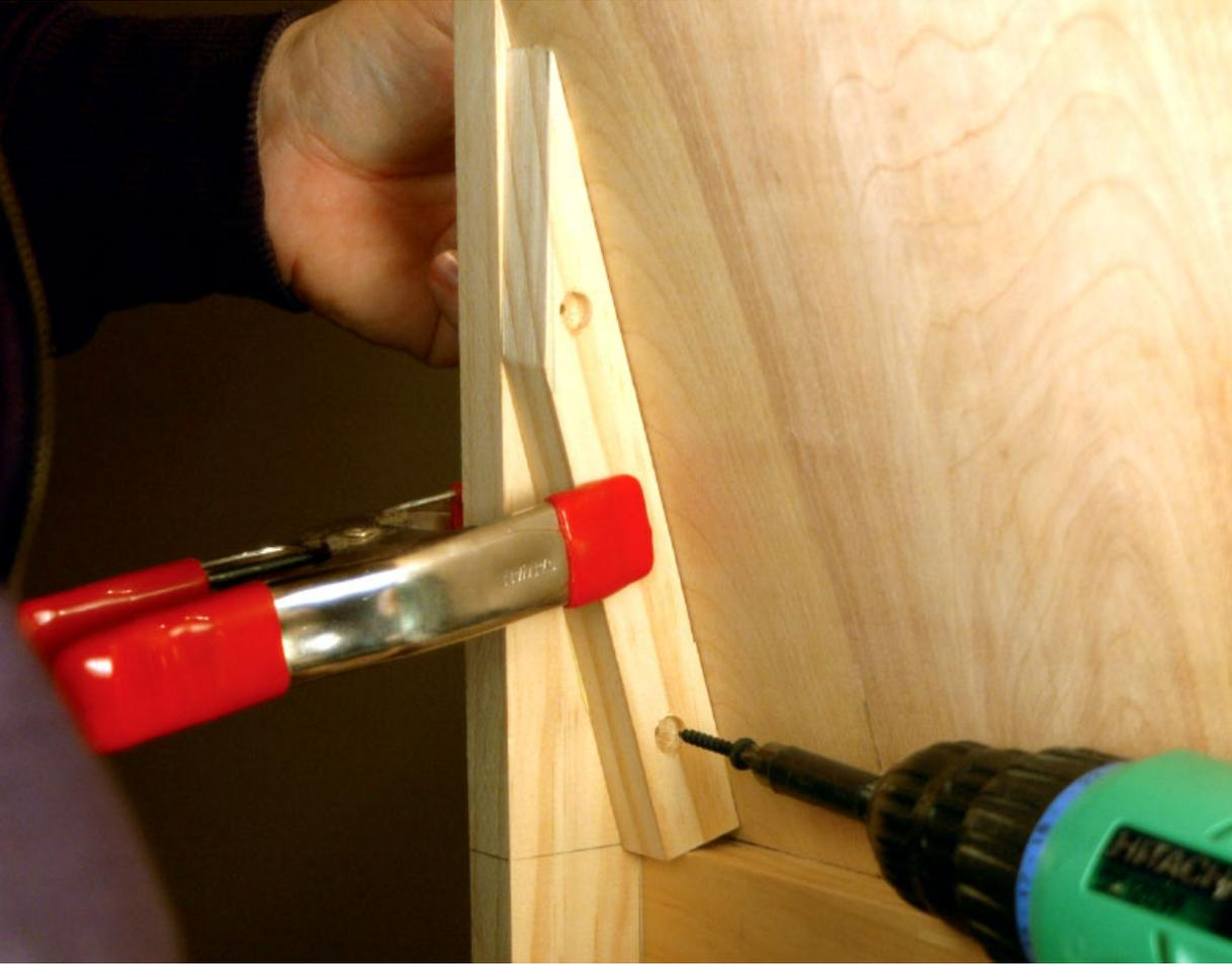
**Step 17** *Some glue, a spring clamp and a couple of screws (in countersunk holes) added the braces and made the back much stronger.*
