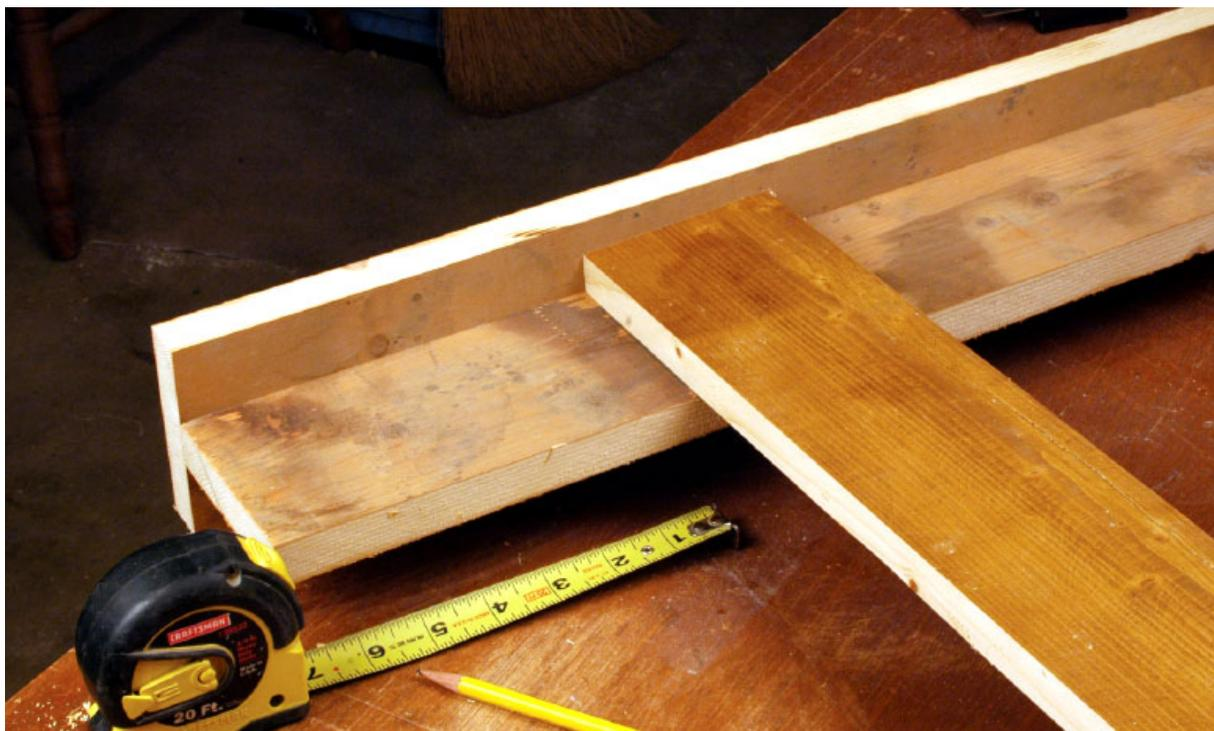
**Step Seven** The lower side stretchers are located up 7" from the bottom of each leg.
