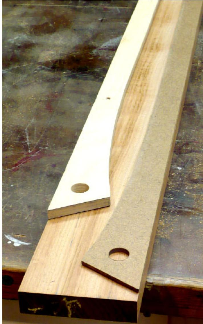
*Start with a blank. A 6"-wide blank is ideal for laying out the slats so you can nest the parts.*
