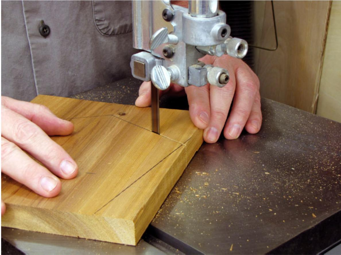
**Figure 2** Use a band saw or jigsaw to cut out the ends.
