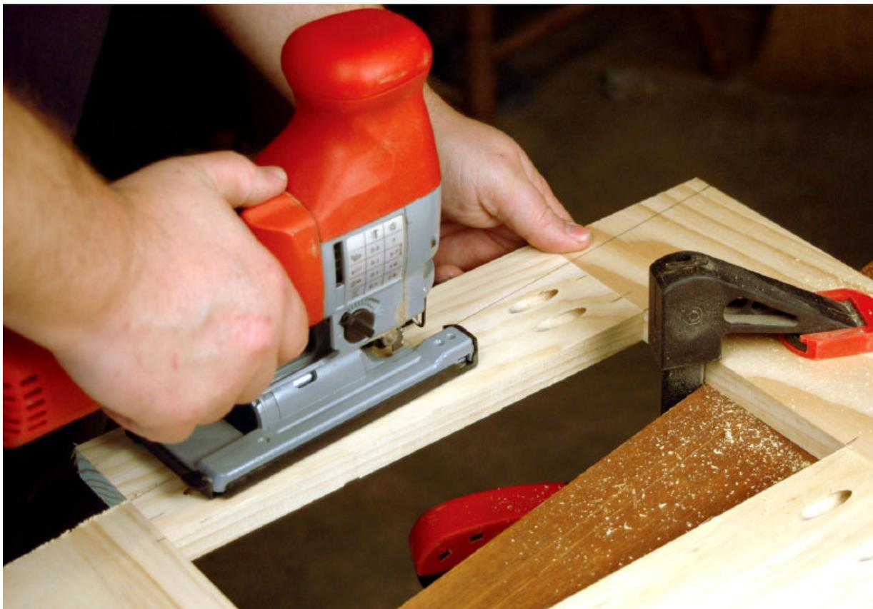
**Step Five** *I used my jigsaw to cut each slope, staying slightly proud of the line, and then cleaned up the edge with my bench plane.*
