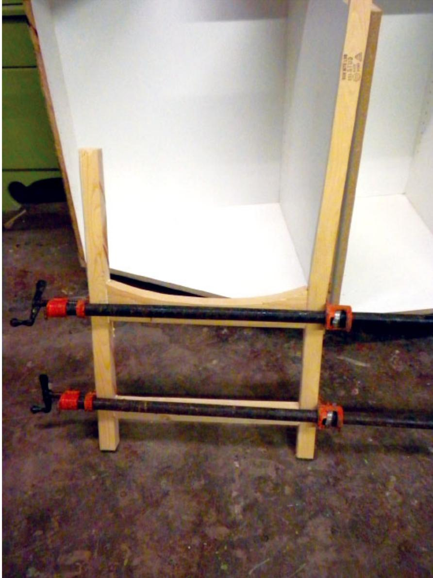
**Step Four** *The strips that I used for this lamination were 8', which was about 18" longer than I needed. I simply let the excess shoot out at the top. It will be trimmed later.*
