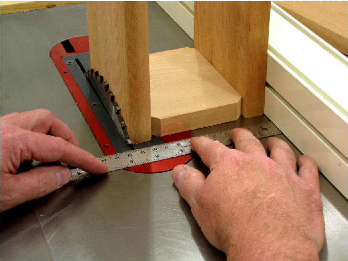
**Figure 2** Here's an easy way to adjust the fence on your table saw for cutting the front and back parts to width.
