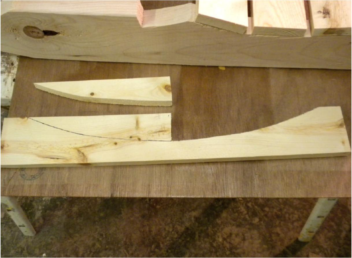
**Step Four** *Using a band saw or jigsaw, I cut along this line and remove the excess by cutting down the middle and then using this “waste” piece as a pattern for the other half of the cut. This ensures that the entire curve is at least symmetrical.*
