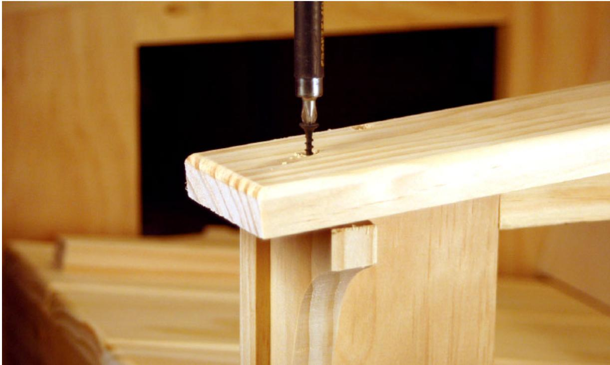
**Step 22** *Now screw down through the arm and into the top of the corbel.*
