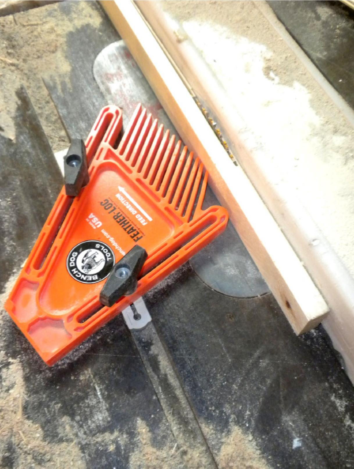
**Step Two** I suggest using a featherboard to keep the workpieces from wandering and producing non-standard strips.
