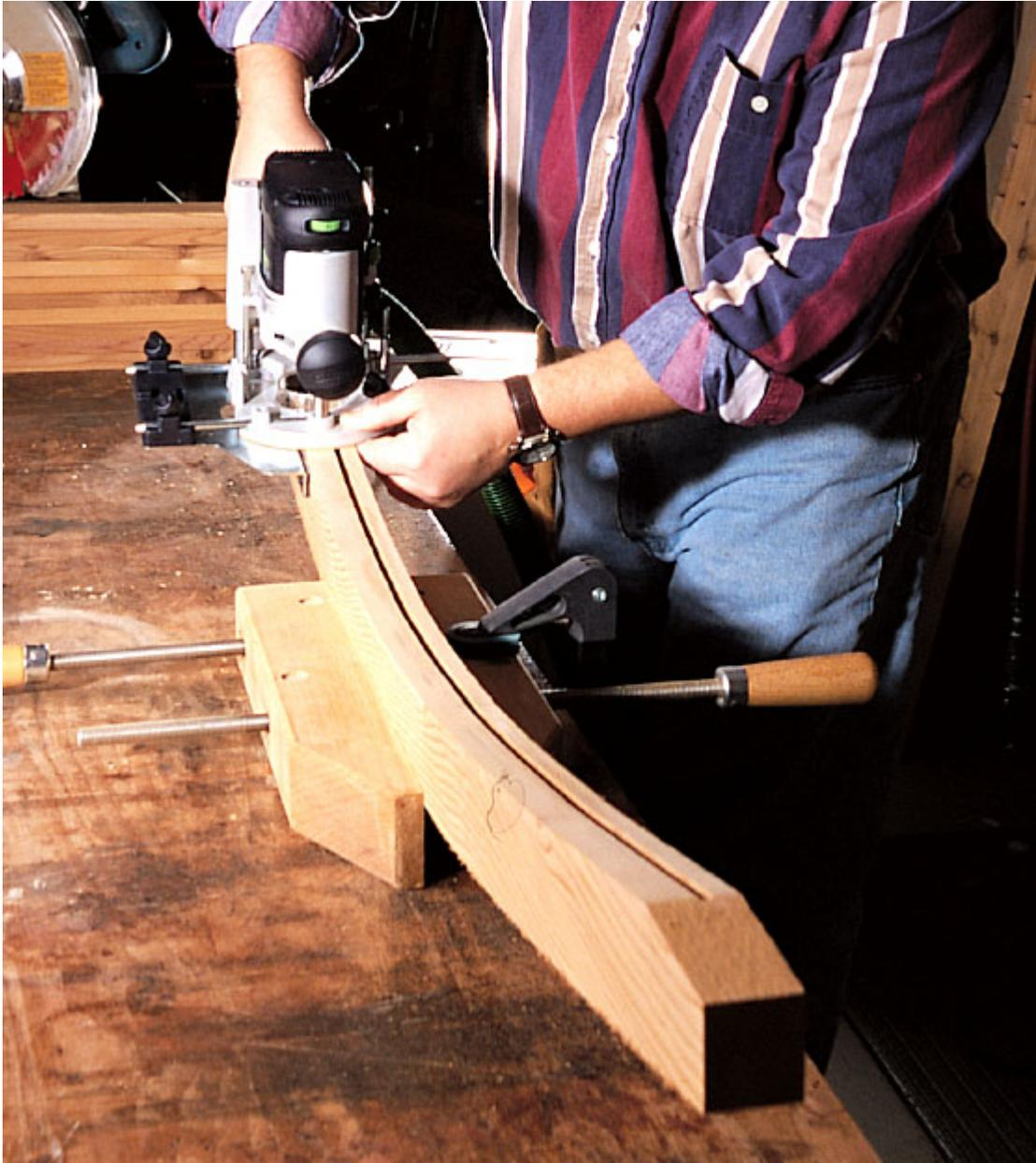
*Holding the arched top rail steady was the most difficult part of routing the top groove for the slats. Remember to make the cut in two passes on each side. In this photo you can see that the rail hasn't been cut for length yet, allowing extra support for the router at the beginning and end of the cut.*
