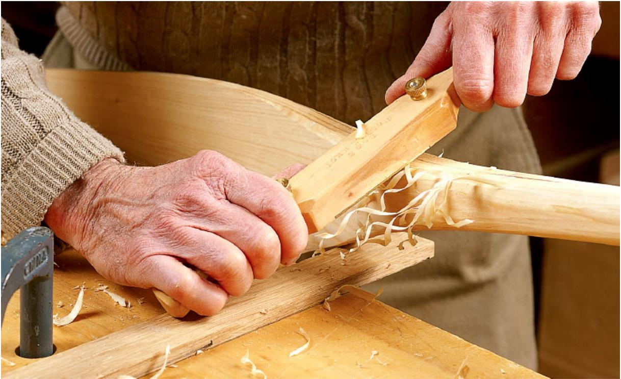
*The spokeshave (I'm using a wooden one here) is used to smooth the transition between blade, shaft and handle. It works pulling or pushing to follow the direction of the grain.*
