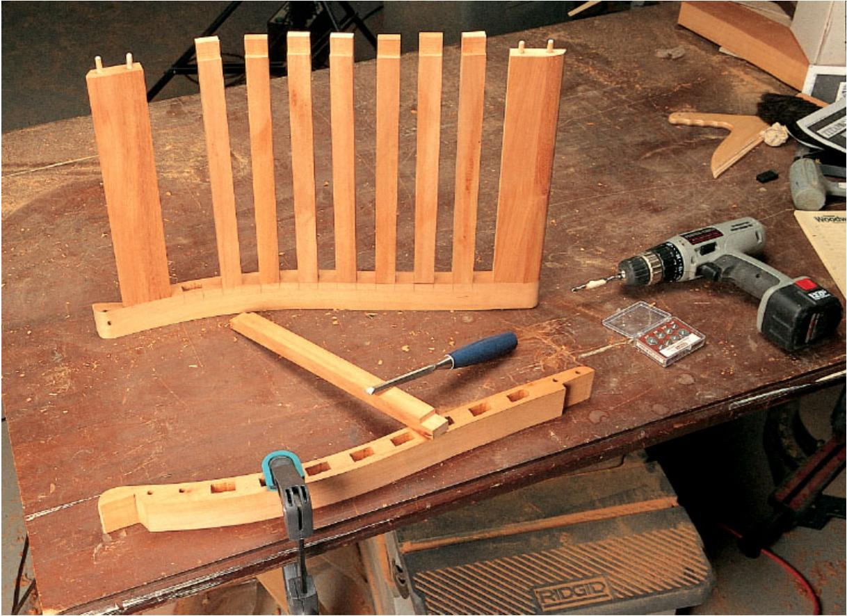
**Step Four** *With the mortises cut in the seat sides, assemble the seat and sand the surfaces flush and smooth. The seat remains loose and is screwed to the frame.*
