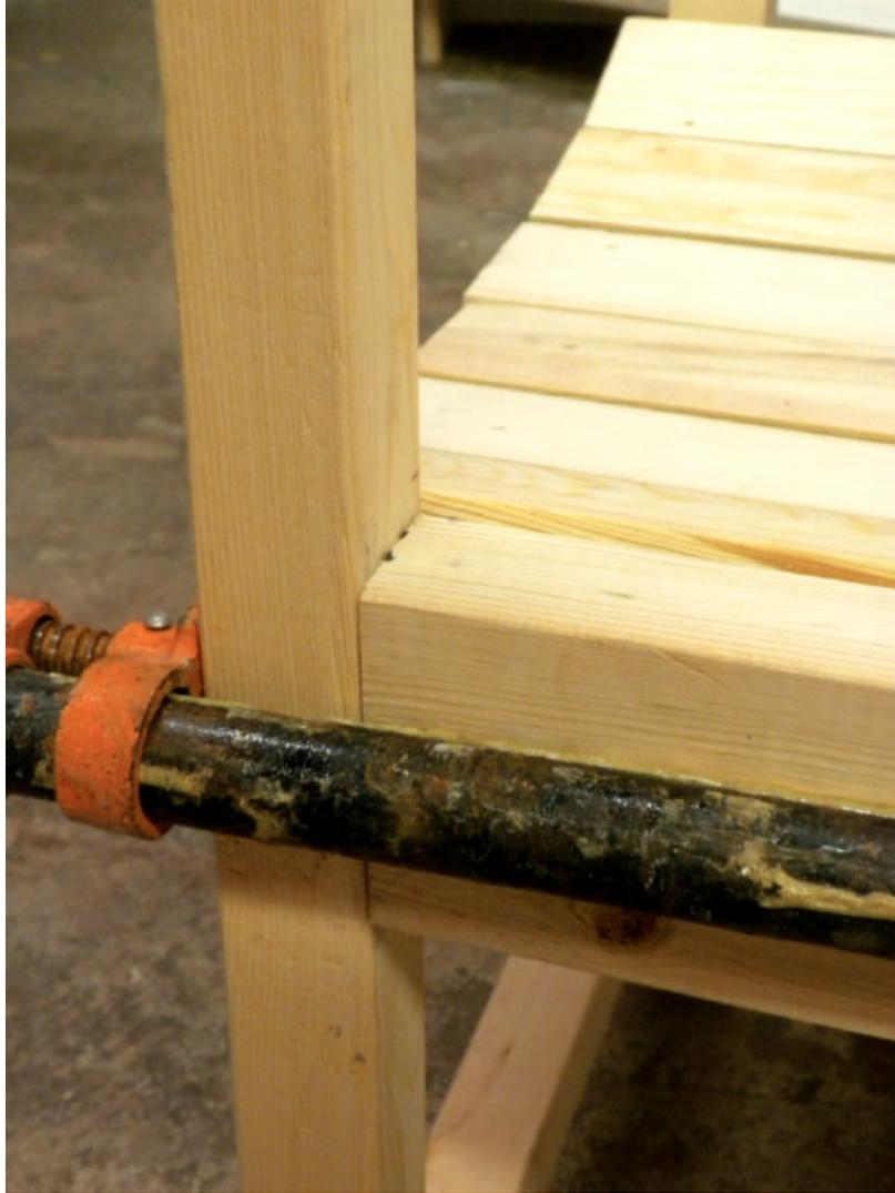
**Step Ten** *Two clamps are sufficient to ensure good, even clamping pressure. I used a 2×4 stretcher at the front of the bench to join the sides—this may be overkill, but it provides a lot of rigidity. I also added an identical one to the back of the bench.*
