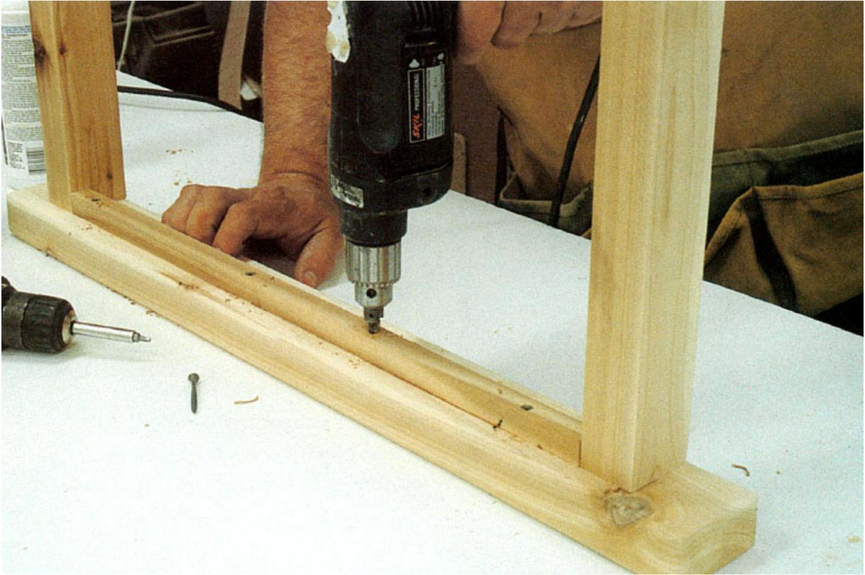
**Step Nine** *The two back support cleats (J) run between the back cross braces (H). Attach them with glue and 2" screws, flush with the upper edge of the braces.*
