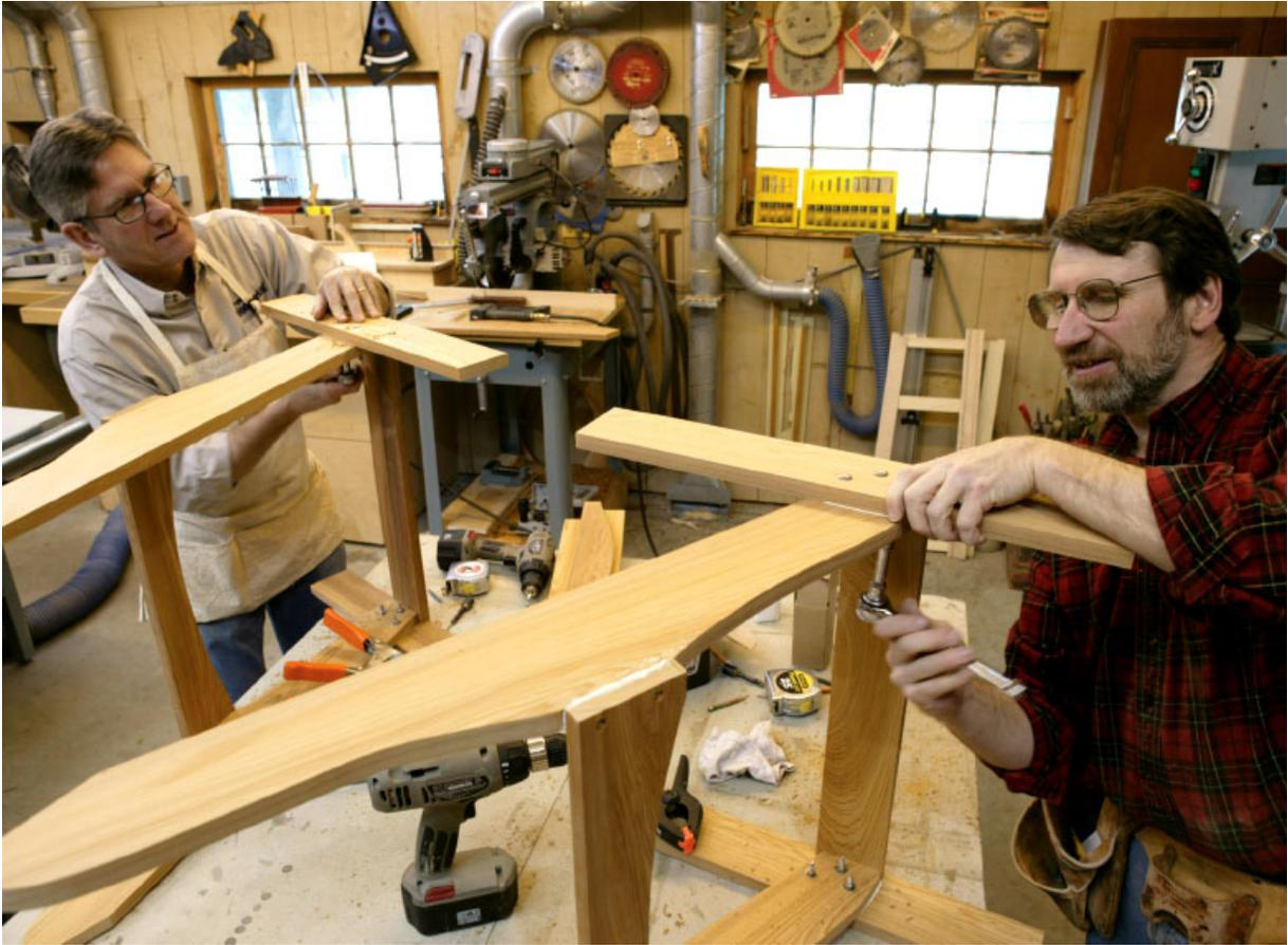
*Bolt the legs and side members together, bolt head to the outside with a nut and flat washer inside. Seat the square shank below the head with a hammer blow. The shank will prevent the bolt from turning in the hole.*
