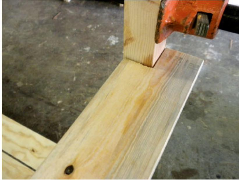
**Step 12** Some of the clamps were used to anchor the lamination to the blocks, while others served to apply pressure to the lamination alone.
