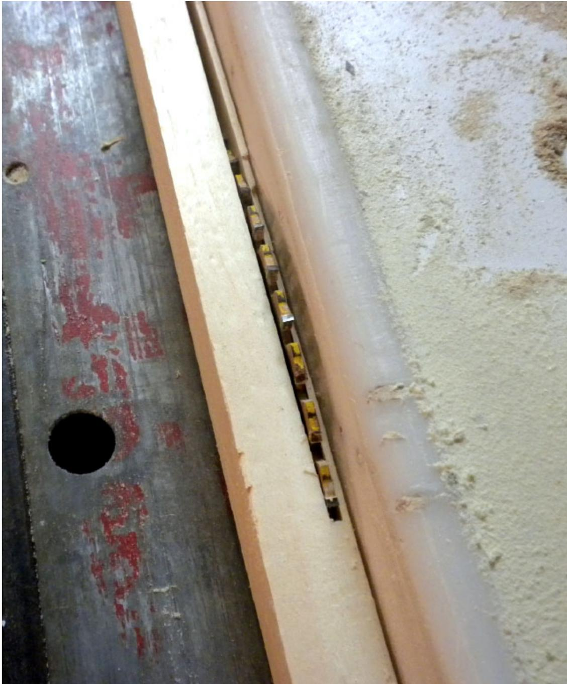
**Step One** To create the laminations for the sides of the bench, I needed 11 strips, slightly thinner than  $\frac{1}{8}$ ", per side to create a  $1\frac{1}{2}$ " thick component. I cut almost thirty strips to get 22 usable ones, and the easiest way to do this is to set the fence in where you need it and then use a couple of standard accessories to safely cut the strips (safety items removed for this photo).
