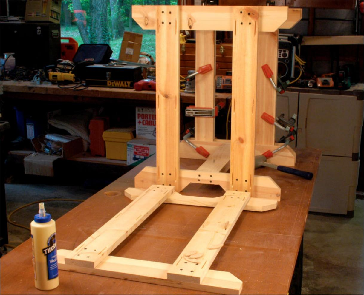
**Step 18** *The assembled outer leg sections were then glued in place with the biscuits all in their slots for proper alignment. They really do make things easier during a large glue-up.*
