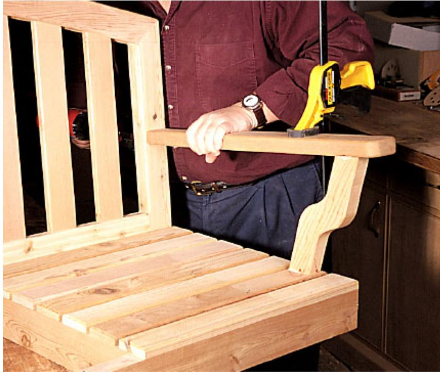
*The back of the arm is simply screwed in place through the back stile, while the support is attached to the arm and seat with dowels and polyurethane glue. Notice the foamy squeeze-out of the glue at the joints.*
