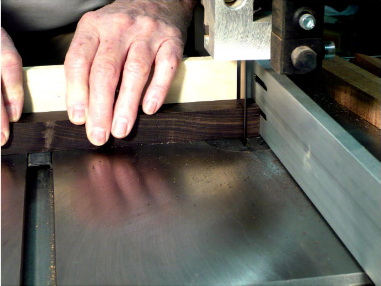
***Perfect Slices.*** After machining a piece of ebony to 1" × 1" × 12", slice 16½"-spacers at the band saw. And make a few extra, just in case.
