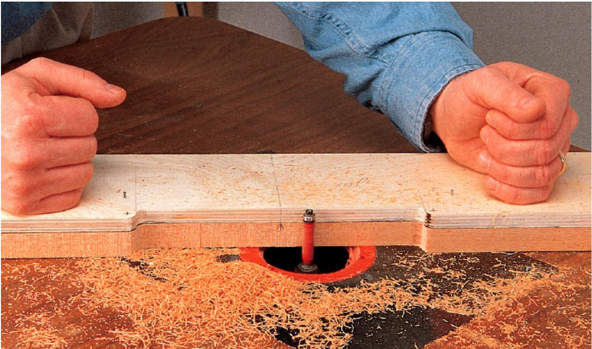
***Step Three: Routing the Parts.*** Pattern routing the parts is easy using the templates. Nail the appropriate template to a roughed out part, using the index lines for reference. Begin routing with the bit cutting against the wood. When you come to a cloud lift, use a climb cut so you don't burn the rounded corner.
