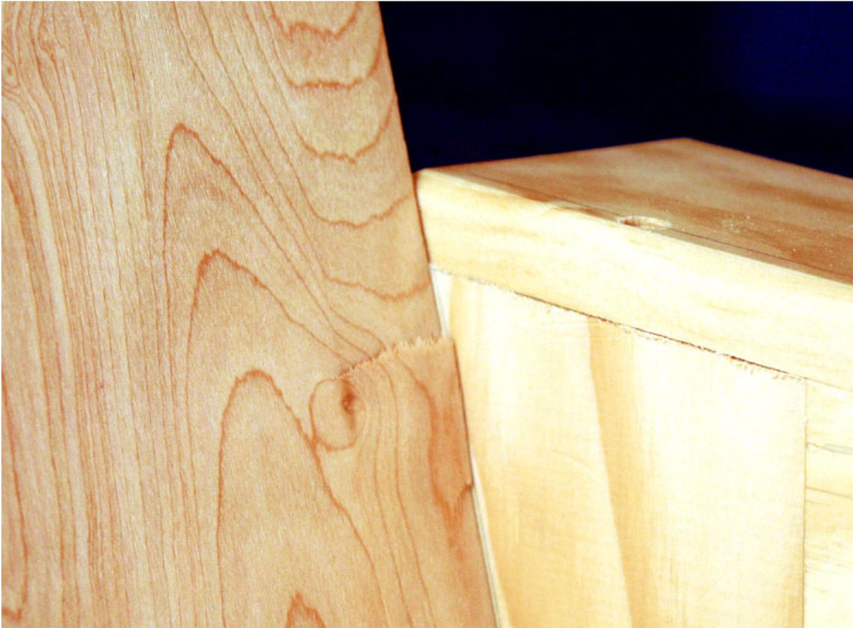
**Step 13** Next, I screwed the back in place and discovered a problem, The back wasn't thick enough to support the screw without the concern (as shown) of forcing the ply's apart when someone sits in the chair.
