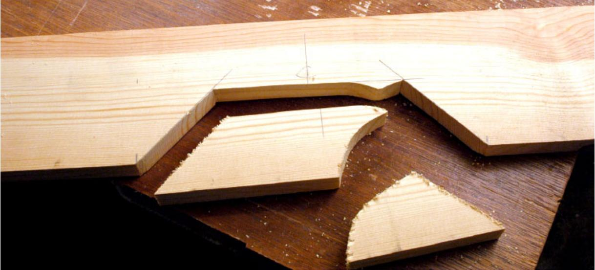
**Step Four** I next cut a sweeping curve from the center of the arch to one of the corners, allowing the waste piece to drop free. I then cut from the open space along the top edge of the arch to the other corner. Both waste pieces are shown here, with only a little trimming at the top of the arch to finish the cut.
