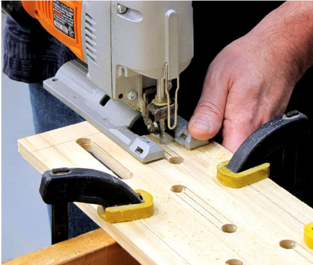
**Figure 1** Drill two  $\frac{1}{2}$ "-diameter holes spaced  $2\frac{3}{4}$ " on center. Connect the holes with lines and make the cuts.
