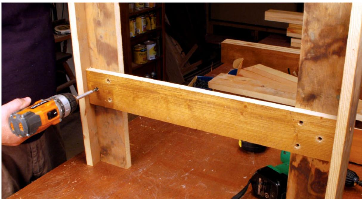
**Step Eight** Screw the side stretchers in place on the outside of the legs.
