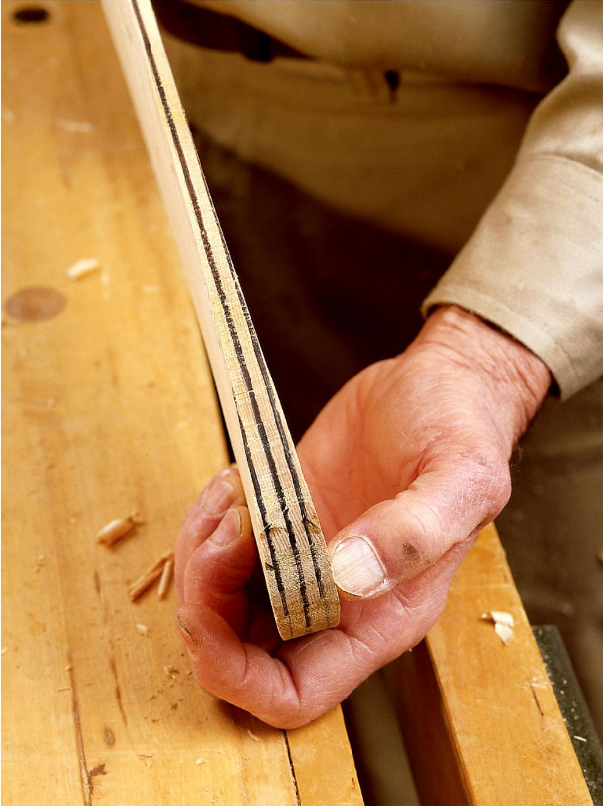
*The point of the blade is left thicker ( $\frac{5}{8}$ " ) to reinforce the point where splits are possible.*
