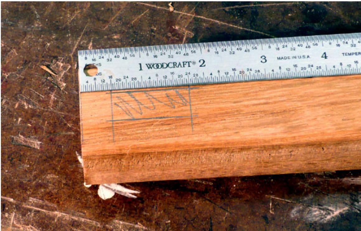
***Time-saving Layout.*** Lay out the mortises on only one leg, which you'll use to set up the stops on your mortise—no need to mark the others.
