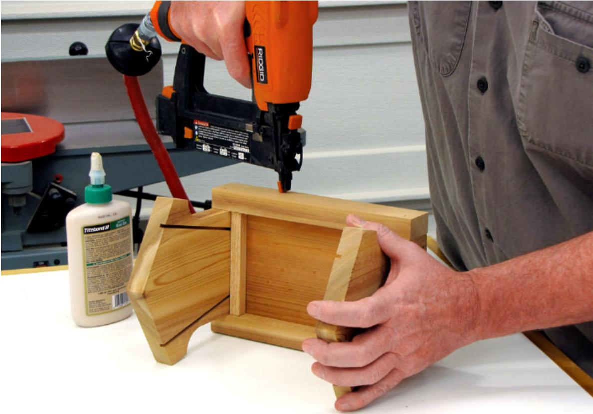
**Figure 6** Attach the tray sides with glue and nails.
