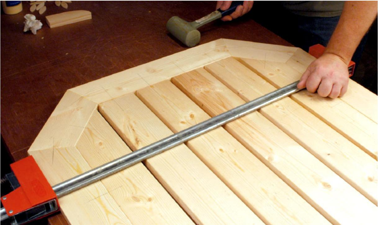
**Step 26** Then add the other outer frame section, tapping and clamping the frame into place to adjust all the joints as you go. Clamp it tight and let it dry.
