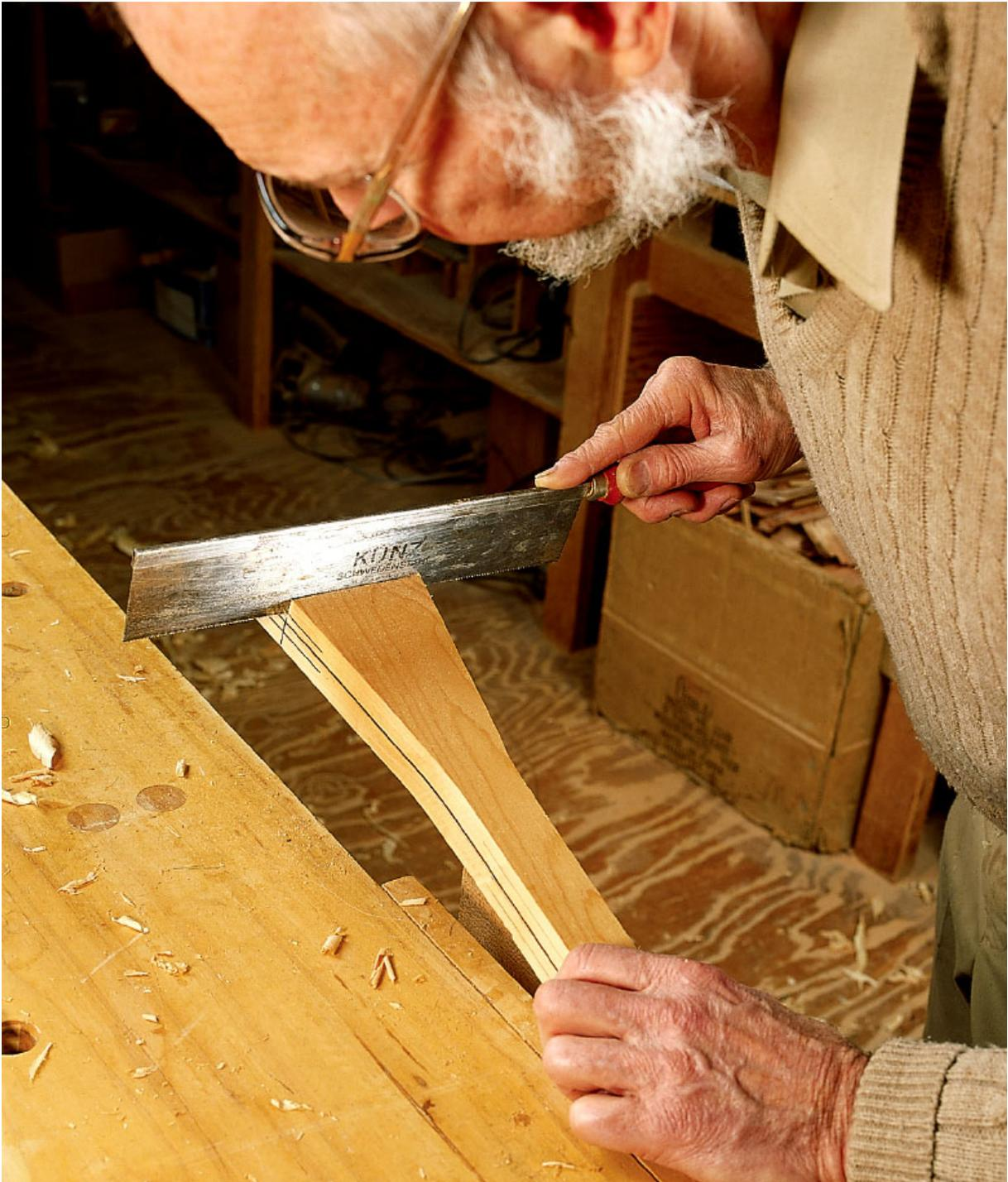
*Saw down to a point on the handle, leaving  $\frac{3}{8}$ " for the grip.*
