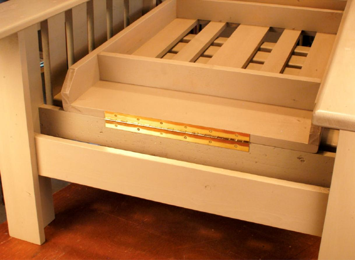
**Step 28** *After painting, the last step is to screw the continuous hinge to the back, then rest it in place on the chair and screw the other leaf of the hinge in place on the back seat support.*
