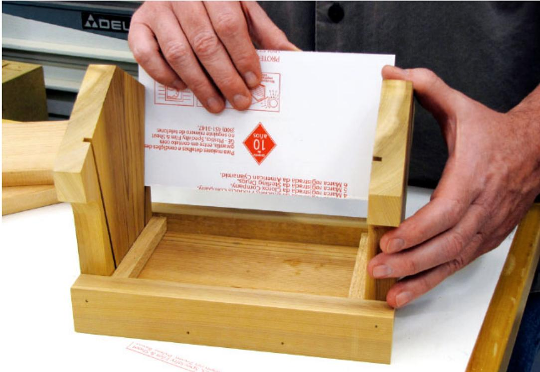
**Figure 7** Fit the acrylic to the feeder, **then** remove the covering.
