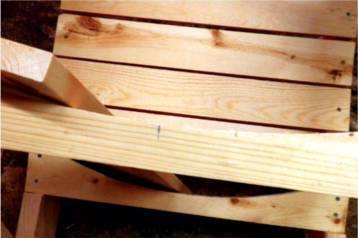
**Step 15** *Laying out the slats for the back takes a bit of experimentation. How many slats should you use? How wide should they be? How do you establish the spacing? Looking at the project from a few different angles helped me to answer these questions.*
