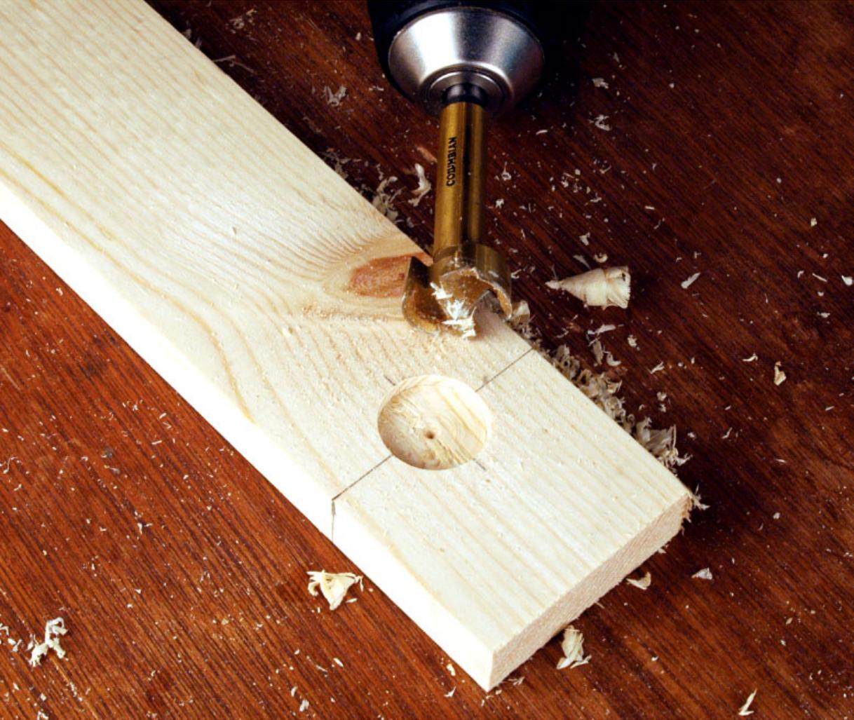
**Step 26** *After carefully marking the location for the dowels on the back support, I drill a shallow hole to protect the top of the dowel from the weather, and to locate the dowel accurately.*
