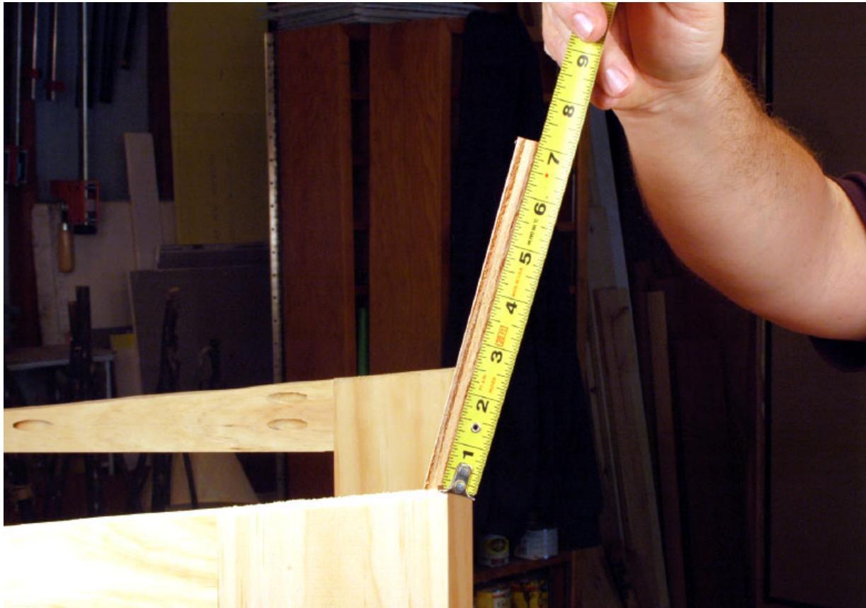
**Step Eight** I slipped the plywood back in place to test the fit, allowing the back to touch the top point of the side, and extend 7" above the sides.
