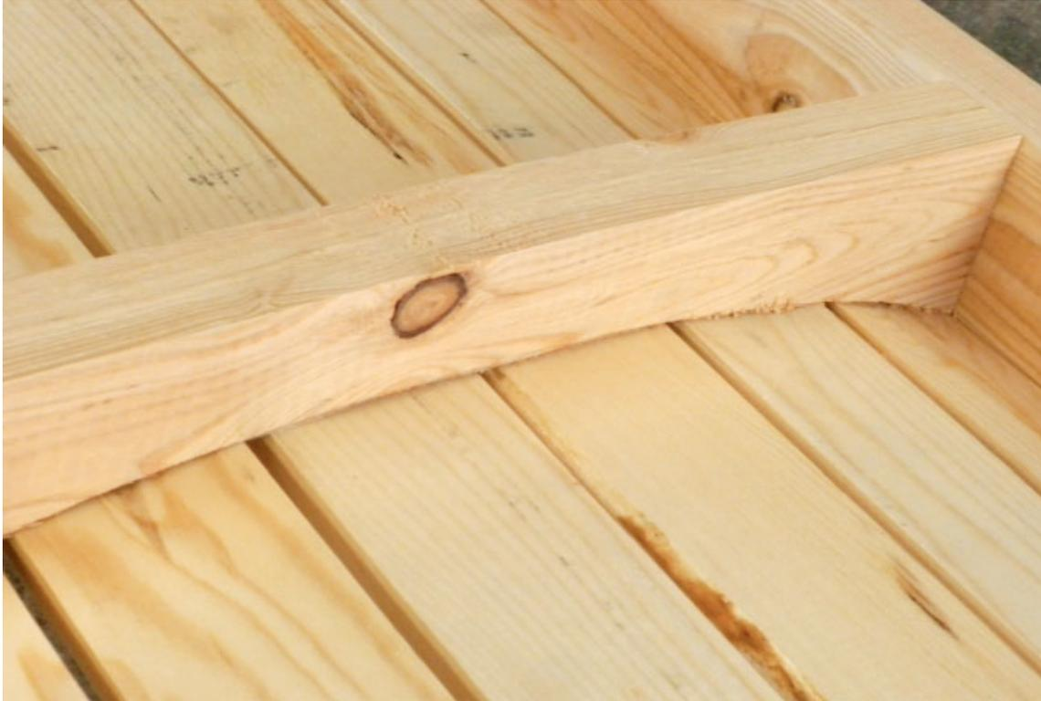
**Step 17** *To provide a safe and sturdy seat, I attached a brace on the underside of the slats. The profile matches the curve on the stretchers that hold the sides together.*
