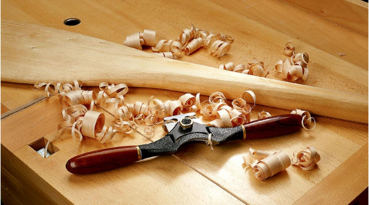
*A spokeshave with a concave sole, such as this one from Veritas, excels at rounding the shaft of the paddle.*
