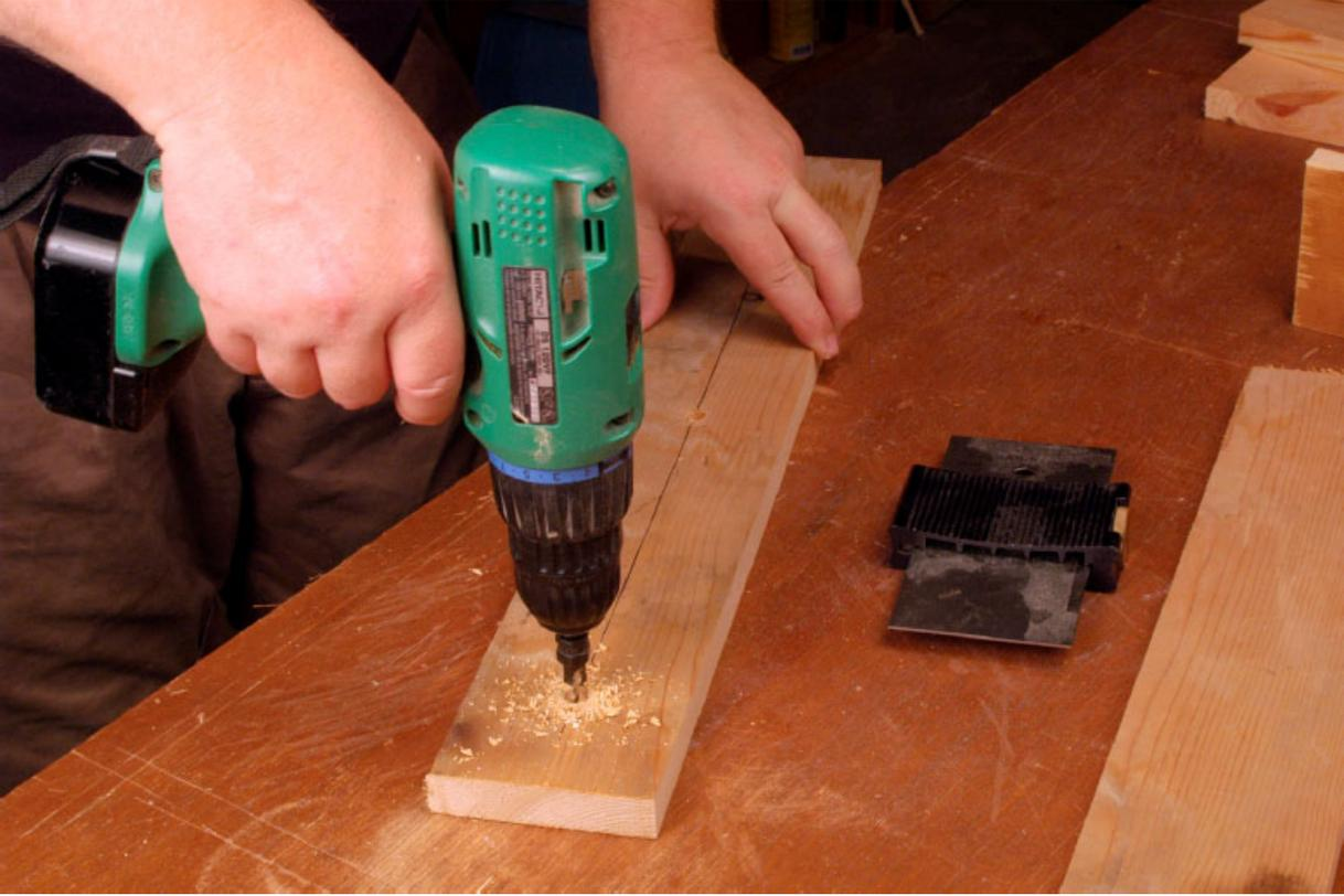
**Step Five** *Drill three or four countersunk holes in each leg flat.*
