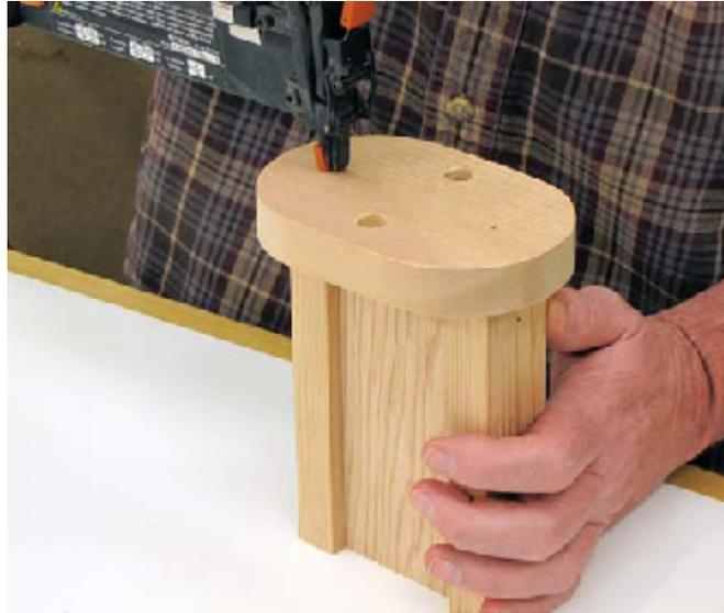
**Figure 4** Center the feeder bottom and glue and nail it in place.
