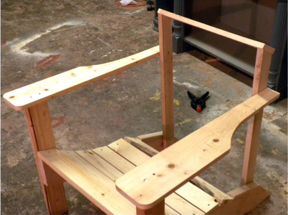
**Step 14** *By sitting in the chair and holding out my arms at a comfortable height, I was able to establish an ergonomically appealing height for the front legs. I cut them to this height and attached the arms and rear legs with screws.*
