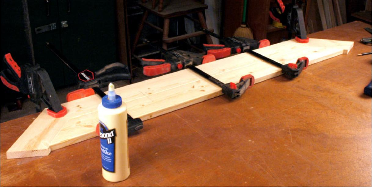
**Step 22** *Glue and clamp these piece together following this same pattern (outside frame first, first slat, then corners) to assemble the one side of the frame. Then repeat this process for the opposite side of the top frame.*
