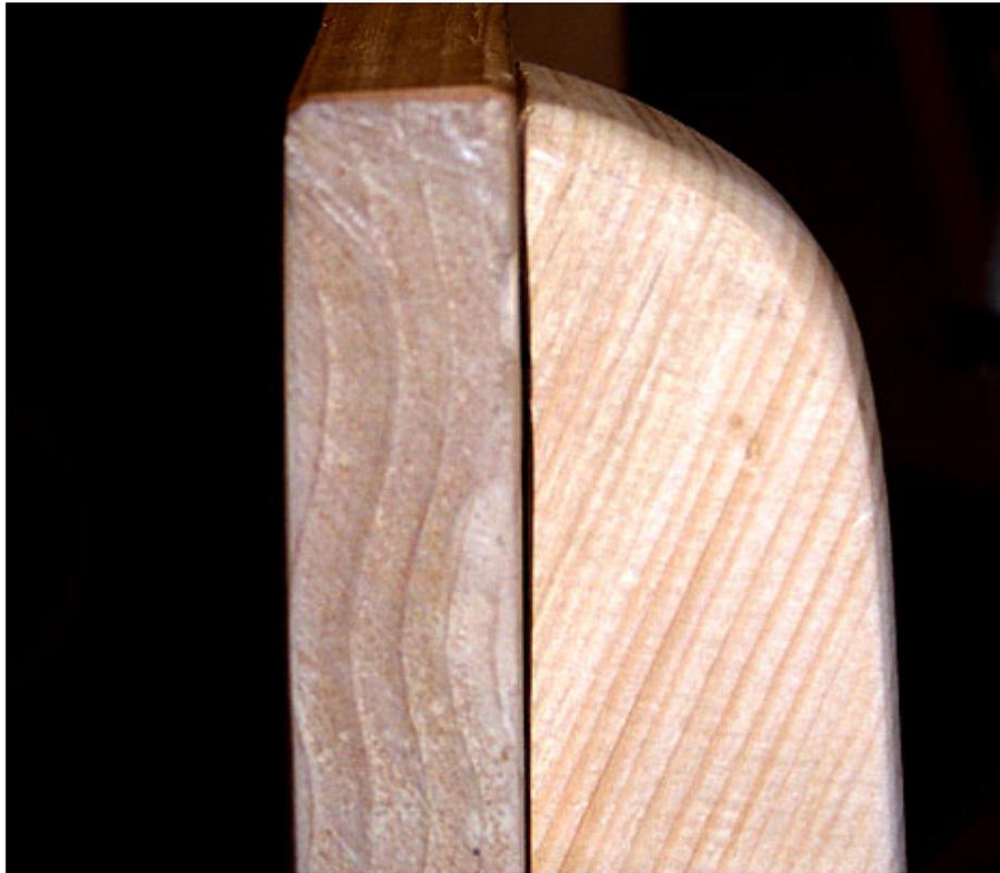
***Plane Speaking.*** Subtle angles and curves add detail to the chair. Work the long edges with a block plane, judging the angles by eye. When it looks good, it is the correct angle.
