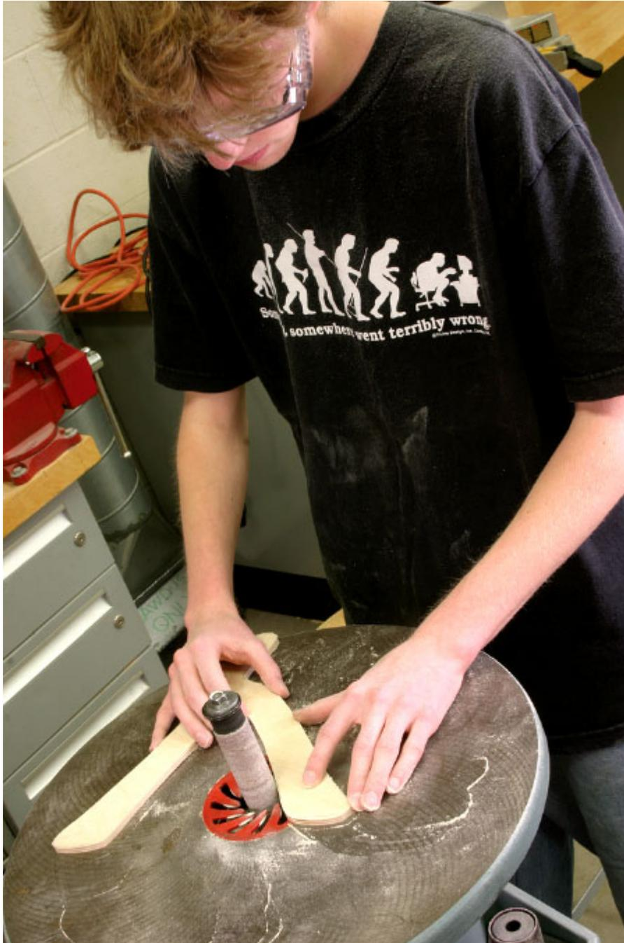
***Smooth Edges Soar.*** At the spindle sander, Todd Geiser refines the edge of his boomerang blank. The spindle sander is an efficient tool for smoothing the perimeter of the boomerang. Getting one smooth and fair line all the way around the boomerang is the goal at this stage.
