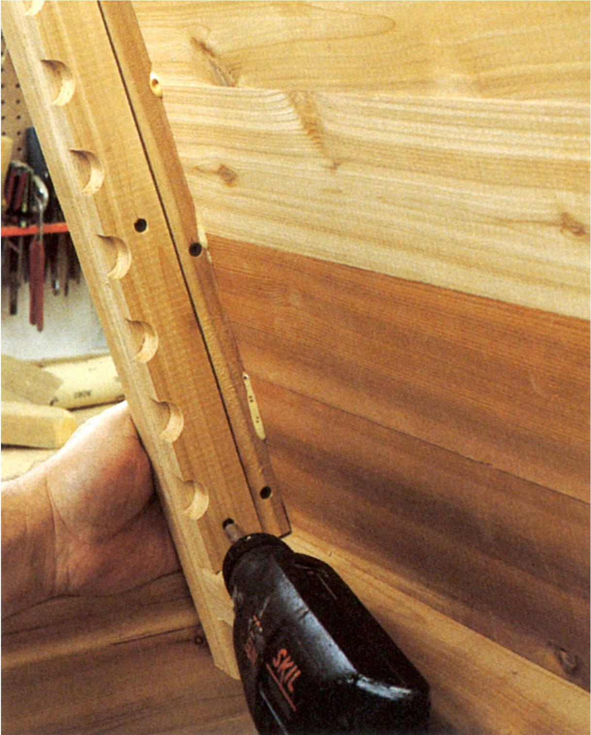
**Step 12** Begin building the adjustable back mechanism by cutting a notched stop board (N). Drill a series of eight 1"-diameter holes along its center line. The holes begin 2" from each end and are centered 2" apart. Cut board N down the center
