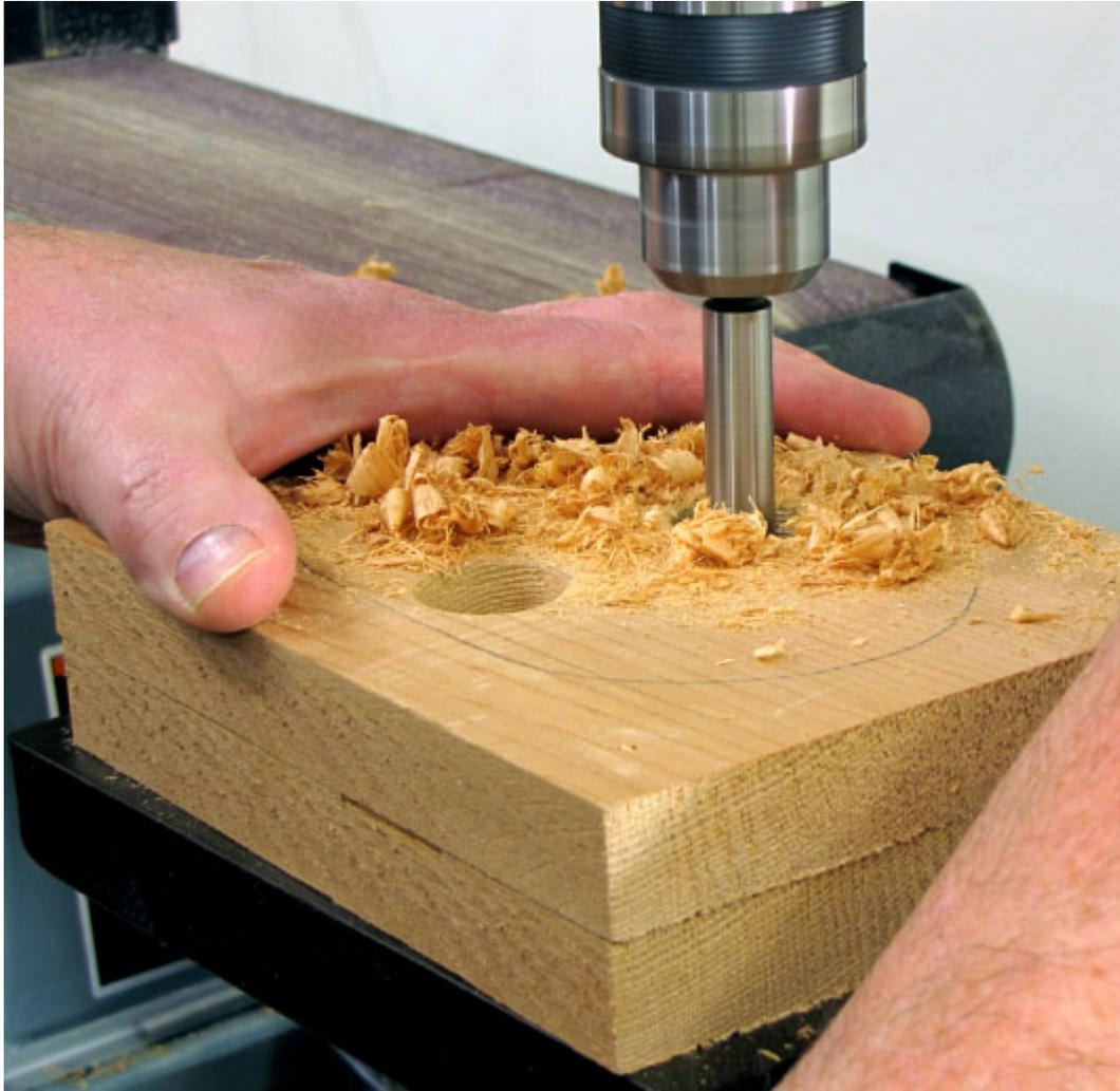
**Figure 1** *Drill all the way through the top piece but only halfway through the bottom.*
