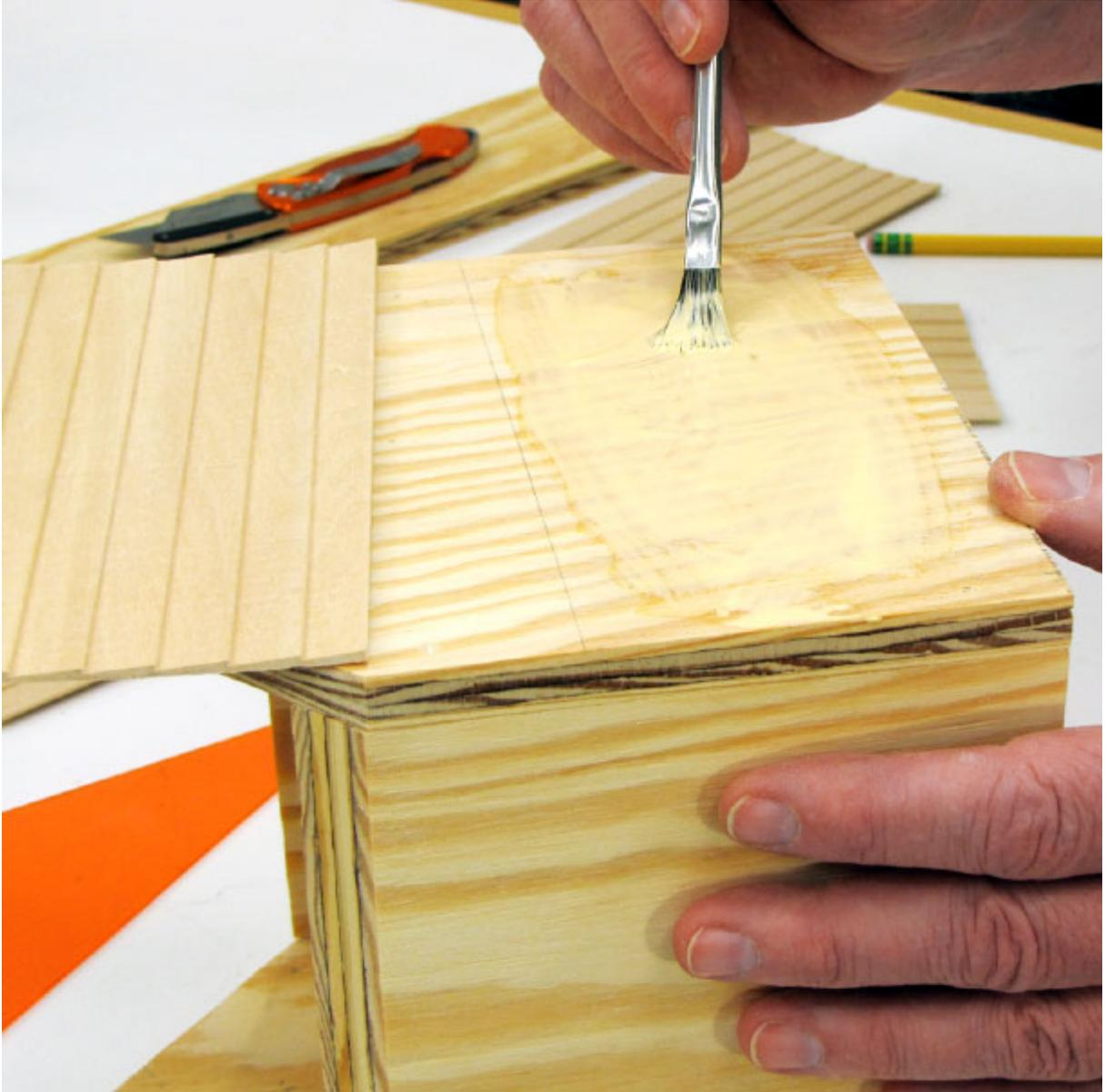
**Figure 5** Spread a thin layer of glue over the area where the first piece of siding will go.
