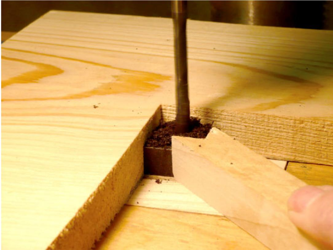
***Jig and Drill.*** Drill  $\frac{5}{16}$ " holes in the center of the spacers. I made a simple bird's mouth, along with a 90° jig, to secure the spacers during this operation.
