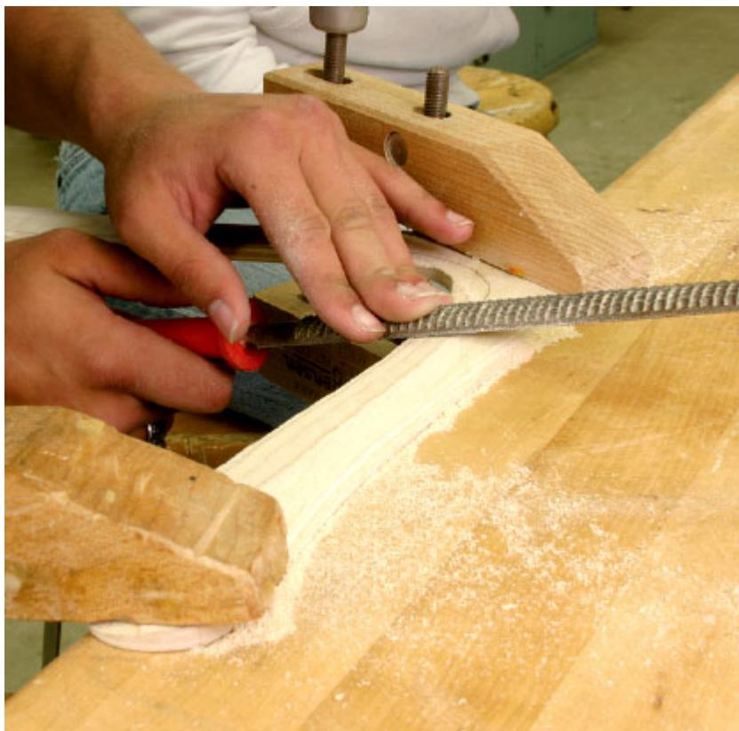
***Rasp Your Airfoil.*** *Clamps help to steady the boomerang blank while the airfoil is brought to life. In this photo, Mike Laba uses a rasp to make quick work of the shaping process. Notice that Mike has positioned the boomerang off the edge of the bench so the the rasp does not damage Mr. Merian's benches.*
