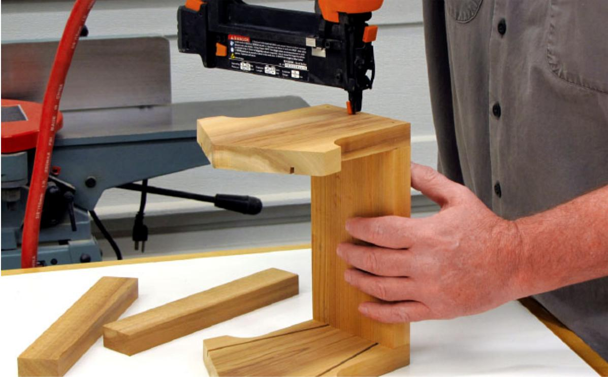
**Figure 5** *Glue and nail the ends to the bottom.*
