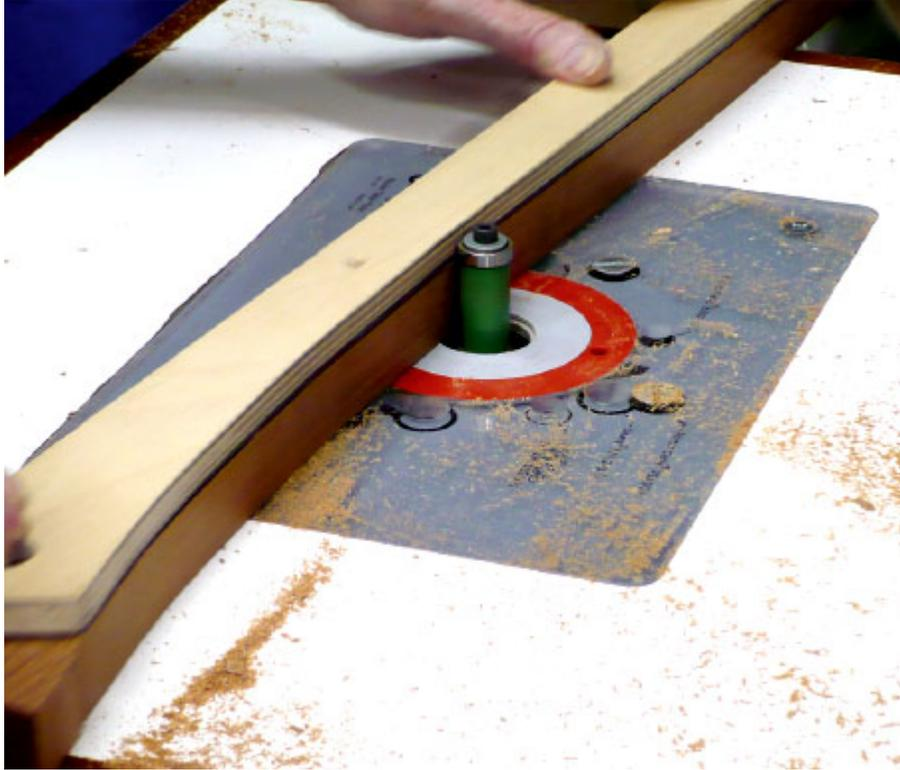
***Pattern-rout the slats.** Jatoba is very brittle and prone to splintering, so attention to grain direction while routing is essential to avoid tear-out.*
