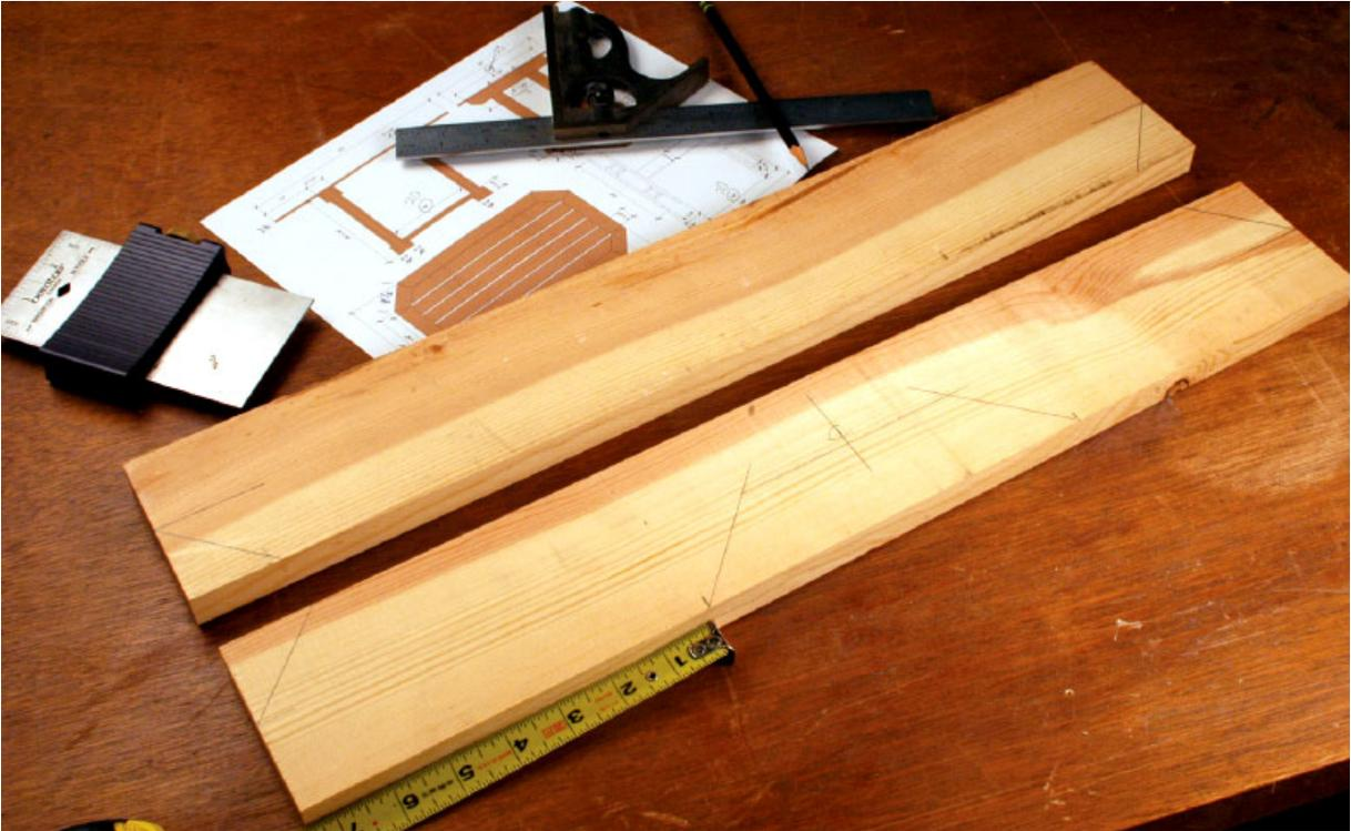
**Step One** Mark the location of the corner bevels on the four upper supports and the four base pieces, and also mark the lower “arch” on the base pieces.
