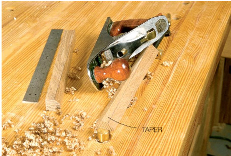
*Clamp the post with one corner facing up. Check the grain direction and start planing. Begin with short strokes at the top of the post and, as your taper lengthens, make your strokes longer.*
