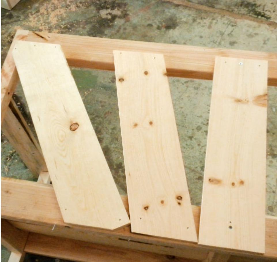
**Step 21** *To begin laying out the seat slats, I clamped the sides in an upright position. Even though the swing was laying on its back, it was the most definitive look yet at how the finished swing would shape up, and it helped me to see how to proceed.*
