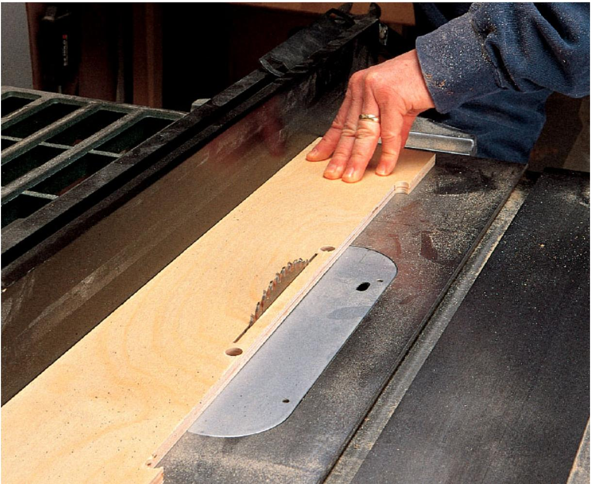
**Step One: Making Templates.** Begin cutting out the 1/2" Baltic Birch templates by drilling holes at the proper corners. Raise the blade on the table saw into the middle of the stock to make the straight cuts. Band saw the rest and clean up the cloud lifts using a disc sander.
