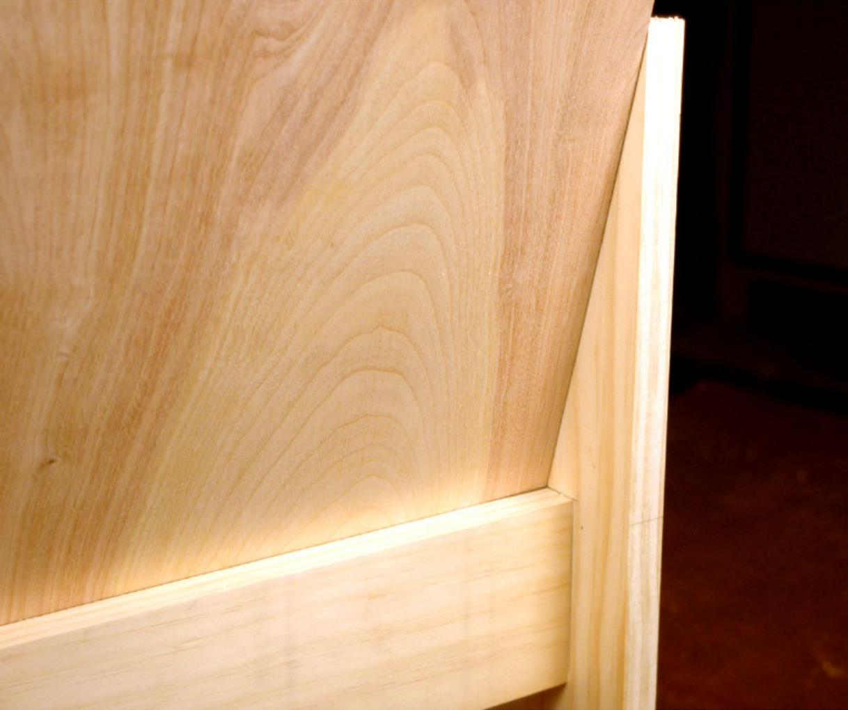
**Step Nine** *The lower part of the back is braced against the back stretcher for more support. I then marked the location of the back on the inside surface of the sides.*
