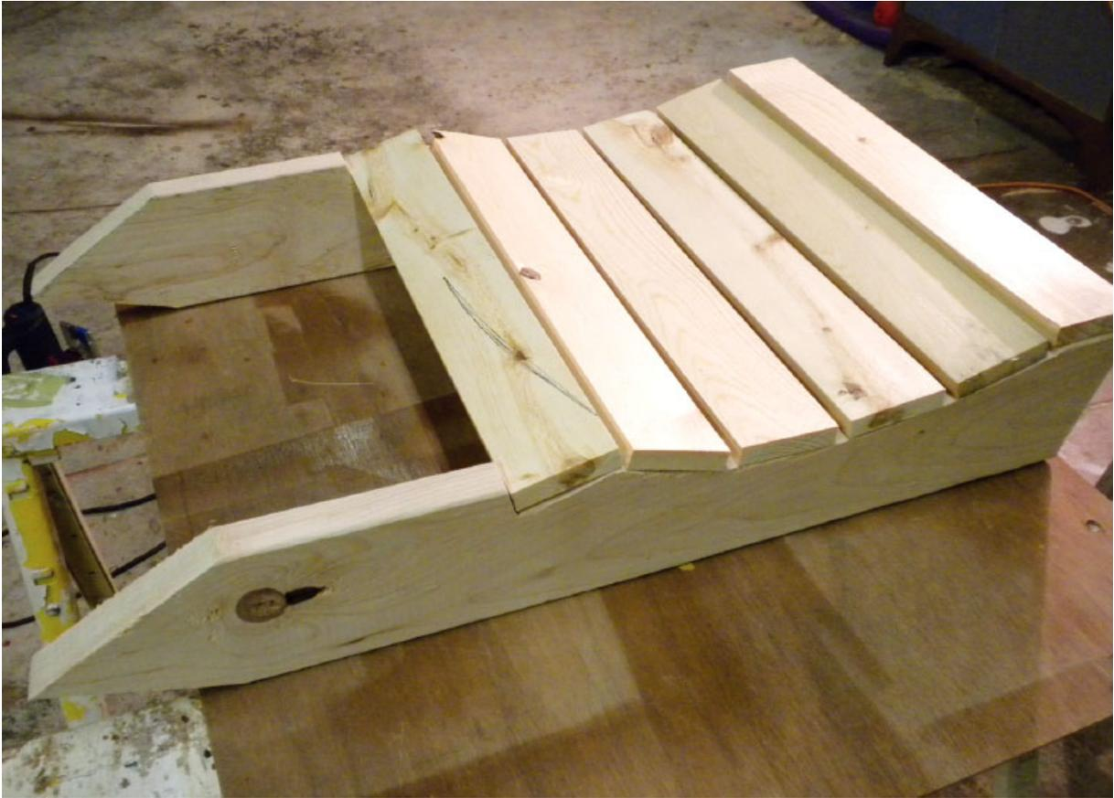
**Step Two** Once the supports have been cut out, the seat slats can be laid across them and secured with screws. Pre-drilling a clearance hole for the screws will prevent the ends of the slats from splitting.
