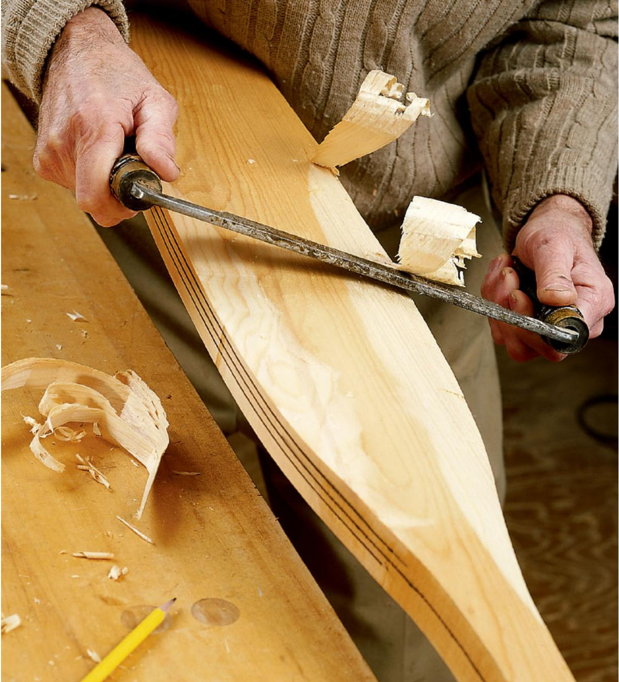
*Use a drawknife to rough the blade to thickness. Bevel the edges first as shown, then take down the center. It may be tough using this tool, so try to hold it the way the photo shows. This should ease the struggle a bit.*
