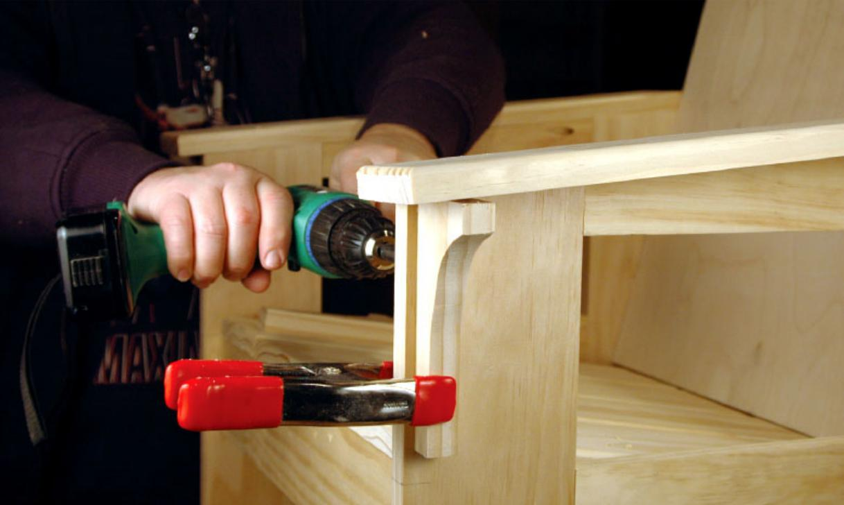
**Step 21** Use the template to mark and cut out the arm support corbels. A jigsaw works, but if you've got a band saw handy, it's easier. Sand the corbels, and then add some glue and screw them in place through the inside surface of the side frames. I held my corbels about  $\frac{1}{4}$ " back from the front edge.
