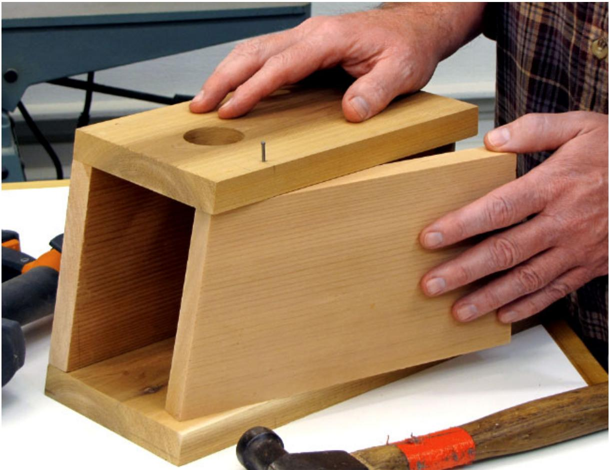
**Figure 5** *Make sure the nails are the same distance from the bottom of the box so they function properly as hinges.*
