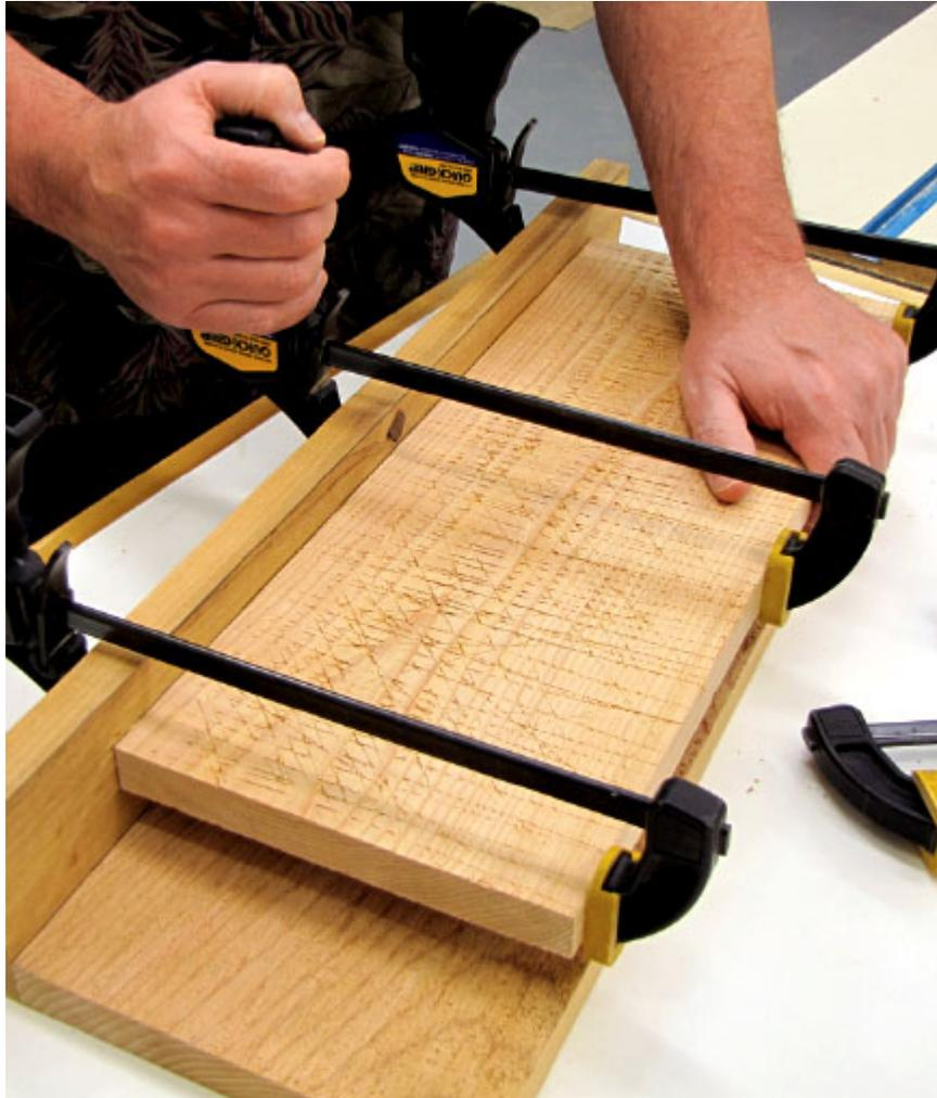
**Figure 3** *It's a little easier to install the divider using just glue and some clamps. A couple of reinforcing nails can be added later.*
