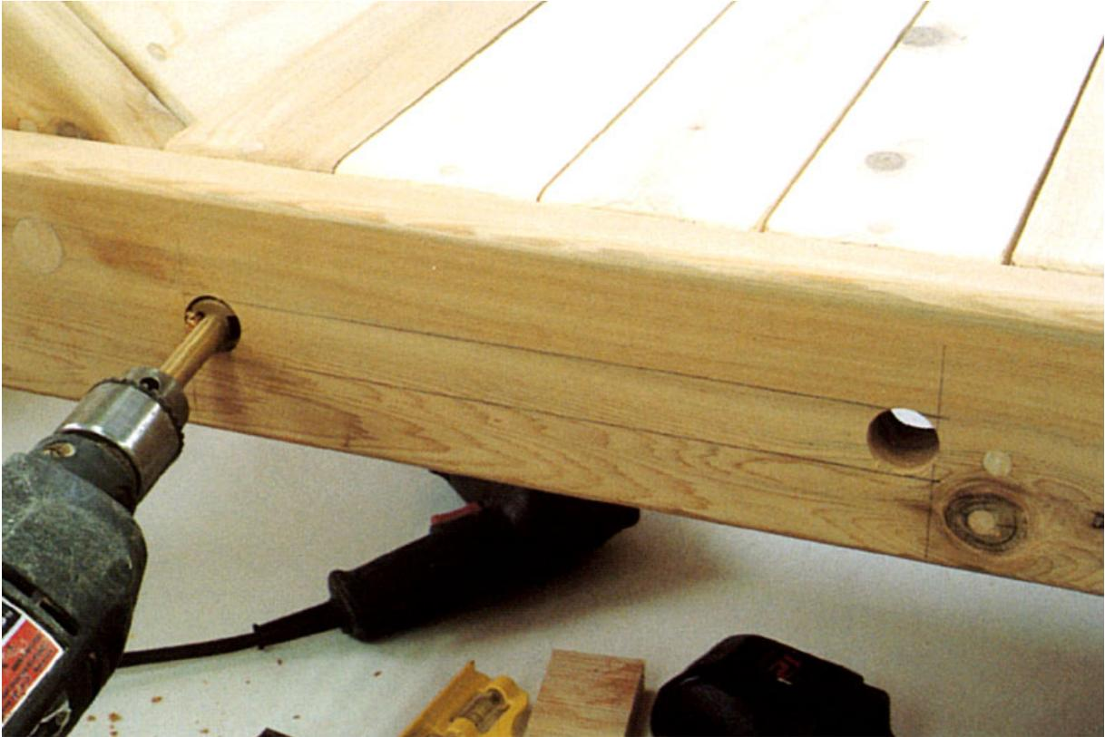
**Step 14** *Cut a 1"-wide slot, 12" long, in one side rail. The pullout can be installed on either side, so locate the slotted opening accordingly. The lower edge of the slot should be 1 ½" above the bottom edge of the side rail. Cut the slot between the center brace and headboard end of the lounge. The slot begins tight to the center brace. Use a 1"-diameter bit to drill holes at both ends of the slot and complete the cut with a jigsaw.*
