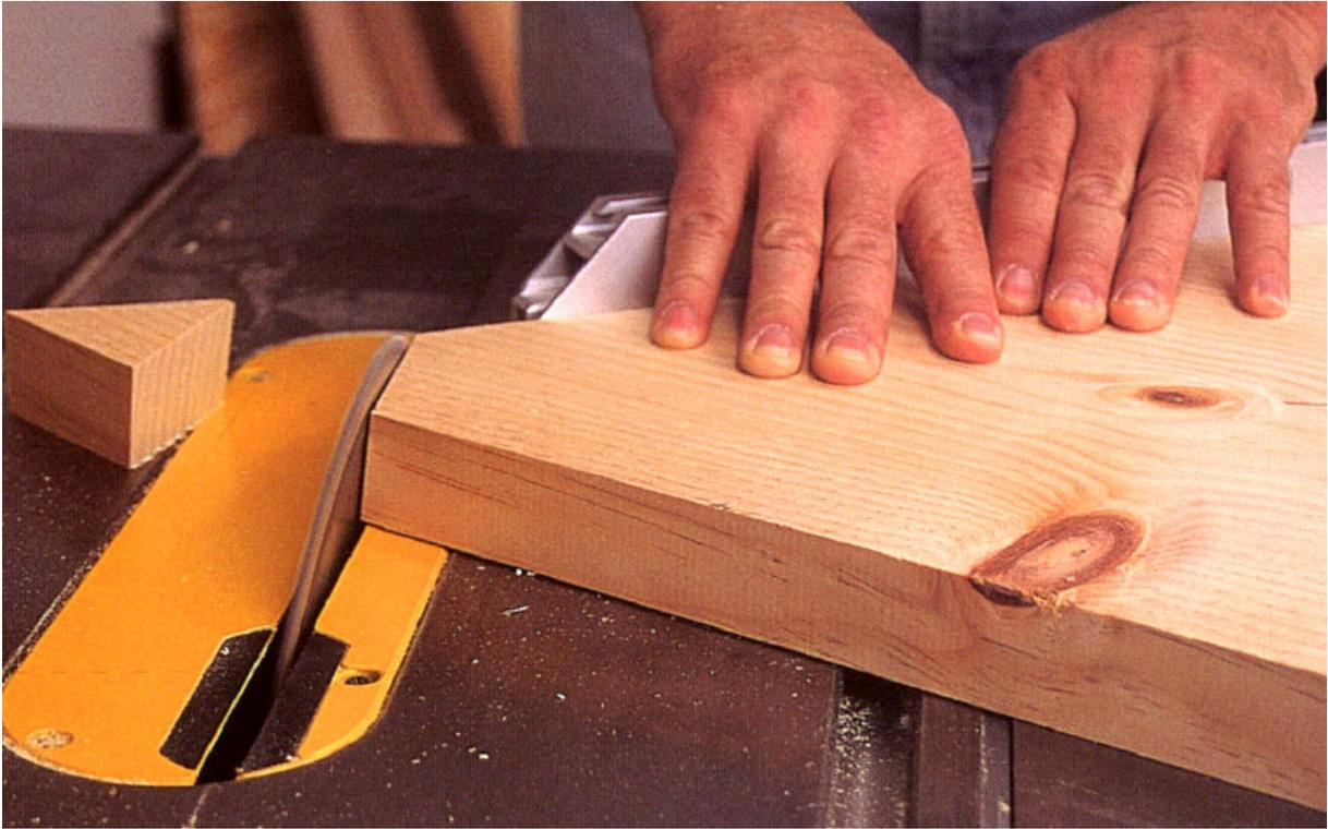
**Step Five** *To clip the ends of the triangle, reset the miter gauge to 30° on the other side of the gauge and set the blade to the required leg-splay angle. Hold the panel against the fence and cut off the end of the triangle. This creates the joint surface for the legs.*
