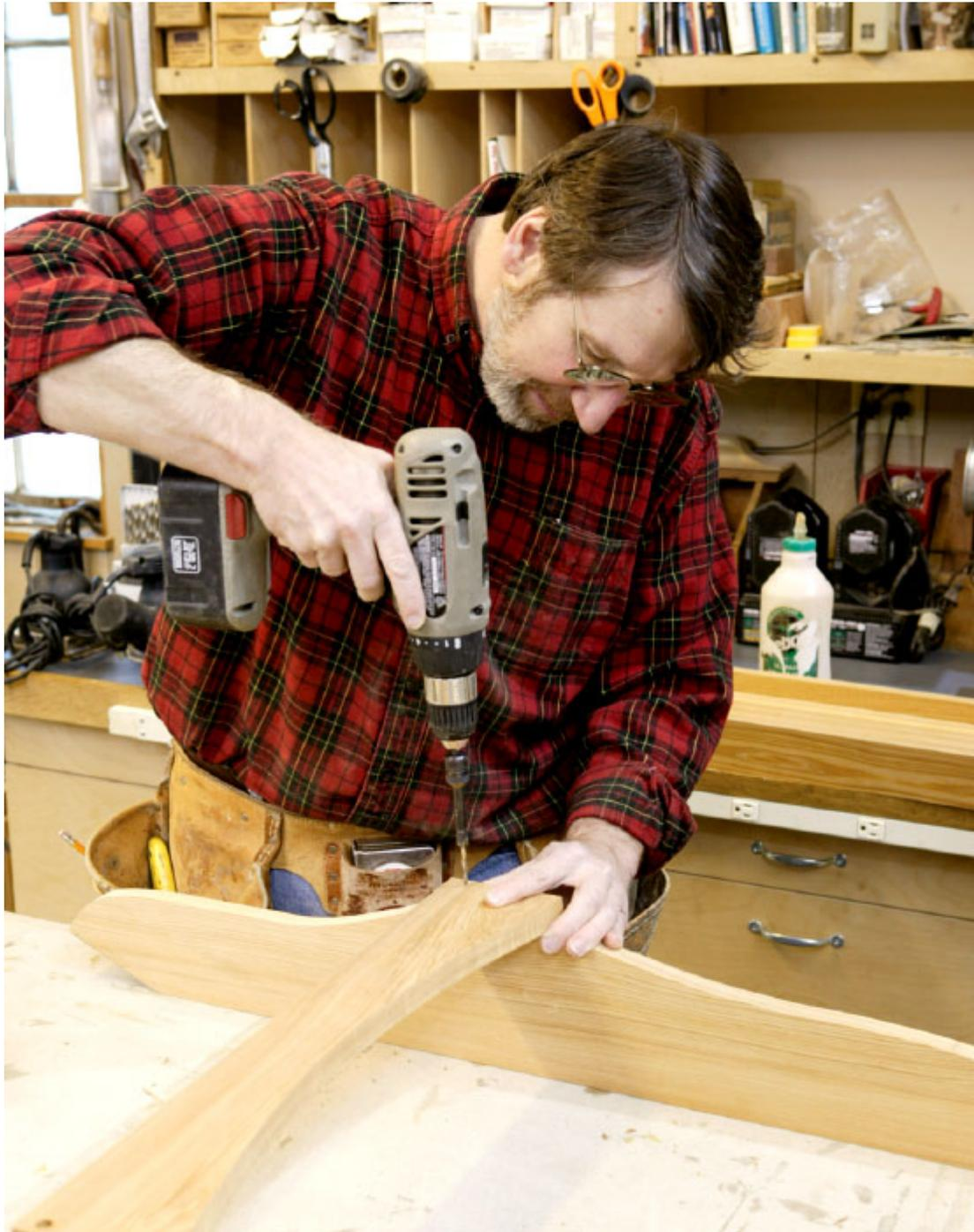
*Start the assembly by gluing and screwing the lower rear crosspiece to the chair sides. For lasting results, use a marine grade or waterproof glue, and stainless steel screws.*
