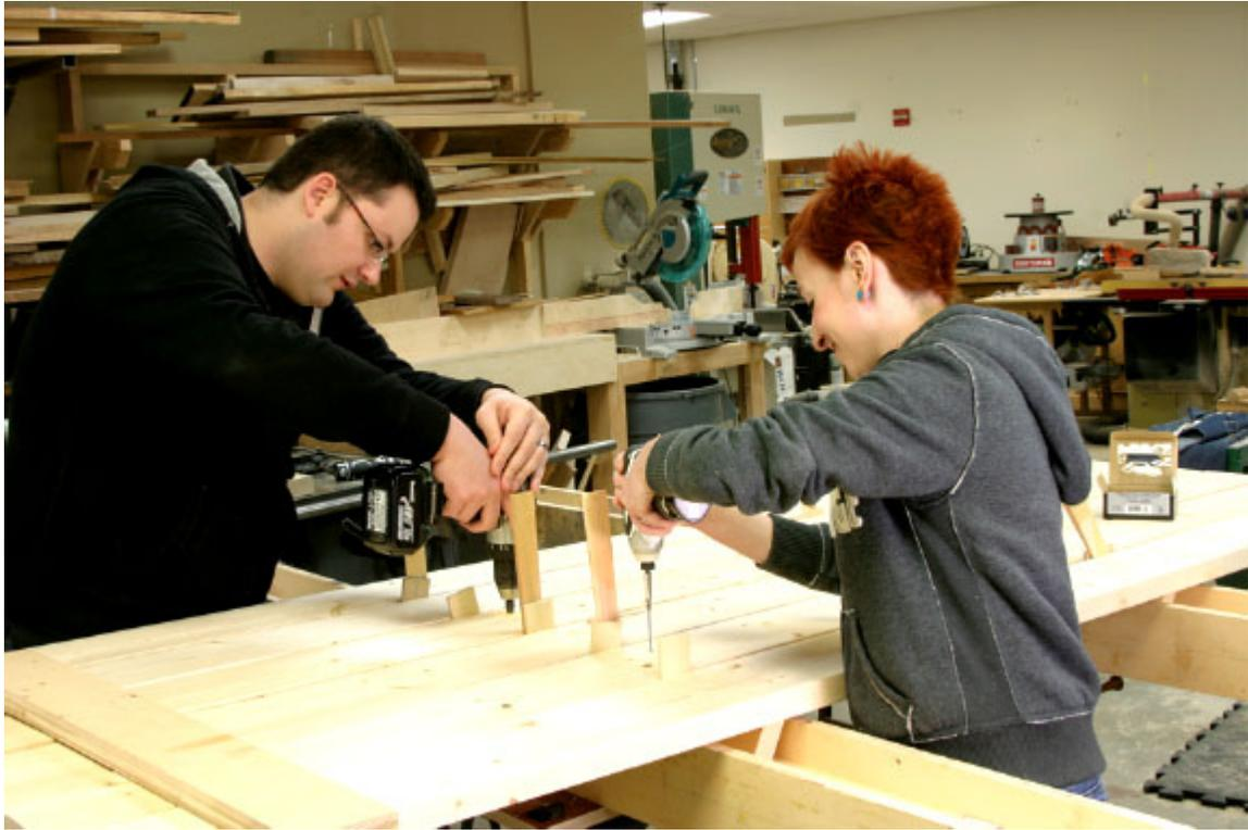
**Spaced Out.** Use shims to space out your top boards. When the top looks good, screw it down.
