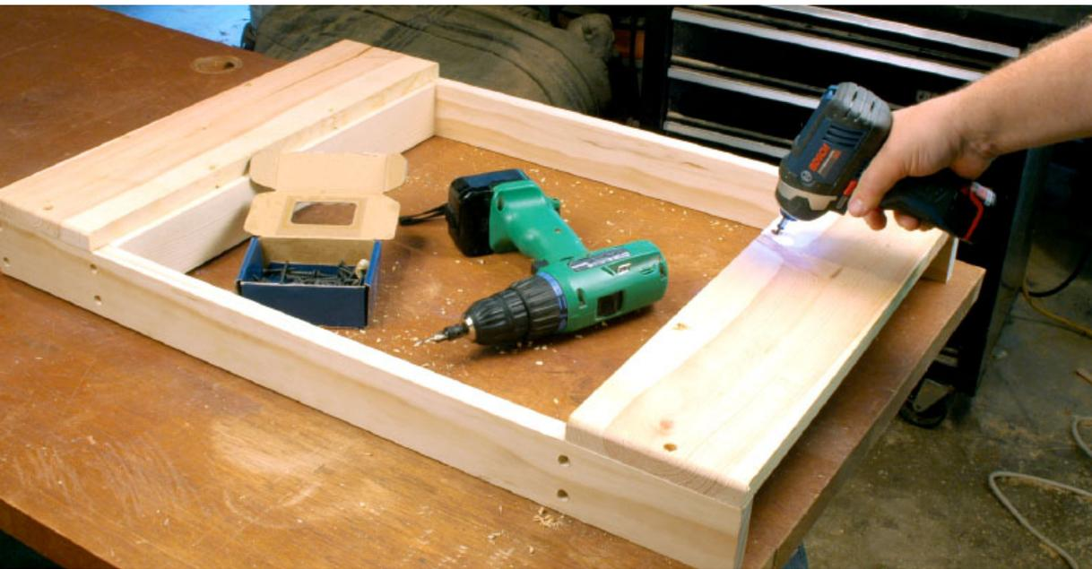
**Step 23** *The rest of the seat slats are screwed into the seat supports on either side. The top and bottom plates are then screwed to the front of the frame, lipping only half way over the two middle cross members.*
