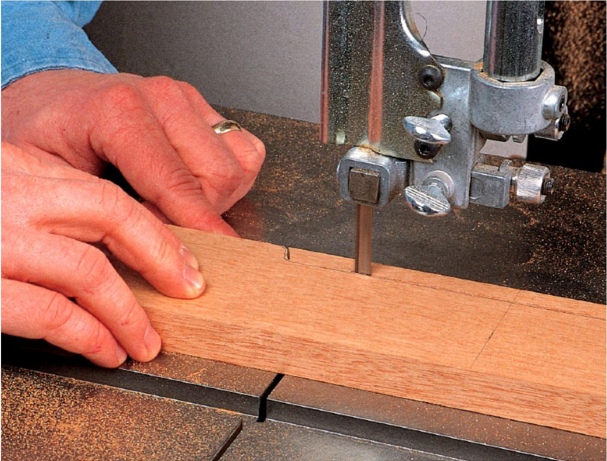
***Step Two: Roughing Out the Parts.*** Use the center lines to index the template on what will be the back of each piece (it will eventually have nails driven into it) and draw the appropriate cloud lift or reverse cloud lift. Cutting close to the line, rough out these pieces on the band saw.
