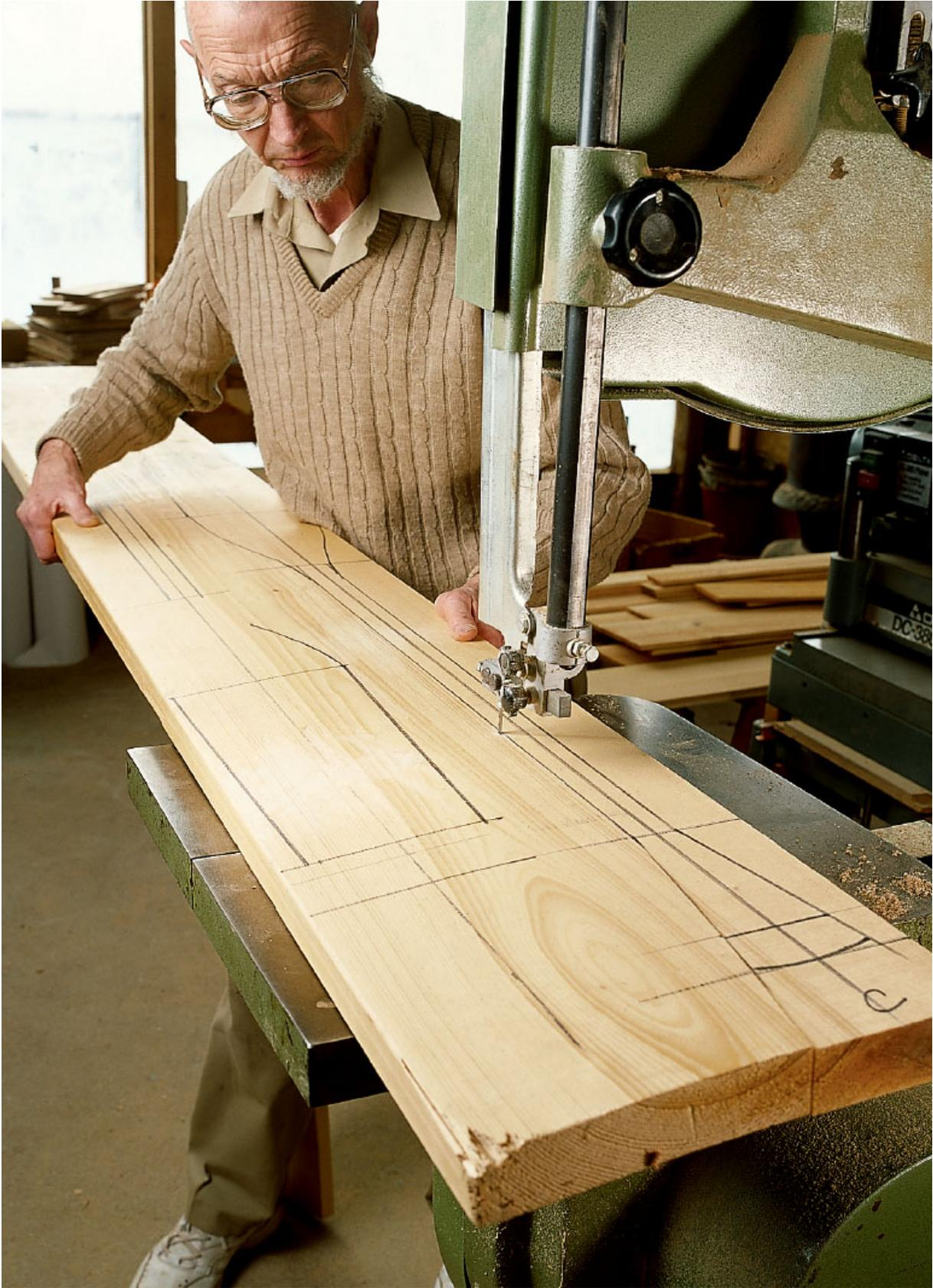
*After planing the plank to 1 1/4" thick, band saw the paddle blank to shape.*
