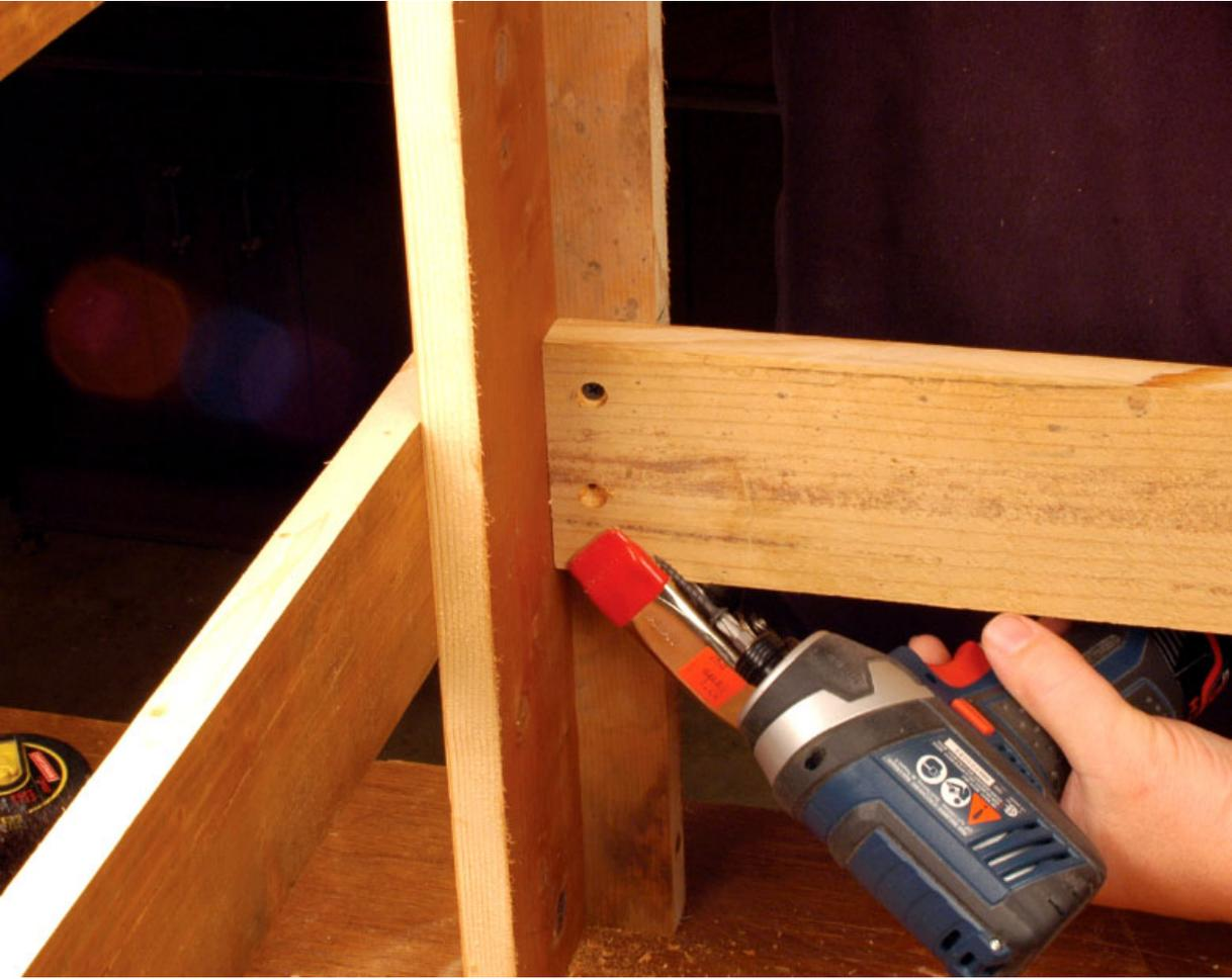
**Step 13** *The front and back stretchers are screwed in place to the front and back legs. Check for squareness where the stretchers meet the legs.*
