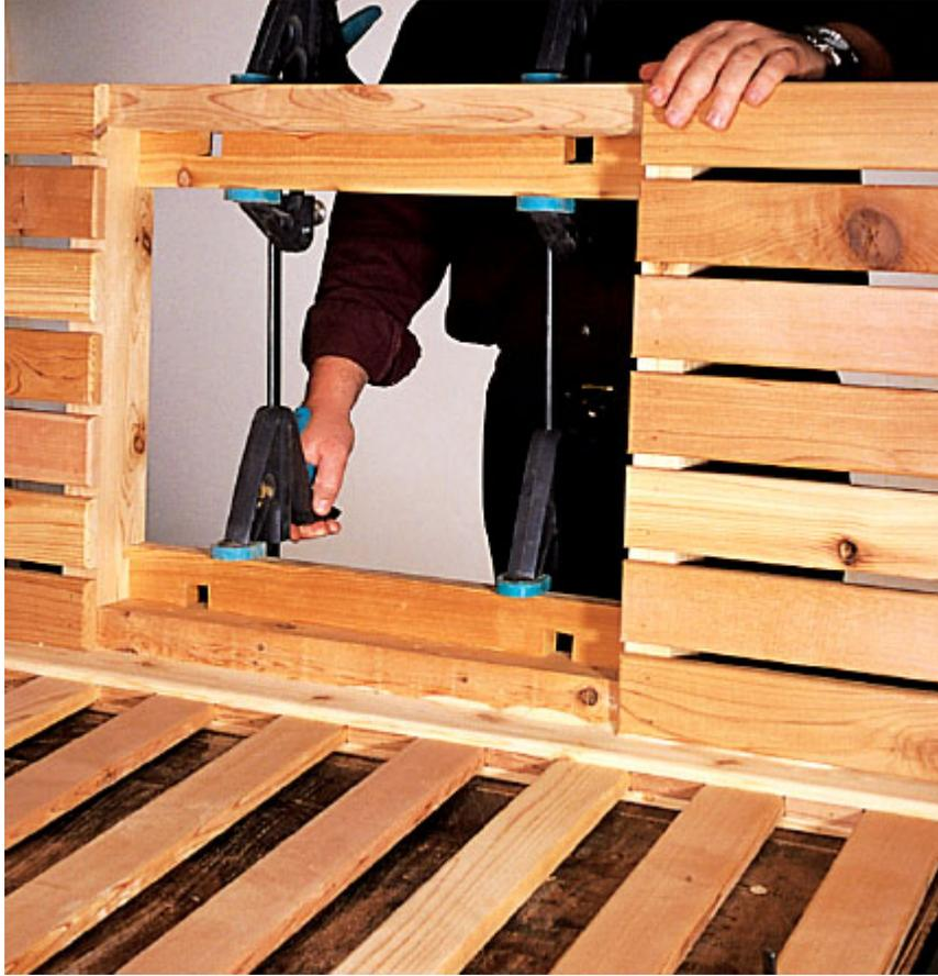
*With the notches cut in the support cleats, the two pieces can be glued in place in the seat frame.*
