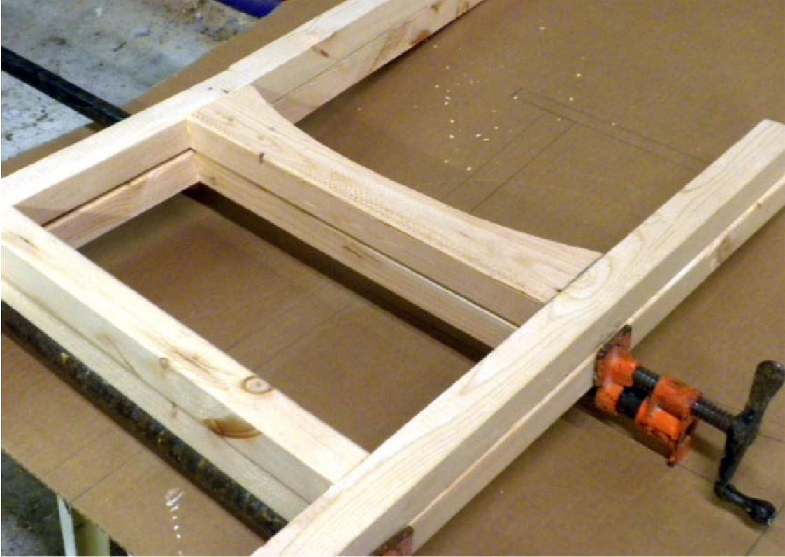
**Step Seven** *Two clamps are sufficient to ensure good, even clamping pressure. With the first side clamped up, the second goes together the same way—and it is usually a little bit quicker, as well, since you’ve just practiced it once. I like to lay the parts on top of the first side to double-check that the sides are identical and that no errors crept in the second time around.*
