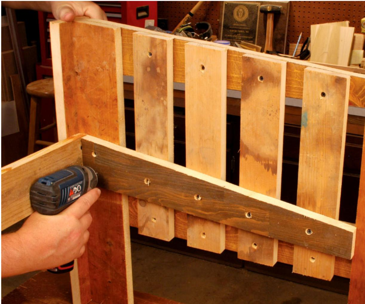
**Step 16** *The seat supports fit flush to the top of the front stretcher, and attach to the slats.*
