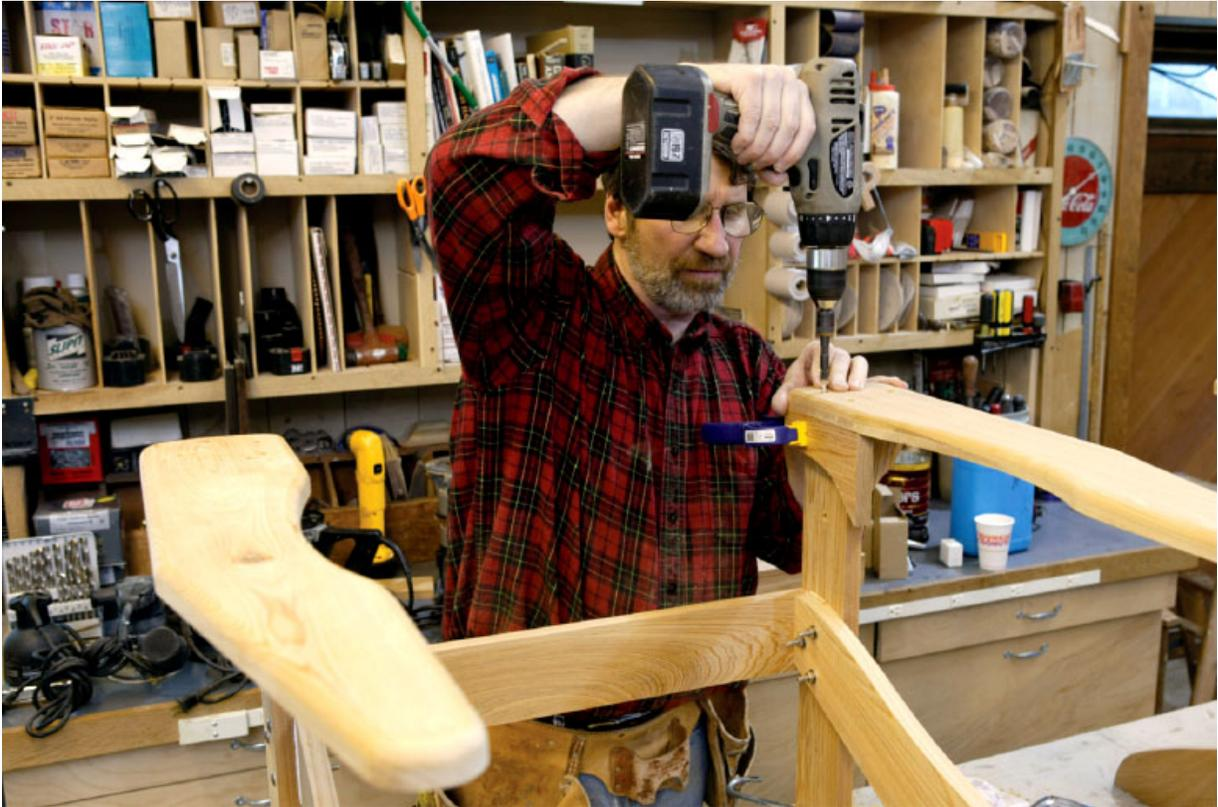
*Use three screws to attach the arm to the leg and arm bracket. Carefully position the arm for a  $\frac{3}{4}$ " overhang of the leg. Use a spacer to help position it. The arm overhangs the front edge of the leg  $1\frac{1}{8}$ " .*
