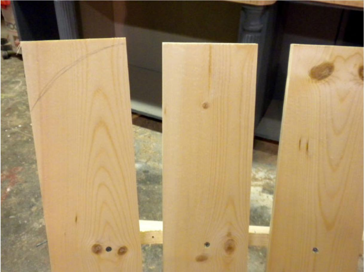
**Step 17** *I decided to soften the look of the back by cutting a curve onto the tops of the two outermost slats. I sketched a line to represent this.*
