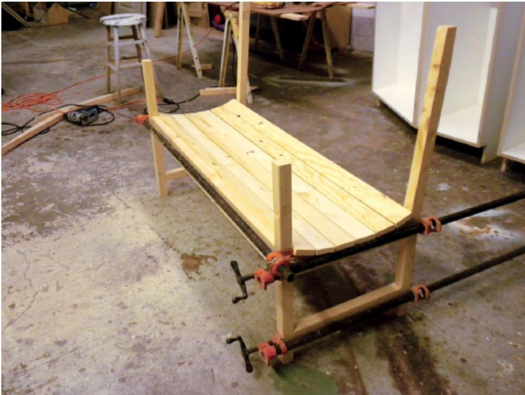
**Step 11** Applying glue to the strips goes fairly quickly—I use a disposable foam brush to make sure that all surface are coated evenly. A certain amount of glue squeeze-out is inevitable. I find that small spring clamps like this are the most convenient way to hold everything in place. I think that every shop should have a bucket full of them—they're inexpensive and very useful.
