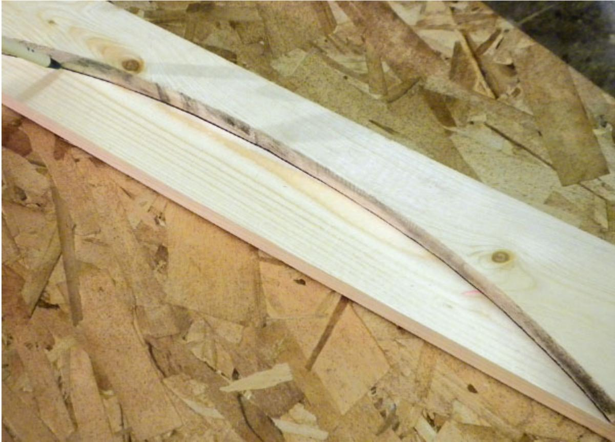
**Step Seven** *Since I was in the mode of cutting curves, I also cut out the back support rail for the top of the back. I used the same technique, but in this case the curve extends to the ends of the slat.*
