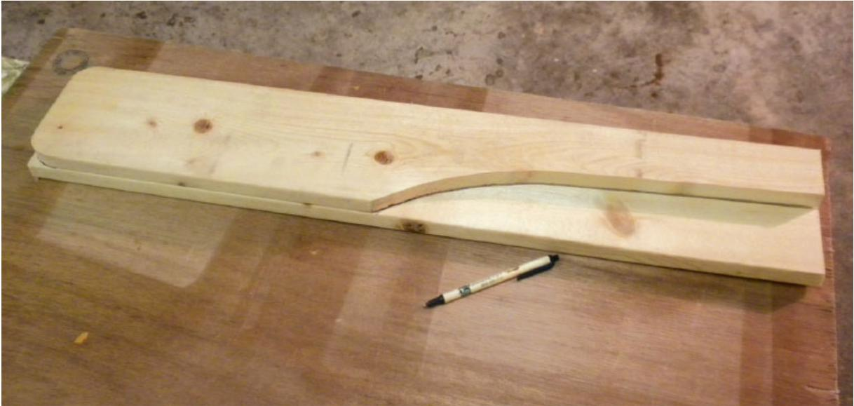
**Step 13** *The sequence of events isn't too critical here—I jumped around a bit and decided to fabricate and attach the arms. In typical Adirondack fashion, they were fairly broad, and they feature a curve that tapers to a 2" width toward the back of the chair. Again, the shape can be personalized, so don't hesitate. Add radii to the front corners of the arms for comfort. Once I had cut out one, I used it as a pattern for the other arm.*
