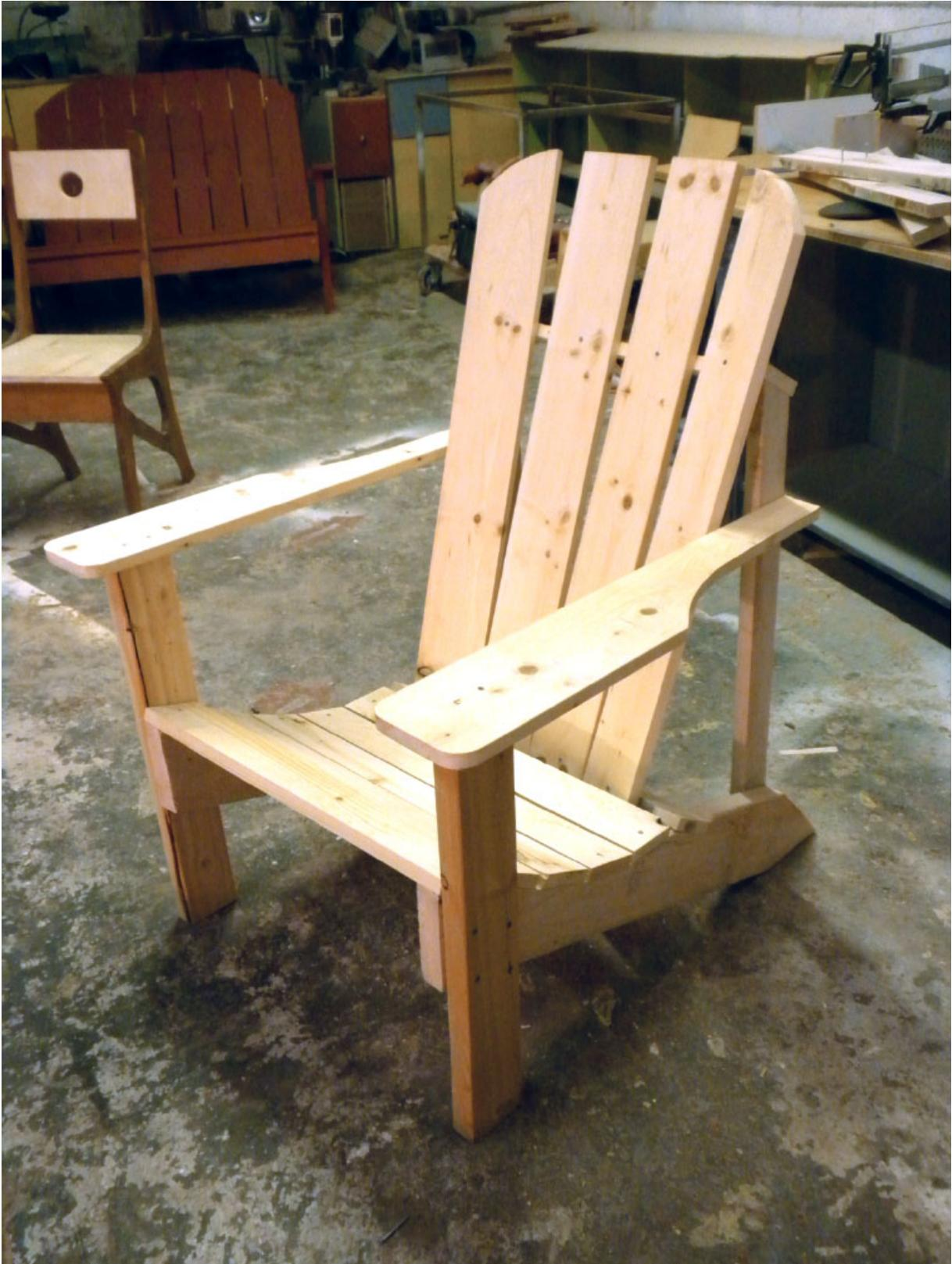
**Step 19** *Cutting the curves on the tops of the two slats made a big difference—the back looks just right to me now.*
