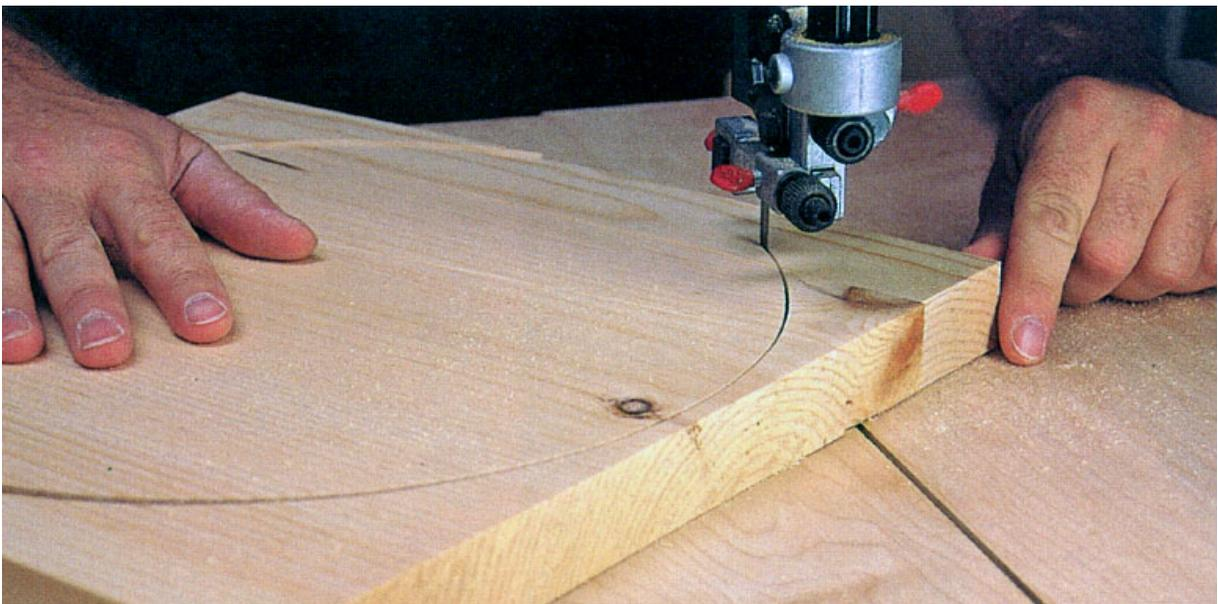
**Step 11** Complete the circle cutout, and sand the edges of the top pieces. Rout a 45° bevel on the top and bottom edges.
