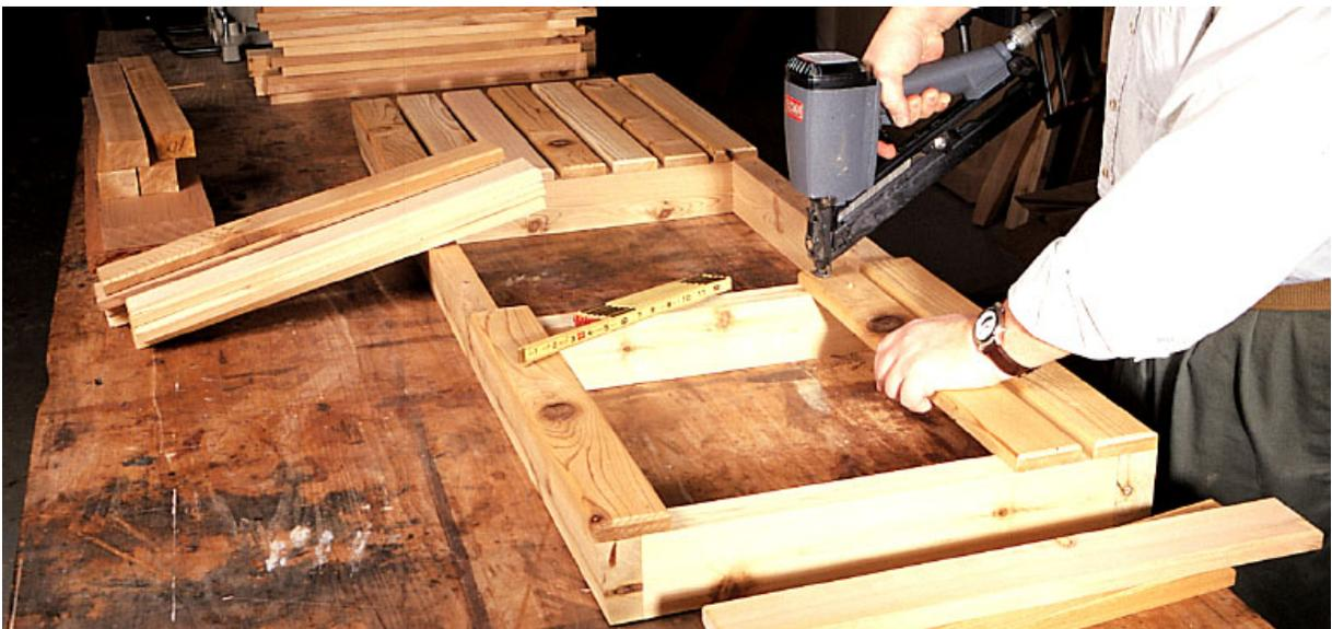
*With the seat frame assembled, nailing the slats in place was a cinch with a pneumatic finish nailer and stainless steel nails. Note the 7-degree bevel on the rear of the back seat rail.*
