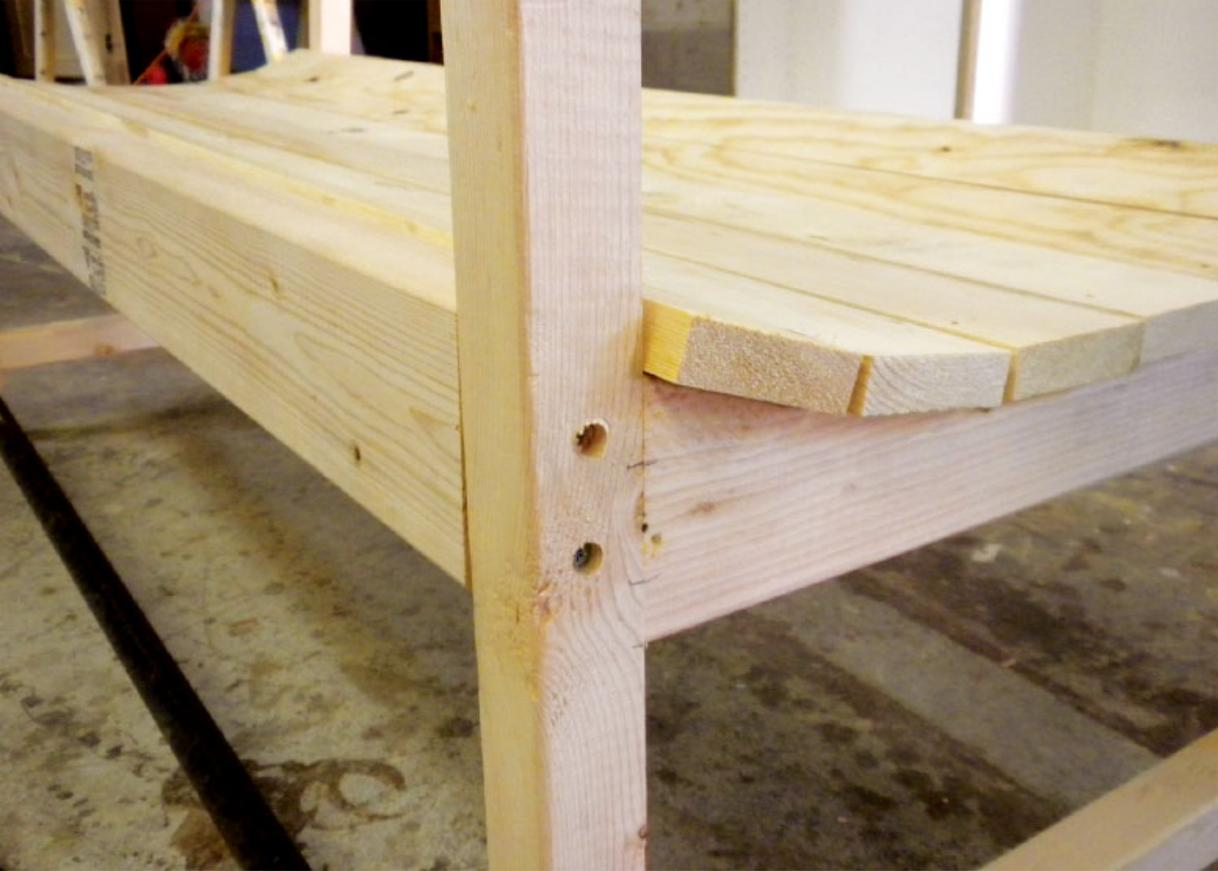
**Step 11** *The stretchers are positioned so that they're top edge is essentially flush with the seat slat closest to them. I secured the stretchers with long screws.*
