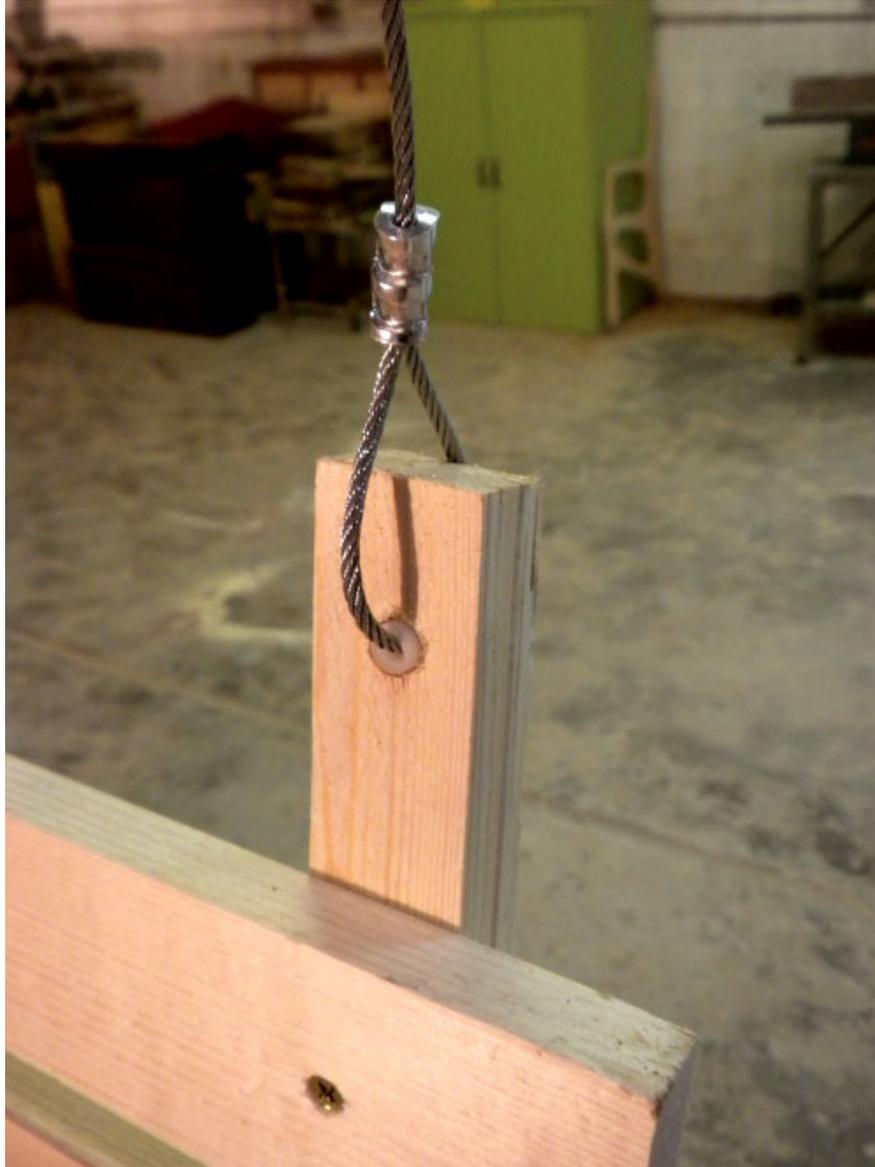
**Step 25** *The cable attachment at the back of the swing was a little different—I inserted a hard plastic ferrule to ensure that the cable wouldn't abrade the surrounding wood.*
