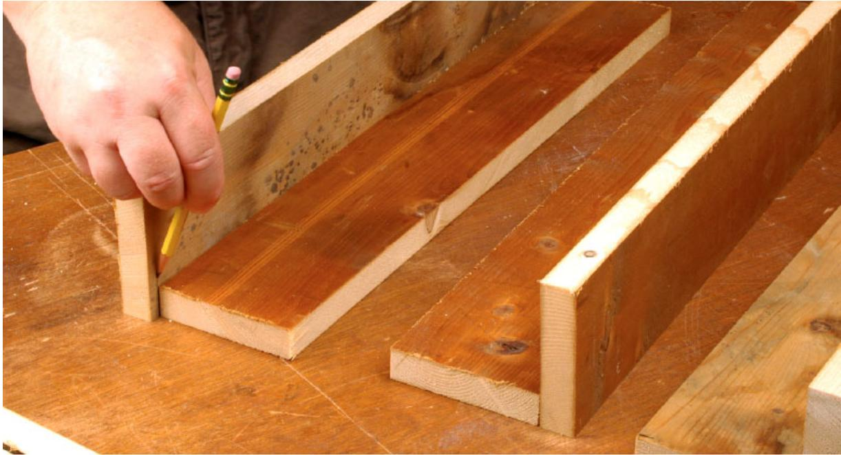
**Step Two** *Transfer the bevel location from the four cut pieces to the side-facing pieces of the legs. Remember that the front and rear legs are mirror images of one another, with the shorter “leg” pair to the rear. The legs are shown above positioned as they will be, with the rear (shorter) set on the left. The L’s will become T’s when the horizontal pieces are screwed to the center of the vertical pieces.*
