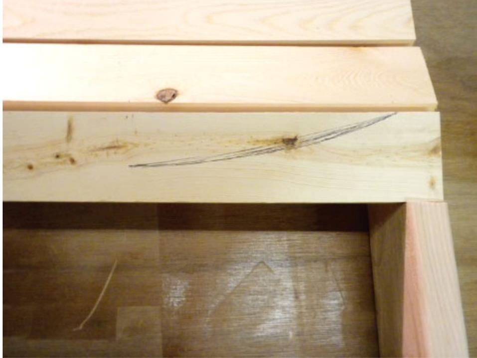
**Step Three** *The back support rail is curved to help create the fan back that is a signature part of the Adirondack's look. My method for cutting this curve is a simple one—I begin by drawing half of the curve (from the outside edge to the midpoint). Leave about one-third of the rail's width intact at the bottom of the curve.*
