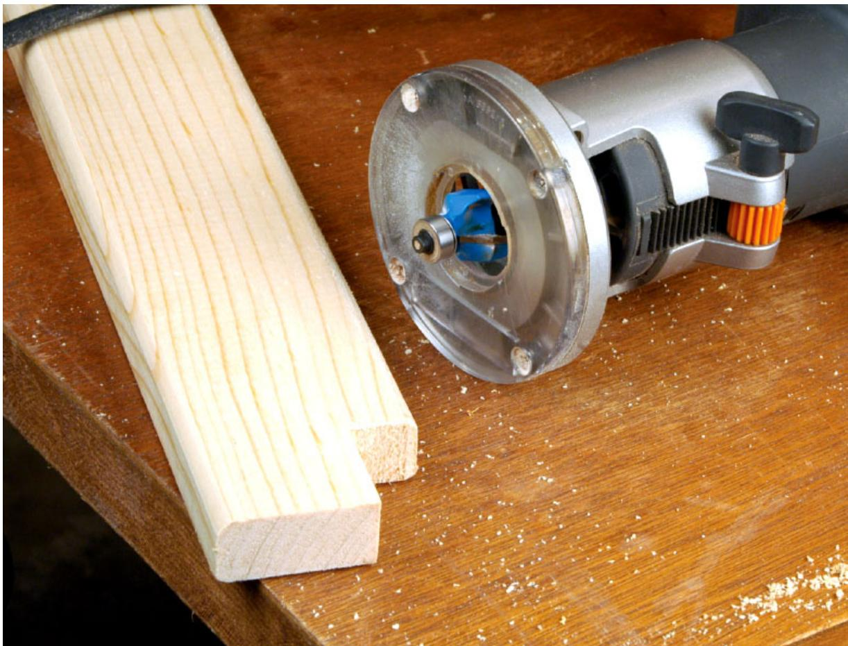
**Step 18** After notching the front seat slat to fit around the legs, I used a roundover bit in my trim router to round the long edges of each slat. Less chance of pinching something
