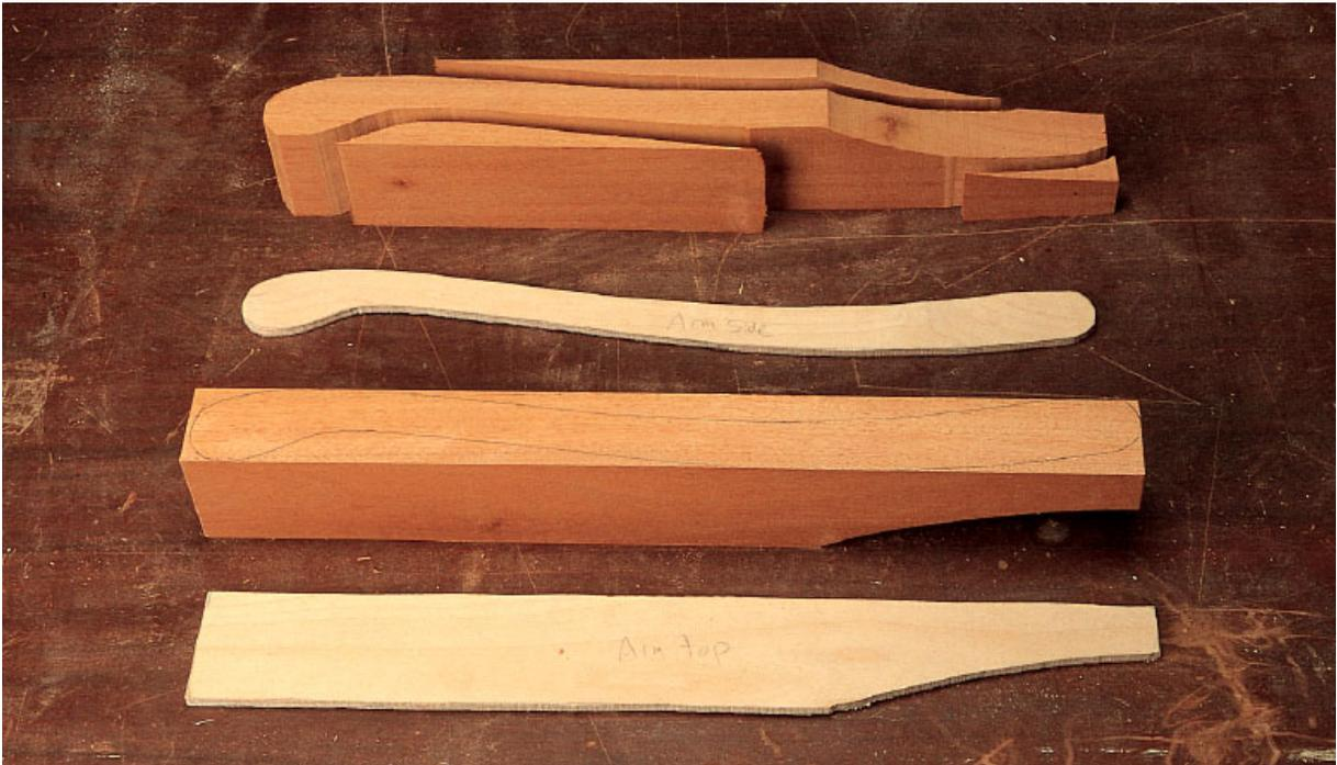
**Step One** On the arms, cut the top surface pattern first (below), then flip the piece onto the inside edge and make the second cut (above). Be sure to make a left and right arm.
