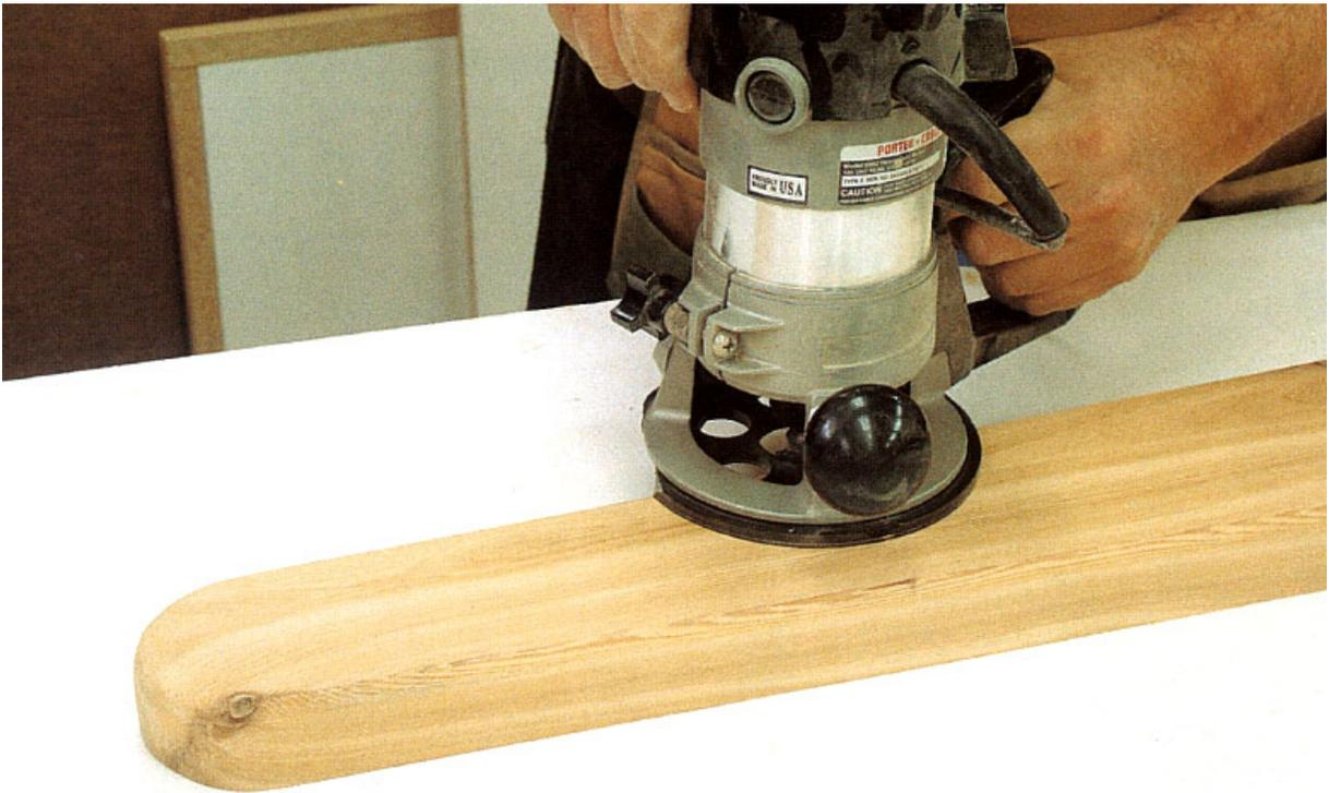
**Step One** Prepare the two sides (A). Cut the radius ends and taper with a jigsaw or band saw. Then round over the edges and ends with a  $\frac{3}{8}$ " roundover bit in a router.
