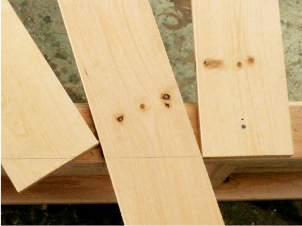
**Step 19** *I used a power planer instead—talk about quick and easy! Taking off about  $\frac{1}{32}$ " per pass worked well.*
