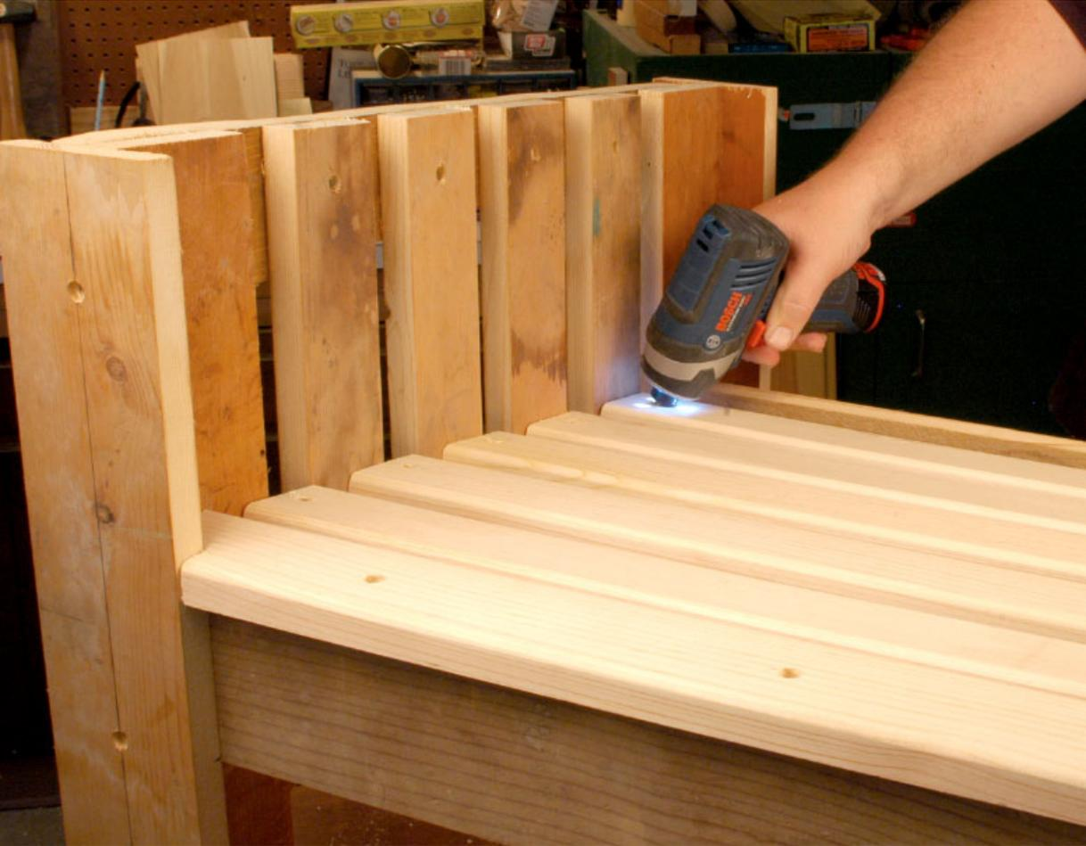
**Step 20** *The rest of the seat slats are screwed into the seat supports on either side.*
