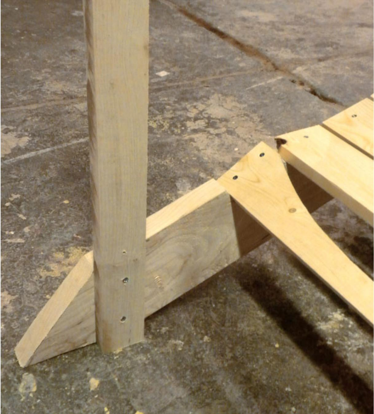
**Step Ten** *The rear legs can be secured to the chair frame at this point. Hold the back edge of the leg flush to the top of the bevel at the rear of the seat support.*
