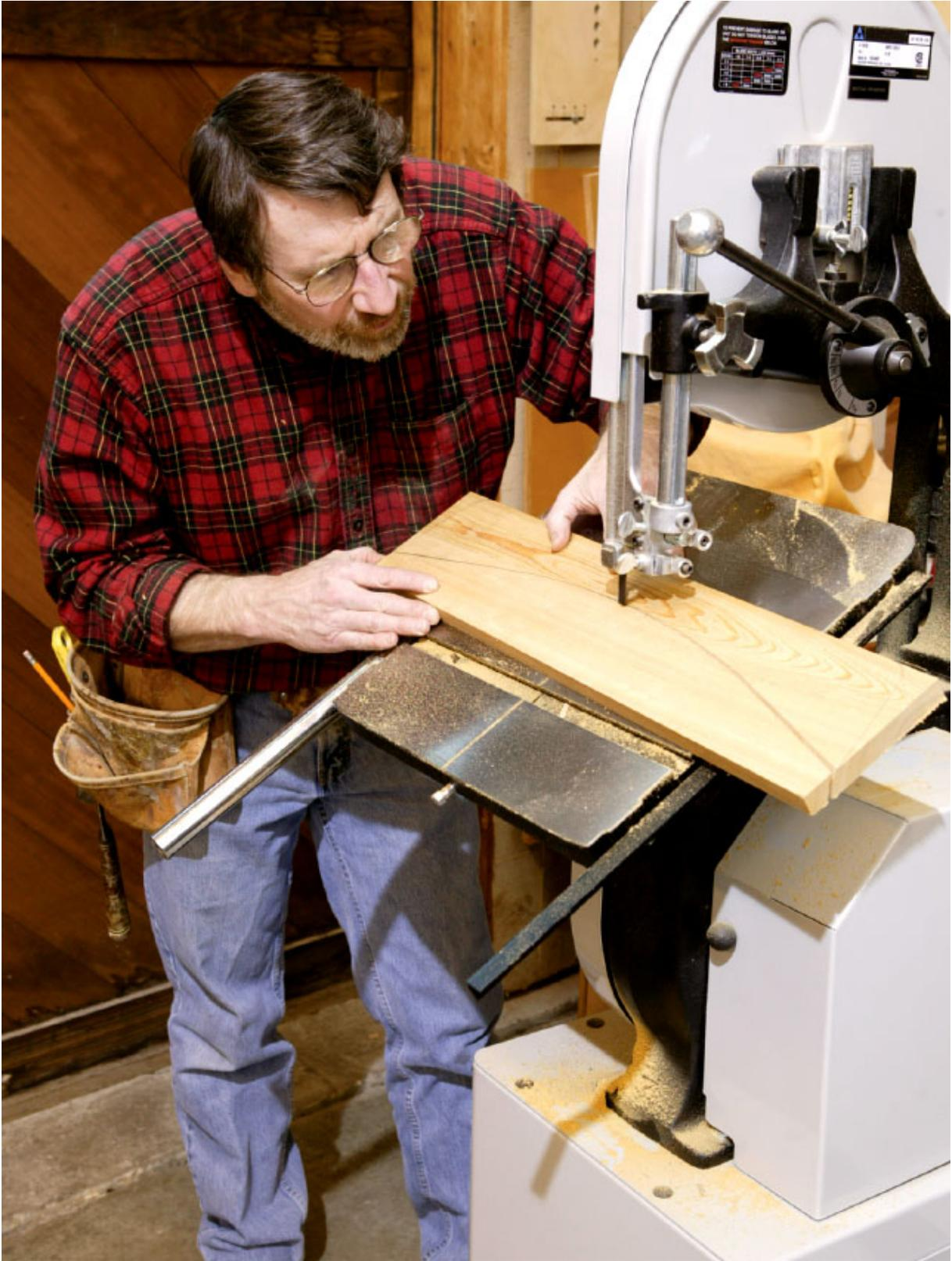
*Cut the upper rear crosspiece's inside curved edge at a 30° angle. Then return the band saw table to 0°, or square, and cut the round ends.*
