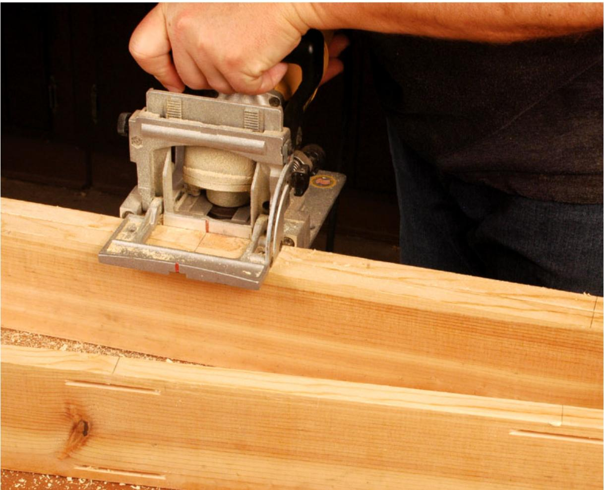
**Step Nine** Moving on to the posts for the legs, I marked biscuit locations for six biscuits (three per edge) along the post-piece edges. I found it easier to make this cut with two of the pieces held together to provide more bearing surface during the cut.
