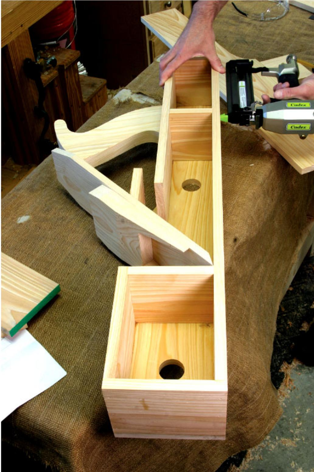
***This Plane Is Hollow.*** Glue and nail all the interior pieces as shown before you screw the second sidewall in place.
