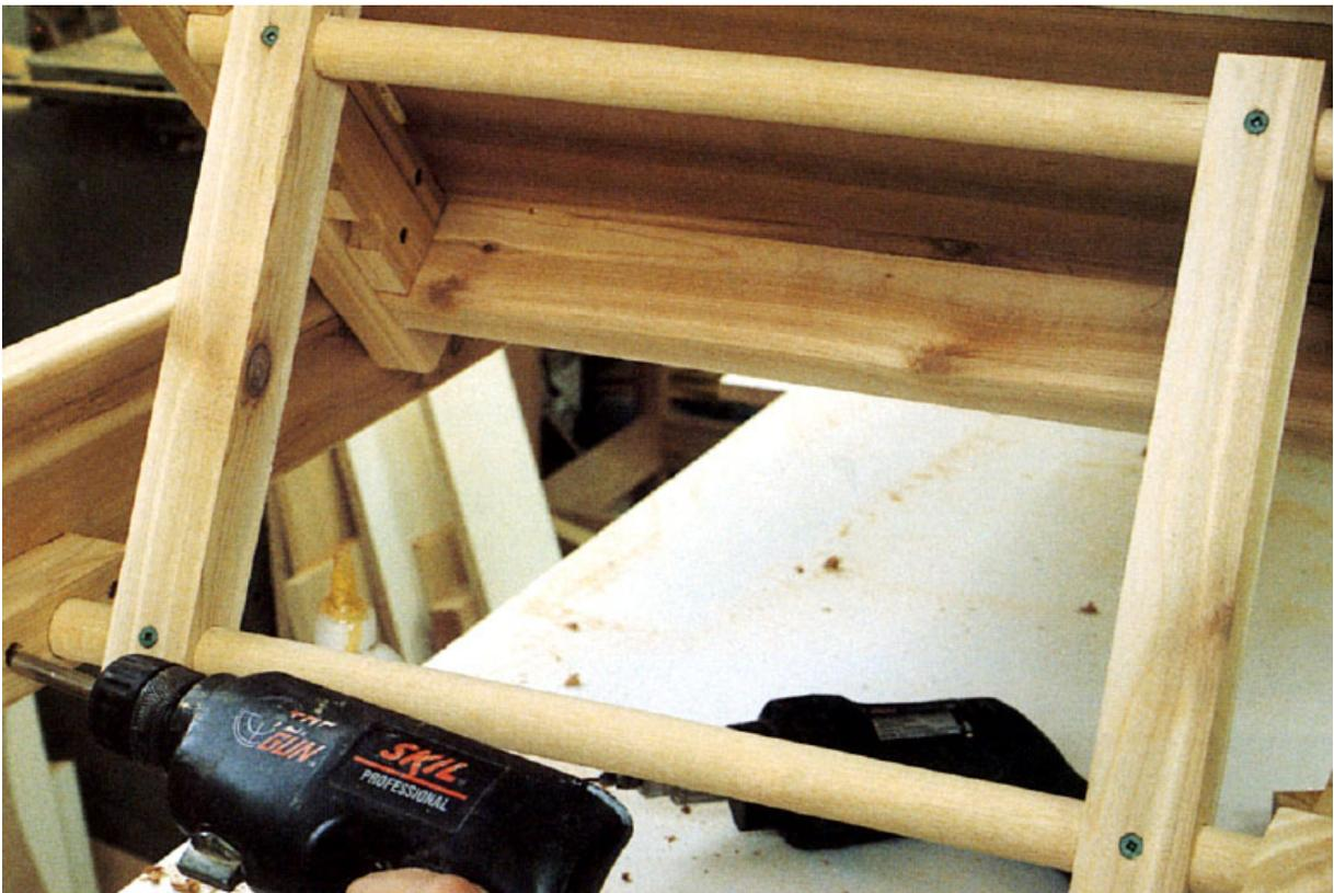
**Step 13** *The adjustable support arm is constructed with two sides (P), two position dowels (R), and two pivot blocks (Q). The pivot blocks require a 1"-diameter hole centered on the block. And the support arm sides require a 1"-diameter hole centered 1" from each end. The pivot blocks should rotate freely on each dowel, and the arms are “pinned” to the dowels with 1¼" screws. Then as shown here, install the support arm assembly by attaching the pivot blocks to the*
