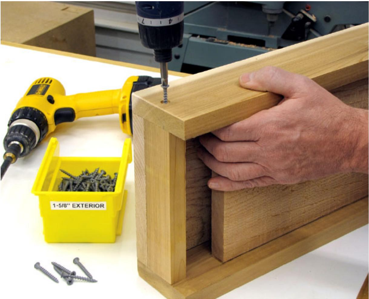
**Figure 5** *Secure the bottom in place with two screws only. You'll need to remove the bottom from time to time for cleaning.*
