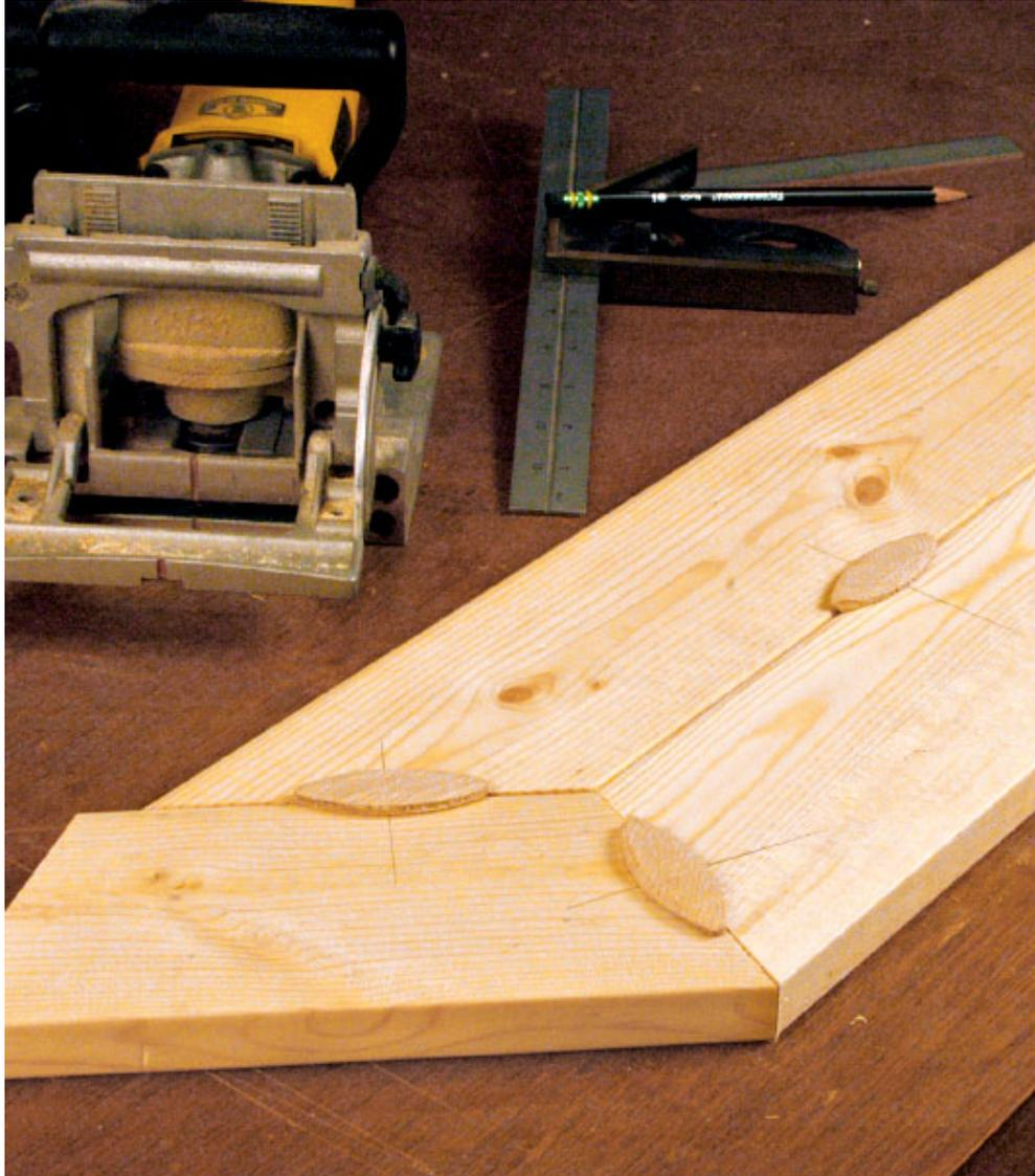
**Step 21** *Assembly starts with one long frame piece and the adjoining two corner pieces. Fit the first slat into that space once the frame is established, then mark and cut for biscuits.*
