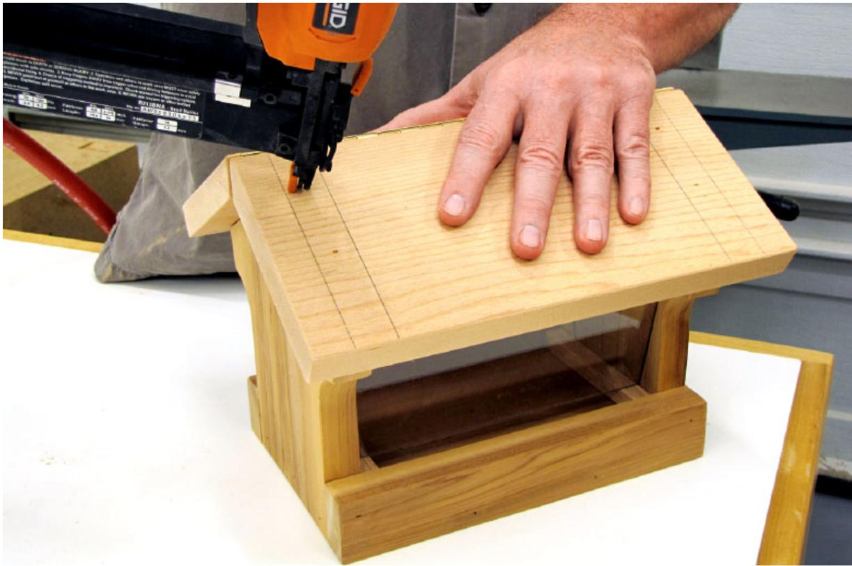
**Figure 9** Lightly draw (mine are dark so you can see them in the photo) locating lines on the roof sections, then glue and nail the roof in place.
