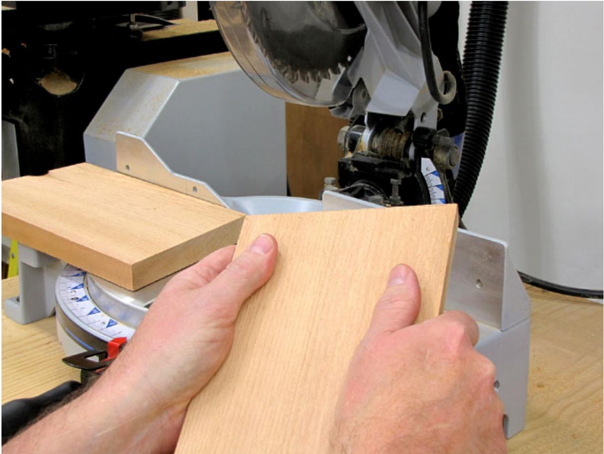
**Figure 1** Either a miter saw, a handsaw or a table saw with a miter gauge can be used to cut the miters on the parts.
