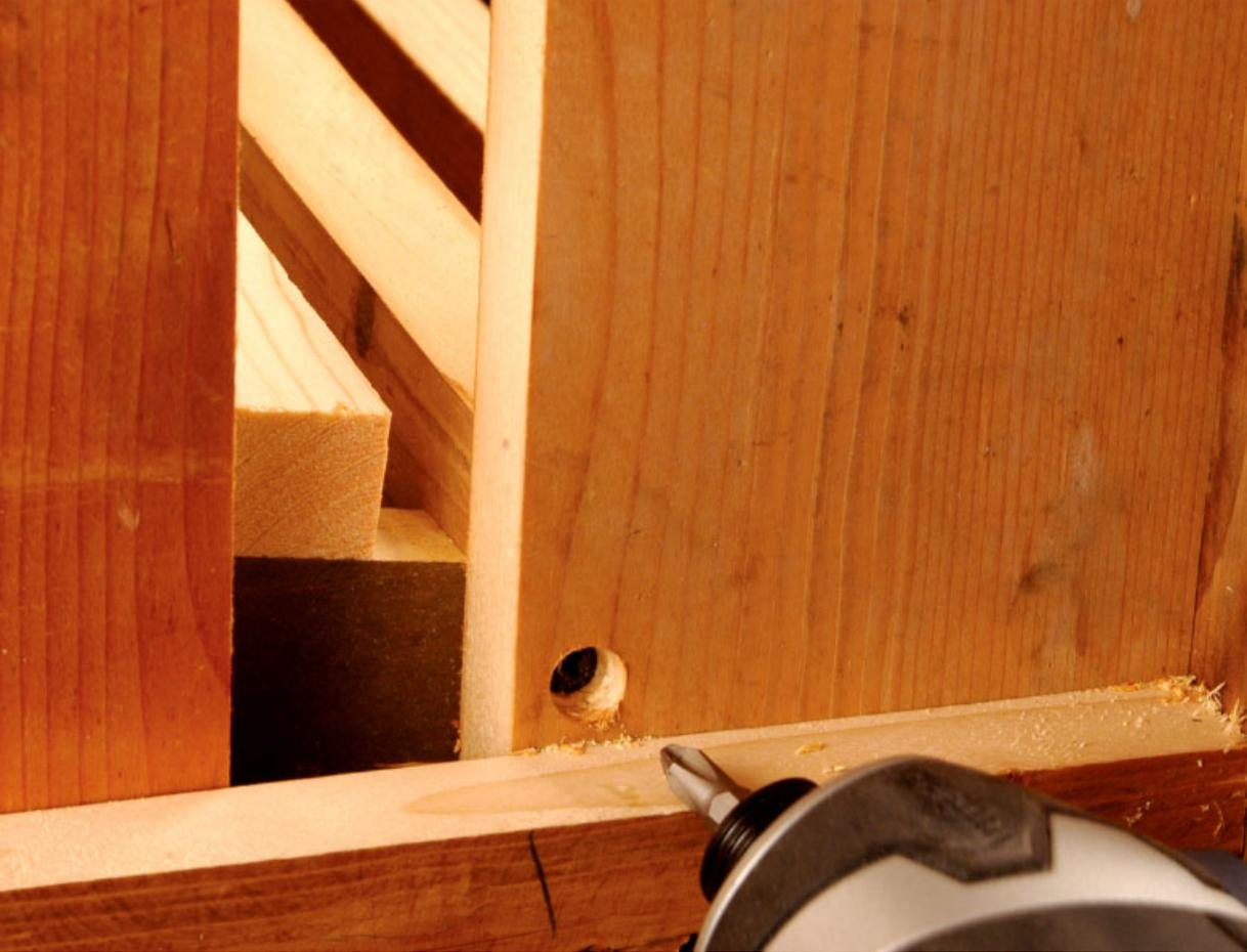
**Step 17** *At the rear of the seat support, a 1 × 3 is screwed in place between the two legs. Another screw from the rear holds the piece against the ends of the supports.*
