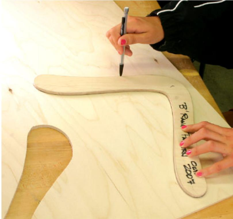
***Start With A Simple Pattern.*** *Melanie Jonas traces a bi-wing pattern onto 1/4" plywood. The next step is to head over to the band saw. This pattern was so popular that I made a wooden pattern for the students to be able to trace.*
