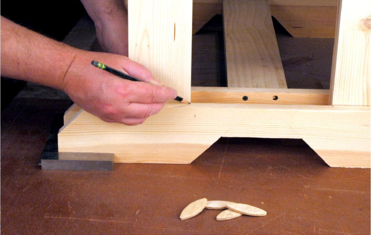
**Step 16** To double check the alignment, I put a couple of biscuits (without glue) in place in each half of the posts and pushed the two halves together. I then marked the post location on the outer bracket feet.
