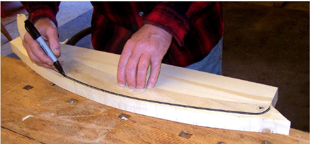
**Marking Multiples.** *A template ensures that both frames match, and it speeds the process if you are making several chairs.*
