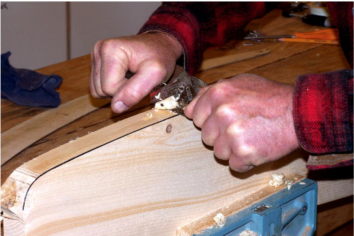
***All is Fair.*** The spokeshave is ideal for removing saw marks and refining the curves. I find it easier to shape the outside before cutting the inside curve.
