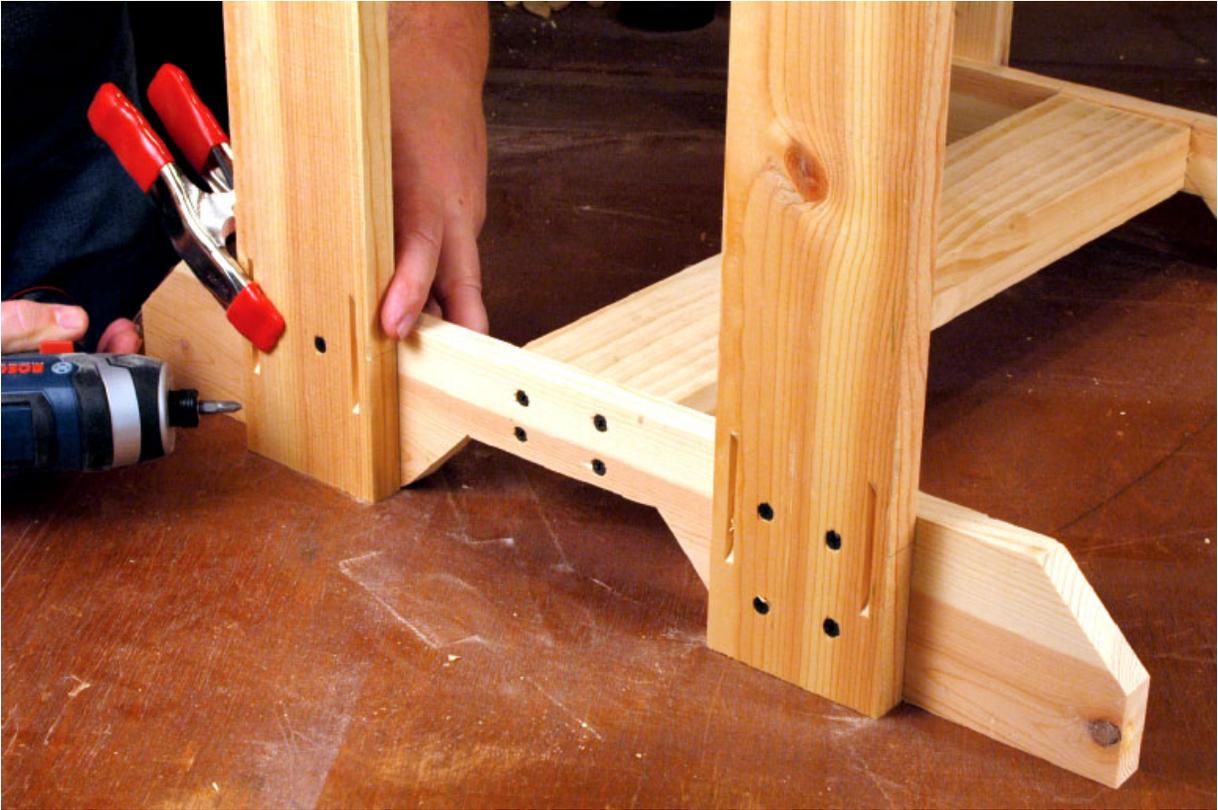
**Step 11** Starting with one end, I screwed one post in place with four screws, then put only one screw in the second post.
