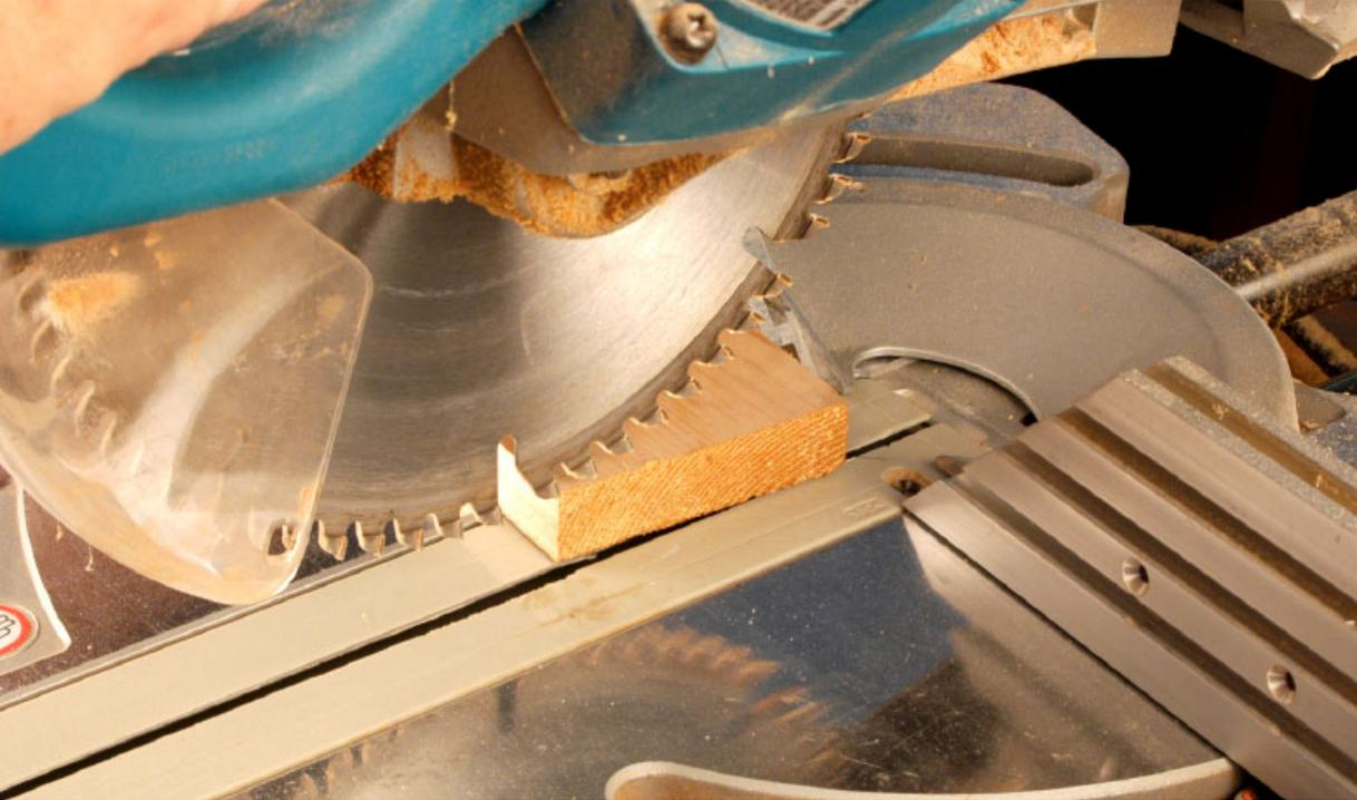
**Step Three** After marking the bevel locations, cut the other four pieces on the flat.
