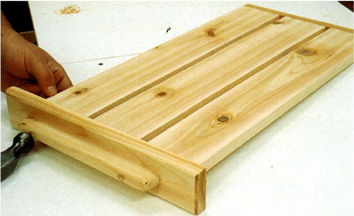
**Step 16** Build the pullout assembly as detailed. Attach the end caps (W) to the table boards (V) with glue and nails. Prepare both the pullout face (X) and handle (Y) by rounding over the edges. Then attach the pullout face to the table with glue and screws through the face into the end caps. Secure the handle with 2" screws in counterbored holes to the pullout face.
