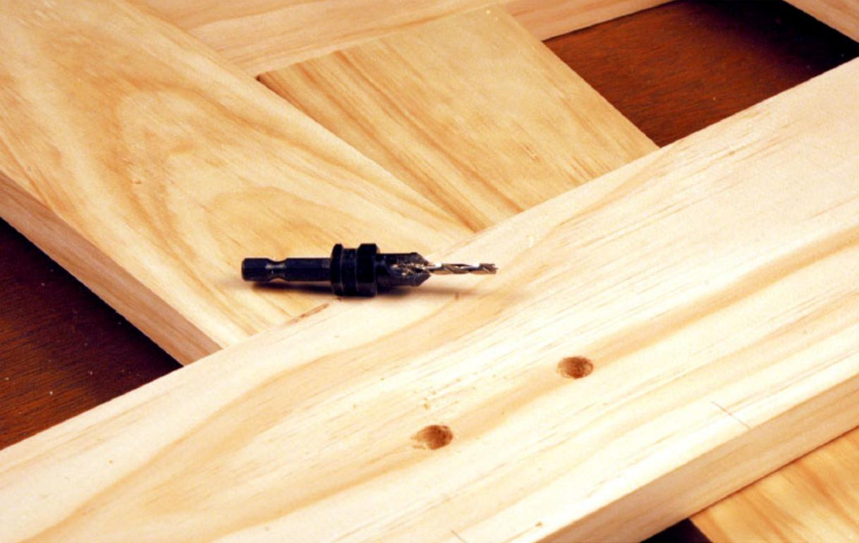
**Step Six** *The four stretchers are screwed in place through the sides. I used my countersinking pilot bit to make the clearance holes, anticipating plugging the holes afterward.*
