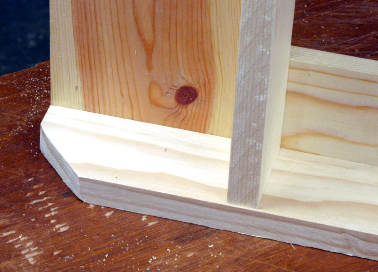
**Step 24** *The rest of the seat slats are screwed into the seat supports on either side. A 45-degree cut at the bottom of the back allows the back to swing to full-back position.*
