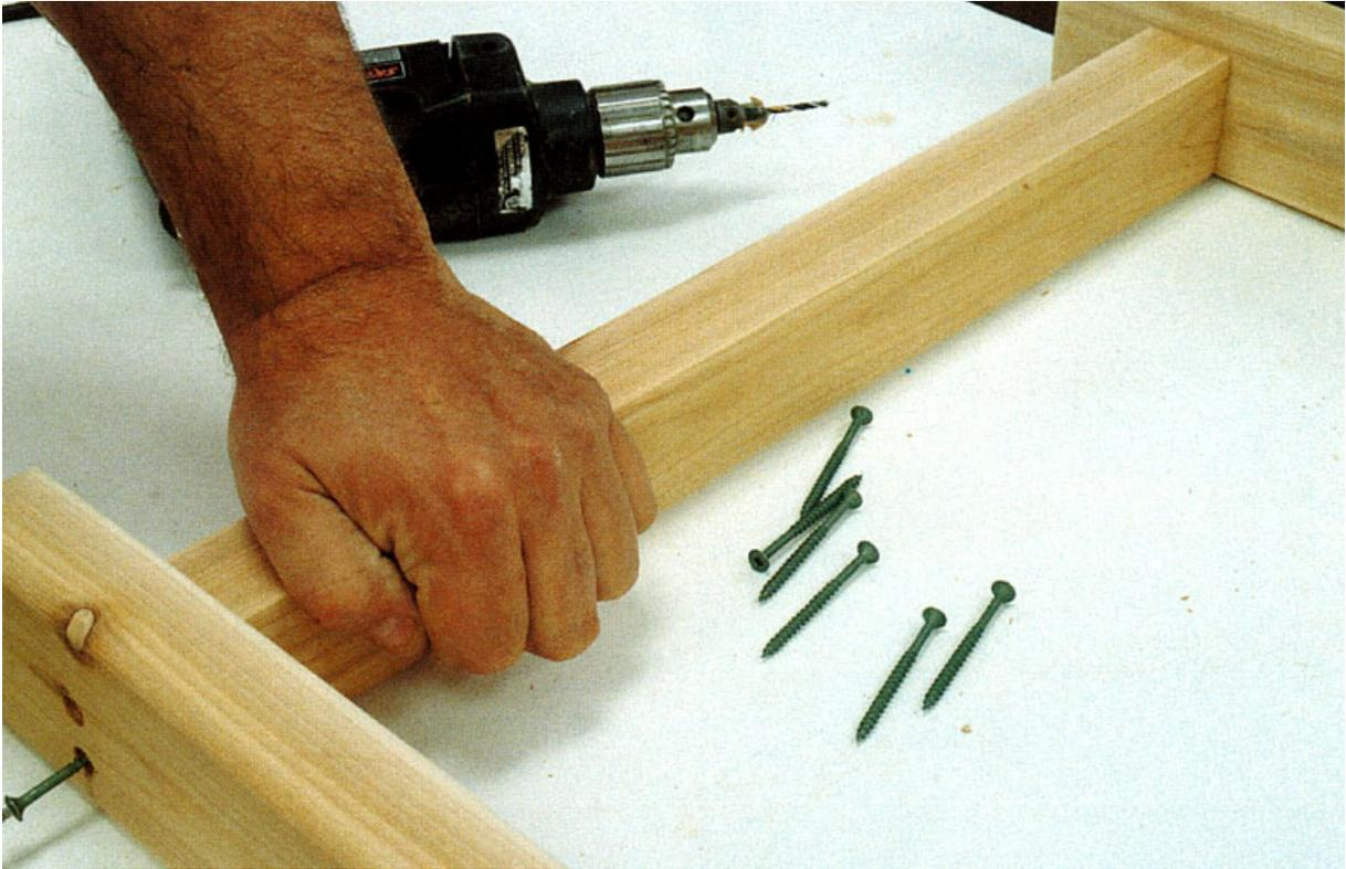
**Step Eight** Cut the two back sides (G). Sand and round over all the edges on both pieces. The two back cross braces (H) join the back sides. They are secured with glue and 2½" screws. As shown here, drill and counterbore screw holes through the outside face of each back side and drive the screws into each brace. Locate them 2" in from each end and flush with the bottom edge of the side boards.
