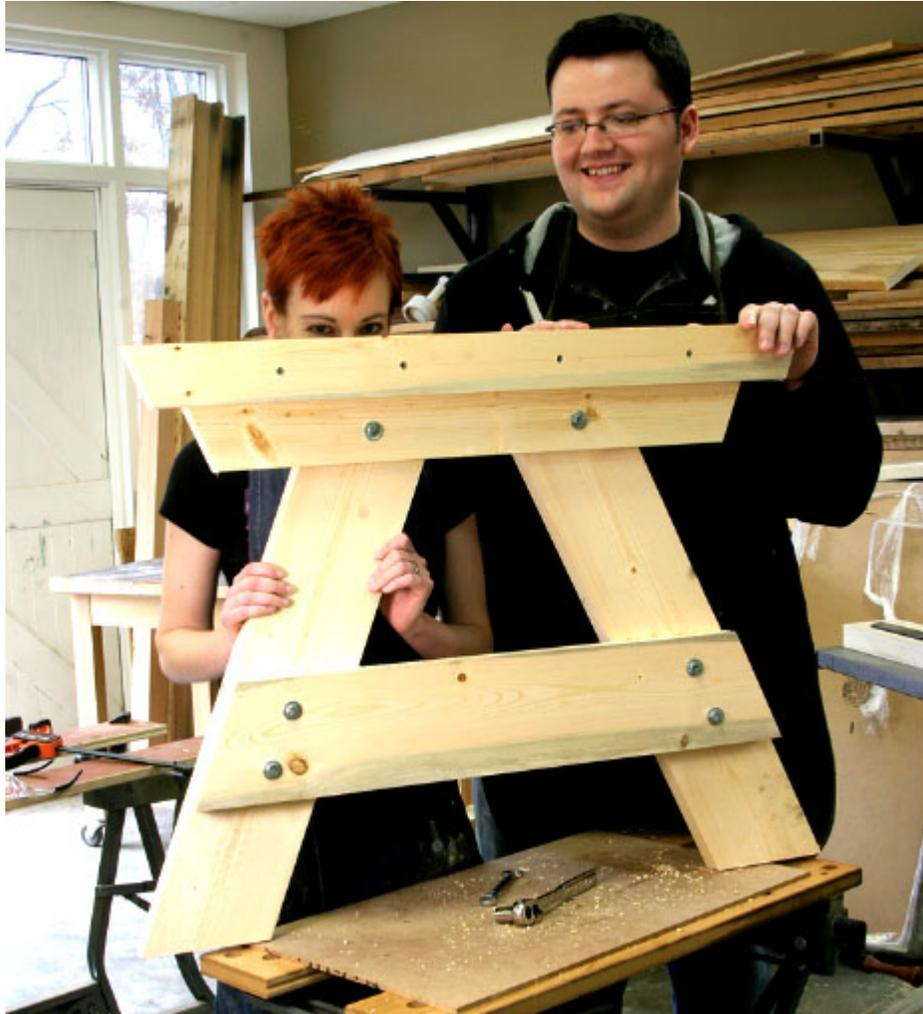
***Ends Are The Beginning.*** Make the two end assemblies first. Then attach the top and diagonal braces.
