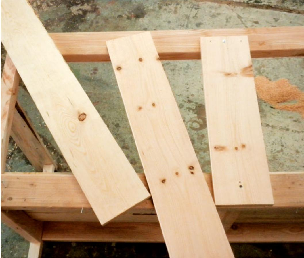
**Step 18** People often recommend flattening the edges of the laminations on the jointer. This wasn't practical in this case because of the shape of the side, but it is an efficient method for simpler shapes.
