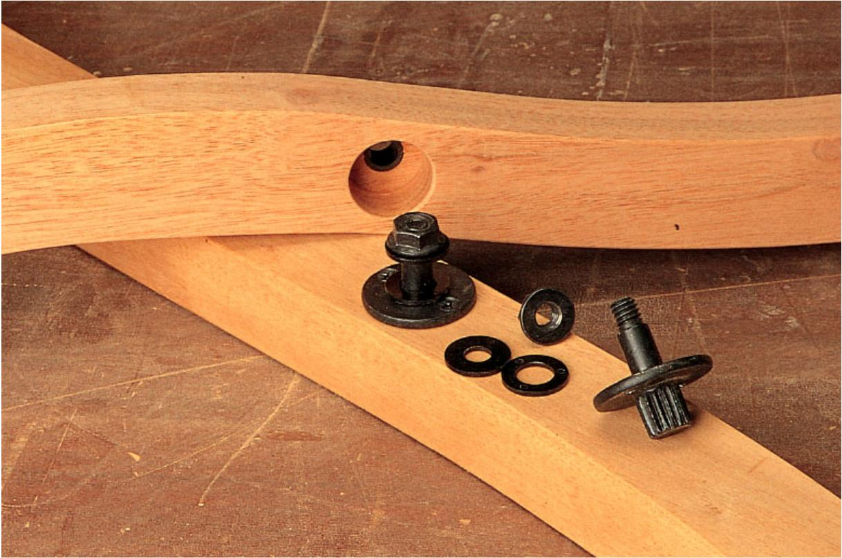
**Step Two** *The pivot hinge hardware allows the chair to fold. But pay careful attention to left, right and inside and out when drilling the two-step holes.*
