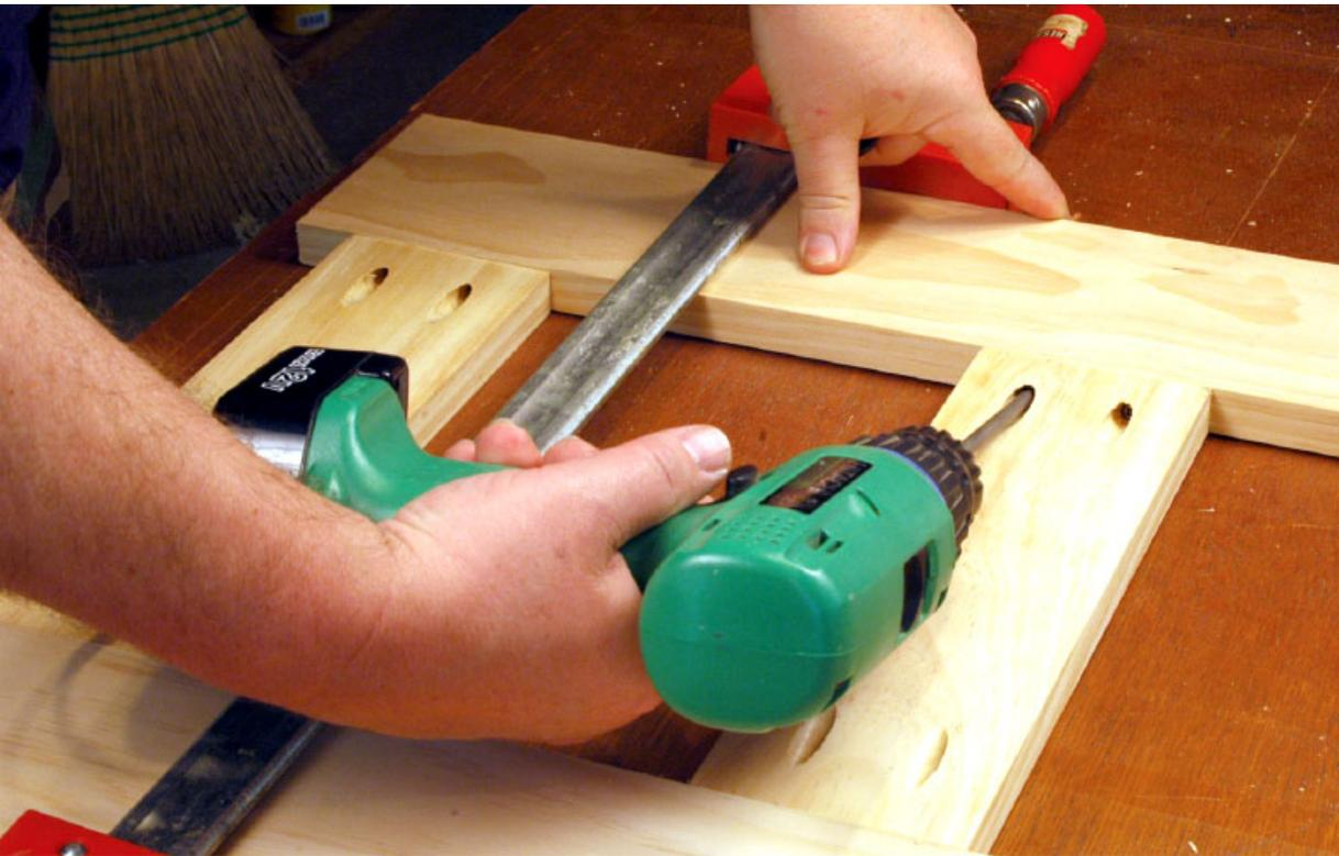
**Step Three** I used a parallel jaw clamp to hold each side frame tightly together as I inserted the screws.
