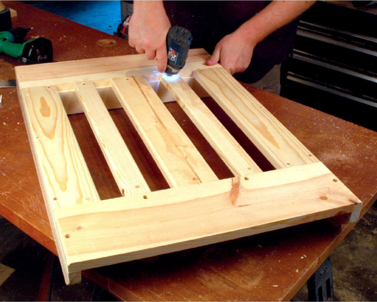
**Step 25** *The rest of the seat slats are screwed into the seat supports on either side. The back slats are then screwed in place.*
