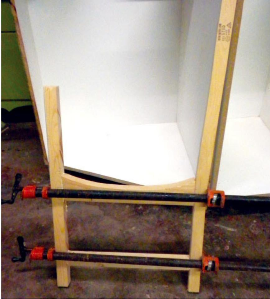
***Step Six*** Two clamps are sufficient to ensure good, even clamping pressure.
