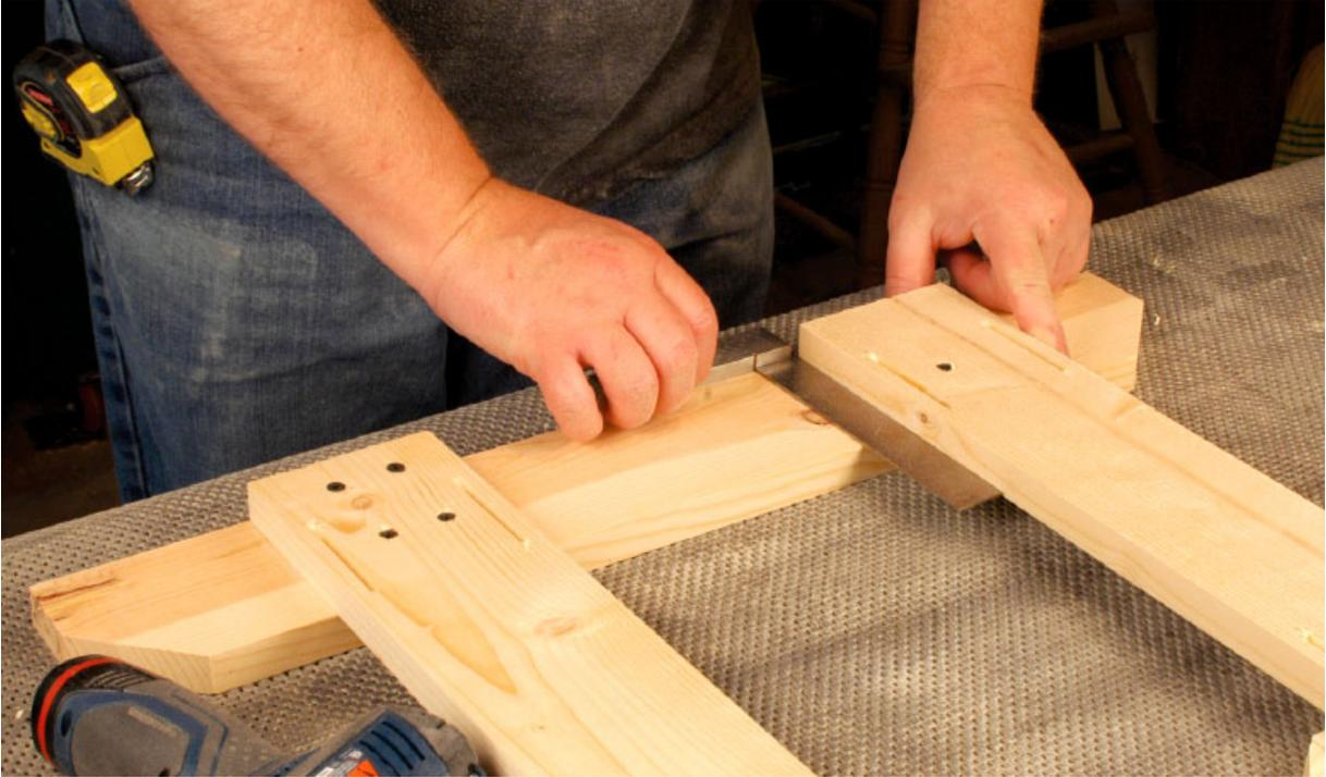
**Step 15** I then screws the second half of the posts to the top supports only, again checking squareness as I moved forward.
