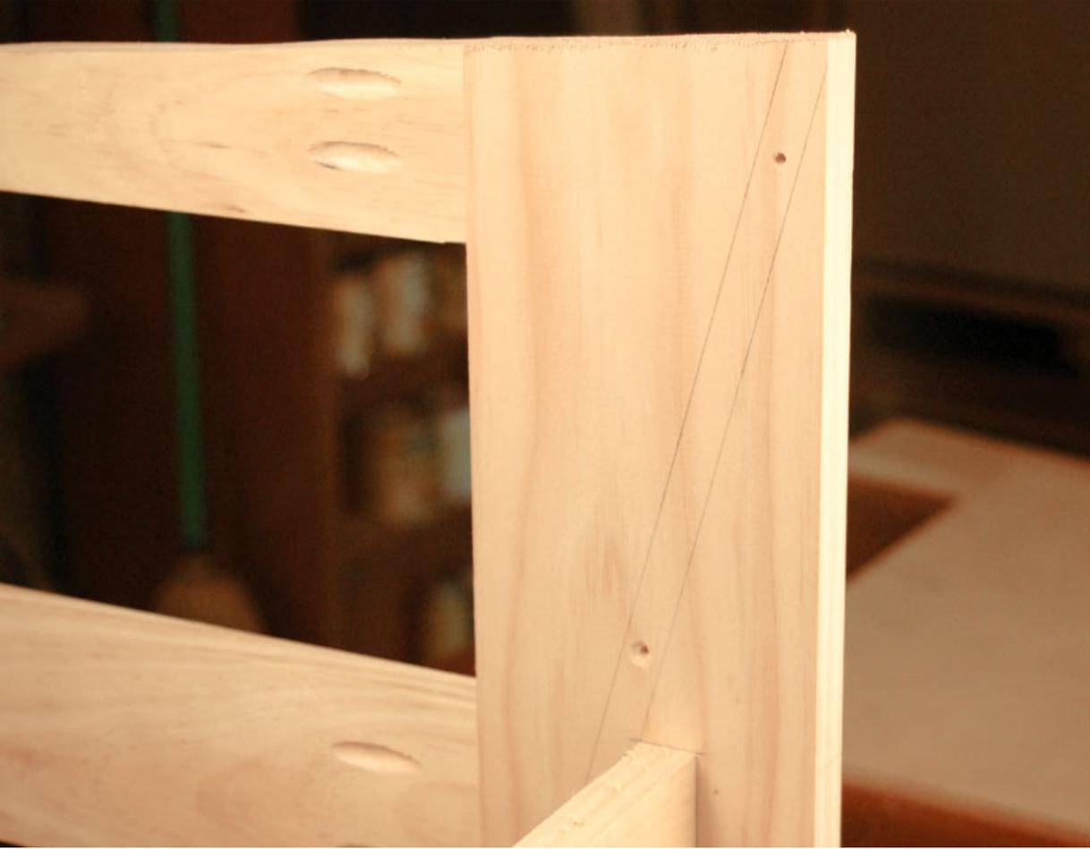
**Step Ten** *With the back removed, I drilled two holes through each side, stopping with just the bit poking through the outside surface.*
