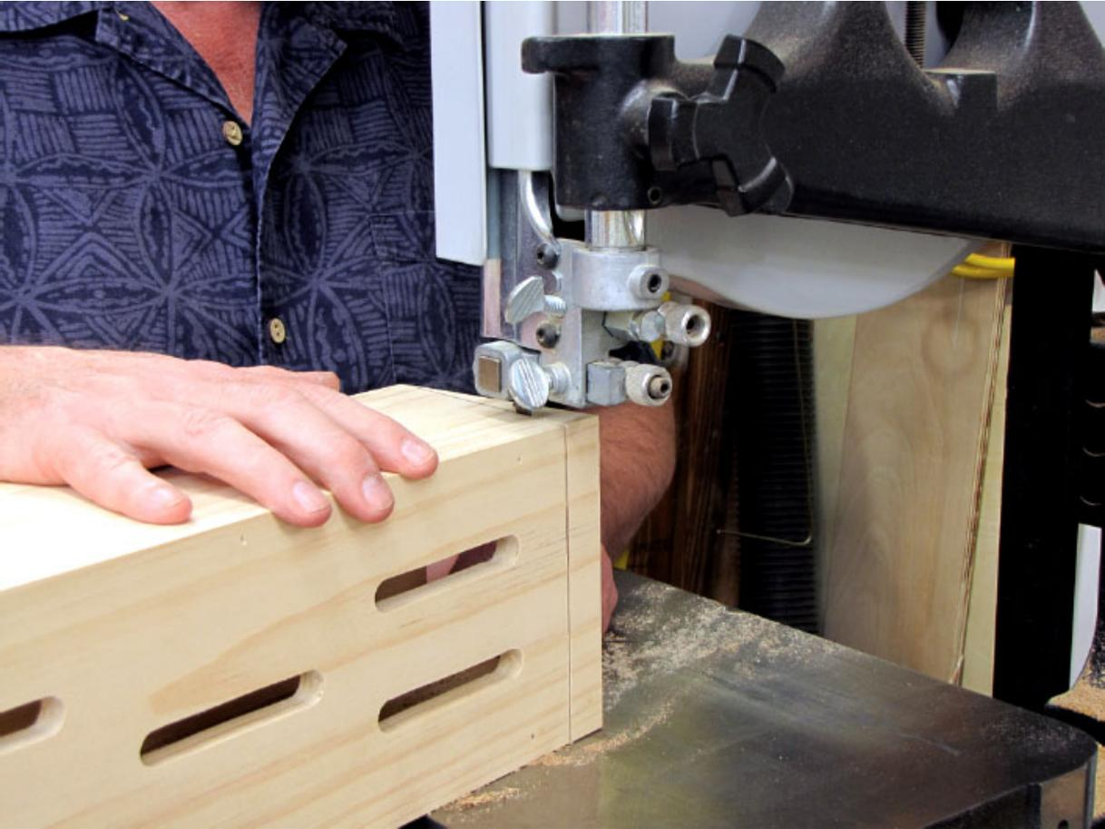
**Figure 3** Assemble the entire box, then cut the 10° top slope on the whole thing at one time using your band saw.
