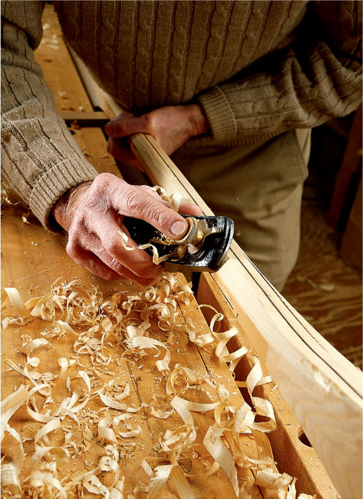
*The block plane will quickly smooth all the edges into a  $1\frac{1}{16}$ "  $\times$   $1\frac{1}{4}$ " oval, as I'm doing here.*
