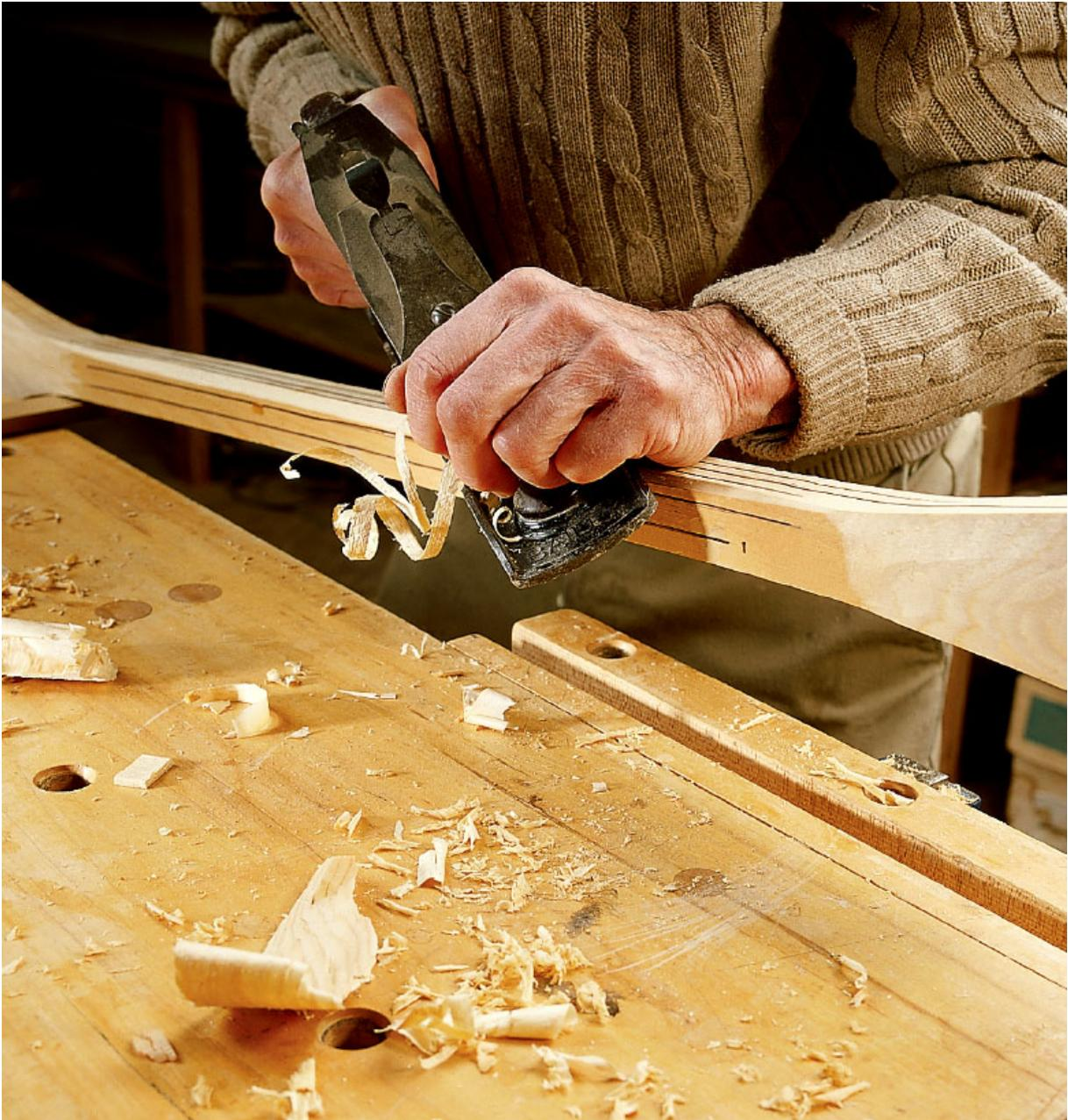
*The shaft is planed into an octagon following guide lines.*
