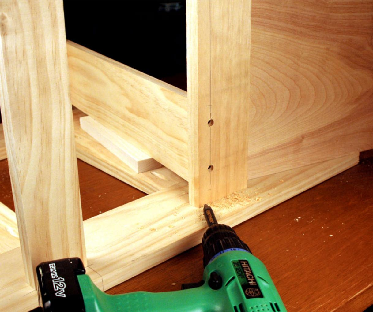
**Step 19** *The slats were then screwed in place through the back stretcher of the chair. I used another scrap piece to hold the side slats  $\frac{3}{4}$ " off the side frame, then evenly spaced the other two slats between them. I used an 18-gauge pneumatic pin nailer to attach the front of the slats to the front stretcher. You could also use countersunk screws, or brad nails for this step.*
