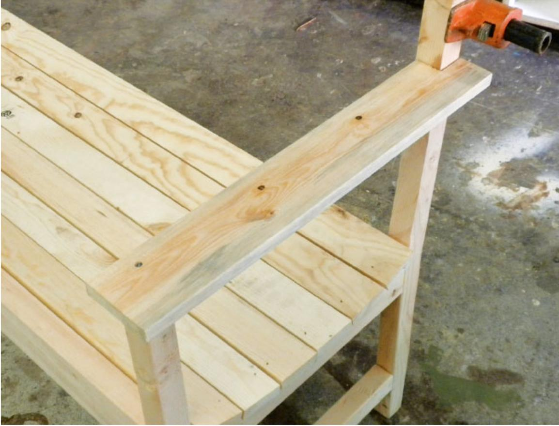
**Step 15** *The arm can be attached to the front leg by simply screwing down through the top of the arm.*
