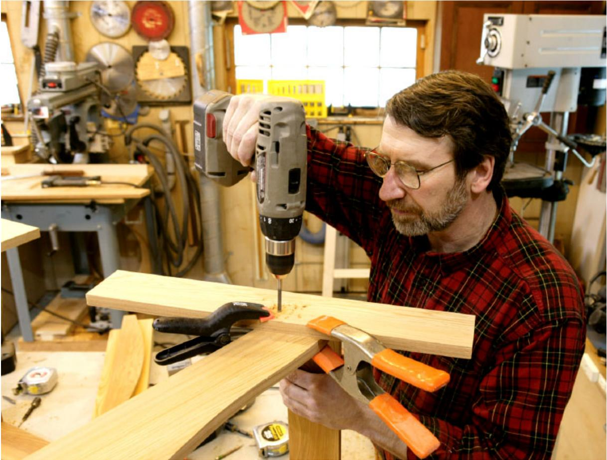
*Drill  $\frac{1}{4}$ " holes through the side members and front leg to accept stainless steel carriage bolts. Use a clamp to hold the parts in position; the leg should be flush to the side's front edge and  $11\frac{3}{4}$ " up from the leg bottom to the bottom edge of the front crosspiece.*
