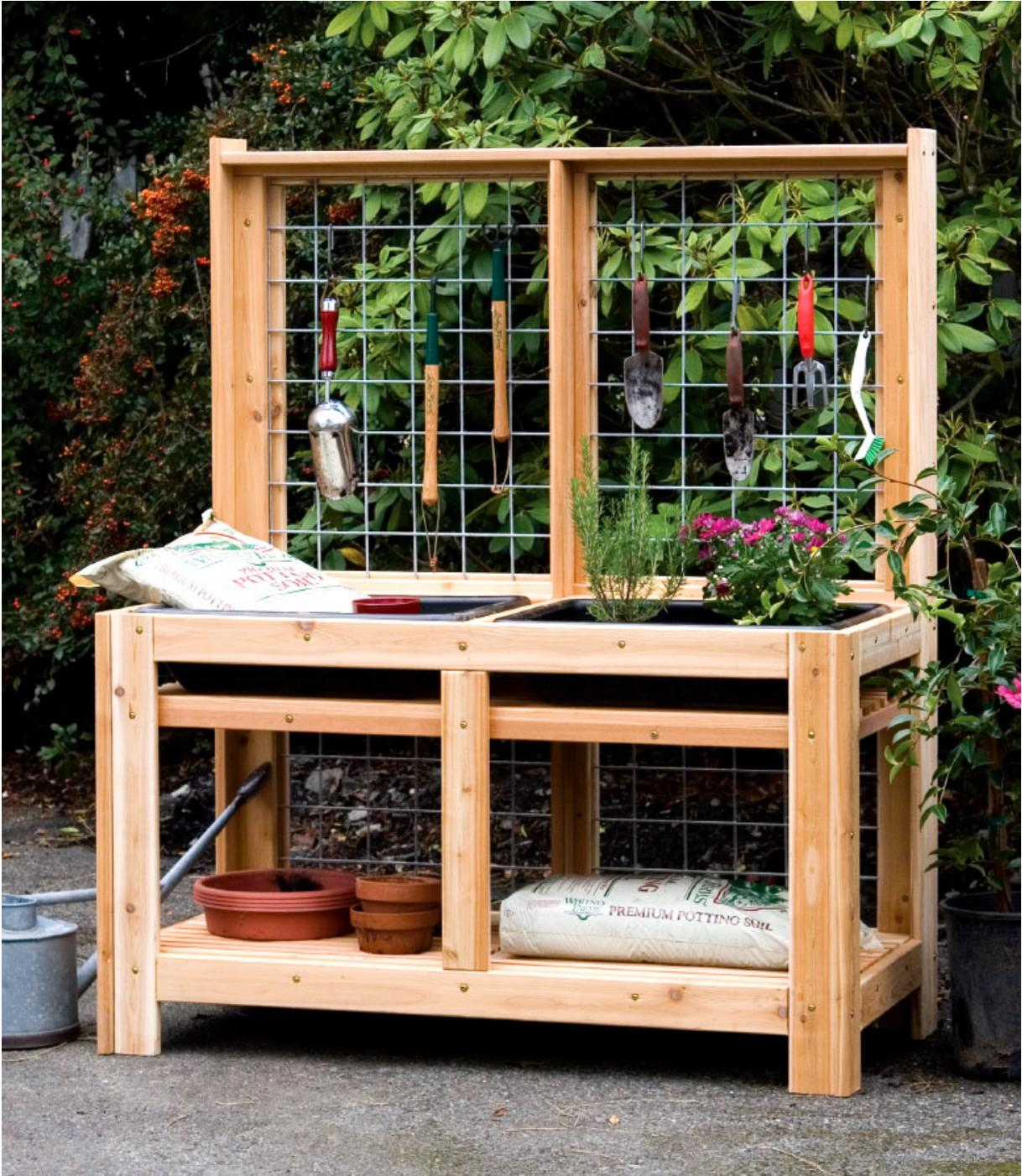
**Step 13** *I didn't apply any finish or sealer to the potting bench. I chose to let the cedar naturally turn to a weathered gray color. I did, however, soak the bottoms of the corner frame pieces in sealer where they rest on the ground.*
