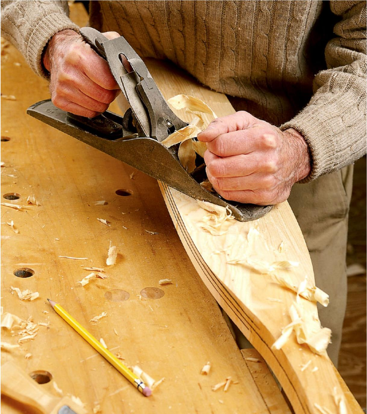
*Use the bench plane to smooth the blade to its final  $\frac{3}{8}$ " thickness. The pencil lines on the edge should give you guidance in this step.*
