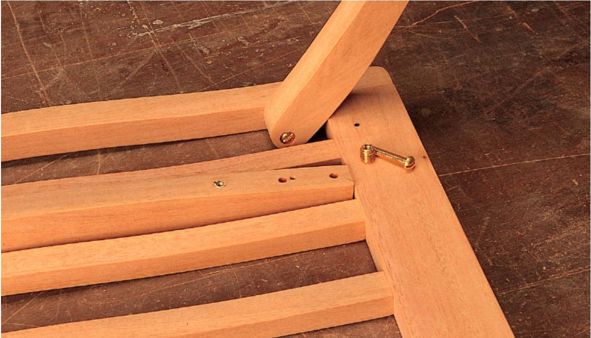
*Attach the footrest legs with threaded inserts and a brass screw.*
