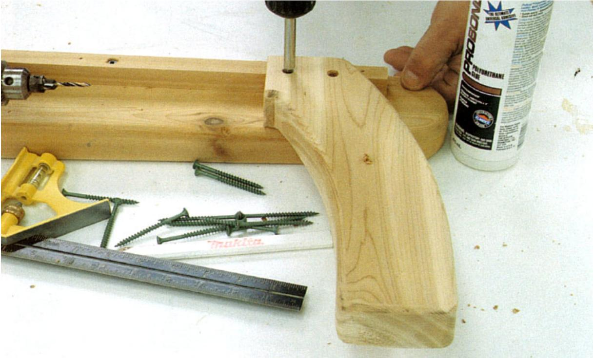
**Step Four** Attach the legs to the side boards using glue and 2 1/2" screws. The outside upper corner of each leg is installed 6" from the side ends. The top flat surface of each leg is 1 1/2" down from the top edge of the side boards.
