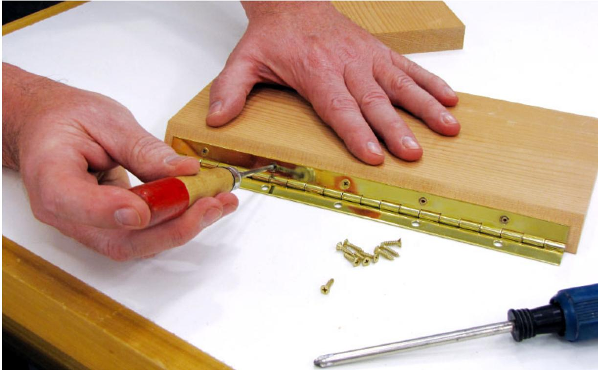
**Figure 8** Use an awl to mark the screw holes. Cedar is soft enough for you to screw into without drilling, but pilot holes are recommended to prevent splitting the wood.
