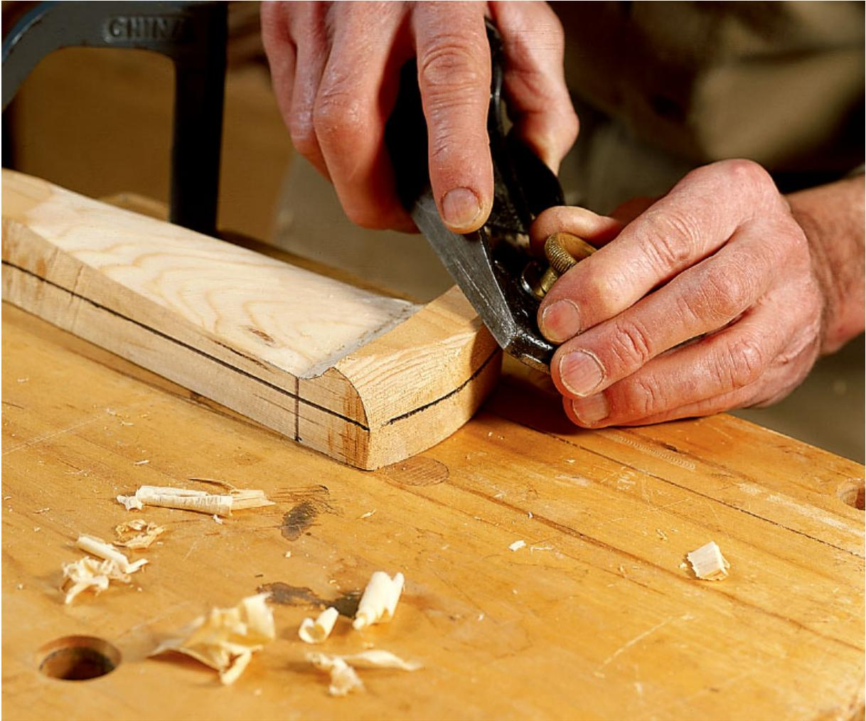
*A block plane will round over a comfortable end. The profile shows well here.*
