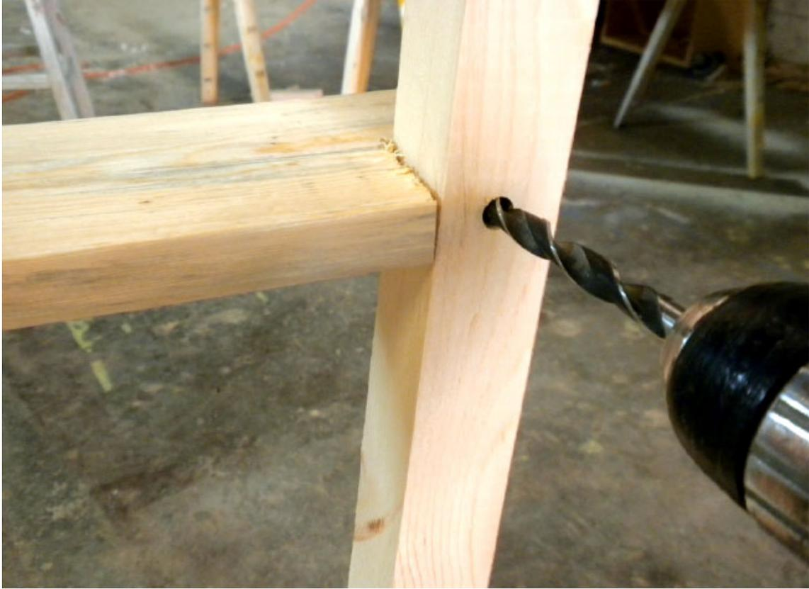
**Step 16** *The back of the arm is easy to attach to the rear leg with a long, counter-bored screw.*
