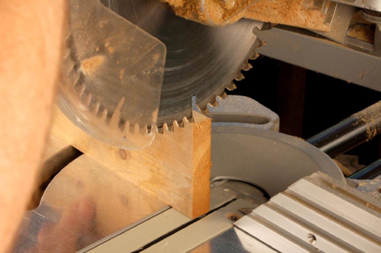
**Step One** *The T-shaped front and back legs have a 5° bevel at the top. It's easiest to cut that bevel before assembly. With the four front- and rear-facing pieces cut to the length given in the cutting list, set the saw for a 5° bevel and trim one end of each piece.*
