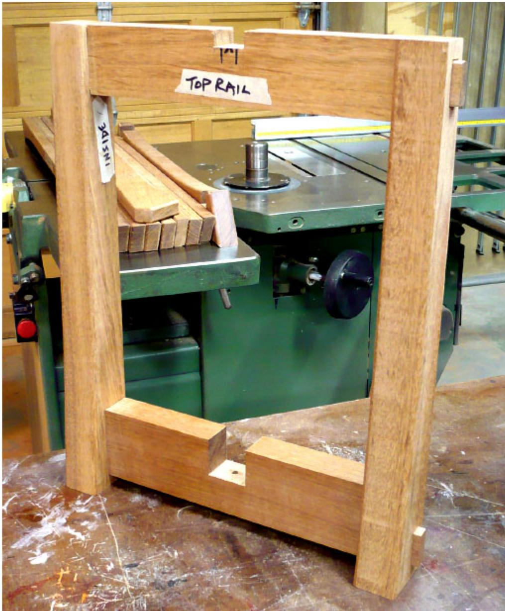
***Test Fit.*** The leg assembly should be test fit to make sure all the bridle joints are correct. Tweak as necessary before glue-up.
