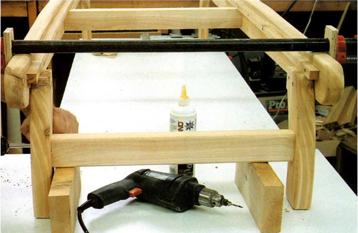
**Step Six** The two leg braces (E) span the distance between each leg set. Cut them to length and round over all the edges with a ¾" router bit. They are attached 4" up from the bottom of each leg, using glue and two 2 ½" screws per joint. Drill counterbored holes on the outside of each leg into the ends of the braces. Fill the holes with wood plugs. The leg braces should be centered on each inside leg face.
