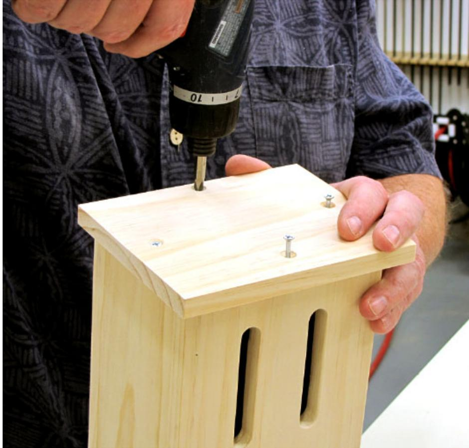
**Figure 4** *Attach the roof with four screws.*
