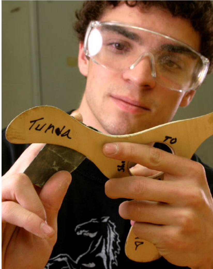
***Fine-Tune With Sandpaper.*** After a couple test flights, Andrew Mihoc adds some refinement to the shape of the airfoils on this tri-blade boomerang with some sandpaper.
