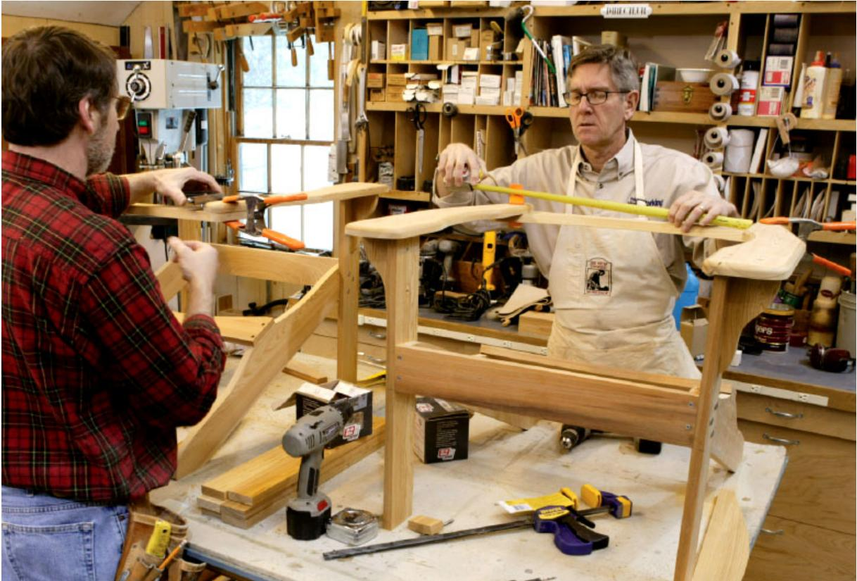
*Hold the upper back crosspiece in place with clamps so that the arms are 20½" apart, then drill each side for two carriage bolts.*
