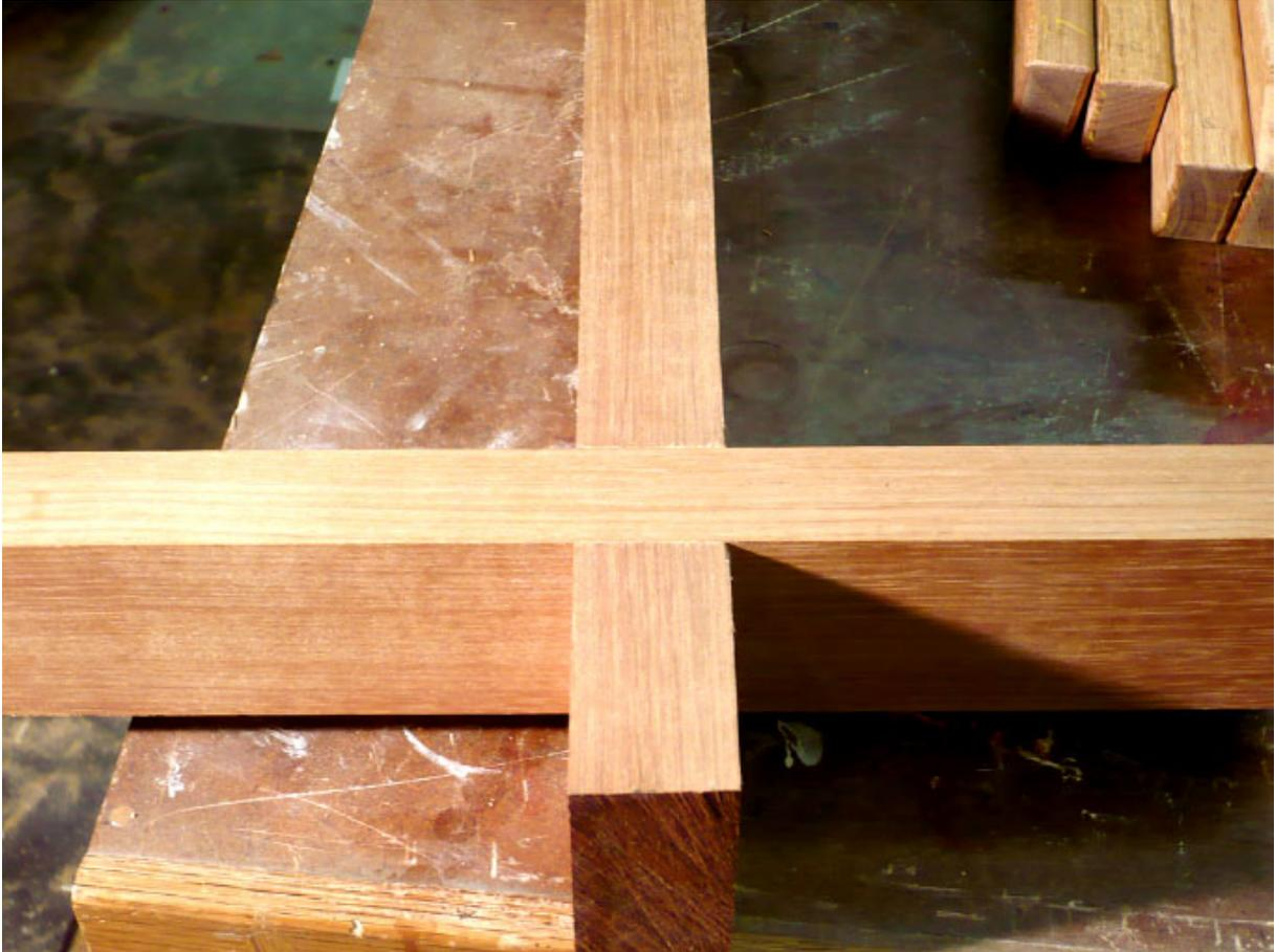
***Tight Is Key.*** Strive for a snug fit between the stretcher and lower rail.
