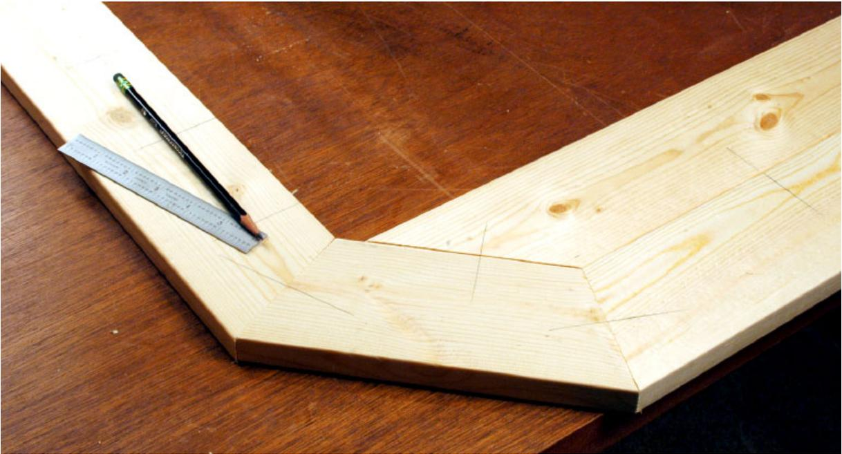
**Step 24** When the outer frame sections are dry, mark the biscuit locations joining the outer sections and the short frame pieces.
