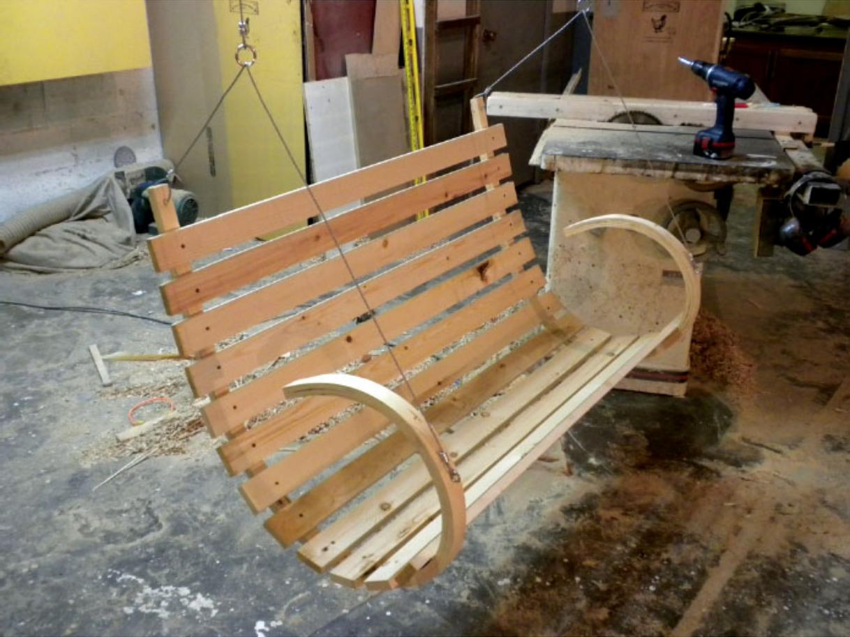
**Step 26** *A small metal hoop serves as a friction-free point of attachment for the cables that will connect the swing to the ceiling. I set the swing up in my shop first to see if it would work.*
