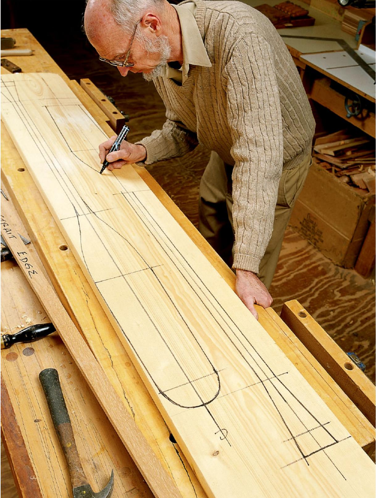
*Layout involves transferring the dimensions from the plans. The centerline with cross lines indicate the major points. Connect the straight lines, then sketch in the curved transitions.*
