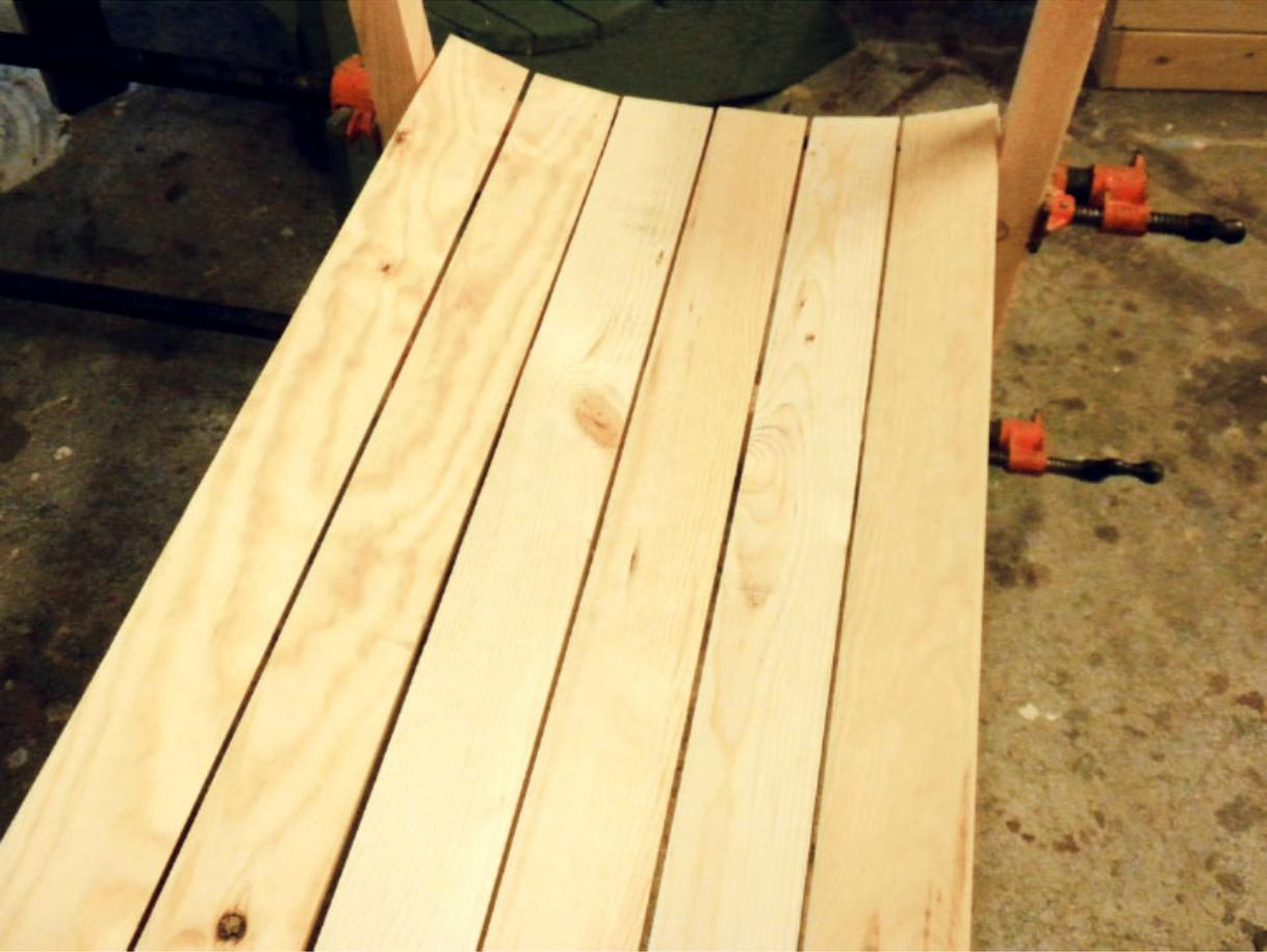
**Step Nine** *Two clamps are sufficient to ensure good, even clamping pressure. I put the front and back slats in first and then just set the middle ones in, maintaining small, even gaps between them all.*
