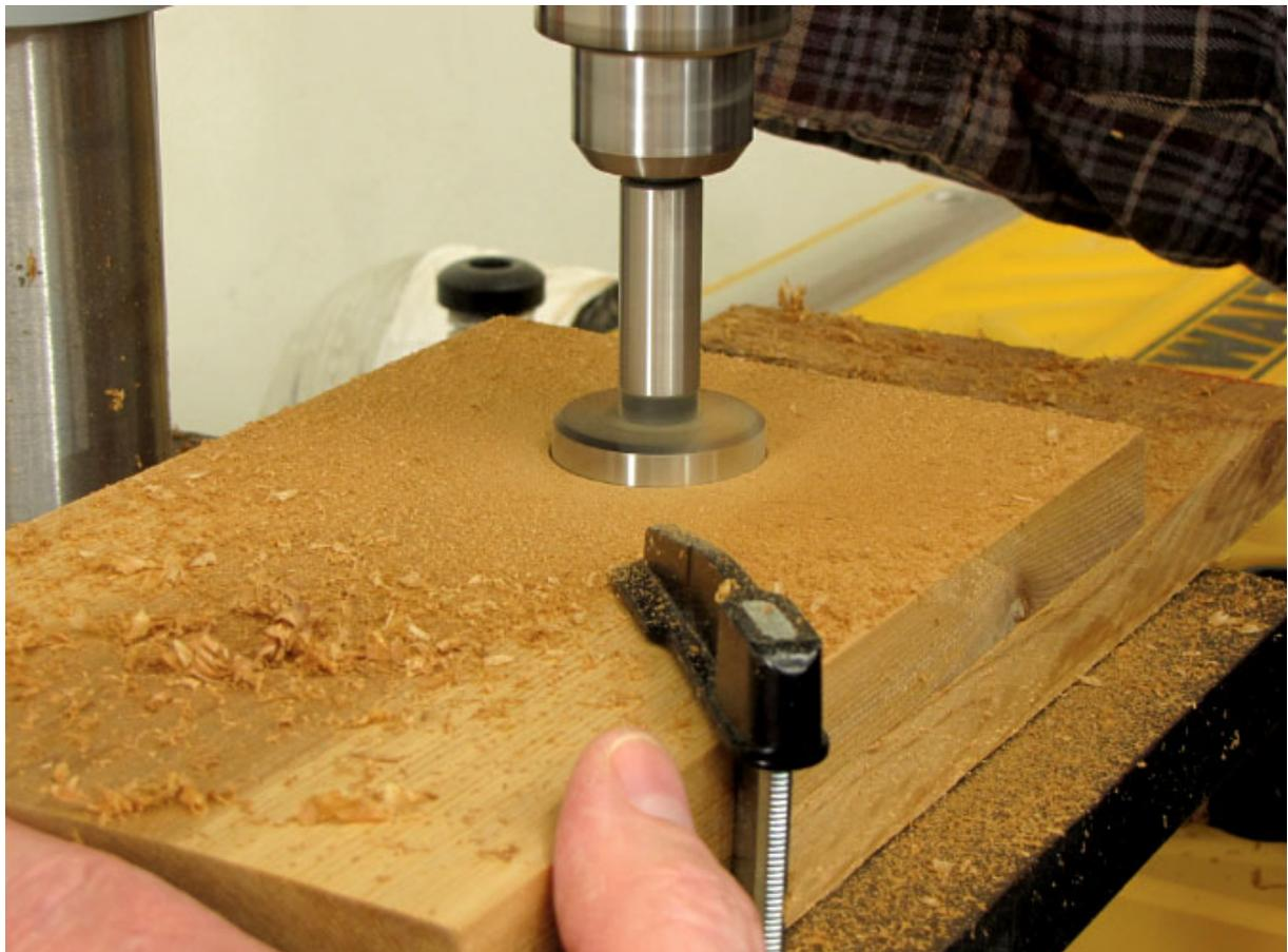
**Figure 4** *A Forstner bit cuts a clean hole with smooth edges. You could also cut the hole using a hole saw.*
