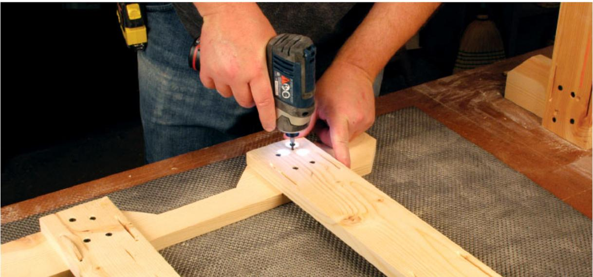
**Step 17** After disassembling the post halves, I finished screwing the posts to the outer bracket feet from the inside face of the post halves.
