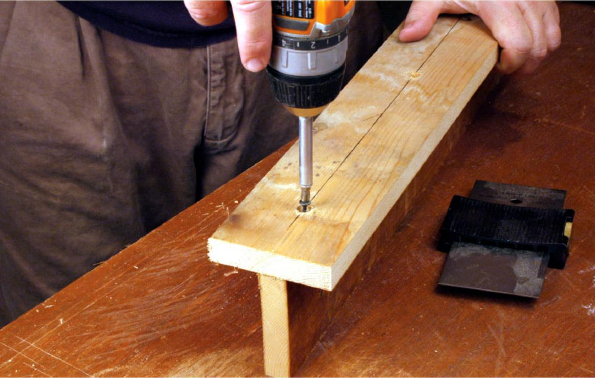
**Step Six** Then screw the leg pairs together, flushing the bevel ends to form the T. Pilot drill and countersink to avoid splitting.
