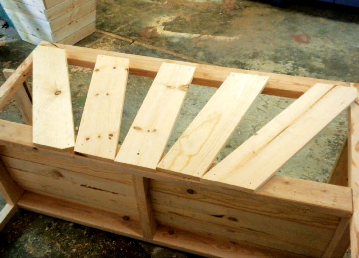
**Step 22** Beginning at the top of the seat, I began screwing slats to the sides, using an extra slat as a spacer.
