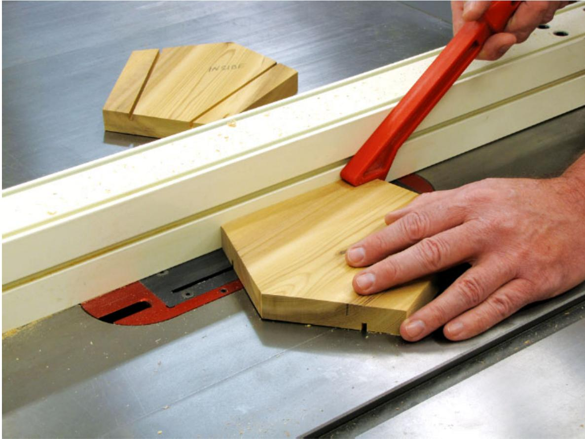
**Figure 3** Use the table saw to cut the slots for the acrylic panels.
