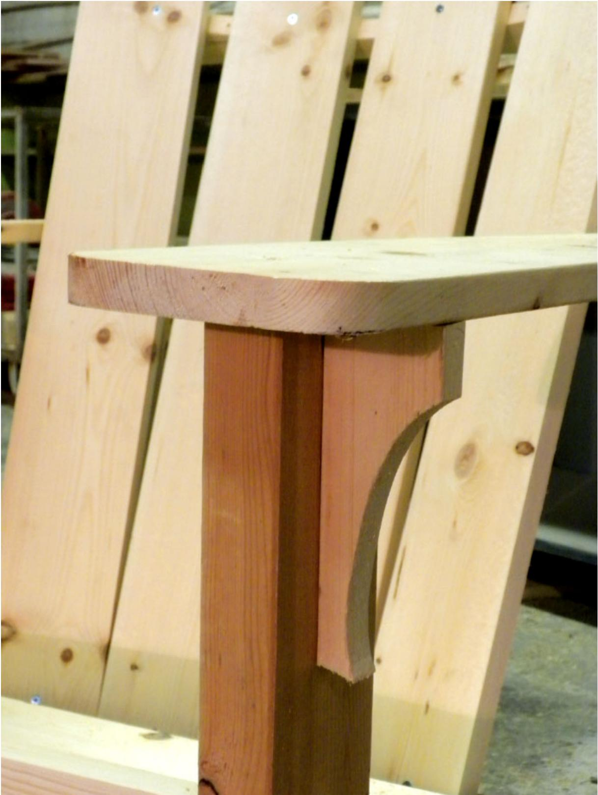
**Step 20** *As both a practical and stylistic touch, I made a pair of small brackets (also known as corbels) to help support the broad arms of the Adirondack, which I was sure would loosen up a bit over time.*
