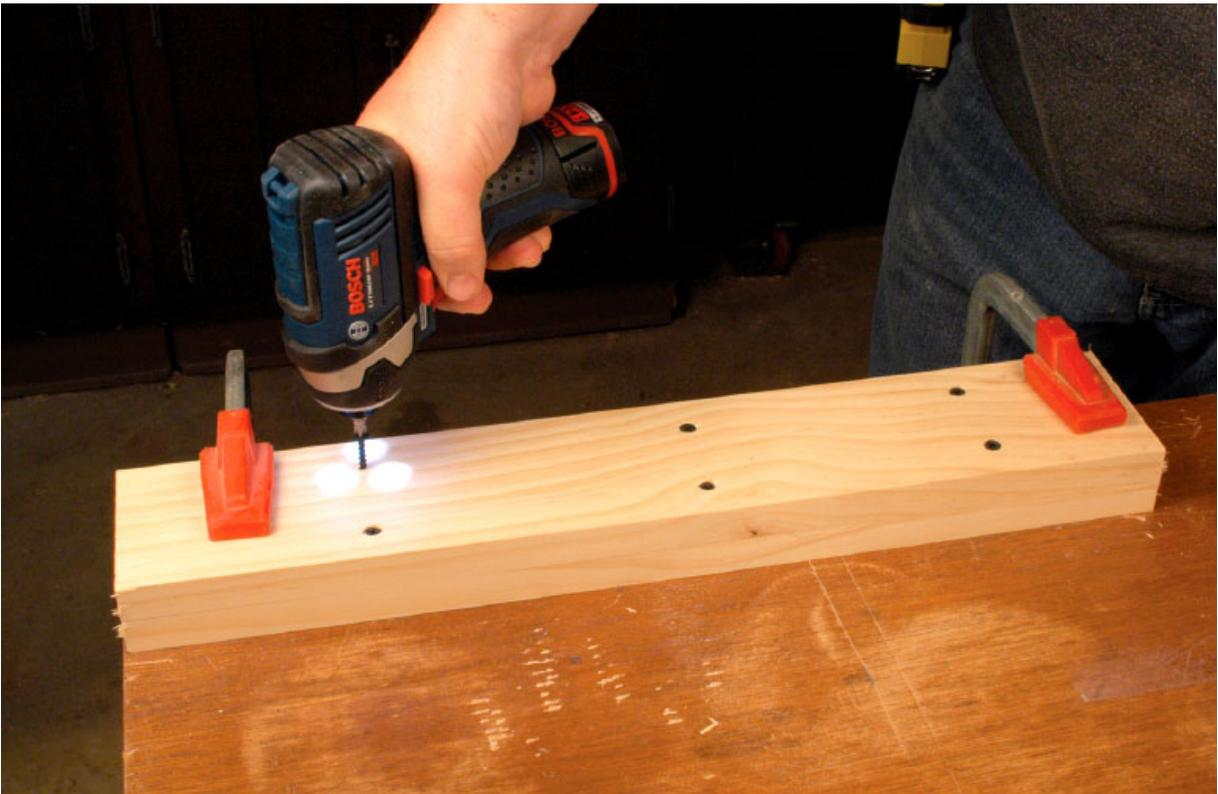
**Step Five** The center beam or stretcher is made of two pieces of 3 1/2"-wide material glued and screwed together from the underside. Since this piece is painted and this is
