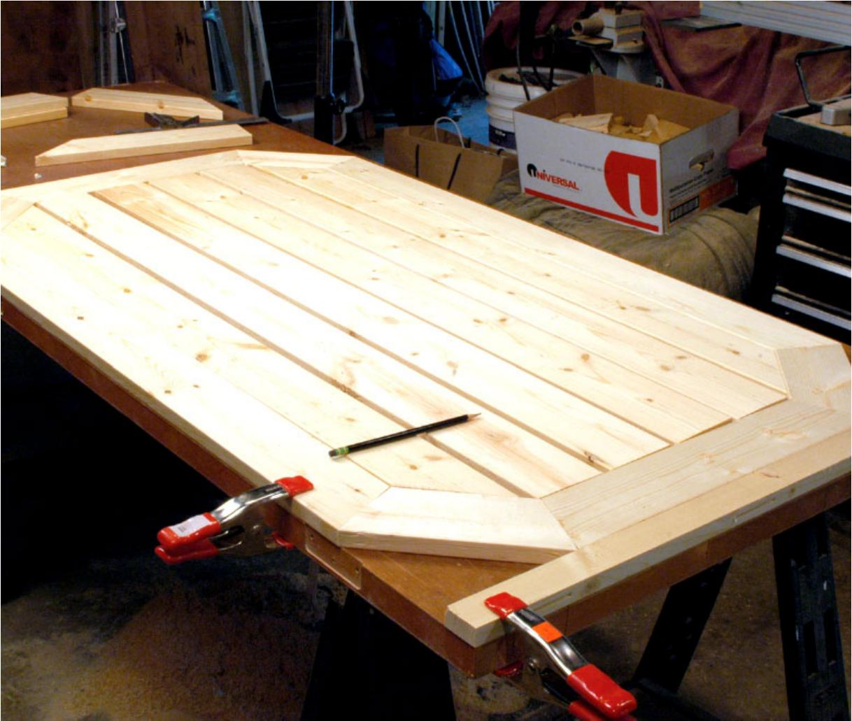
**Step 20** *I made a squareness guide on my work surface to help me lay out and cut all the miters for the top pieces. Start with the squared corner, then work around the outside of the frame, finally filling in the center slats.*
