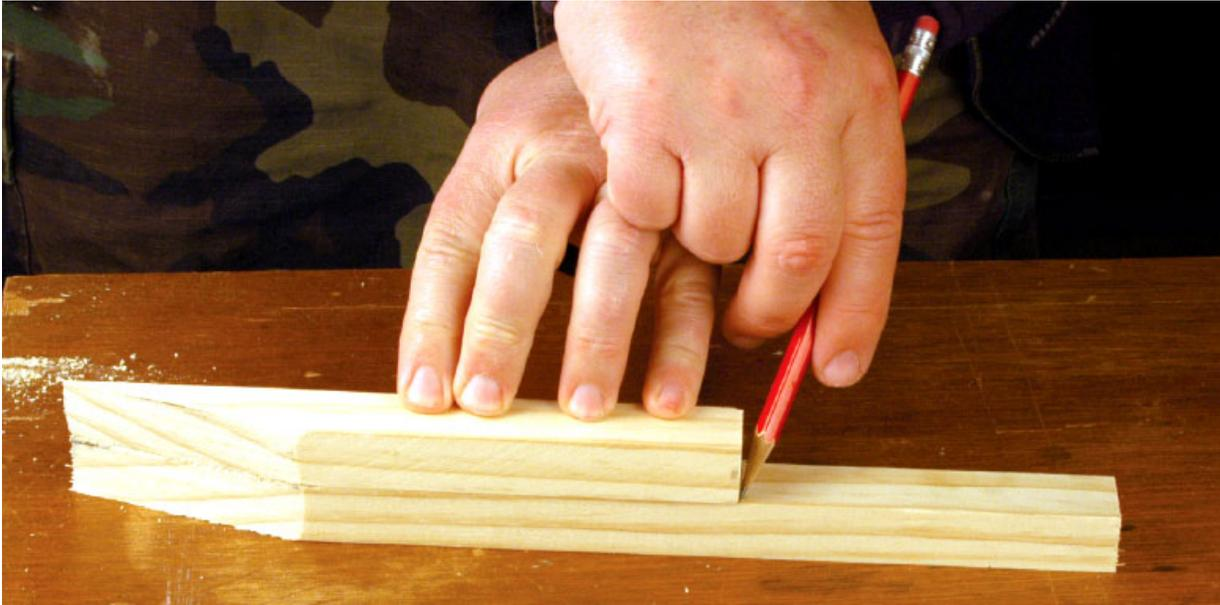
**Step 16** *I then marked both pieces for length, and made the cuts.*
