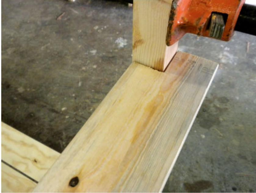
**Step 13** *The arms could be shaped any way you like (taking a page from Adirondack chair design, perhaps), but I kept it simple here. They do need to be notched at the back edge so that they can fit around the rear leg.*
