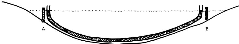
*Figure 80. The vertical height at points A and B is the same. These points are said to be on the same contour.*
