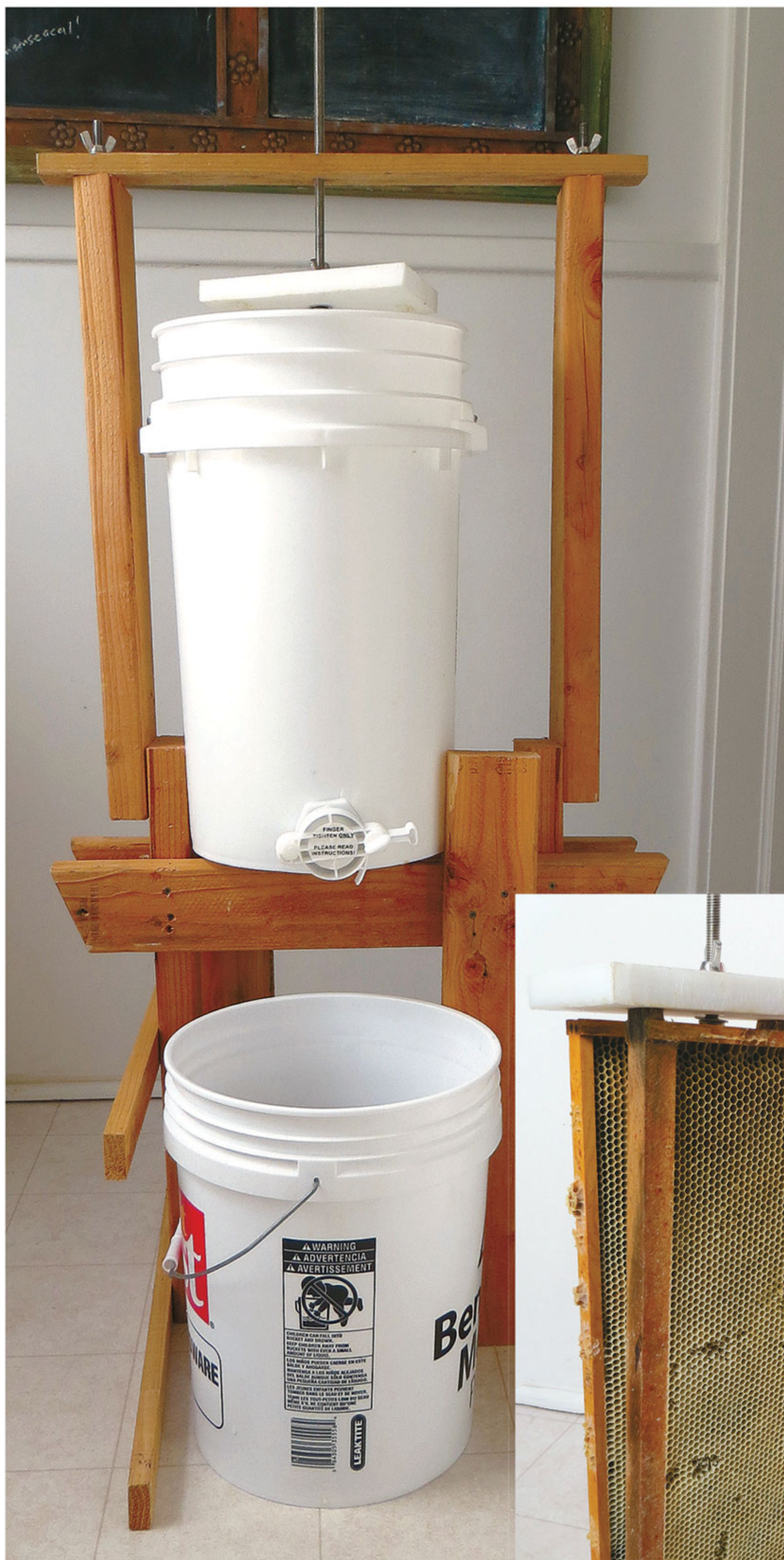
Using plastic pails and an electric drill to power a spinner, James Noble extracts honey.
