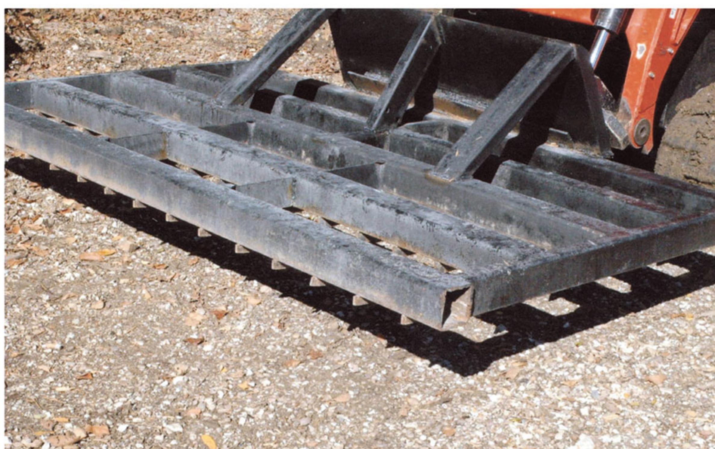
From chisel plow frame to pothole patcher for the skid-steer.
