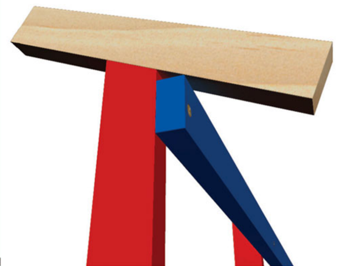
Figure 9: Fine tuning the position of the front wall's top plate.
