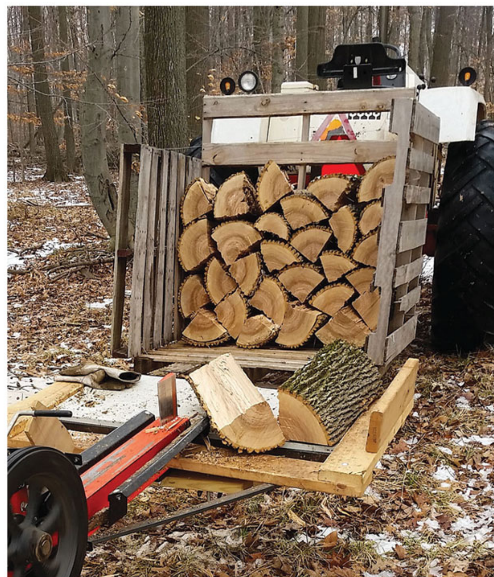
Using wood pallets and fence wire creates an easy-to-make system to contain firewood.
