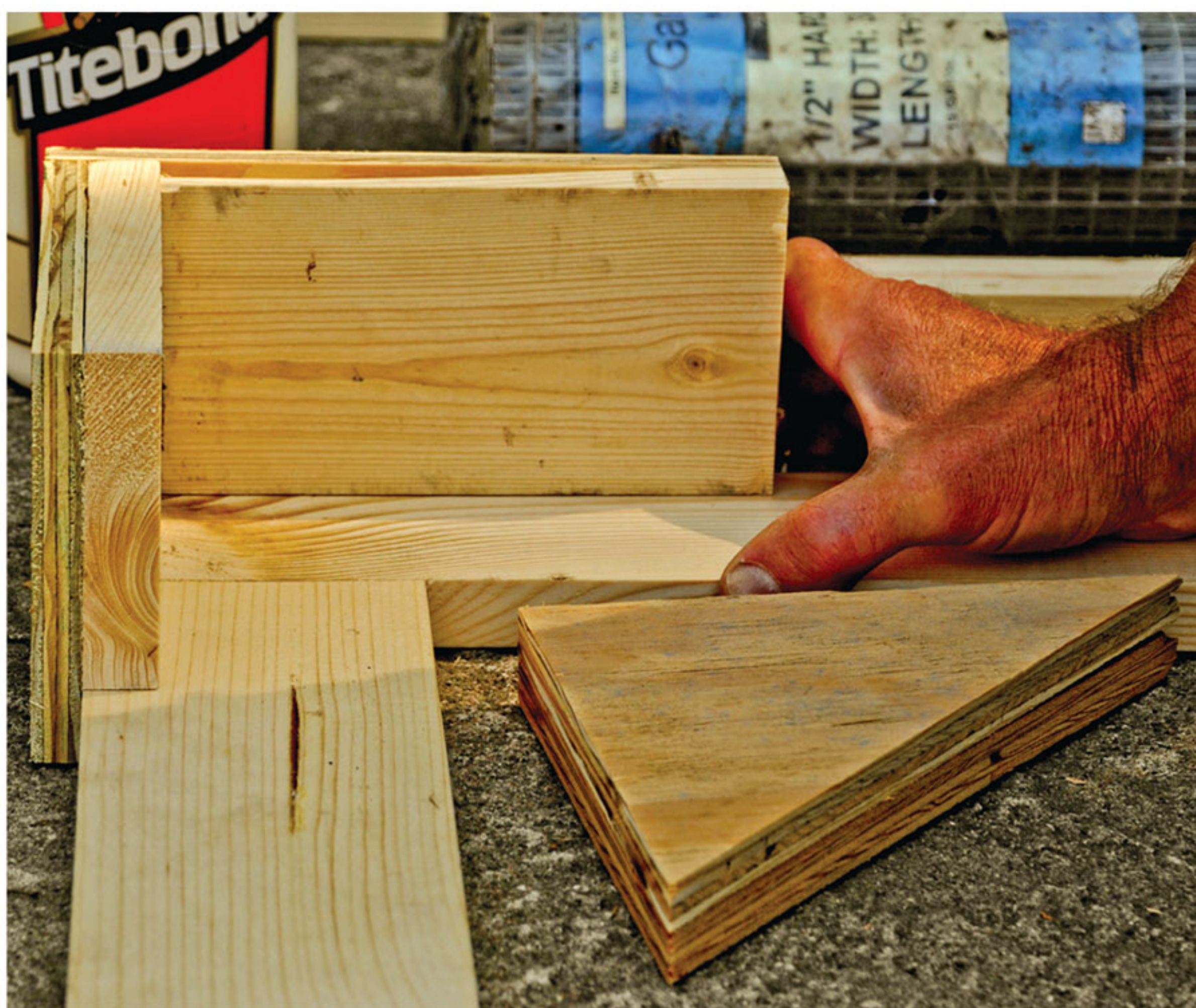
Constructing a corner jig ensures that all frame pieces will end up square, and it can also help with construction of the J gussets.
