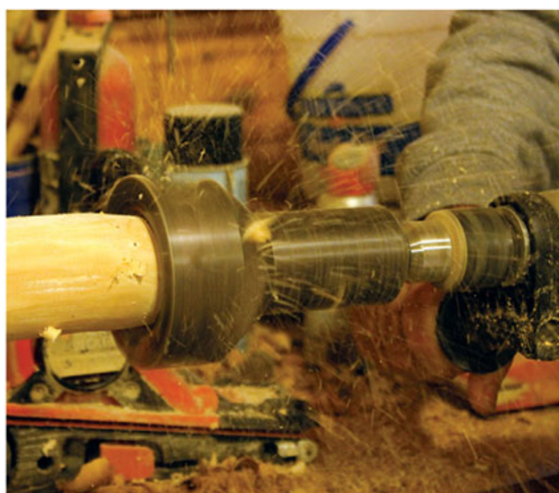
Tenon cutters help get it done safely and accurately.
