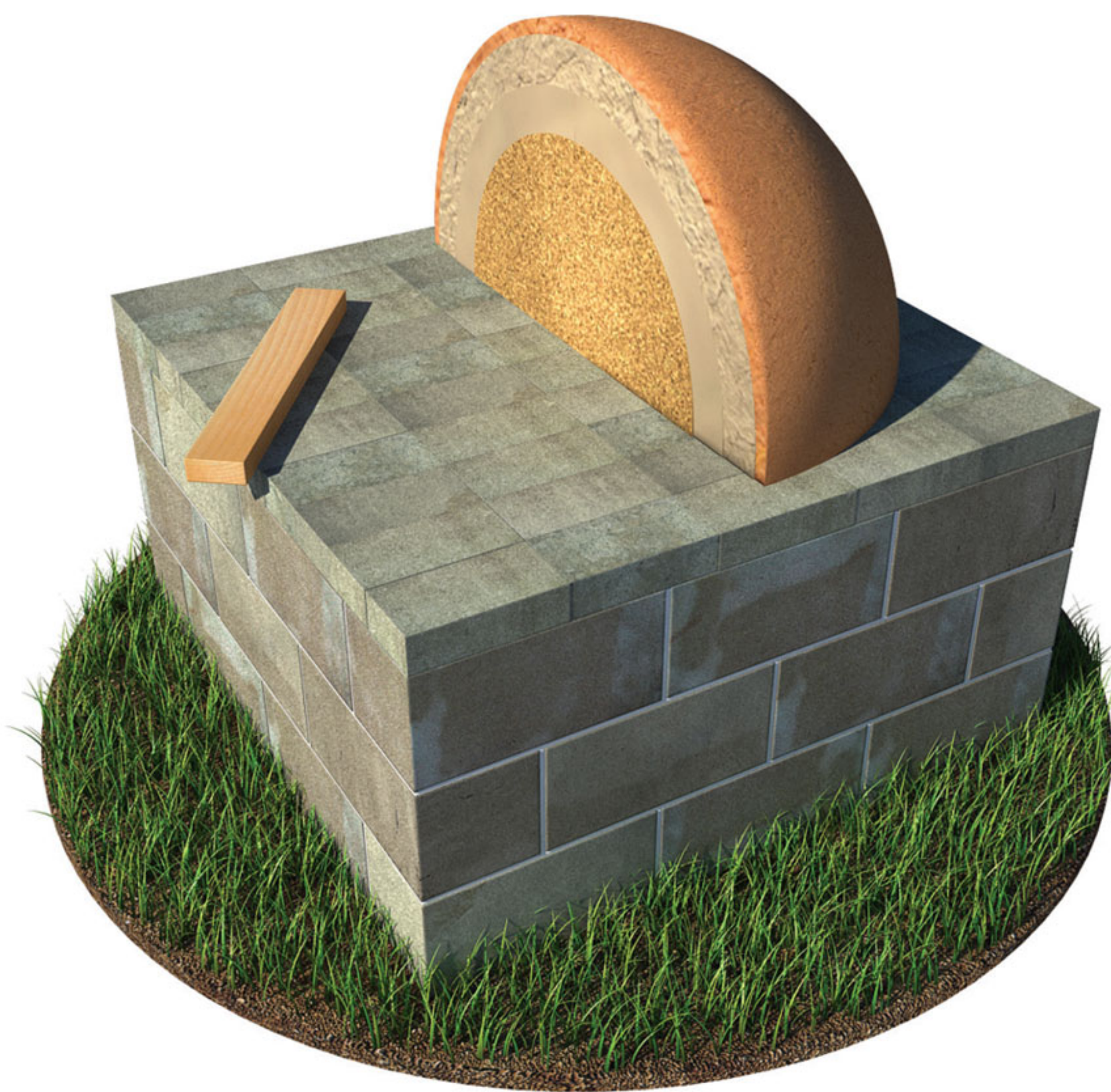
FIGURE 3. A cross-section of the oven shows the sand and three adobe layers.
