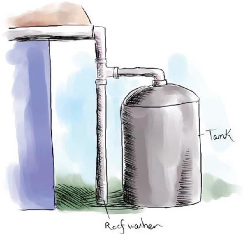
**One type of roof washer, using a tube.**
