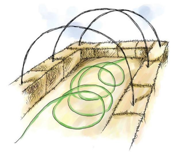
Water hose under the floor of a greenhouse built with bales of hay.
