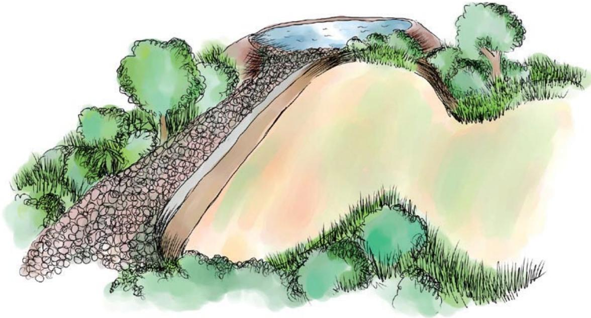
**Flood dam slows water flow and directs it to a reservoir.**
