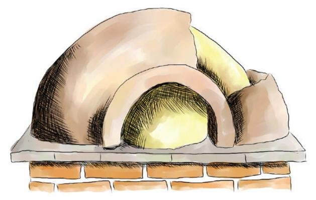
Mud oven under construction with sand inside.
