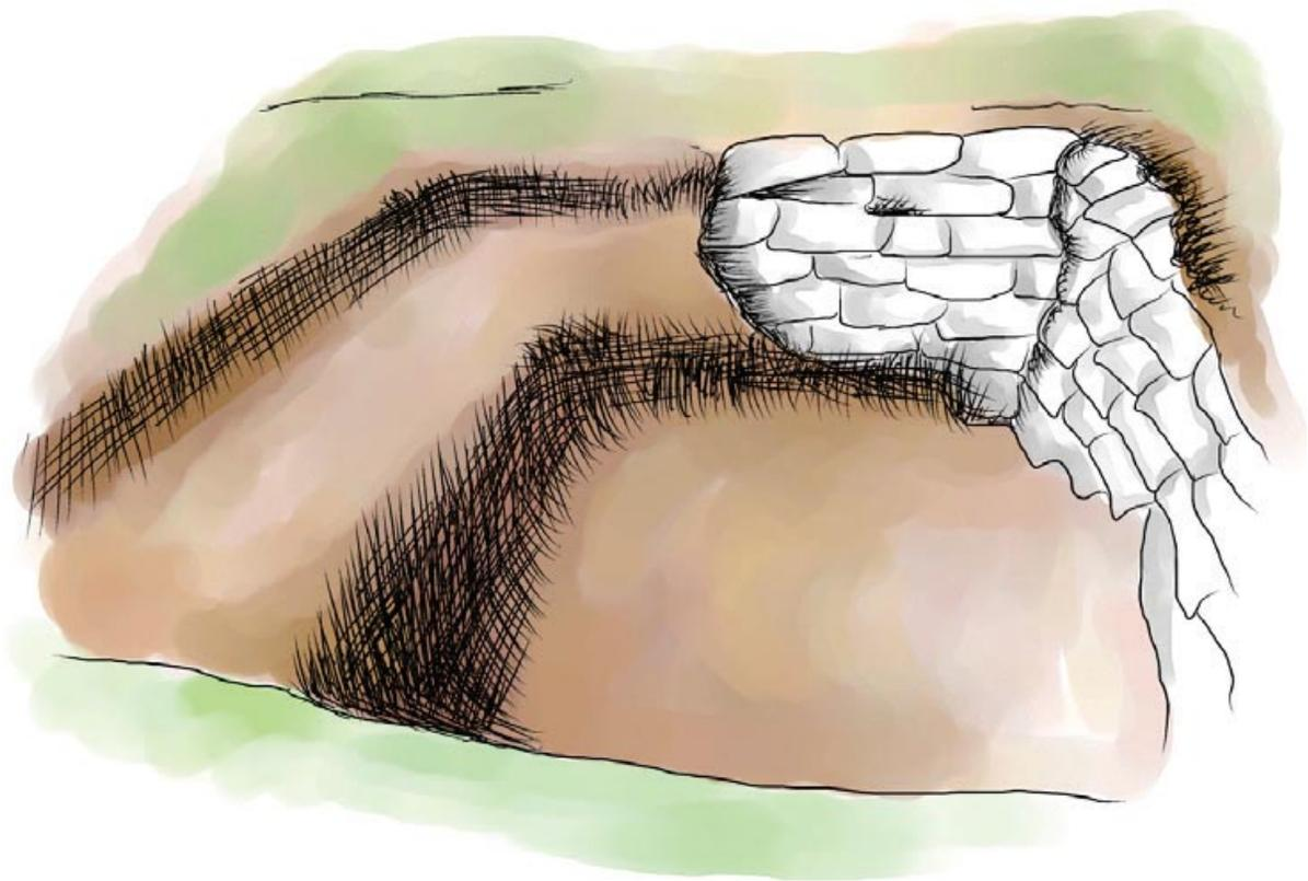
1. The tank is set at least a quarter of the way into the ground, so you have to dig a smooth hole the size and shape of your tank, leaving room for the earthbags.
