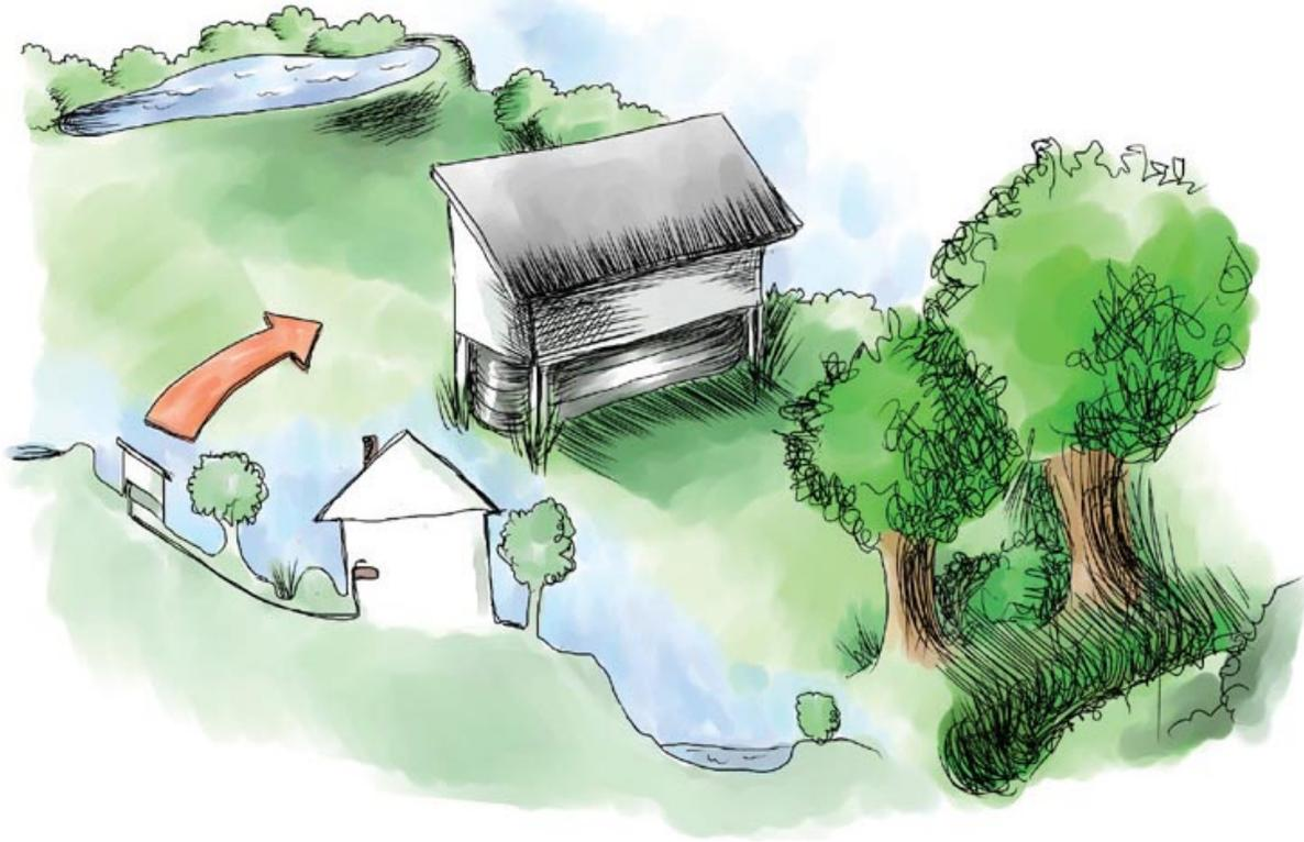
Gravity fed water from dams and rainwater collection at the top of a slope.
