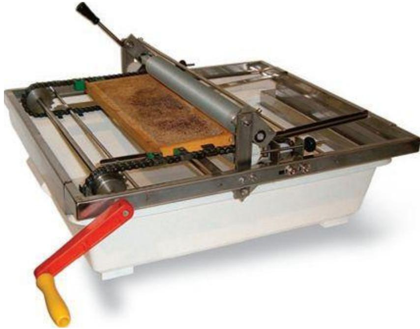
**A Cowen Silver Queen model extractor showing the frame guide in front, the blades below, and the chain they move on. This model is sitting on a table that is the support for a drainage tank.**
