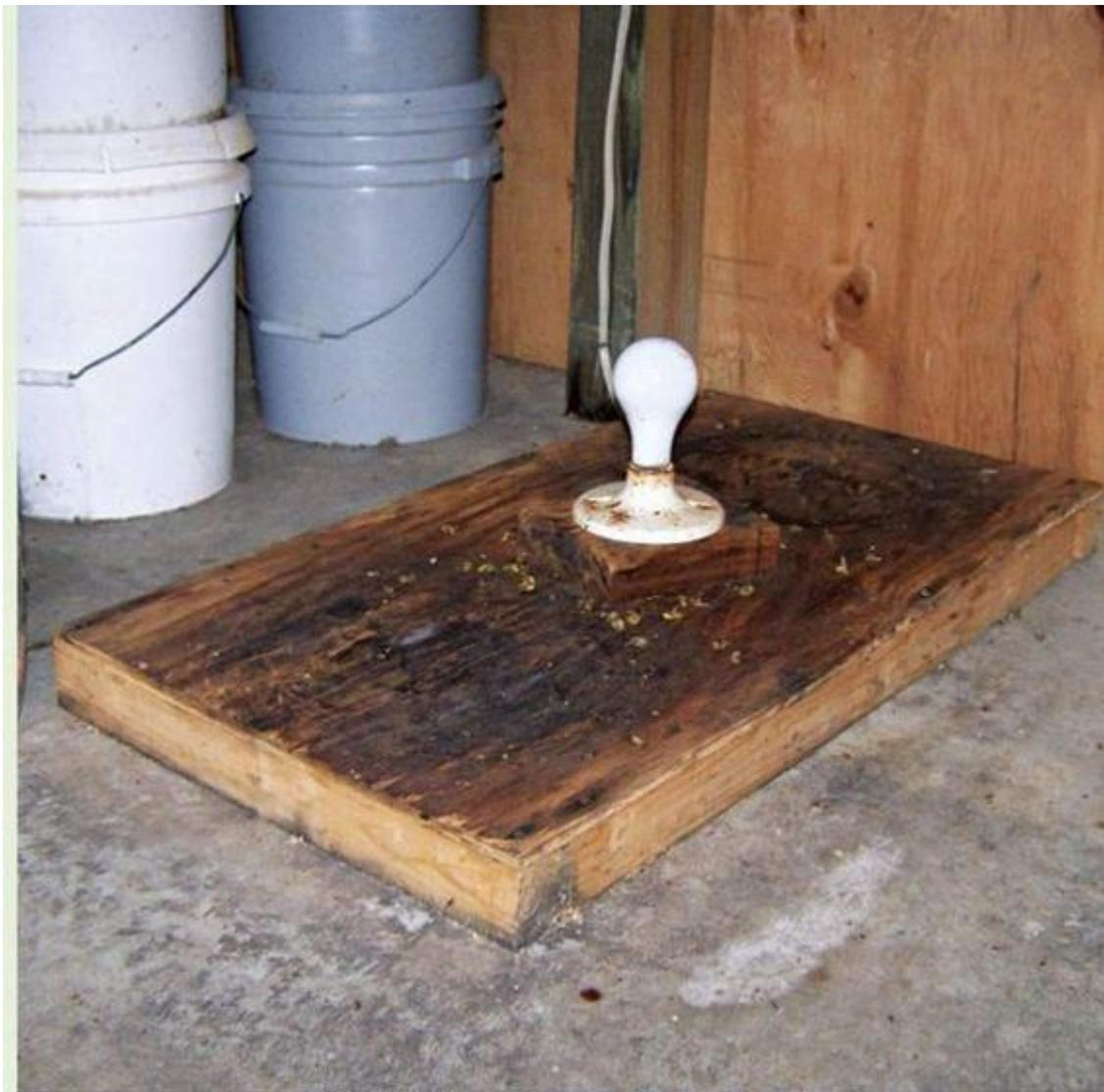
**The Styrofoam box is covered with industrial strength aluminum foil (for durability). When the honey pails are placed on the platform, above, the light is turned on and the box placed over the honey pails, resting on the platform. The Styrofoam box doesn't need to be extremely durable or of heavy duty construction (and definitely not heavy because you will be lifting it a lot). A well-insulated box is what is most important. 📸**
