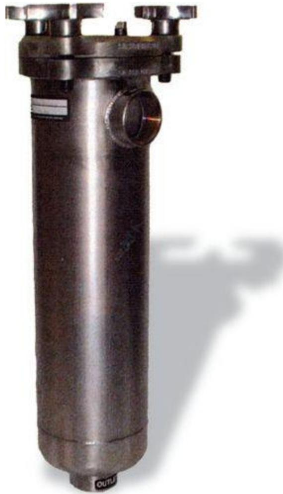
**Honey is warmed with a flash heater by pumping it through pipes in a tank filled with temperature-controlled hot water or vegetable oil. From there, the honey passes through a filter, then on to a wax spinner or storage tank.**
