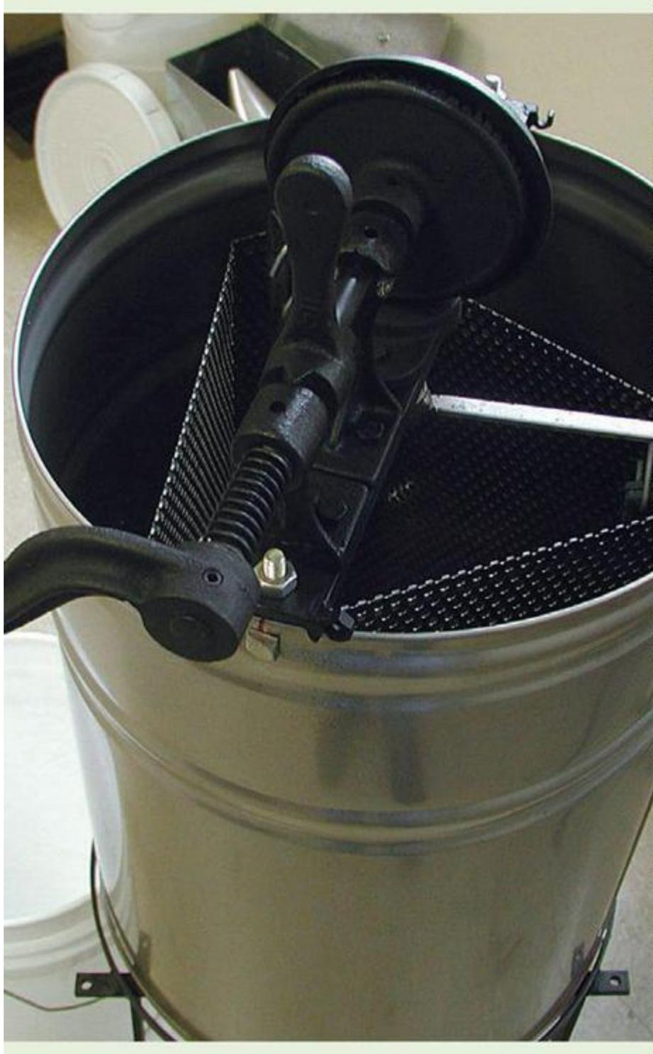
***Inside a Typical Radial Extractor Frames are set in a regular radial extractor much more efficiently than in tangential***
