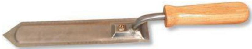
**Heated offset uncapping knife with an inline thermostat, the top-of-the-line model**
