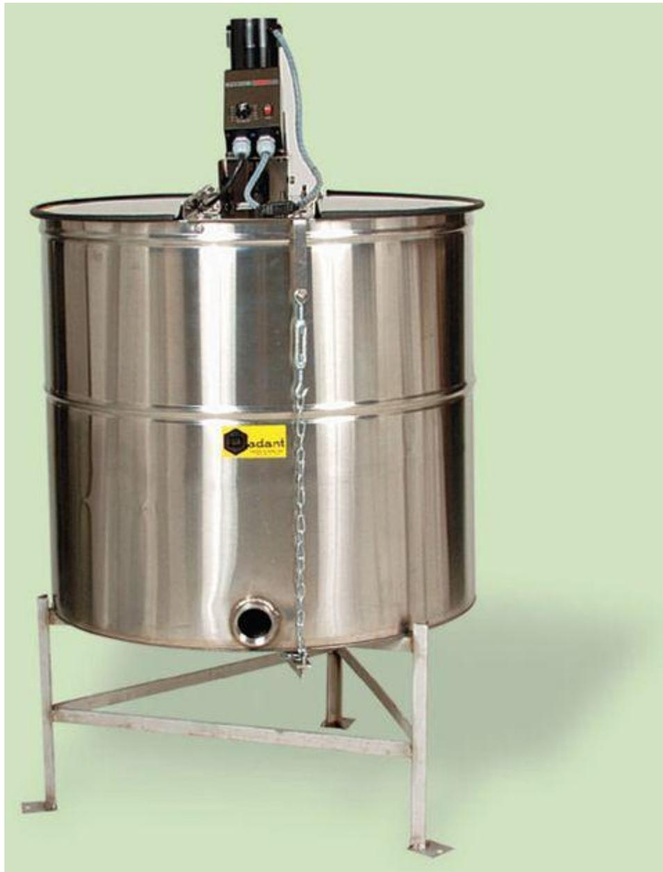
**Moderate-sized radial extractors, such as these nine-frame models, are small enough to work by hand, but certainly go faster if motor powered. 🚗**
