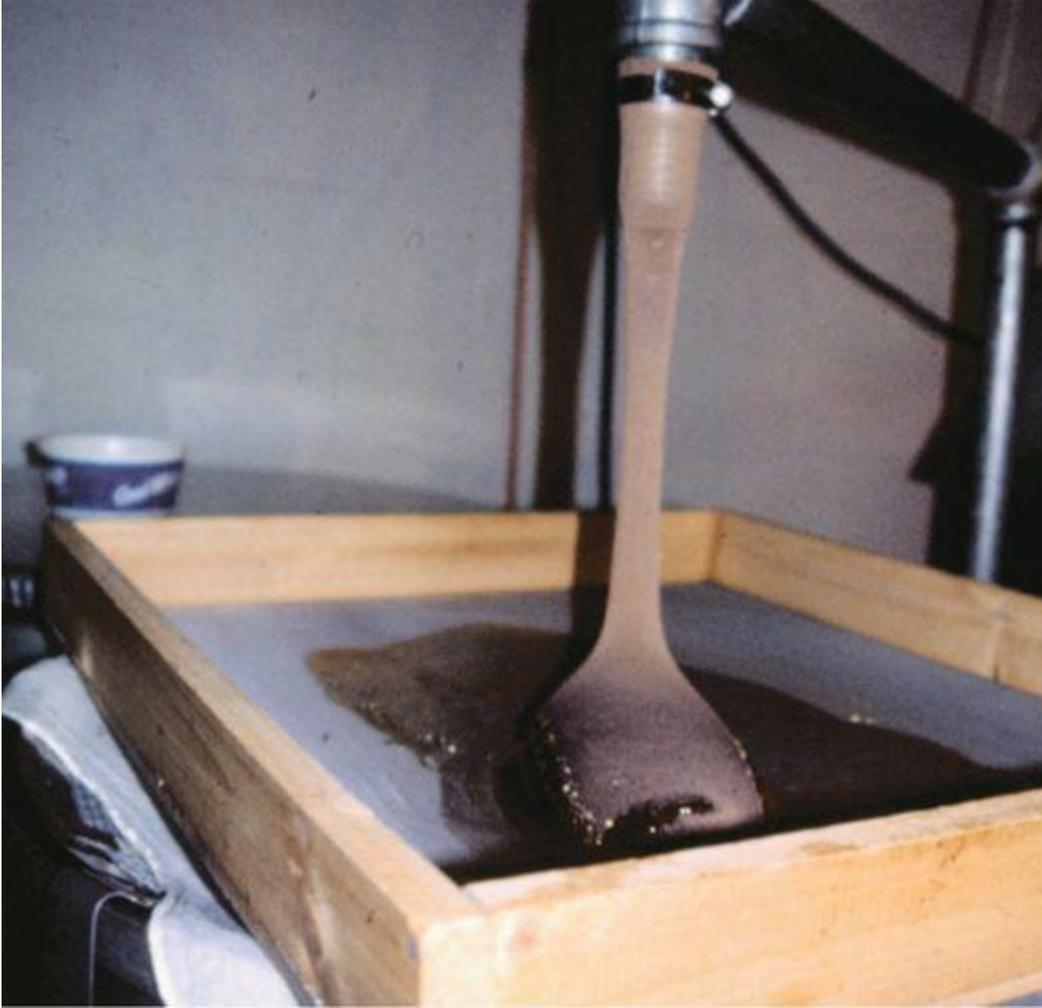
**Pressure filters remove most particulate matter, but the honey must be warmed to work well. These units can usually handle about 5 gallons (19 L) per minute.**
