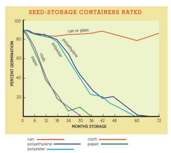
The type of storage container you use has a significant effect on how long seeds will last in storage.
