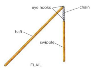
A simple homemade flail helps with the task of extracting seeds.
