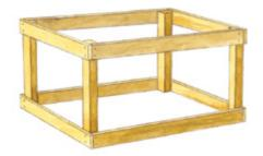
You can construct a simple frame for an isolation cage out of 1×2s.
