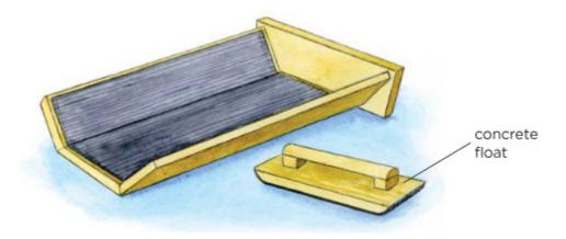
A threshing box is a wooden box that has slanted sides and is open at the top and at one end. Cover the sides and the bottom of the box with pieces of corrugated rubber matting. Do likewise with the surface of an inexpensive wooden concrete float.
