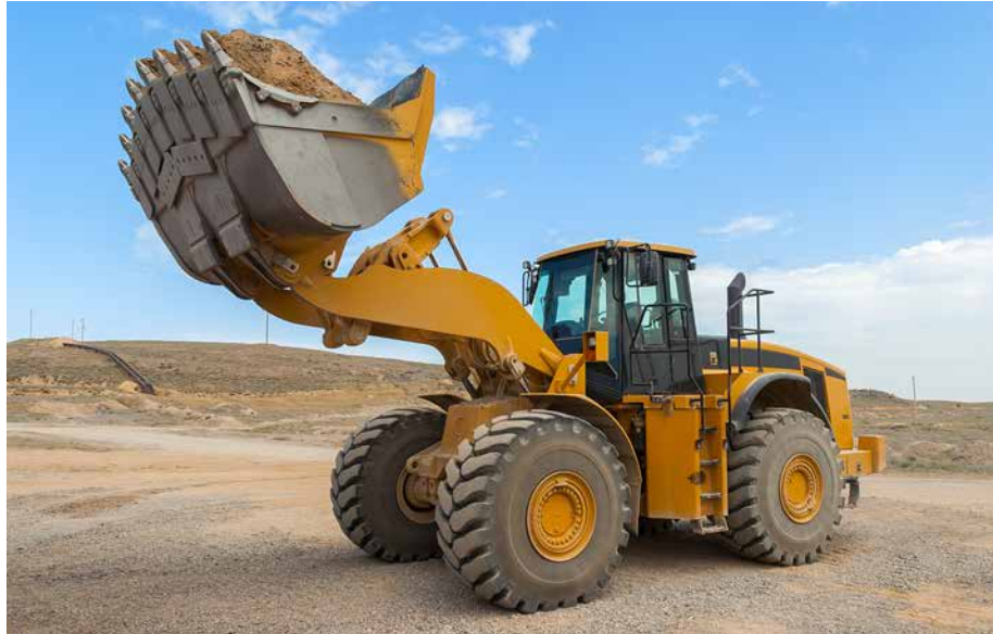
FIGURE 5.3. Wheel-driven front end loader.
