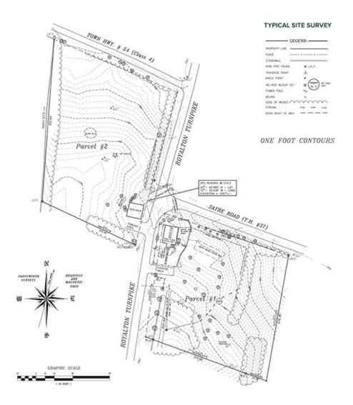
At the site scale we start with a base layer of information that is usually heavily informed by a site survey by a professional civil engineer or surveyor. The survey provides an invaluable level of detailed site information that includes contours, utilities, access, infrastructure, forest cover, and the exact locations of each.
