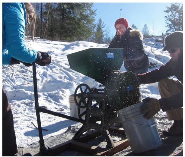
I was lucky to find a mechanical rice dehuller in an old barn in Vermont, which was made in Japan and works very well.
