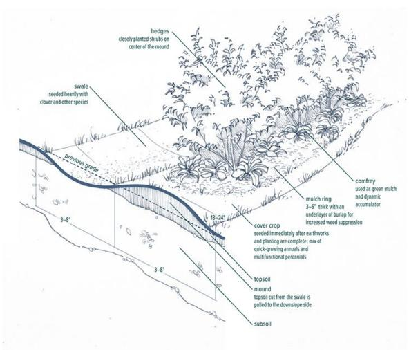
Swales at our research farm are constructed by digging into a swath of earth along the contour and placing the material along an even mound below. That mound is then planted at its height with berry and tree crops.
