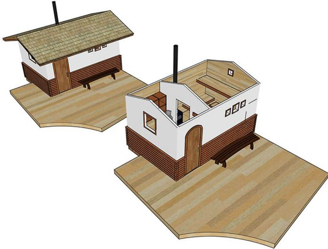
A three-dimensional model facilitates better communication and understanding between designer, client, and builder. The detailed model increases both the efficiency of the construction process and the quality of the end product. Illustration courtesy of Whole Systems Design, LLC
