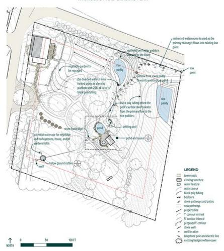
A detailed drawing of a proposed grading and hydrological system that takes the working master plan a step further. These plans are used to estimate materials and cost, think through the system in greater detail to identify challenges, and as a reference throughout the building process. Illustration courtesy of Whole Systems Design, LLC
