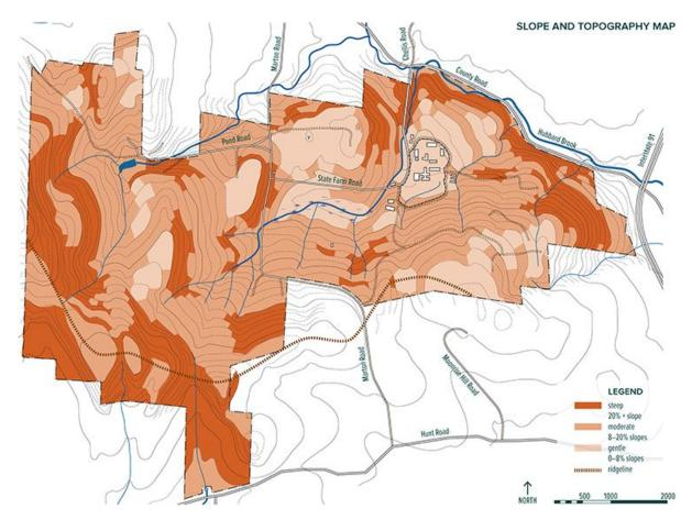
In landform analysis we're looking at the shape of the land. Using the contour lines available, slopes are classified into different levels of severity and assigned an accompanying color or hatch so it becomes clear, in broad strokes, what areas lend themselves to certain uses. Illustration courtesy of Whole Systems Design, LLC
