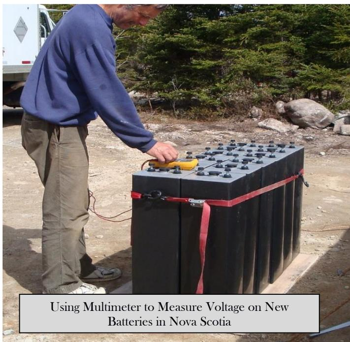
Using Multimeter to Measure Voltage on New Batteries in Nova Scotia
