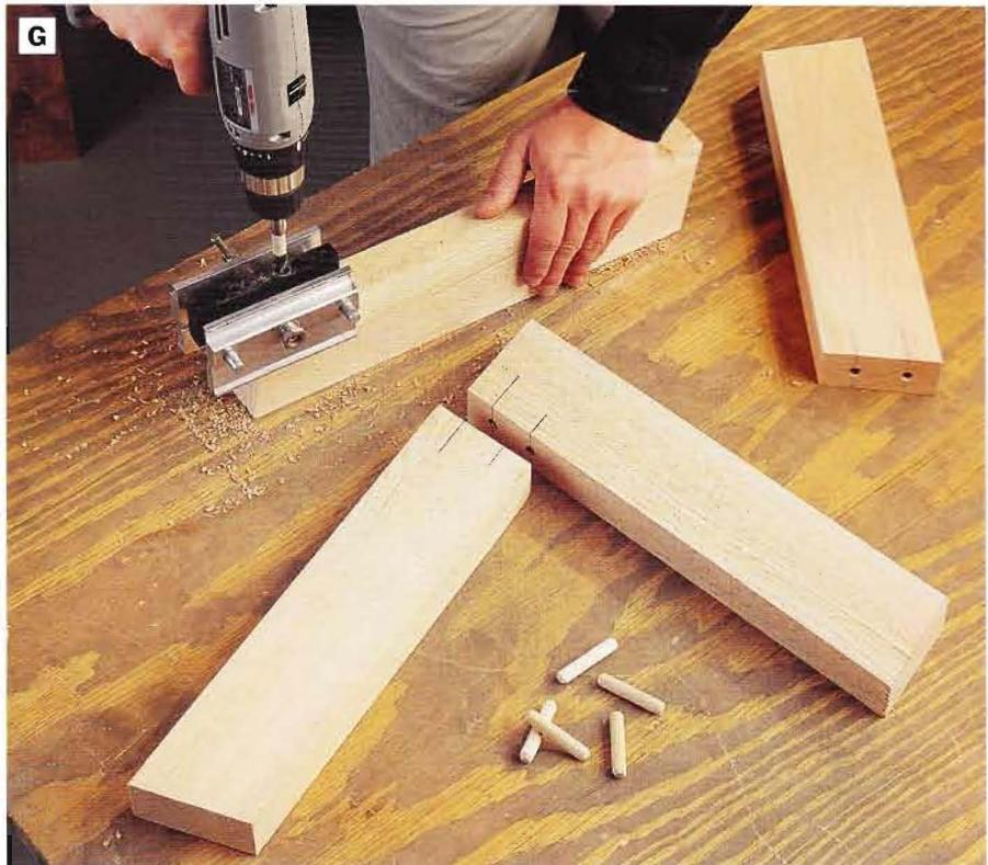
PHOTO G: Join the bench legs to the arm supports with pairs of 2-in. fluted dowels. Use a doweling jig when you drill the holes to be sure that the dowel holes are drilled straight across the joints. Wrap a piece of tape around the drill bit to serve as a temporary depth stop.
