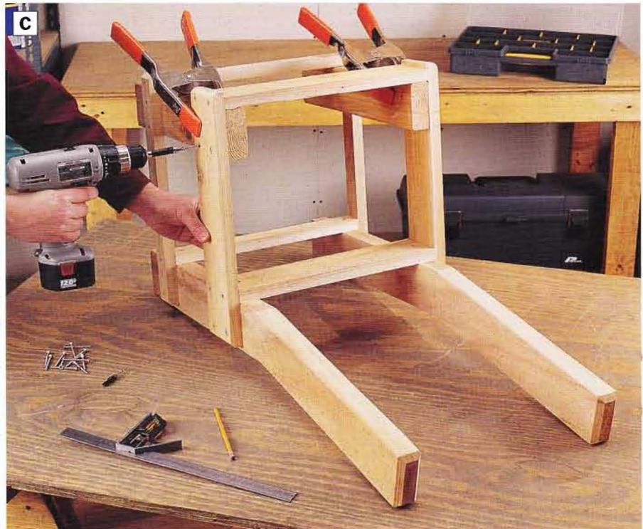
PHOTO C: Attach the upper and lower frames to the back and front legs with countersunk screws.
