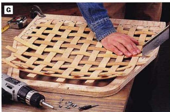
**PHOTO G:** After screwing down both ends of the first four cross strips on the back frame, continue weaving in the rest of the cross strips with their ends free. Then trim the weave to fit into the angled portions of the frame and screw the strips down one at a time.
