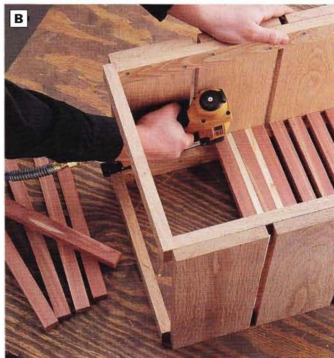
**PHOTO B:** Nail the cedar bottom slats to the top edges of the long and short cleats to form the bench bottom. Separate the slats with  $\frac{1}{2}$ -in.-thick spacers as you fasten the slats in place.
