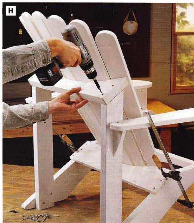
PHOTO H: Set the back assembly in place between the two arm assemblies and clamp the parts together. Drive screws through the upper and lower cleats into the back supports and back legs.
