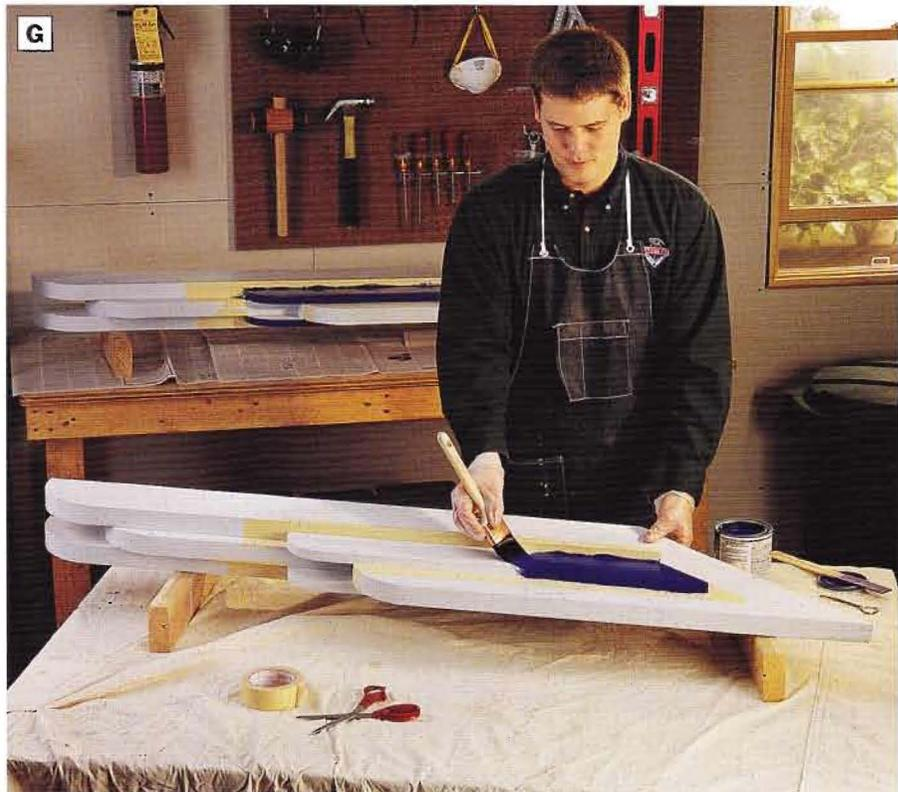
**PHOTO G:** Mask off those hammock parts that you want to paint in contrasting colors. Use wide tape and “burnish” the edges of the tape with your fingernail where paint colors meet to keep one color from bleeding into the other as you paint. Paint one color at a time and allow it to dry.
