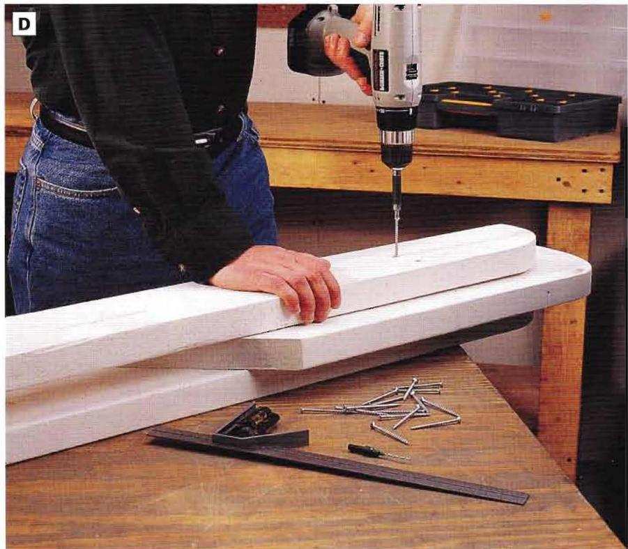
**PHOTO D:** Lay the other outer base piece on top of the base assembly and drive screws through it to attach it to the inner base pieces. Countersink pilot holes for the screws so you can conceal them with wood putty or auto body filler.
