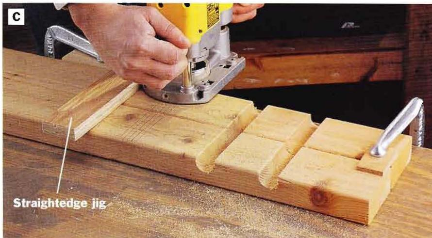
PHOTO C: Gang-rout notches in the back supports to ensure that the notches will line up perfectly on both pieces. Use a  $\frac{3}{4}$ -in. core box bit, and cut the notches in several passes of increasing depth. We clamped a short T-square style straightedge jig to guide the router when cutting.
