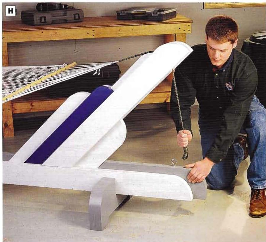
**PHOTO H:** Hang the hammock. Stretch the hammock ropes over the center support on each upright and pull the hammock until taut. Tie off the hammock securely to the lag screw hooks.
