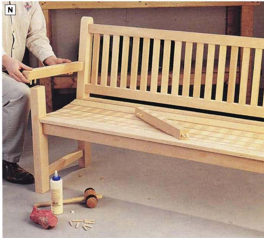
PHOTO N: Glue dowels into holes drilled previously in the arm rest. Coat the mating surfaces with glue, then attach the arm rests to the end assemblies and tap into place with a wooden mallet.
