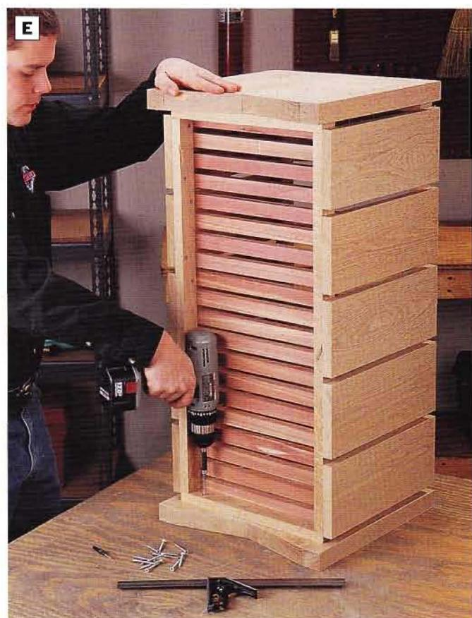
**PHOTO E:** Set the side panels into position on the short cleats, so the front edges of the sides overhang the bench front by  $\frac{1}{4}$  in. and the tops of the sides are flush with the top cleats. Screw through the short cleats to attach the sides to the bench.
