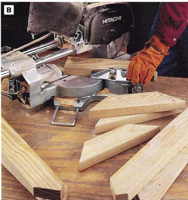
PHOTO B: Saw the long and short seat pieces to length, then miter-cut the ends to shape, according to the drawings shown on page 43. A power miter saw makes this task easy.
