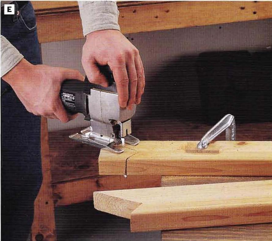
**PHOTO E:** Cut birdsmouth notches on the upper ends of the angled braces with a jig saw so the braces will interlock with the center table stretcher. Clamp each brace to your worksurface to hold it steady while you make the cuts.
