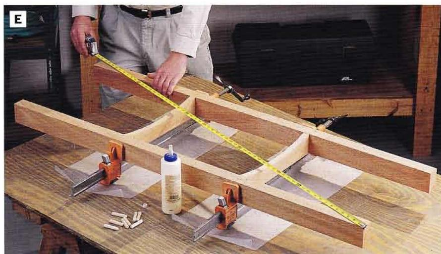
PHOTO E: With the dowel joints of the braces and stretchers glued up, clamp the seat assembly and check for square by measuring the diagonals. Adjust as needed by repositioning the clamps.
