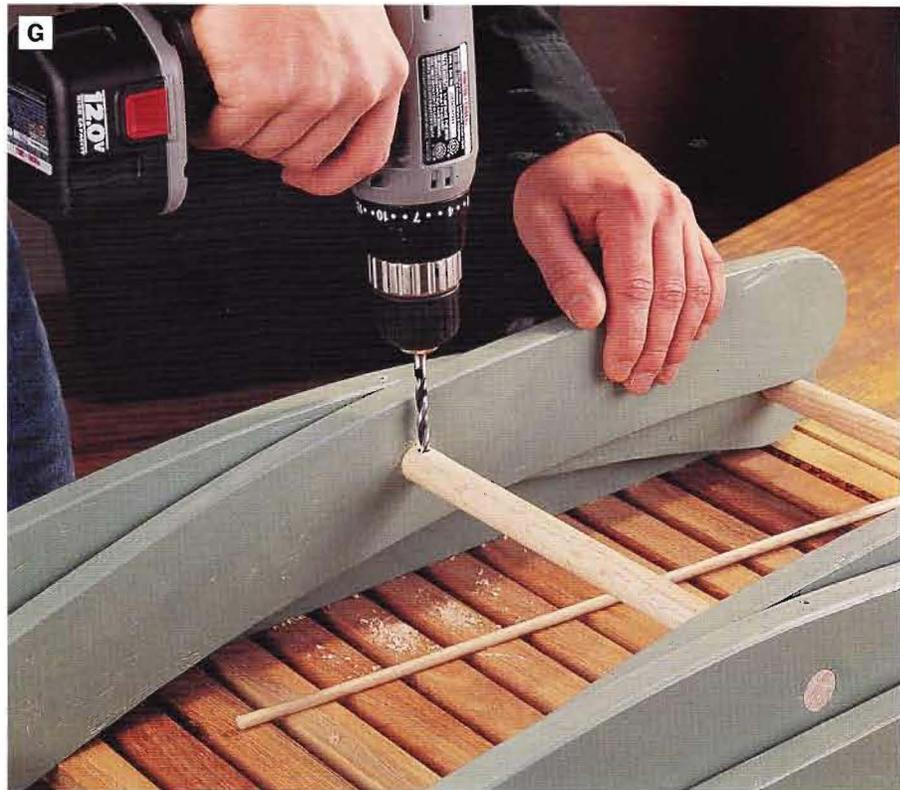
**PHOTO G:** Lock the inner legs in place by drilling and inserting  $\frac{1}{4}$ -in.-dia. dowels through the leg pivot dowel. Position the lock dowels to leave a slight bit of room between the legs, so they can move easily past one another without damaging the painted finish of the parts.
