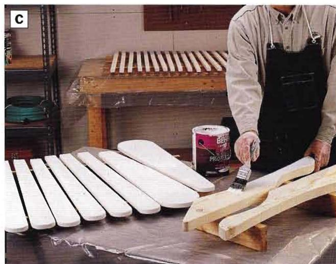
**PHOTO C:** Sand the chair parts smooth, and prime all surfaces with exterior latex primer. Primer will seal the wood and provide an even bonding surface for topcoating with paint.
