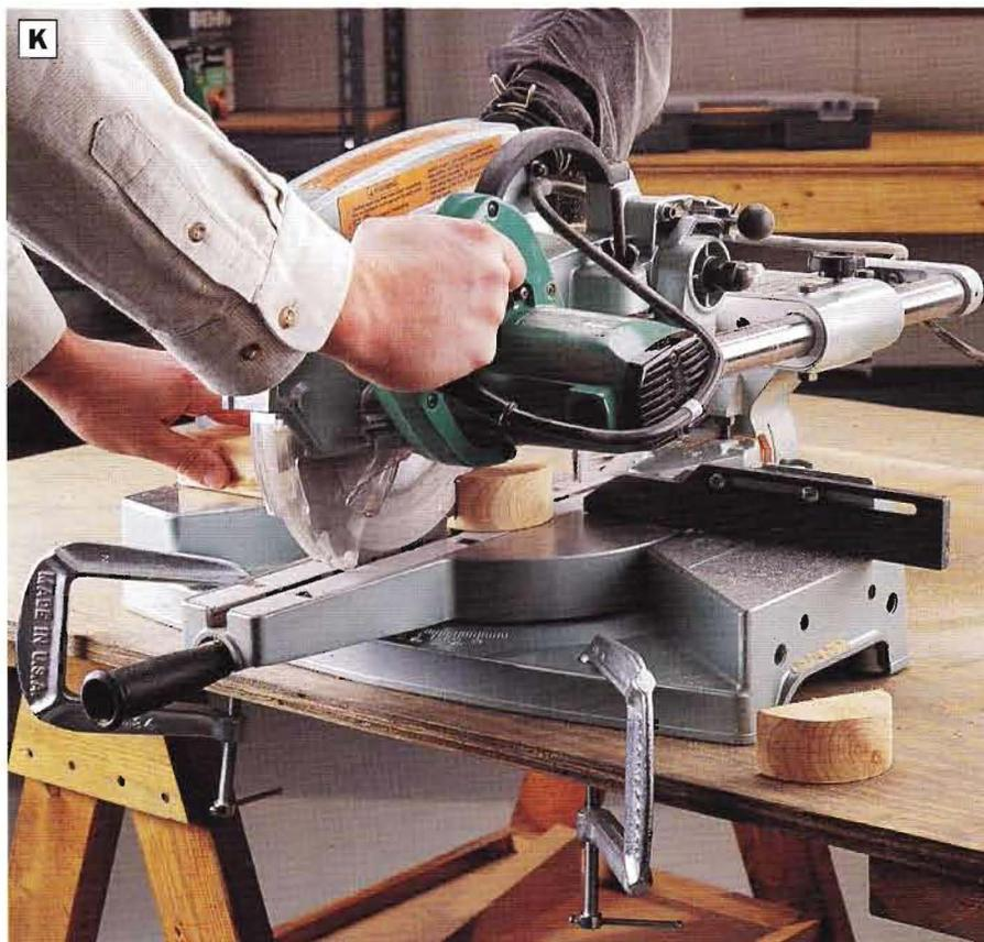
**PHOTO K:** Cut  $1\frac{3}{4}$ -in. radiuses on either end of a section of  $2 \times 4$  cedar. Cut off these curved ends with a power miter saw or radial-arm saw. The pieces will serve as leg stops on the foot rest. Cutting short workpieces from longer stock keeps your hands a safe distance from the blade.
