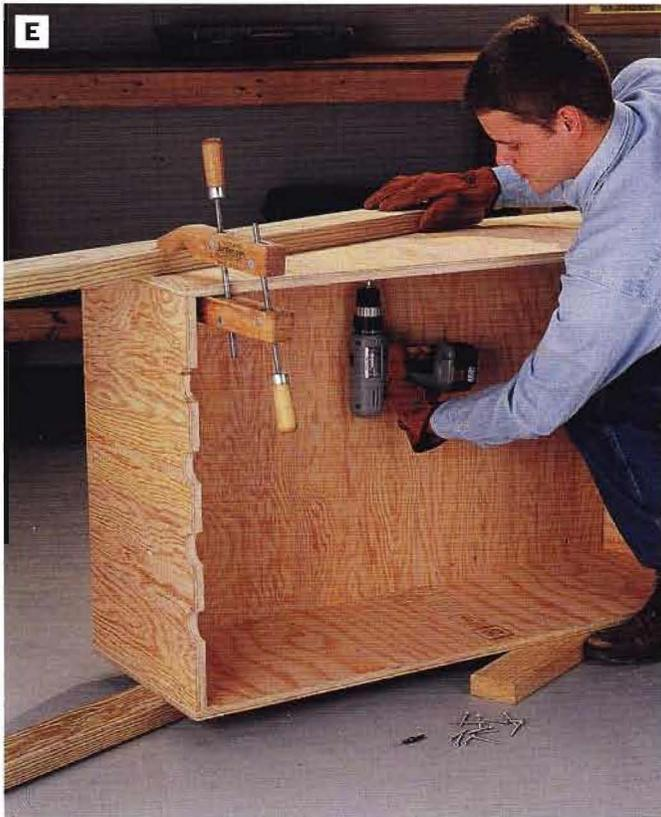
**PHOTO E:** Mark the locations of the handles on the cart box, and install the handles with moisture-resistant wood glue and 2-in. galvanized deck screws. Clamp the handles in place as you attach them.
