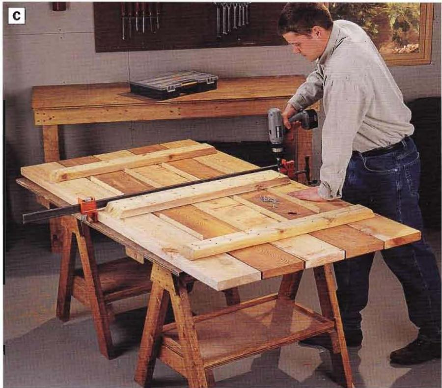
**PHOTO C:** Mark locations for the three table stretchers on the bottom of the tabletop, then fasten the stretchers to the table slats with 2½-in. galvanized deck screws. Set ¼-in. spacers between the slats before you fasten the stretchers to keep the slats held evenly apart.
