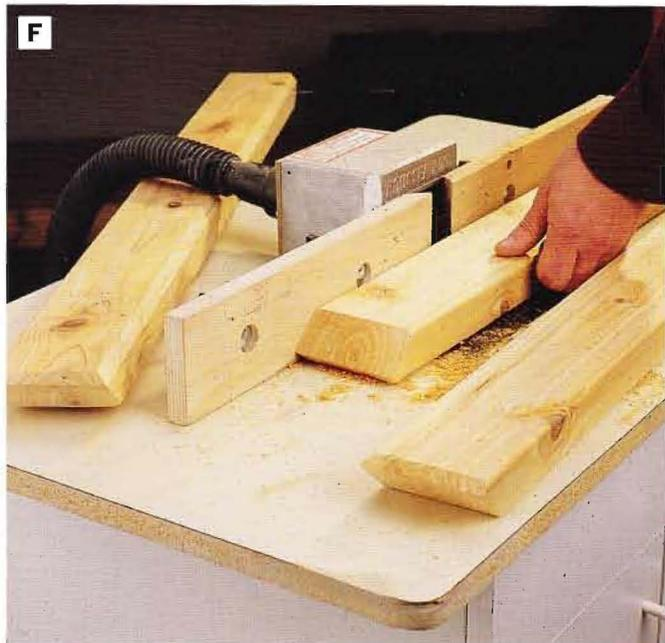
**PHOTO F:** The bottom edge and both ends of each apron piece are chamfered. Make these cuts at the router table, using a piloted chamfering bit set to a height of 3/8 in.
