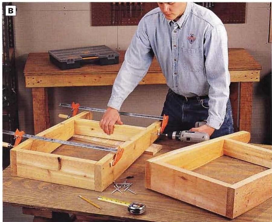
**PHOTO B:** Fasten the legs to the upper and lower crosspieces with deck screws. Position the upper faces of the lower crosspieces so they are  $10\frac{3}{4}$  in. from the bottoms of the legs.
