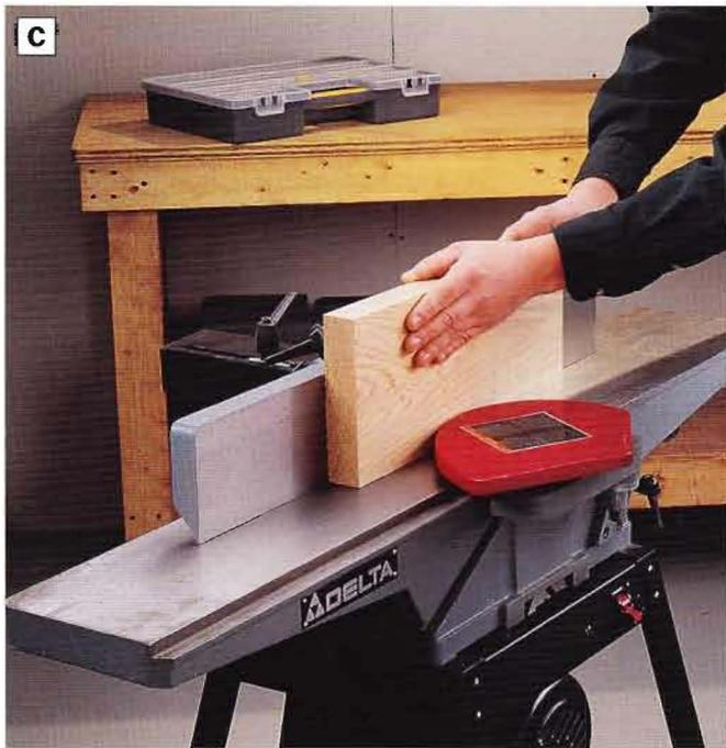
**PHOTO C:** Flatten the edges of the workpieces that will make up the side panels on the jointer or with a hand plane. Unless the boards are perfectly flat, gaps will show when you glue up the side panels.
