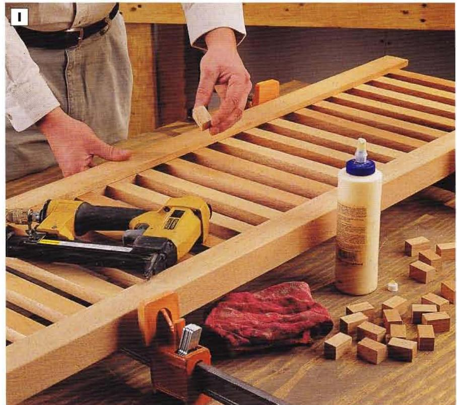
**PHOTO I:** Attach the top rail to the back assembly by applying glue along the three inside faces of the rail's groove and clamping. Install spacer blocks between the slats on this rail as well.
