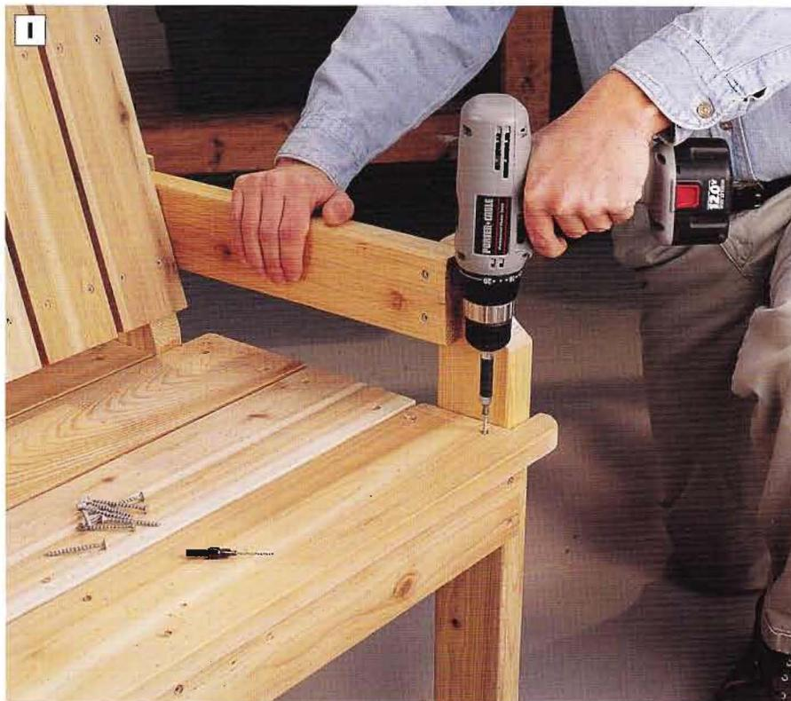
**PHOTO I:** Once the seat slats have been cut to length and, in the case of the rear slat, ripped to width, sand the slats smooth. Then drill countersunk holes and secure the slats to the seat frame with deck screws. The front slat will need to be notched and shaped before it is installed.
