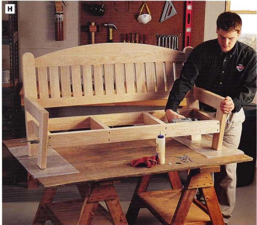
PHOTO H: Fasten the arm assemblies to the bench by driving screws through the back stiles and into the arm supports. Screw from inside the bench to attach the end bench struts to the legs as well. Clamp the arm assemblies in place first, to make installing the assemblies easier.
