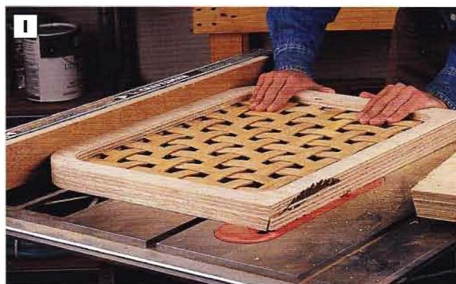
**PHOTO I:** With the table saw blade tilted to 15°, cut a beveled edge on the seat and back frames where they will meet each other at an angle.
