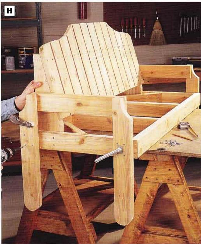
**PHOTO H:** Clamp the leg assemblies to the seat/back assembly. The bottom edge of the seat frame should be  $11\frac{3}{4}$  in. up from the bottoms of the legs and extend  $\frac{1}{2}$  in. beyond the front legs.
