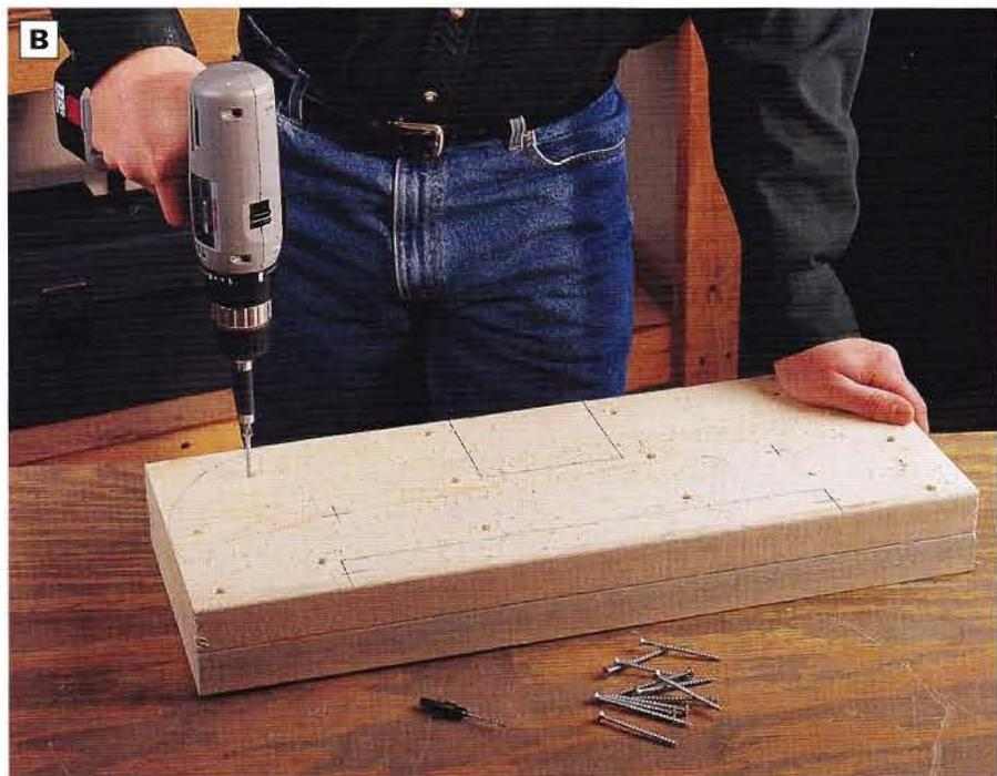
**PHOTO B:** Fasten pairs of leg blanks together with the layout side facing out. Use glue and countersunk screws to attach the parts. Cut the three legs to shape with a band saw or a jig saw, and smooth the cut edges.
