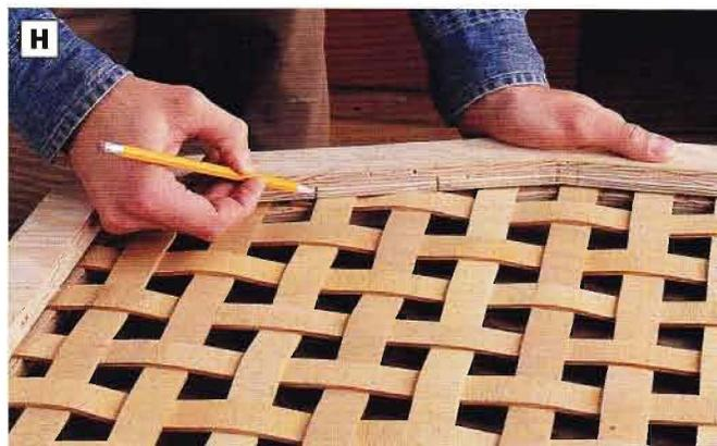
**PHOTO H:** Mark the unrabbeted back frame in those areas that will need to fit around doubled-up weave strips. Remove this frame piece and notch out the marked areas with a sharp chisel.
