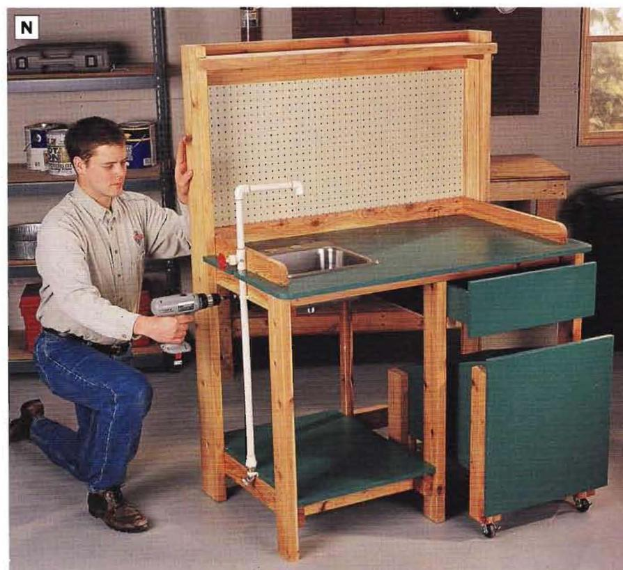
**PHOTO N:** Use strap clamps to attach the plumbing assembly to the bench.
