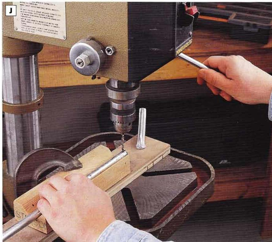
**PHOTO J:** Cut a V-shaped notch in a scrap of 2 × 4 to help steady the axle as you drill holes for cotter pins. Fasten the notched cradle to another scrap, and clamp the jig to the drill press table. Drill through the rod using a slow speed setting and firm—but not excessive—force on the bit.
