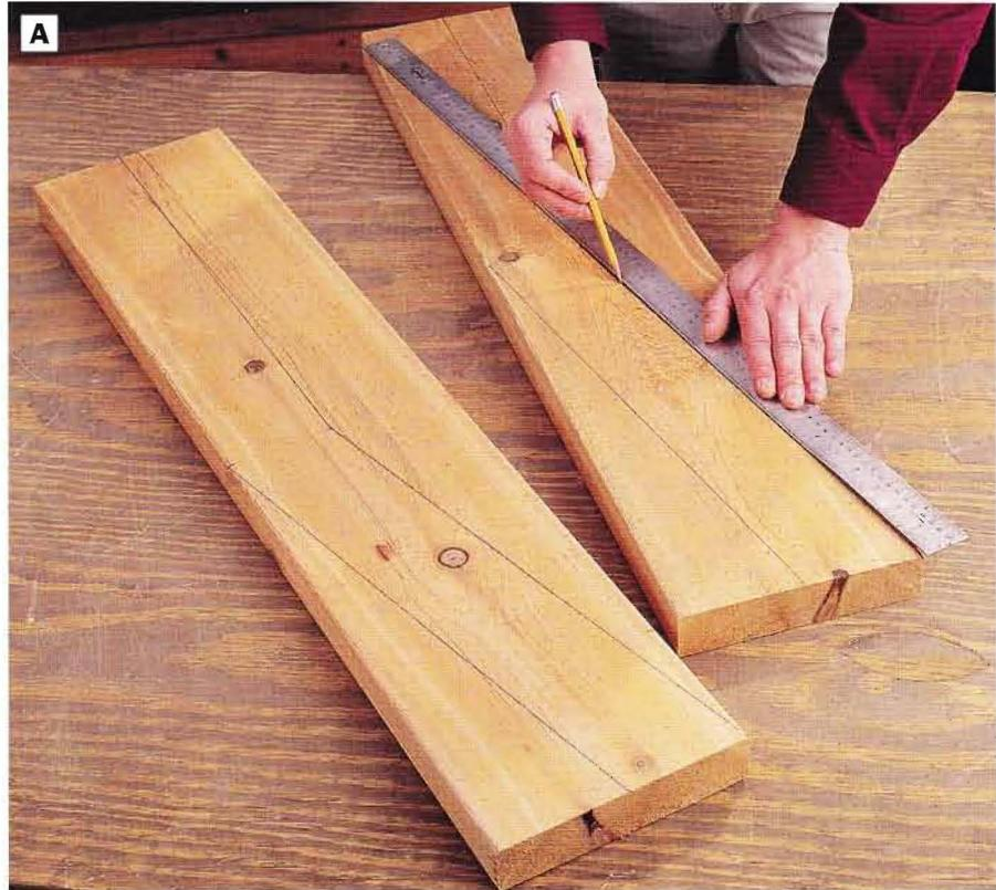
**PHOTO A:** Lay out and cut eight back chair legs to shape. Use the *Back Legs* drawing, page 25, to establish reference points for drawing the leg shapes. Connect the points with a straightedge.
