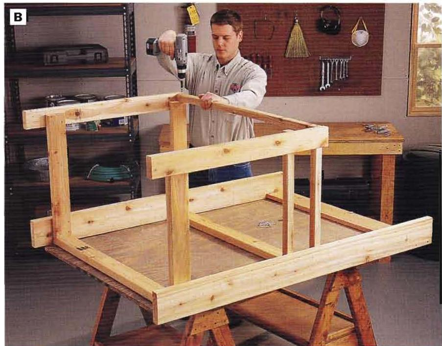
**PHOTO B:** Assemble the bench framework by attaching the two back stretchers, shelf stretcher and top front stretcher to the end assemblies. The ends of the stretchers should butt against the inside faces of the front and back legs. See Step 4 for exact stretcher placement.
