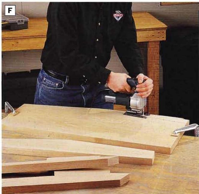
**PHOTO F:** Cut the back supports, back rest and seat to shape, using the detail drawings on page 49 as a guide for establishing the profiles.
