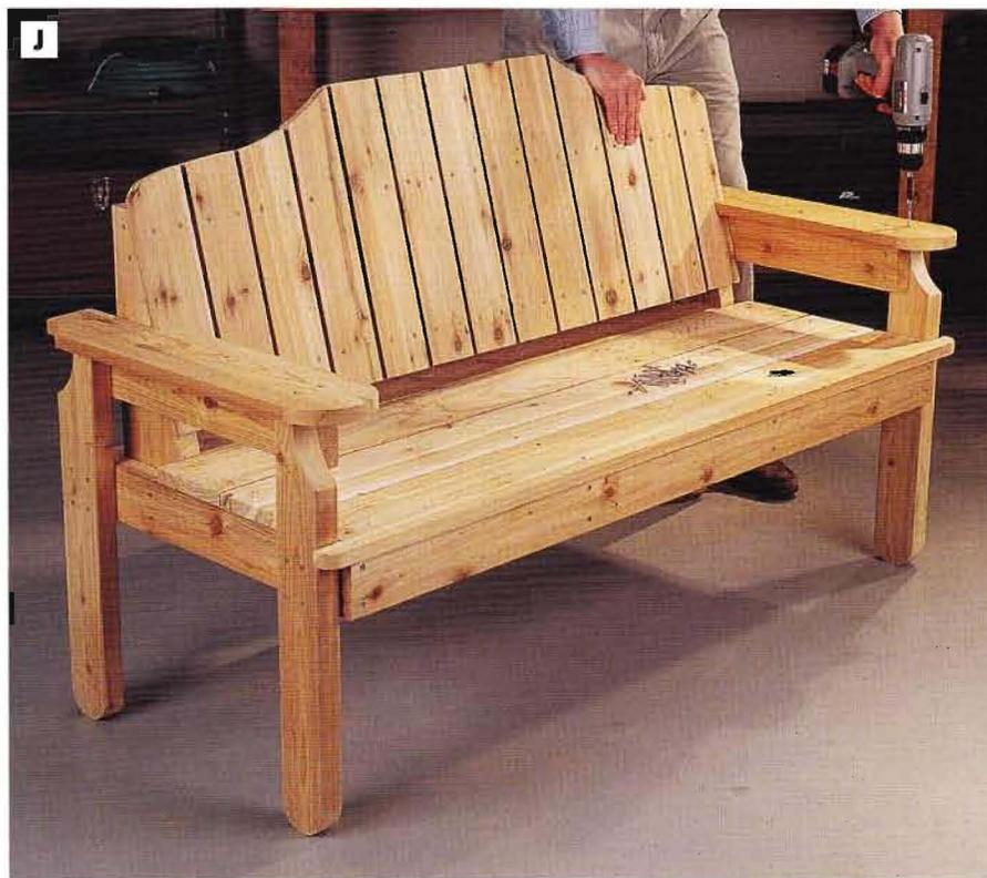
**PHOTO J:** Cut the arms to size and shape and fasten them to the arm supports with countersunk screws. You'll need to cut a small beveled notch on the back inside edges of the arms so the arms can butt tightly against the outermost back slats.
