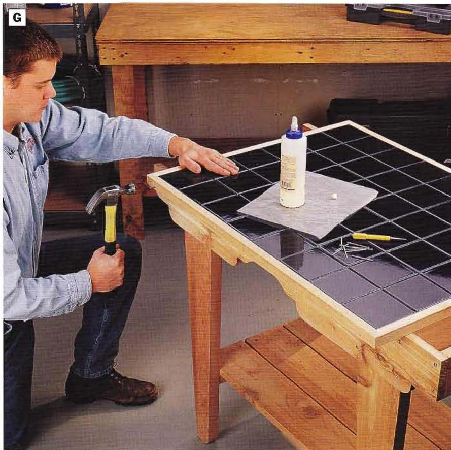
**PHOTO G:** Wrap the tile top with  $\frac{3}{4} \times 1$ -in. cedar edging, mitering the corners. Fasten the edging pieces with wood glue and 6d galvanized finish nails, nailing into the plywood subtop. Then recess the nailheads with a nailset.
