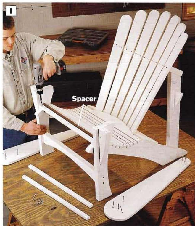
PHOTO I: Remove the arm pieces to provide clearance for attaching the seat slats. Install the seat slats along the profiled areas of the back legs starting with the shaped seat slat. Space the slats evenly apart along the back leg. A 1/4-in.-thick scrap spacer will help keep the slat spacing uniform as you install the slats.
