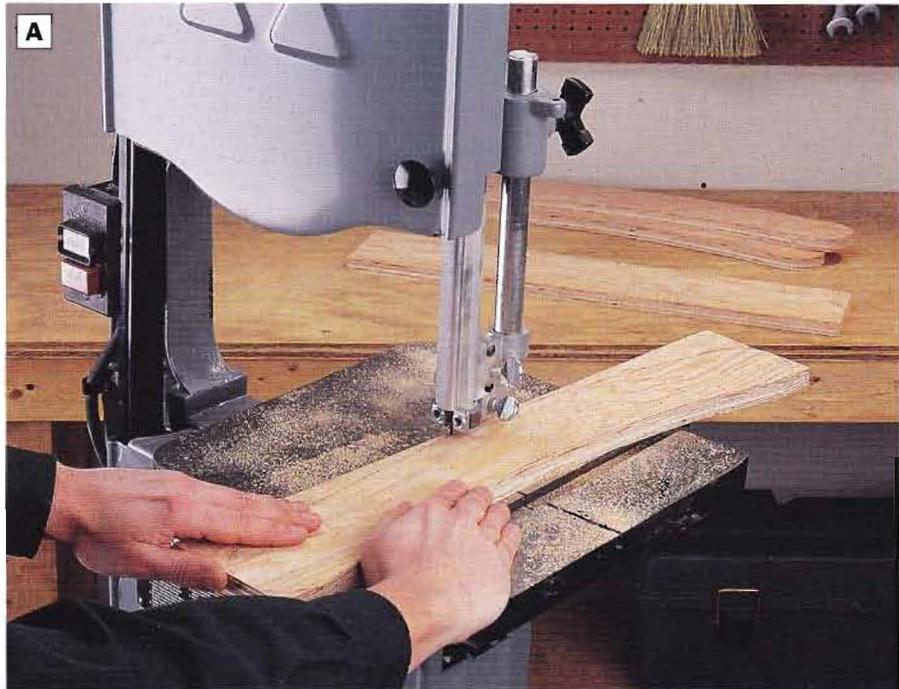
**PHOTO A:** Lay out and cut the four table legs on the band saw or with a jig saw. Since the profiles of the legs match, mark and cut one to serve as a template for tracing the profiles onto the other three leg blanks.
