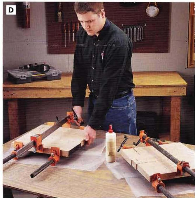
**PHOTO D:** Glue and clamp up two side panels, alternating the clamps top and bottom to distribute clamping pressure. If the boards are cut longer than necessary, don't worry if the ends don't align at this stage.
