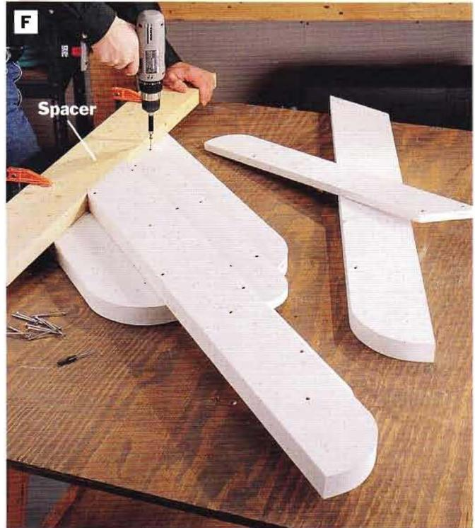
**PHOTO F:** Prime the parts for the uprights, and use a scrap 2 × 6 as a spacer to offset the outer upright parts from the center three support pieces. Drive screws through the outer pieces to build each upright.
