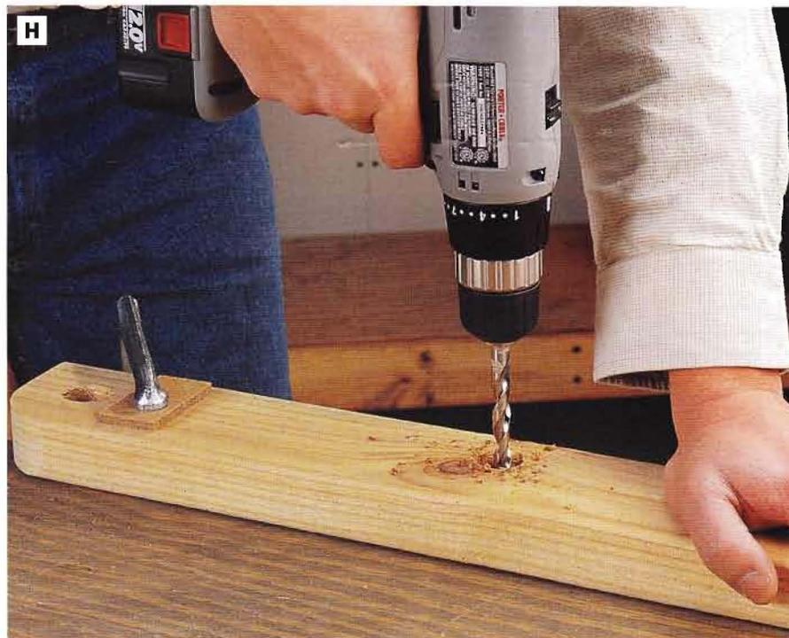
**PHOTO H:** Drill  $\frac{3}{8}$ -in.-dia. holes through the back rails, centered on the 1-in.-dia. counterbore holes. These holes will house pivot bolts for the adjustment brace that supports the chair back and holds it in one of three positions.
