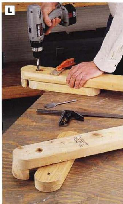
**PHOTO L:** Drill holes through the foot rest rails and the legs. The parts will attach with bolts so the legs can pivot on the rails.
