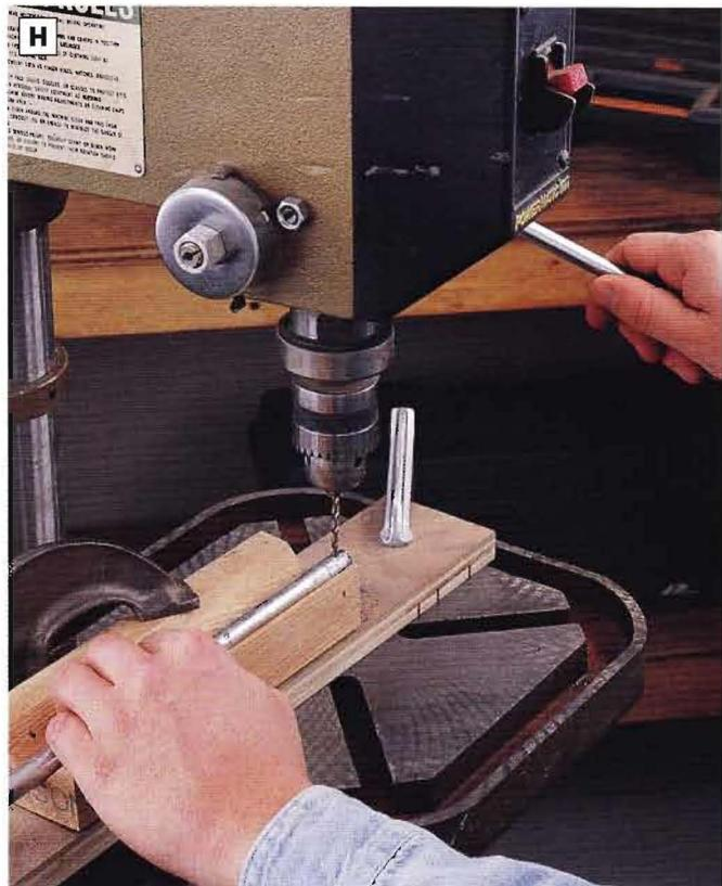
**PHOTO H:** Cut a V-shaped notch in a scrap of  $2 \times 4$  to help steady the axle as you drill holes for cotter pins. Fasten the notched cradle to another scrap, and clamp the jig to the drill press table.
