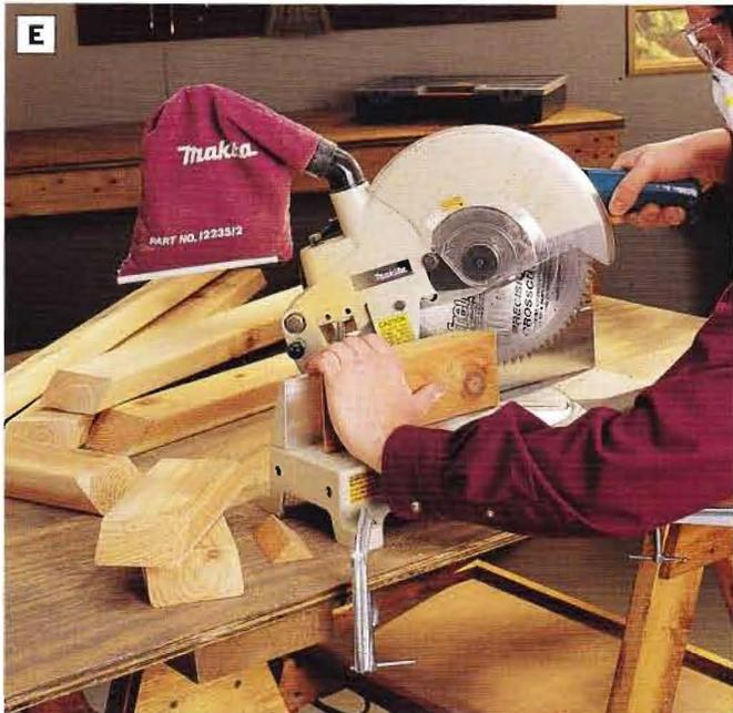
**PHOTO E:** Miter-cut the ends of the leg braces and table aprons to 45°. The safest way to make these cuts, particularly on the short leg braces, is to use a power miter saw or table saw rather than a circular saw.
