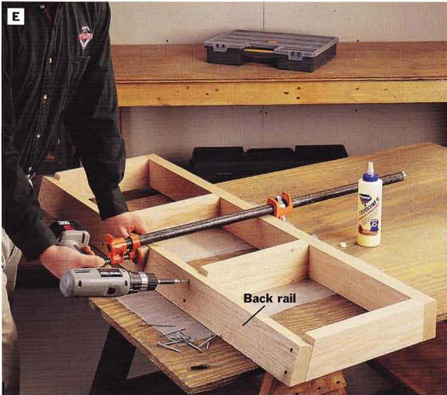
**PHOTO E:** Build the bench frame by installing four struts between the front and back bench rails with glue and screws. In this photo, the bench frame is upside down. Notice that the beveled edge of the back rail lines up with the edges of the struts, leaving an offset on the other edge.
