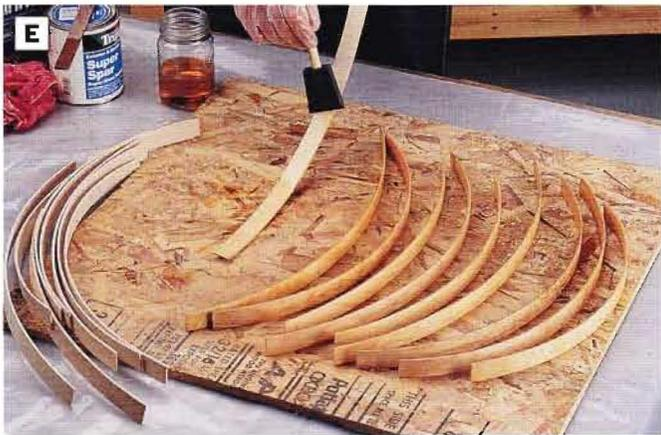
**PHOTO E:** Seal all surfaces of the seat and back weaving strips with two coats of spar varnish. Varnish the rabbets on the seat and back frames as well as the mating surfaces on the other seat and back frame.
