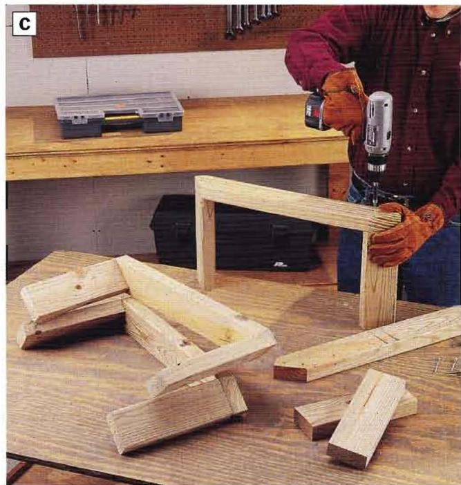
PHOTO C: Set a long seat on top of two braces, and drill countersunk pilot holes through the ends of the seat piece into the braces. Use 3-in. galvanized deck screws to secure the parts.
