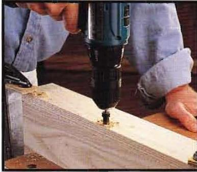
**STEP 1:** Drill a counterbored pilot hole deep enough into the wood so the counterbored portion of the hole can accommodate both the screw head and a plug.
