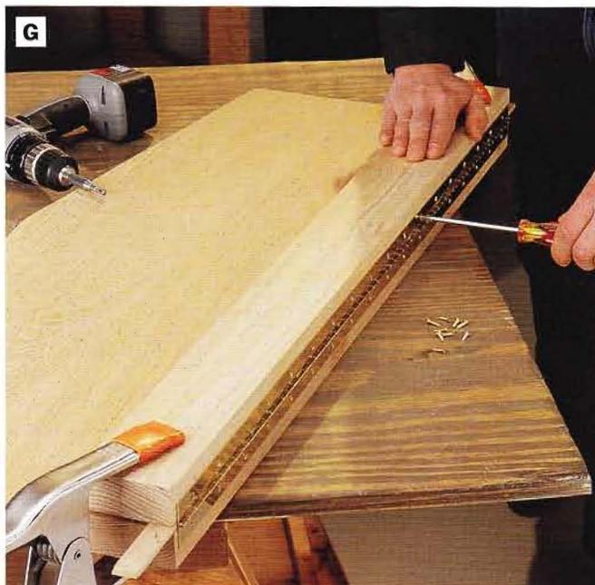
**PHOTO G:** Insert thin spacers between the fixed seat slat and the seat to provide for hinge clearance. Clamp the parts and install the hinge.
