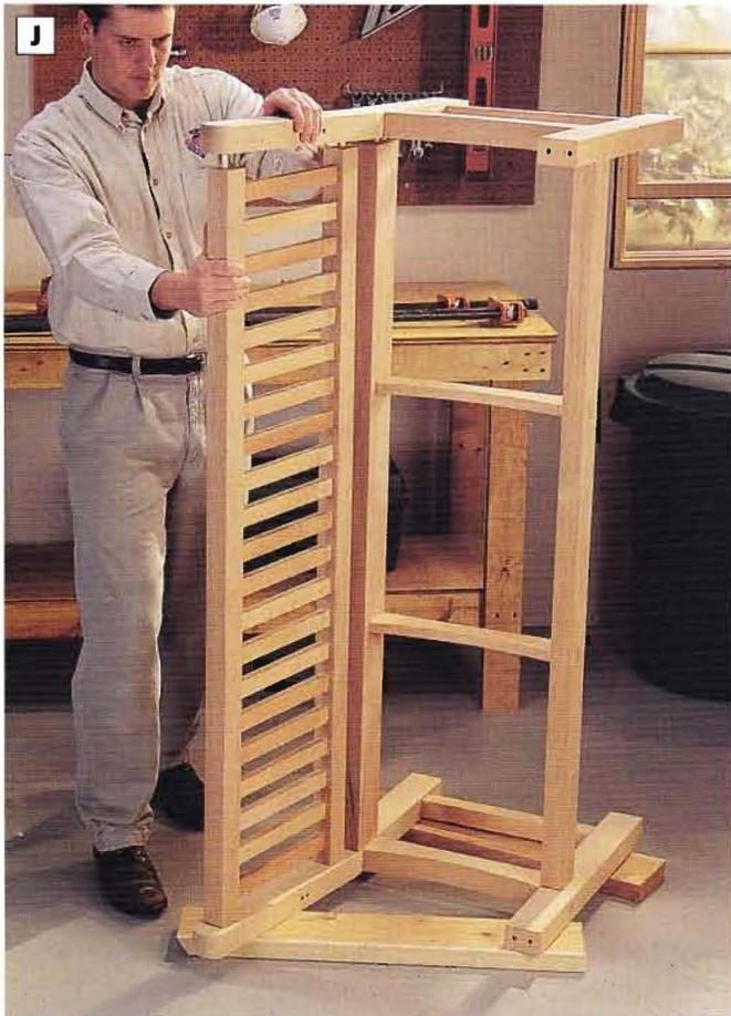
**PHOTO J:** After the rear seat slat has been attached, lay a leg assembly on the floor and set the back and seat into position. Then set the other leg assembly in place. Use glue and dowels in all the joints.
