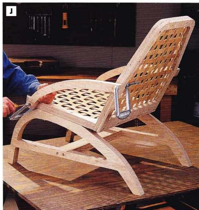
**PHOTO J:** Clamp the arm in position and connect it to the seat and back with 2-in. machine screws installed in threaded inserts.
