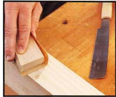
**STEP 3:** Trim any protruding portion of the wood plug flush with the surrounding wood using a flush-trimming handsaw. Then sand the plug area smooth.
