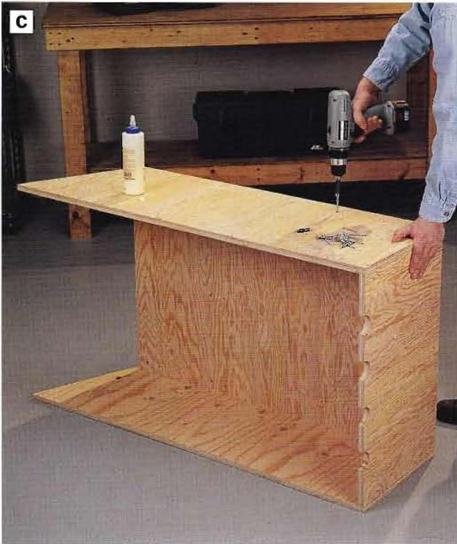
**PHOTO C:** Build the cart box. Fasten the cart back to the bottom, then screw the sides to the back and bottom. Install the cart front last. Strengthen the joints with glue when you attach the parts.
