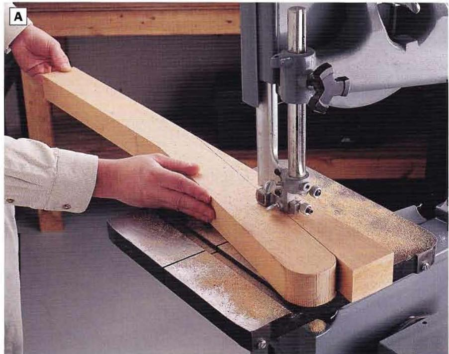
**PHOTO A:** Lay out and cut the back legs. A band saw works best for making uniform cuts in thick stock, like this mahogany. Feed the workpieces slowly through the blade, steering from both the side and the back to follow your layout lines.
