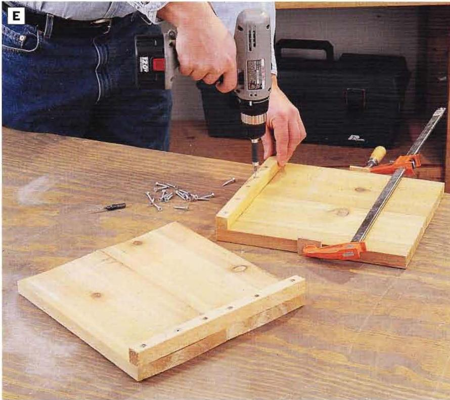
**PHOTO E:** Clamp pairs of 6-in.-wide boards for the end panels and fasten each panel together with a cleat. Use 1¼-in. galvanized screws to join the parts. These two cleats are permanent parts of the planter.
