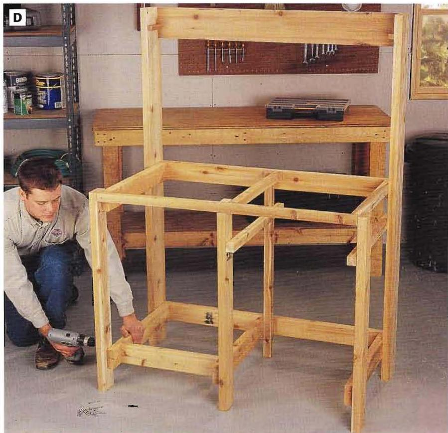
**PHOTO D:** Install the front bottom stretcher 3 in. back from the front ends of the lower stretchers to position the middle support assembly. Fasten the bottom stretcher in place, then attach the middle support assembly to the top front stretcher and back stretchers.
