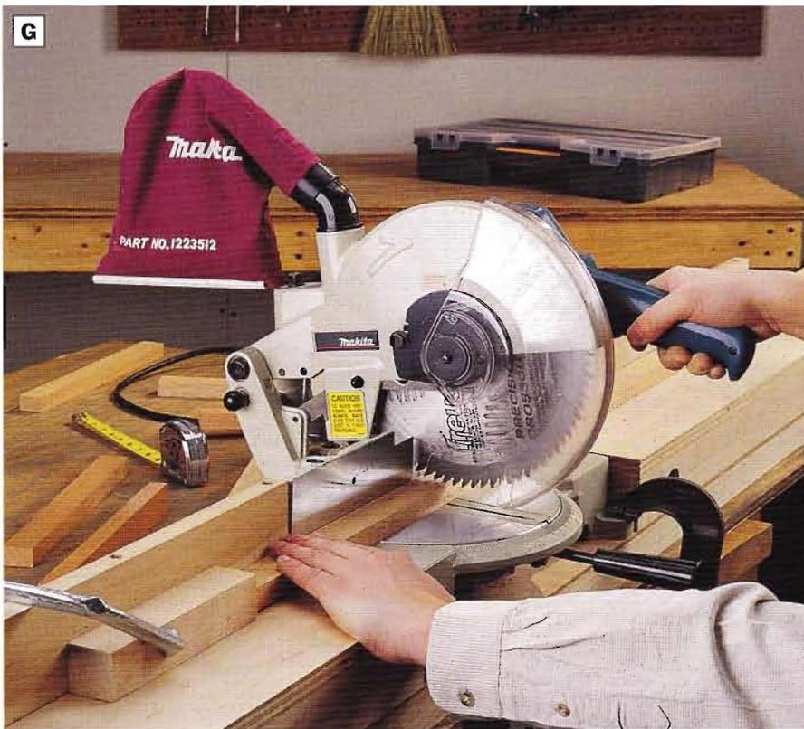
**PHOTO G:** A power miter saw makes quick work of cutting the back slats to a consistent length. Clamp a stopblock to the saw fence  $13\frac{1}{4}$  in. from the blade, and cut the slats.
