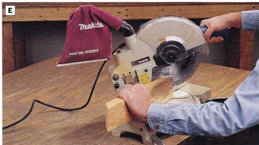
**PHOTO E:** After cutting the two corner braces to length, miter-cut the ends to  $45^\circ$ . The corner braces will fit inside the seat frames between the rails and the end cross braces.
