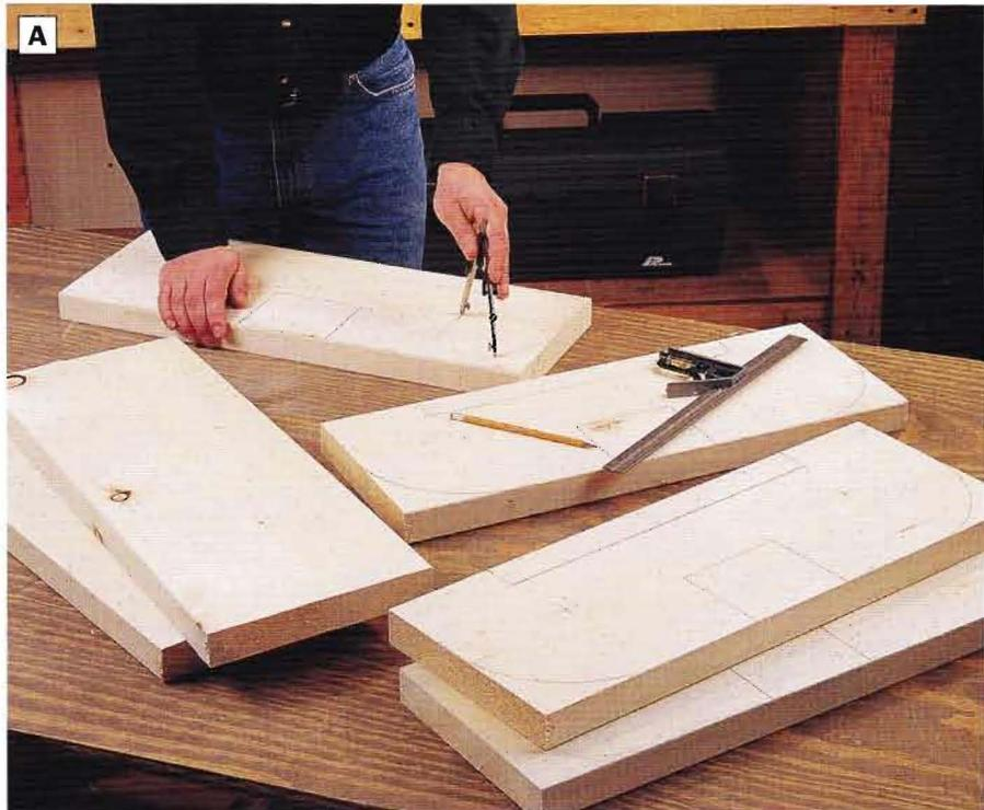
**PHOTO A:** Cut six leg blanks to size. Then use a compass and combination square to lay out the shapes of the legs on the leg blanks.
