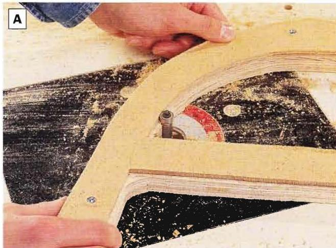
**PHOTO A:** Rough-out each leg with a jig saw, then screw a hardboard leg template to it and rout the leg flush to the template with a flush-trimming bit on the router table. Set the bit's depth so the bearing rides along the template as you rout the leg shapes.
