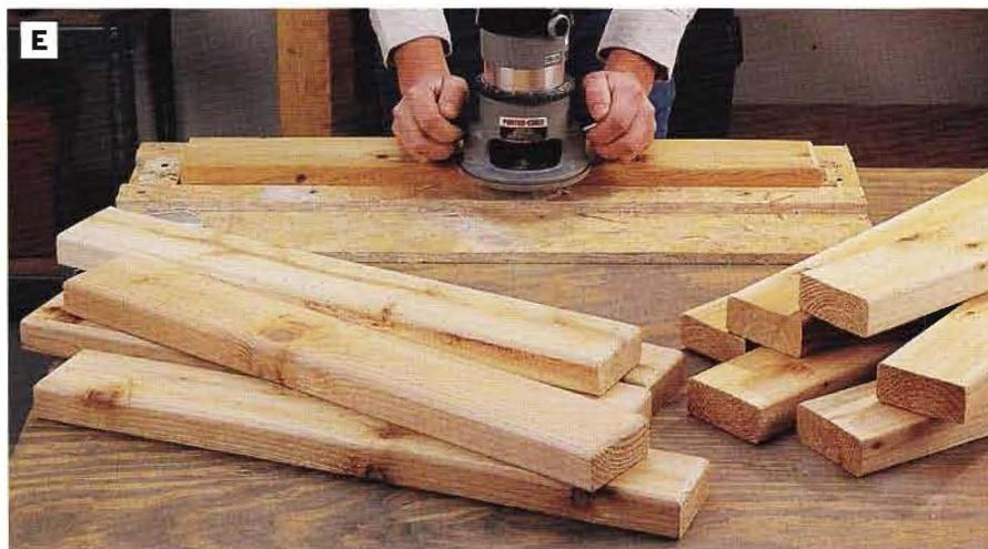
PHOTO E: Cut the 19 seat slats to length, and ease the top edges and ends of each slat with a  $\frac{1}{2}$ -in. roundover bit in the router. We used a plywood jig clamped to the benchtop to “frame” each slat on all sides and hold it steady while routing. This way, the slats require no further clamping.
