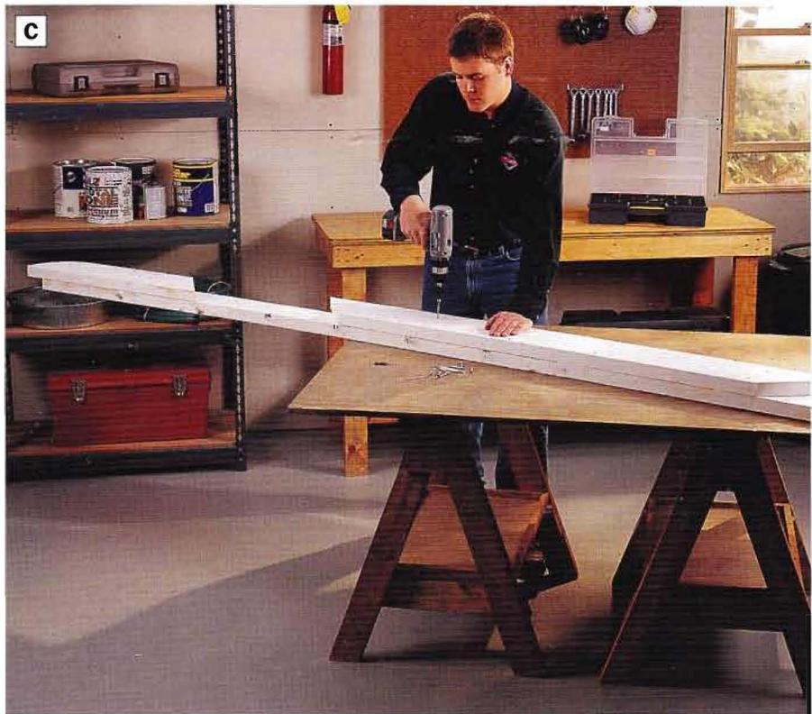
**PHOTO C:** Fasten the inner base and base ends to one outer base. Center the inner base on the outer base. Be sure to leave enough room between the inner base and base ends for the uprights. Use spacers and add ¼ in. Attach the parts with 2½-in. galvanized deck screws.
