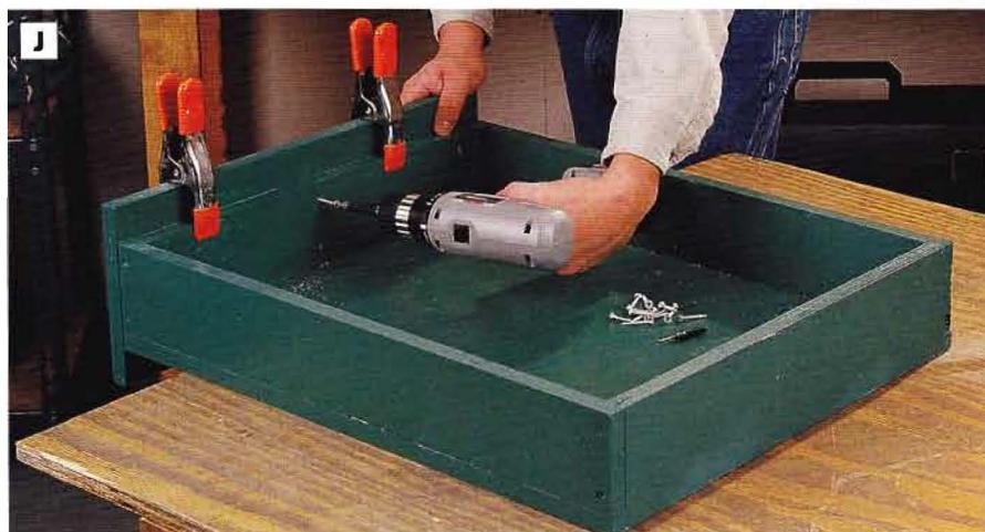
PHOTO J: Clamp the drawer face to the front of the drawer box so the ends of the drawer face are flush with the drawer sides. The face should overhang the top and bottom of the drawer by 1 1/2 in. Fasten the drawer face with 1 1/4-in. deck screws, driven from inside the drawer.
