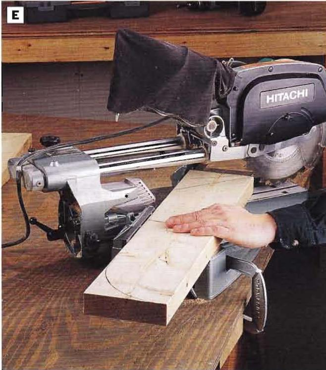
**PHOTO E:** Lay out and cut parts for the uprights. Each piece is angled to 45° on one end and has a radiused corner on the other end. A power miter saw will cut the angled ends accurately and quickly.
