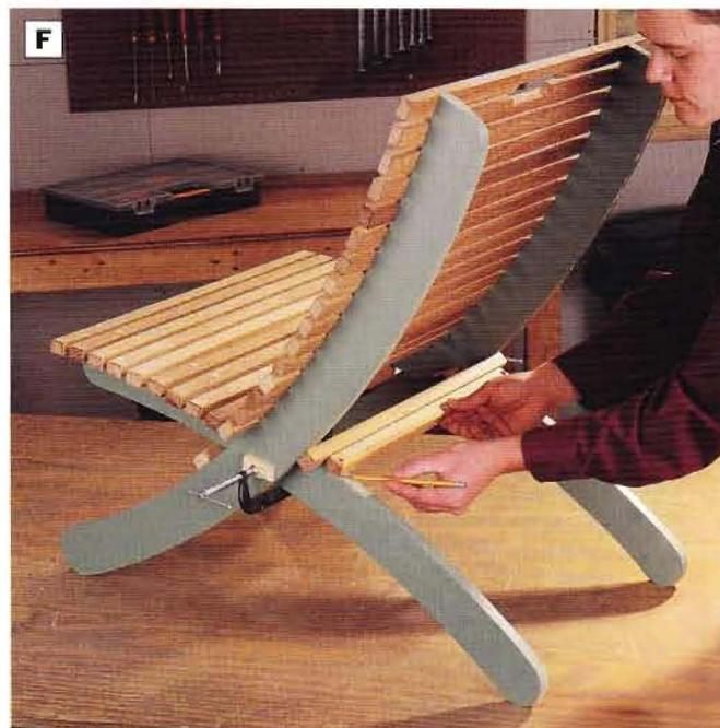
**PHOTO F:** Slide the seat assembly into the back assembly and use C-clamps to hold the chair together. Set the short crossbar against the lower long crossbar, mark its position, and install it with screws.
