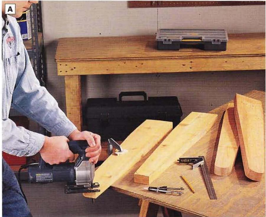
**PHOTO A:** Once you've cut the leg tapers and shortened the front legs, mark and cut the rounded feet with a jig saw. Clamp each leg to your workbench to make sawing the feet easier.
