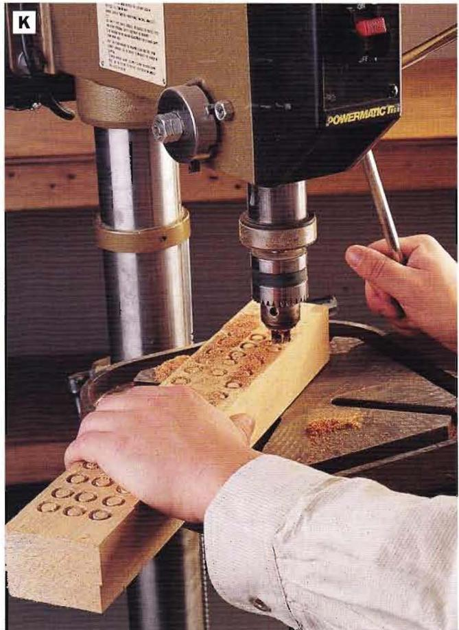
**PHOTO K:** Mount a  $\frac{3}{8}$ -in. plug cutter in your drill press to cut wood plugs for the screws. Cut about 56 plugs into the face grain of a length of mahogany. Bore the plug cutter  $\frac{1}{2}$  in. deep into the wood.
