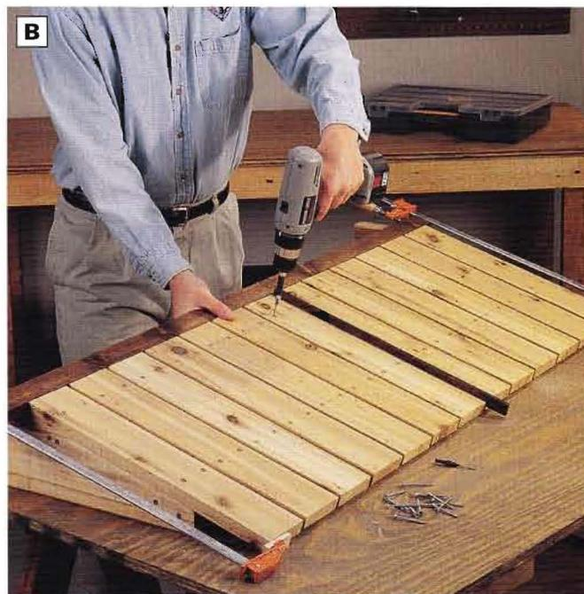
**PHOTO B:** Establish slat positions by attaching the end slats flush to the outer edges of the back supports, then clamping a straightedge across the bottom. Use a long ¾-in.-thick spacer to position the intermediate slats as you fasten them in place.
