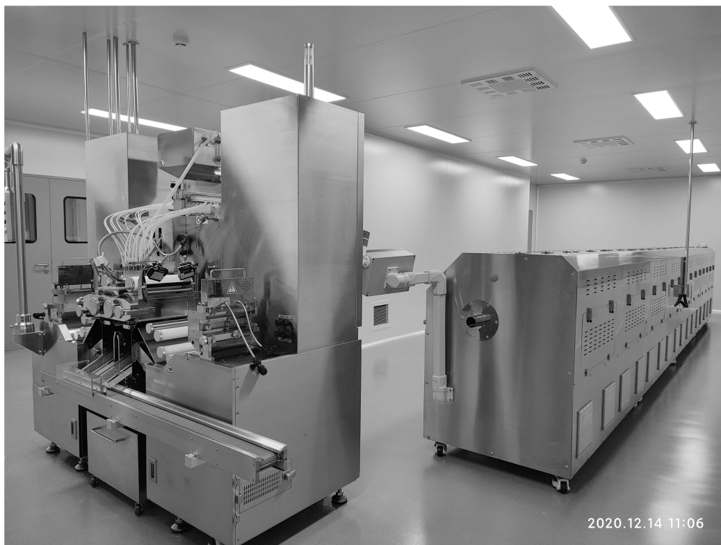
Figure 4.5 Soft-gel production line. By courtesy of GANOHERB GROUP.
