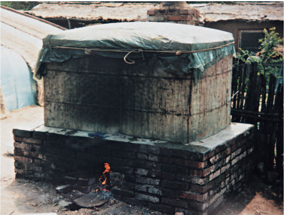
Steel tanks partly filled with water and heated with a wood fire are used in China to pasteurize loose medium or bags of medium. (Tian)
