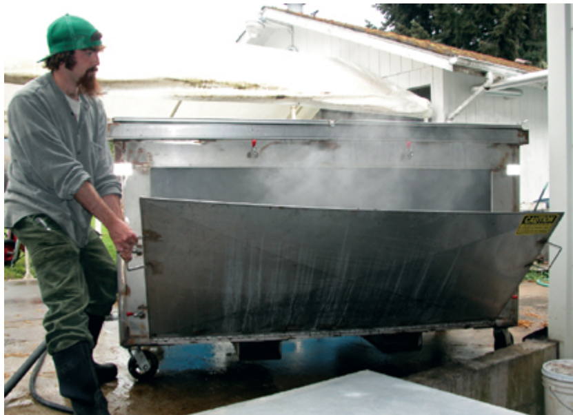
FIGURE 171 A specially designed stainless steel pasteurization chamber. Steam is injected through a port on the side. Once pasteurization is complete, the door is lowered and doubles as a ramp for unloading the straw.
