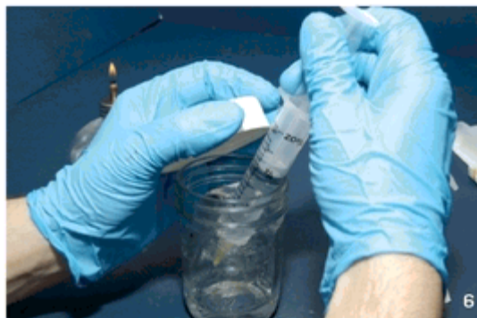
6: Filling and emptying the syringe several times to create an even distribution of spores.
