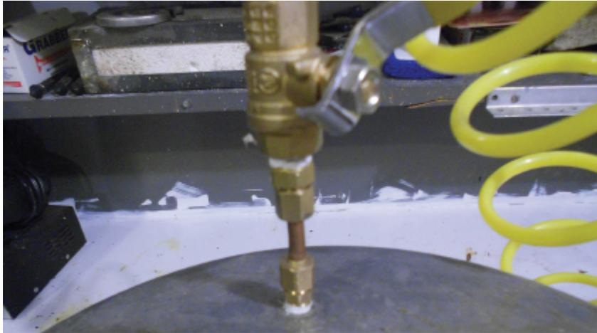
When filling the pressure cooker/boiler do not overfill it. Don't go more than  $\frac{1}{3}$  full or you could have dangerous overpressure. Believe me, just a small amount of water will run Weedeater steam conversion for a long time, especially considering this is something you cannot fire and forget. If you heat your boiler you *must* be present at all times.
