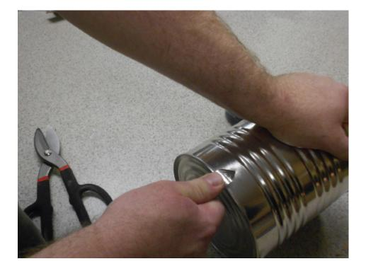
Using a can opener, punch air holes around closed end of can. (Don't punch any air holes in the side you will have toward you, or smoke will blow in your direction.)
