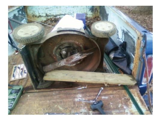
While waiting on the parts, I laid the mower on its side in the bed of my truck (being careful to keep the gas tank side up) and wedged a 2×4 between the truck bed and the mower blade to keep it from spinning while I unscrewed the blade. I did use some kerosene to loosen the nut (Liquid Wrench is almost pure kerosene).
