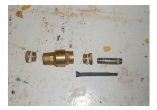
The idea is to create a single acting steam engine (meaning the steam only acts on one side of the piston) by using a pushrod inserted through the spark plug hole to push open the check valve when the piston is at Top Dead Center (TDC) so the steam will push the piston down just like the gas explosion did when it was an internal combustion engine.
