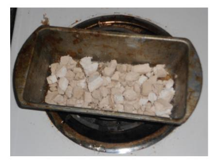
Heat the gypsum no more than two pieces deep in a pan. Alternatively, you can heat the pieces over a fire for 20 minutes or more in a pan or can heat to a dull red.
