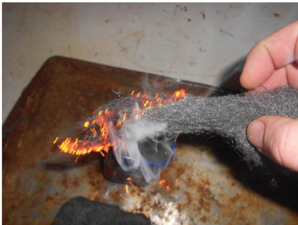
Once you have lit a fire with a lantern battery or a 9-volt battery and seen how easy it is, you can take the back off a flashlight, turn it on and use the battery and the metal flashlight case to do the same thing. Once you understand the science behind it, you can readily adapt it to other types of batteries. I have even repeated this process using cell phone batteries.
