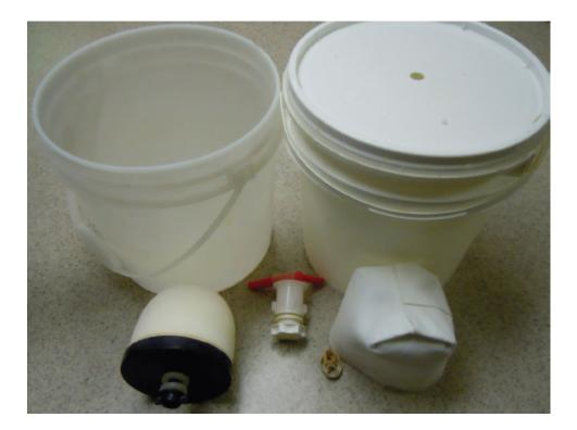
There are many ways of accomplishing the task. I used small plastic buckets from a local bakeshop, but you could use any foodsafe container of any size as long the upper bucket can sit over the top of the lower container without crushing or falling over when filled.
