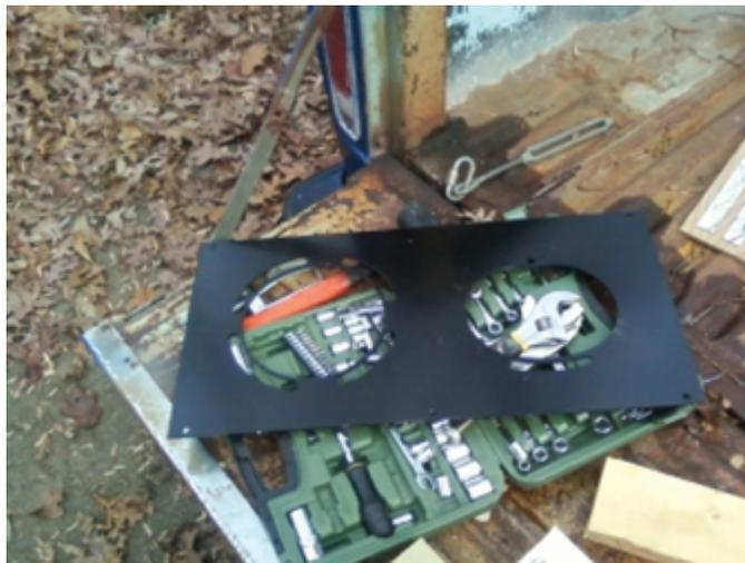
Once the plate arrived, I measured it and built a frame of scrap 2x4. The plate measured 12x24 so I cut two 2-foot lengths of 2x4 and 2 9-inch lengths. After screwing them together, it made a perfect frame.
