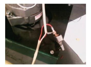
In order to use the generator, you must have a battery; this is because the voltage regulator needs to be energized to function. This generator is really just a souped-up battery charger, as the alternator's voltage regulator puts out the exact right voltage for charging car batteries. (Imagine that . . .)
