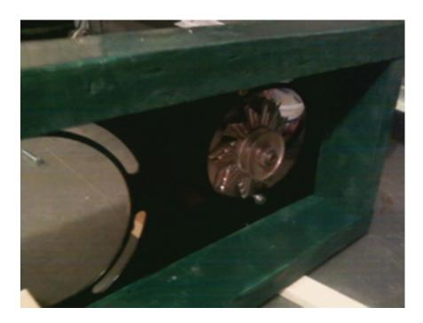
As soon as the paint dried I screwed the plate to the box and attached the alternator. It fits just like an alternator in a car. One screw fits in a whole in the plate, while a bolt fits in an adjustment slot in the plate and through the alternator and locks with a nut. To tighten the belt you loosen the bolt and move the alternator in the adjustment slot.
