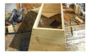
• Staple a sheet of hardware cloth to the bottom of the box. This helps with mites and temperature regulation. Depending on your climate, you may need to set the hive on a board (or otherwise enclose the bottom) in the winter to keep the hive warm.
