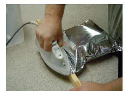
• Seal each bag, either using an impulse sealer, an iron and the bag clamp from the previous project, or the edge of a board.
