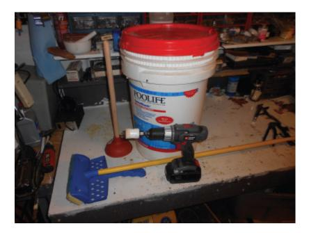
I cut a hole the size of the handle in the center of a tight-fitting bucket lid.
