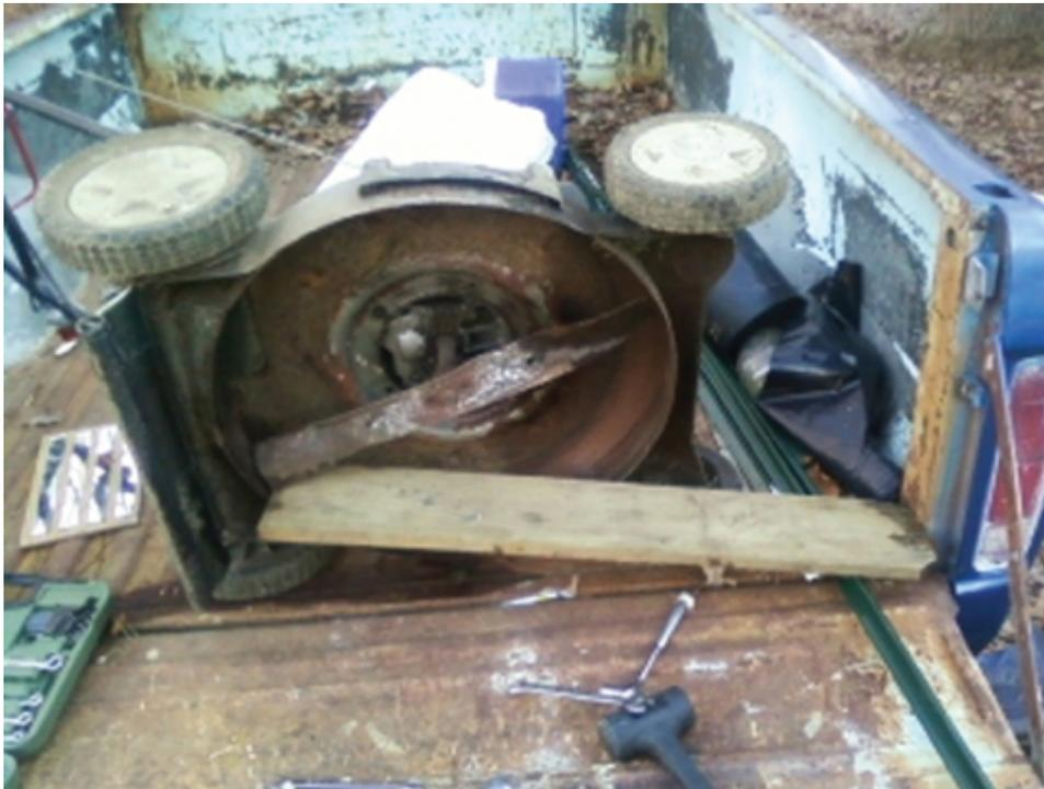
While waiting on the parts, I laid the mower on its side in the bed of my truck (being careful to keep the gas tank side up) and wedged a 2x4 between the truck bed and the mower blade to keep it from spinning while I unscrewed the blade. I did use some kerosene to loosen the nut (Liquid Wrench is almost pure kerosene).
