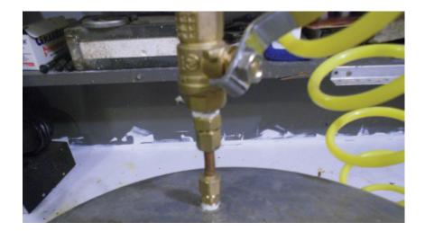
When filling the pressure cooker/boiler do not overfill it. Don't go more than <sup>1/3</sup> full or you could have dangerous overpressure. Believe me, just a small amount of water will run Weedeater steam conversion for a long time, especially considering this is something you cannot fire and forget. If you heat your boiler you *must* be present at all times.
