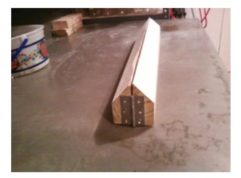
Since I made the boards longer than needed, later I plan on drilling a small hole between the two boards, so that I can insert a vacuum sealer hose inside the bag and can partially evacuate the air before sealing so that I can use a smaller and less expensive  $O_2$  absorber.
