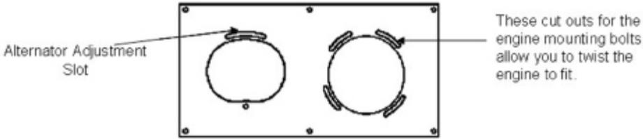
**Plate Diagram Alternator cutout on left; engine cutout on right (courtesy of the epicenter)**
