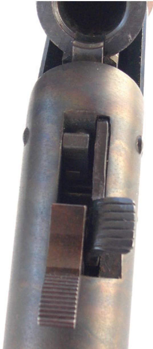
Note the transfer bar safety of the H&R shotgun.
