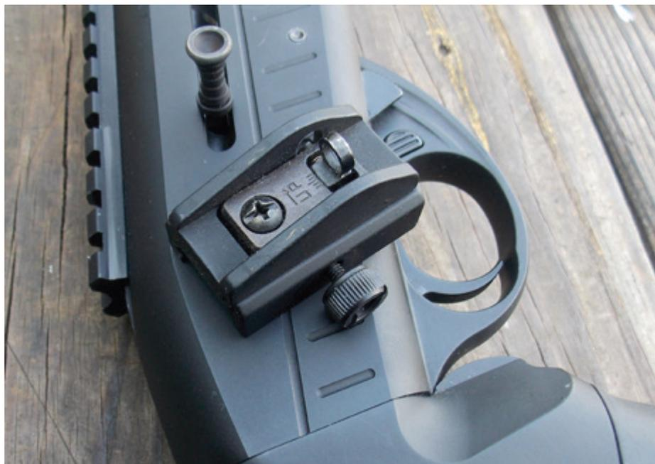
**When using aperture sights, the type that are tightened onto a rail should be checked often. These fell off the Tec-12 during a training session.**
