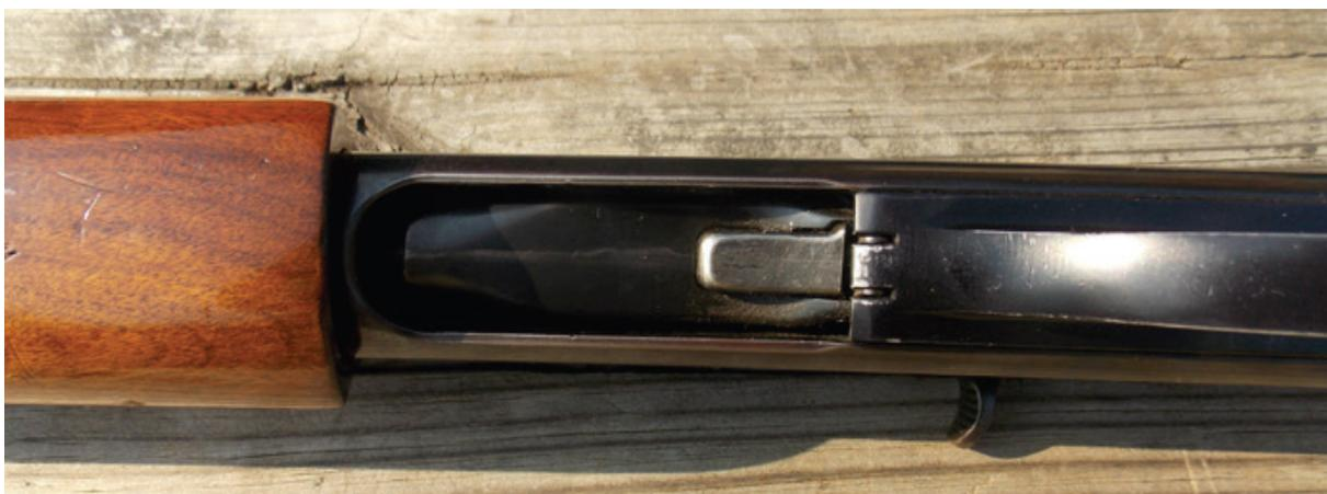
The Remington 1100 bolt release is located in the magazine well.
