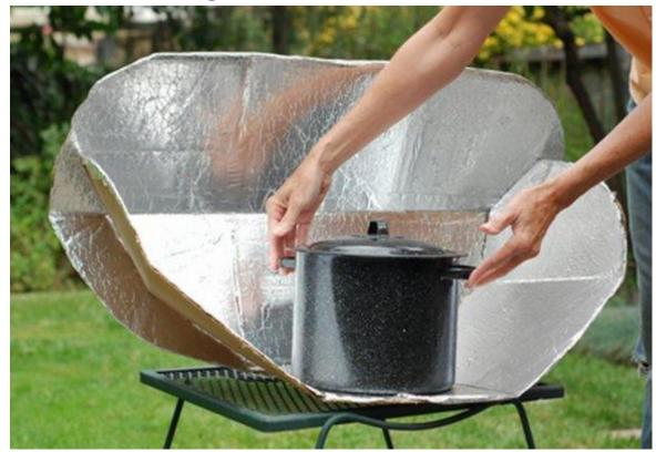
A solar cooker is often considered to be a science fair project for children. The efficiency of a solar cooker is often understated for this very fact. This solar cooker isn't simply a shoe box lined with aluminum foil—this cooker will be capable of reaching over 250F. Although not amazing compared to gas stoves, it will enable cooking without any consumption of fuel at all. Talk about resource management!
