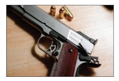
The proper condition for a 1911 is cocked and locked.
