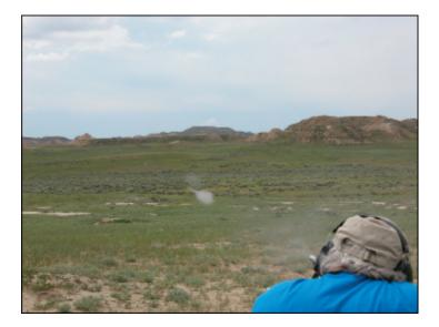
The puff of gray downrange is a bullet disintegrating in flight. This is due to hoop forces generated by too fast a spin rate for the bullet and velocity.
