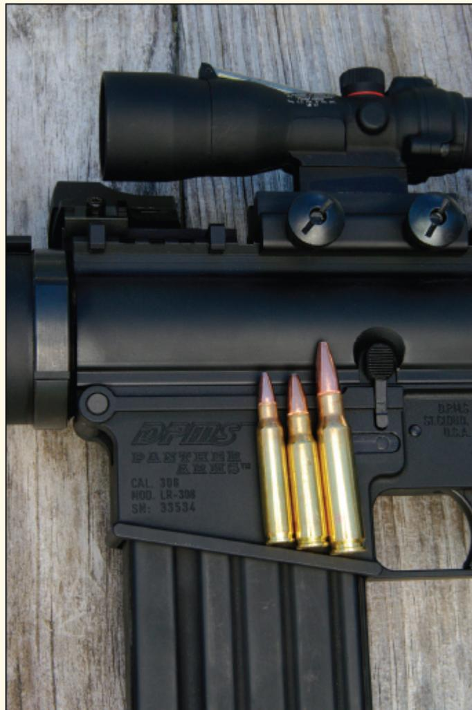
The three cartridges used in the test: .223 Remington, 6.8 SPC, and .308 Winchester.
