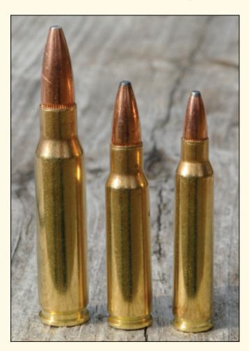
The three cartridges tested, .223 Rem, 6.8 SPC, and .308 Win. The advantages of the .308 in terms of power are obvious in the size difference.
