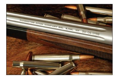
For example, a whitetail deer is similar to a man in size. The .30–06 Springfield is one of the most popular cartridges used to hunt them. With a 150-grain bullet at 2,910 ft/s, it produces 2,801 foot-pounds of energy. A 9mm 124-grain bullet at 1,150 ft/s has 364 foot-pounds of energy. So in effect we are shooting a deer with a bullet carrying 670 percent more energy than that popular self-defense cartridge carries to stop a bad guy the same size as the deer.
