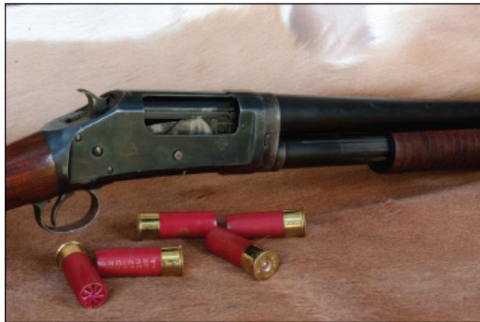
The Winchester 1897 is an early pump-action shotgun and it paved the way for today’s tactical shotguns.
