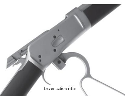
Where the bolt action has a box magazine, the lever action's magazine is tubular and positioned directly under the barrel in most cases. Depending on the make, model, and caliber, expect the capacity to be around 6 to 10 rounds. While not great for a sustained firefight, that should be plenty for most defensive encounters.
