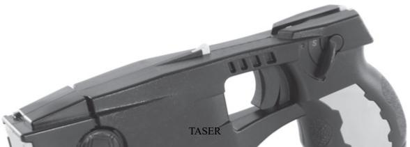
The TASER works by firing two small metal probes at the attacker. These probes are connected to the TASER unit by means of thin wires. The probes have small hooks on the ends and are designed to penetrate clothing and be difficult to remove. The user then activates the electric current, which travels through the wires to the attacker. Firing the TASER is rather intuitive as it is shaped like a handgun.
