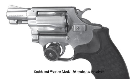
Revolvers come in three models: single action, double action, and double action only, all of which refer to the way the handgun is cocked.
