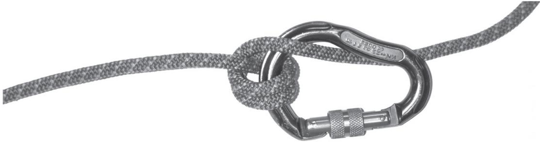
The Munter Hitch is an extremely popular hitch, but when the weight of the load is substantial, a Double Munter Hitch is often used. The extra wrap creates additional friction, allowing the weight of the load to be better controlled.
