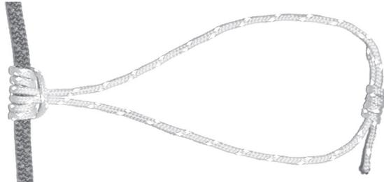
The Prusik is a simple and time-tested way to attach a smaller diameter rope to a larger diameter rope. It is used to halt the progress of rope, tie an object to a rope, or even ascend a rope by using two additional ropes. Attach two long Prusiks (about three feet each in length) to the rope you wish to climb. Place a foot in each Prusik loop and alternate sliding the loops up the main rope. It will take some coordination but in this way you can actually take steps up a rope.
