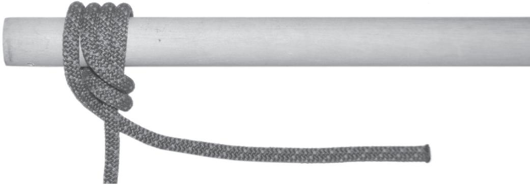
This hitch is popular in a variety of professions from longshoremen to theater stagehands. It is secure yet never completely tightens, which allows it to be quickly and easily untied. This hitch is unique in that no “knot” is actually tied. It uses friction wraps to withstand the load. The hitch can be loosened by unwrapping it, thus allowing the load to be lowered if desired.
