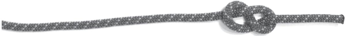
The Figure Eight Stopper Knot, or the “Figure Eight” as it is usually referred to, is a simple stopper knot that is often used by sailors and climbers to prevent rope from pulling through rope bags, pulleys, or the eyelets of sails. It also serves as the basis for several other knots.
