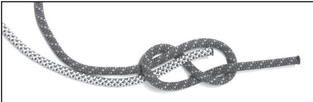
**5** Trace the second rope along the first until it also forms a figure eight parallel to the first.
