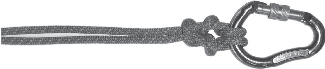
An extremely strong hitch often used by dock workers, the Cat's Paw can be tied in the middle of a rope and placed over a rail or post. One of the main benefits of using the Cat's Paw is that, in theory, one of the weighted ends of the rope could break and the Cat's Paw would cinch down and hold the load in place with the remaining intact side of the rope.
