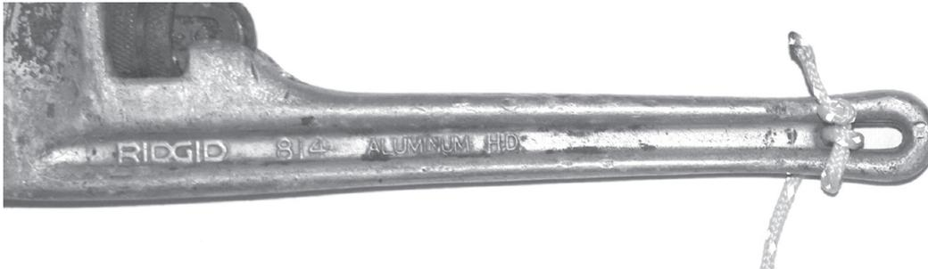
Another simple and handy way to attach a lanyard to an object is the Knute Hitch.
