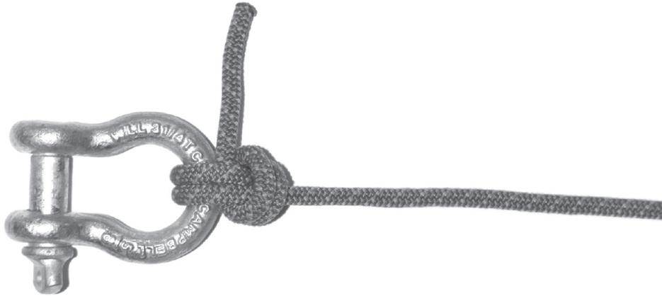
This variation of the Anchor Bend dates back to the early 1900s. It is an easy-to-tie and secure way to attach a rope to an anchor point.
