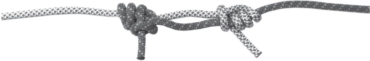
The Adjustable Bend Knot is a slide-and-grip knot that will slide along the rope and absorb the energy created by the momentum of a fall. The knots will slide along the rope as they grip tighter until they are coupled.
