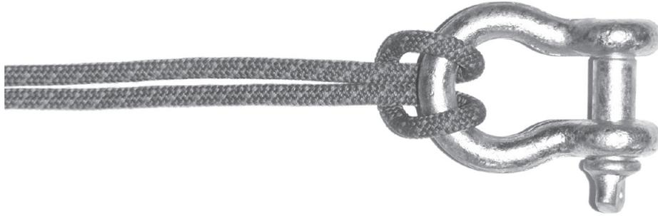
This hitch is most often used to attach an object to a lanyard. A piece of jewelry, a knife, a flashlight, or any other item can be secured with this simple hitch.
