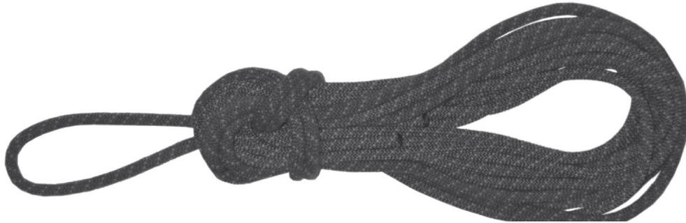
This coiling method is quick, easy, and simple to untie when the rope is needed in a hurry. You expedite the process by doubling the rope prior to coiling, and it ends up with a practical loop for hanging.
