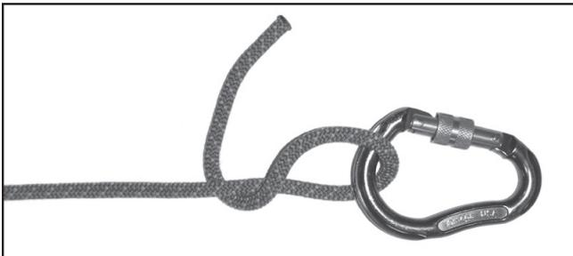
**3** Pass the working end across the loop that has been formed.
