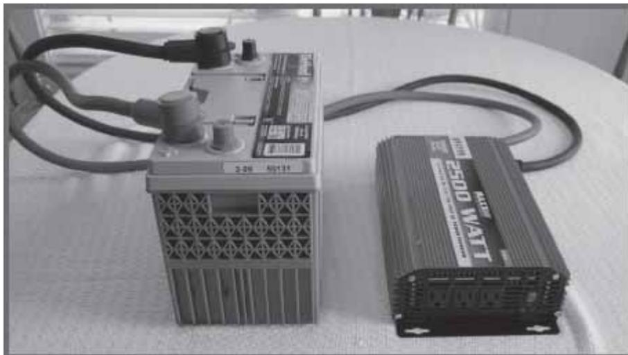
**A deep cycle lead-acid battery connected to a 2,500-watt inverter**
