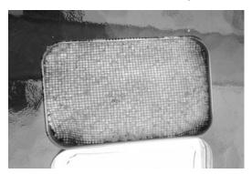
**#4** Carefully pour the alcohol directly onto the screen. You don't need a lot; just 3 tablespoons will suffice in most cases. After closing your fuel bottle and placing it well away from the tin, light a match and place it directly onto the screen. The alcohol fumes should light instantly. Be advised, alcohol burns very hot and the flame can be difficult to see. If you aren't sure whether the stove lit or not, slowly move your palm near the stove to feel for heat.
