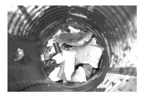
**#2** Once the water is just below boiling, put the can in the pot. If need be, add a little more wax to keep the can from floating up. Keep the water at a steady simmer. While you won't "burn" the wax by having the heat too high, a rolling boil will bounce the can around.
