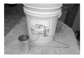
**#1** Drill two small holes near the rim of the bucket, directly across from one another. The holes only need to be large enough for the wire hanger to fit through.
