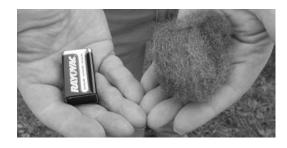
**#1** For this project, all you do is connect the positive and negative battery terminals with a piece of steel wool. The wool will quickly begin to heat, glow, and flame up.
