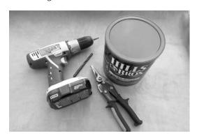
**#1** It should go without saying, but your metal can should be empty and clean. It doesn't need to be spotless, but it should be washed out reasonably well. With your safety goggles and work gloves on, start by drilling some air holes in the can. This doesn't require Pythagorean precision, but the holes should be roughly equidistant from each other. Make two rows of holes, one about 2 inches from the bottom and another about 2 inches from the top. You only need about six holes in each row.
