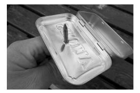
**#3** Slide the wick through the hole, leaving an inch or less exposed above the lid. The wick should be long enough such that about 3 inches or so of it will coil up into the oil under the lid.
