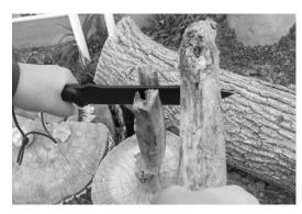
**#4** Once the blade bites into the wood completely, concentrate your blows on the exposed part of the blade. Slowly, you'll drive the blade all the way through the wood, splitting it in half.
