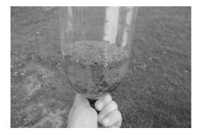
**#5** Finally, add a layer of gravel. This layer should also be roughly 2 inches thick. Nothing fancy is needed, no special kind of gravel, but smaller stones are better than larger ones. Just collect a couple of handfuls from the ground, rinse them off, and toss them into the bottle.
