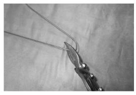
**#4** Run the wire hanger through the two holes, threading it through the soup can. Bend the ends of the wire hanger on the outside of the bucket.
