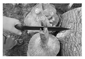
**#3** Hold the knife handle in one hand and firmly hammer on the knife blade with the other.
