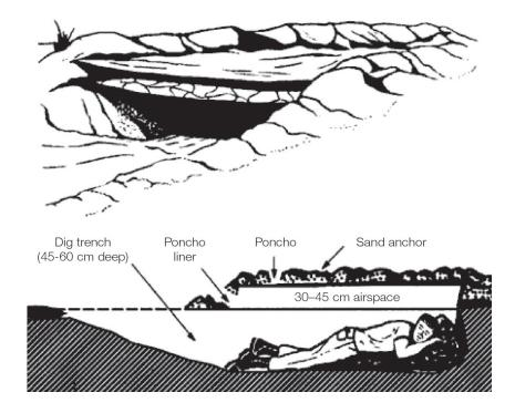
If you have extra material, you can further decrease the midday temperature in the trench by securing the additional material 30 to 45 centimeters (12 to 18 inches) above the first. This layering of the material will reduce the inside temperature. White is the best color to reflect heat; the innermost layer should be of darker material.
