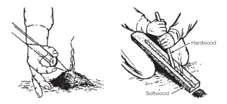
Fire-starting methods: lens (left) and fire-plow (right)
