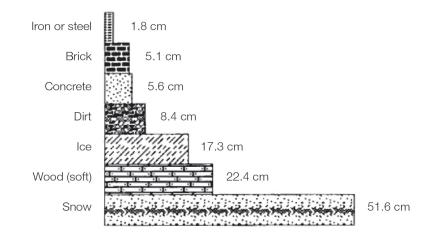
Thickness of materials needed to reduce residual gamma radiation transmission by 50 percent
