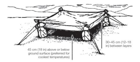
**Note:** If you have enough material, fold it in half and form a 30- to 45centimeter (about 12- to 18-inch) airspace between the two halves. This airspace will reduce the temperature in the shelter.
