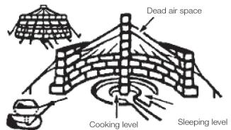
Suspension line tie-downs go through hole, are watered down, and freeze in place.
