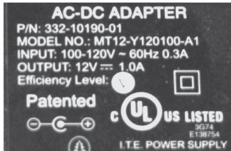
Look at the line that starts with “output.” See the “12V”? That means that this power pack takes the 120 volts AC from the wall and converts it to 12 volts for the device it powers. Notice that little symbol next to the 12V with the solid line over the dashed line. That symbol means the 12 volts is *direct* current, not alternating. And finally, the “1.0A” means it can provide a maximum of 1.0 amps.
