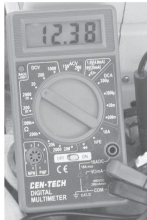
Voltmeter showing battery voltage reading
