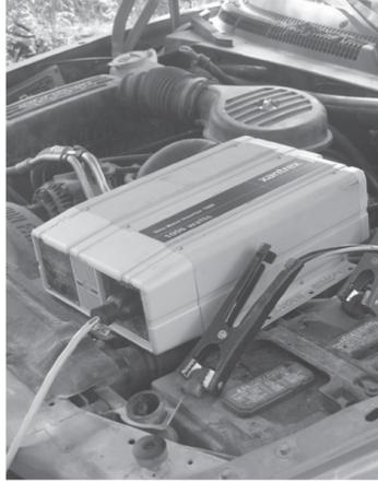
Inverter cables connected to car battery
