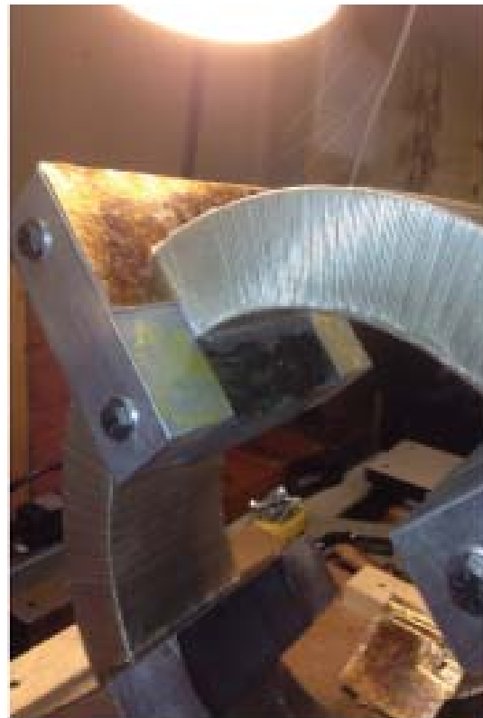
Installing cut mica plates
