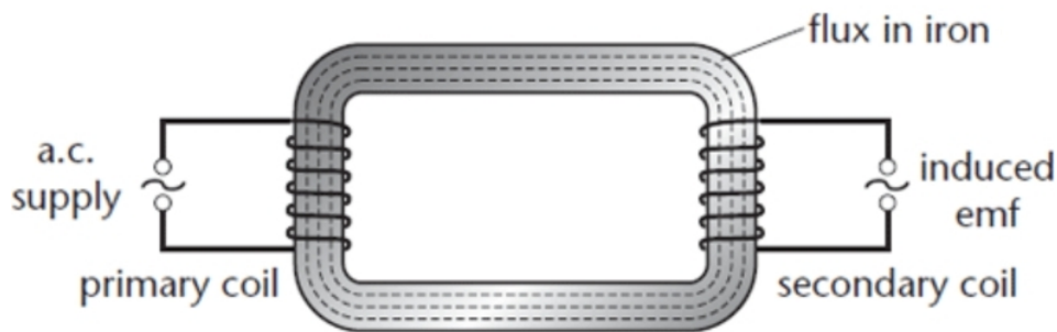
Flux linking two transformer coils
