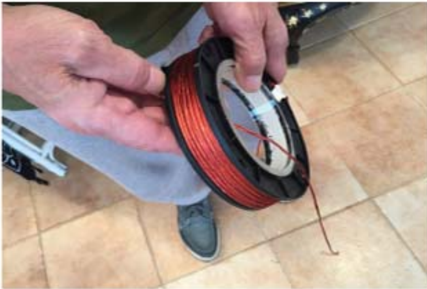
Exciter Coil with Litz wire
