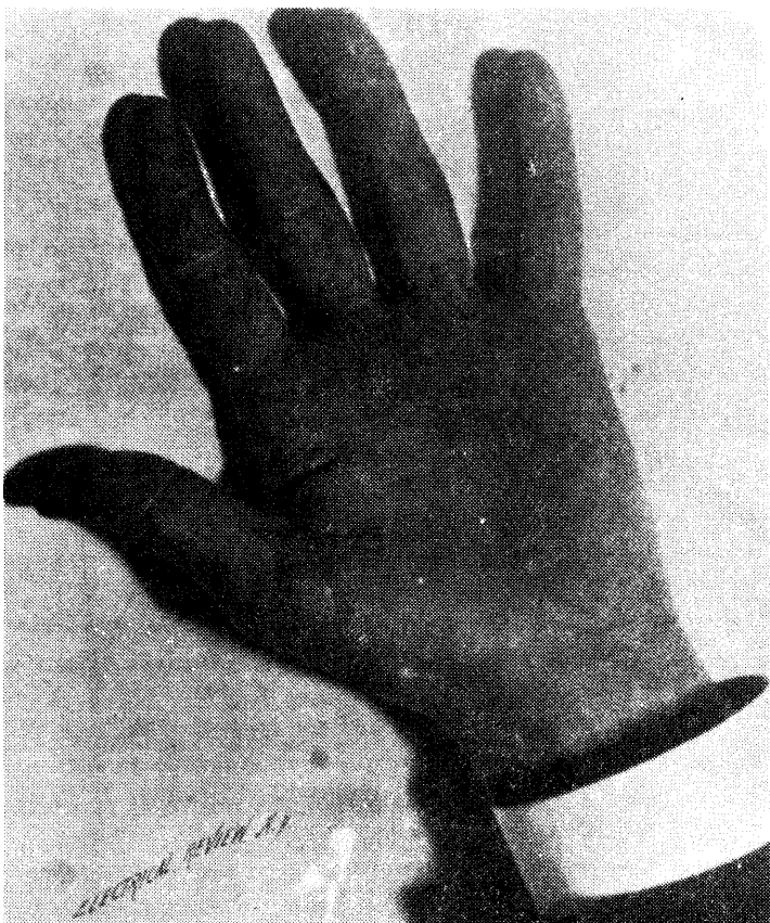
PHOTOGRAPH OF THE EXPERIMENTER'S HAND MADE BY THE LIGHT OF A SINGLE IMPROVED VACUUM TUBE OF 1,000 CANDLES. EXPOSURE TWO SECONDS; DISTANCE FROM THE TUBE FOUR FEET.
